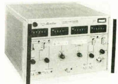
ator, which provides full-sweep coverage of L, S, C, X, and Ku bands in a single-range, self-contained instrument. The unit makes it possible to use a single setup to test over the range from 1 to 18 gigahertz or over any combinations of selected portions of these ranges.
