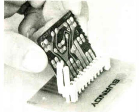
Although it is gold-free, a zero-entry-force printed-circuit connector developed by Burndy Corporation promises contact features usually attributed only to gold. The socket employs the Burndy gas-tight high-pressure technique introduced in a leadless IC receptacle [*Electronics*, Dec. 4, 1972, p. 139]. The contacts of the new connector have sharp points which displace the oxides on the mating tabs of the printed circuit board and thereby develop a reliable interface.
