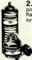
**2. TEMPILAQ<sup>®</sup>:** materials of calibrated melting points suspended in an inert, volatile non-flammable vehicle. Available in over 100 systematically spaced temperature ratings from 100° to 2500°F. TempilAQ indicates its temperature rating by liquefying within  $\pm 1\%$  of its rating. Available in bottles or spray cans.
