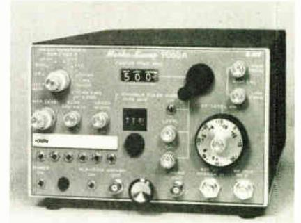
continuously variable sweep-width control. Sweep repetition is alterable from 1 sweep per 10 seconds to 100 sweeps per second, and sweep duration (or scan rate) can be set from 2 to 5 milliseconds, thus permitting use in sweep-testing of CATV systems. Price is \$1,150.
