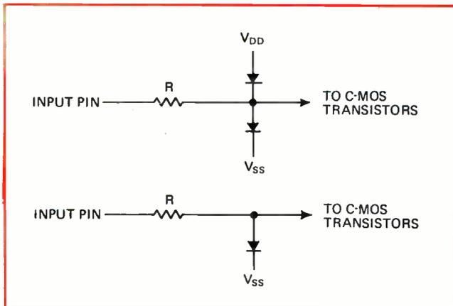
**4. On guard.** All C-MOS devices require input protection against damage from static charges during handling. Typical one- and two-diode schemes are shown here. The designer should not count on these diodes for his special circuits because different manufacturers use different protection schemes.
