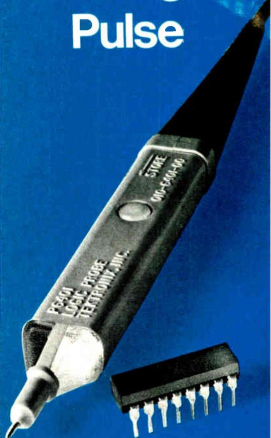
The TEKTRONIX P6401 Logic Probe positively identifies logic states (high, low, abnormal, open, over voltage) of TTL and DTL circuitry. No level setting or adjustments; just touch and see.
