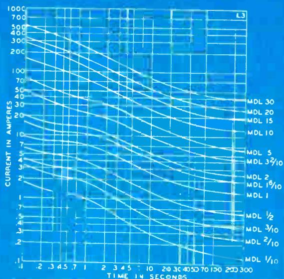
Time-current characteristics of BUSS® fast-acting fuses
