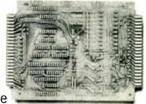
**3.** Loaded-Board Testing. Our circuit test systems with "guided-probe" troubleshooting allow technically unskilled operators to pinpoint errors quickly and reliably. This means you no longer need to use valuable technicians for chasing down routine soldering and insertion errors.
