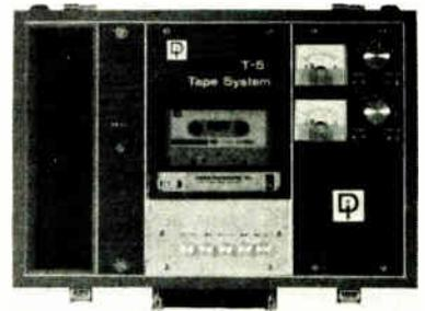
In the fm mode its passband extends from dc to 1,000 hertz; in the direct mode it covers 100 to 10,000 Hz. The T5-2 sells for \$2,700; delivery time is six to eight weeks.
