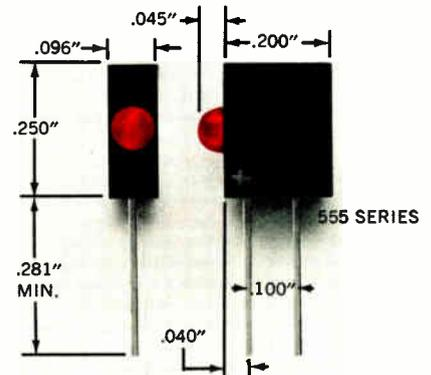
LED logic state fault indicators available in 14 models with voltage ratings from 1.7 to 14. Suitable for dense packaging on printed circuit boards—up to 10 units to the inch—IC compatible. With built-in series resistor. Polarity identified. Low power consumption.
