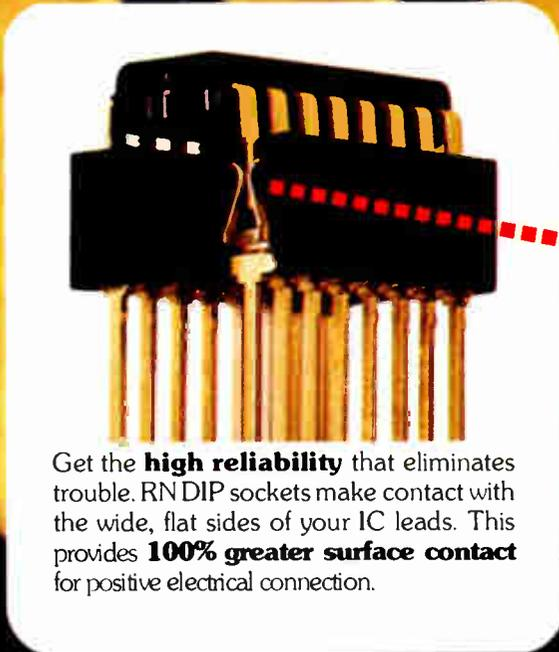
Get the **high reliability** that eliminates trouble. RNDIP sockets make contact with the wide, flat sides of your IC leads. This provides **100% greater surface contact** for positive electrical connection.
