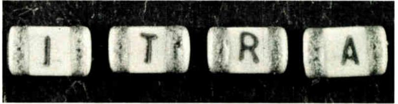
For the most part, all tiny chip capacitors look alike. But chips of the same size can have different capacitance values, as well as different tolerances. And if accidentally mixed together, as can easily happen on the production floor or in the stock room, there is no simple way to sort them without measuring the capacitance of every chip.
