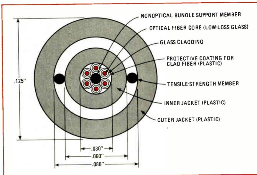
**Conductor.** Forward-area Army communications may soon be relying on fiber-optic cables only 0.125 mils in diameter to carry voice messages and digital signals.
