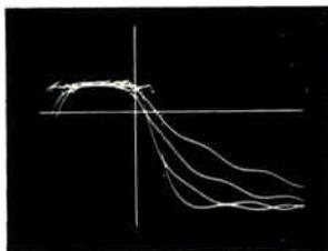
The 1090 offers numerical readout of any selected data point. Selection is made with an easily moved cursor. Wherever the vertical cursor intercepts the waveform the alphanumeric readout on the CRT displays time from trigger and voltage
