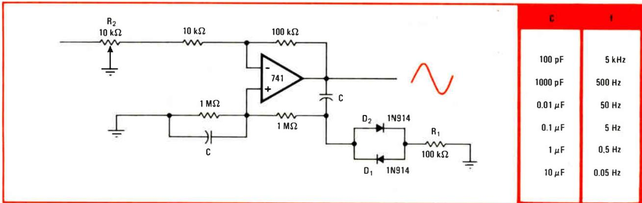
**Stabilizer.** Front-to-back diodes in oscillator's feedback path acts as stabilizer, yet do not cause hunting or distortion, as lamps or zeners sometimes do. Capacitors, which control frequency, are matched; amplitude control is by potentiometer, which also affects frequency.
