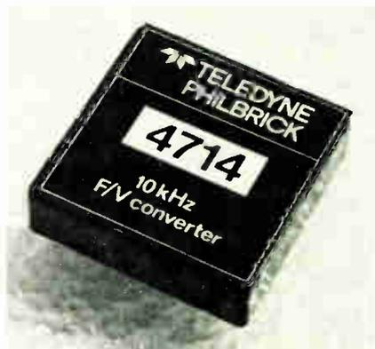
making it suitable for use in low-cost fm demodulation equipment as well as in wide-range frequency monitors. The input, which is compatible with transistor-transistor and diode-transistor logic, represents less than one TTL load and requires pulse widths of at least 20 microseconds for the converter to achieve
