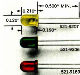
Your choice of green, yellow and red, with axial leads for dense packaging requirements. Wide viewing angle for easy readability. Low power consumption, low cost, IC compatible. 10mA operation for typical brightness. Size is identical to the most popular red LEDs.
