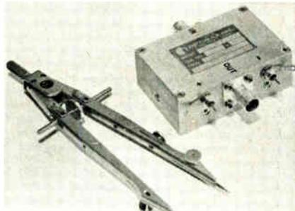
3-inch by 2-inch by 1.02-inch module requires a maximum of 180 milliamperes at 20 v dc for its primary power, and can put out +28 dBm (at the 1-dB compression point). The amplifier comes with a choice of BNC or SMA connectors. Small-quantity delivery time is 30 to 45 days.
