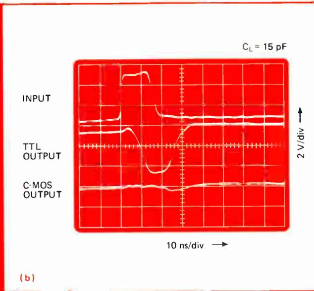
**1. Voltage-noise Immunity.** Sharp transfer characteristic (a) of a C-MOS gate accounts for this device's superior voltage-noise immunity over a TTL gate. C-MOS ac-noise immunity is better, too. As shown in (b), a C-MOS gate will reject a 15-nanosecond pulse, while a TTL gate will transmit it. A TTL gate will also pass 25-megahertz noise (b), whereas a C-MOS gate will not.
