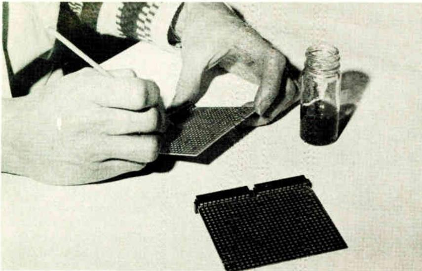
**Mask-maker.** Brushing and screening are two of several methods by which new water-soluble masking materials can be applied to printed-circuit boards. The materials keep solder away from selected areas as the board moves through a wave-solder machine.
