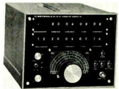
covers 1 to 25 megahertz in four ranges. Character-rate and vertical and horizontal blanking signals are provided through two rear connectors to permit interfacing the instrument with character-generating read-only memories and other user-supplied equipment.
