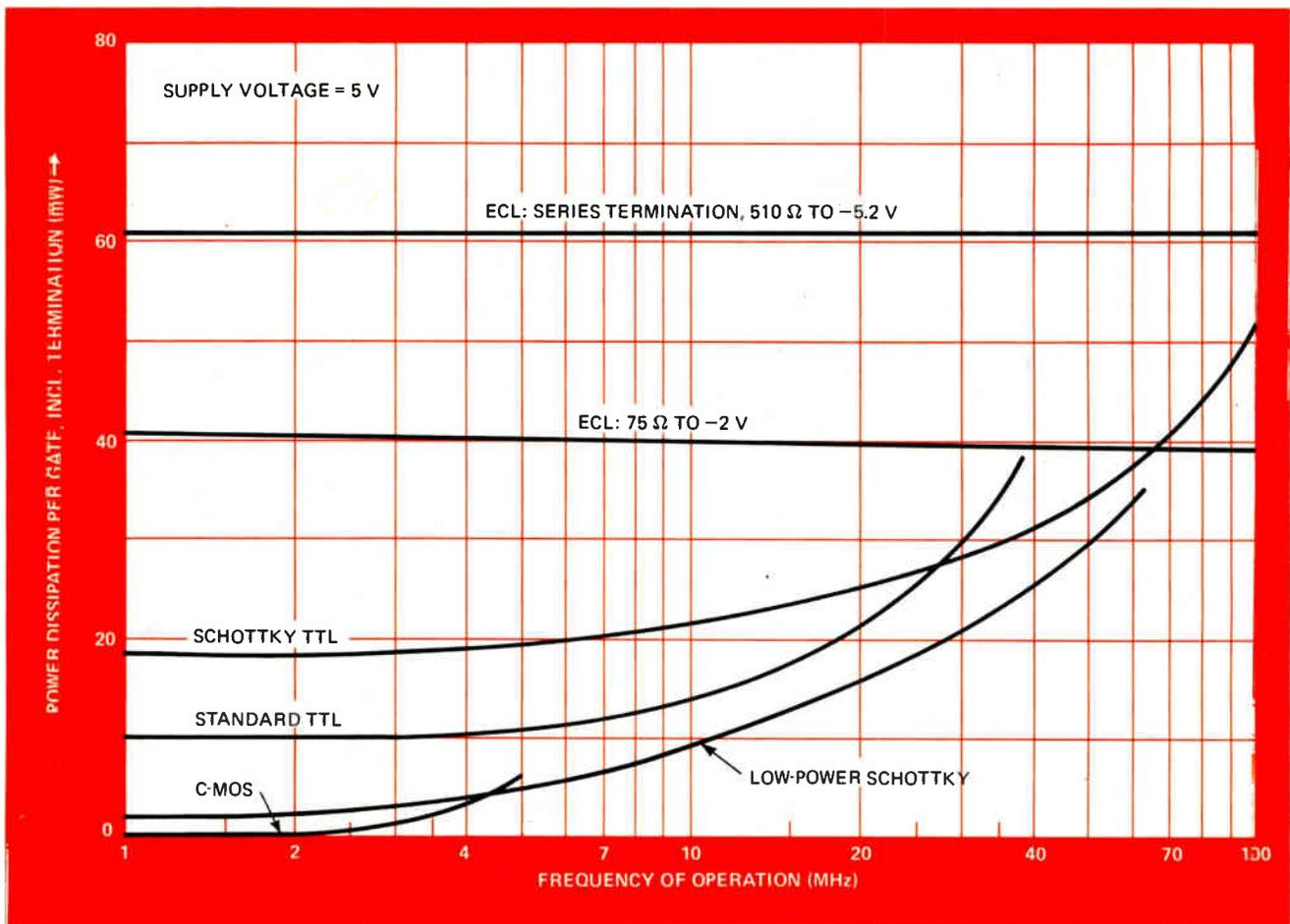
**3. Power comparison.** Probably the principal advantage of C-MOS is its exceptionally low power dissipation, which is significantly below that of any other commercial logic family. The power dissipation of a C-MOS device depends principally on operating frequency.
