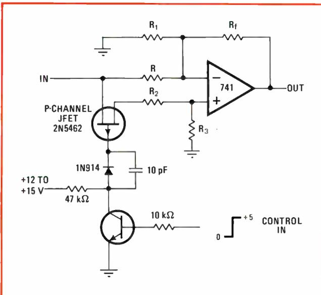
**FET inverts op amp.** Amplifier gain can be programmed either positive or negative, depending on whether the field-effect transistor is conducting or not conducting. Gain is the ratio of  $R_f$  to  $R_i$ ; for gains of  $\pm 1$ ,  $R_f$ ,  $R_2$ , and  $R_3$  are all equal value, and  $R_1$  is half the value.
