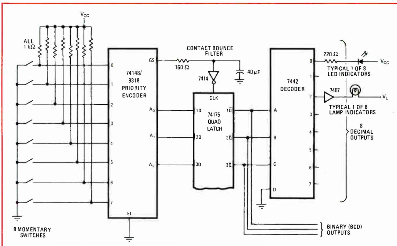
**Interlock.** Momentary switches are interlocked from simultaneous operation by encoding them into a set of latches and then decoding the latch states to drive indicators or other apparatus. Circuit is more reliable than mechanical interlock, and switches can even be remote.
