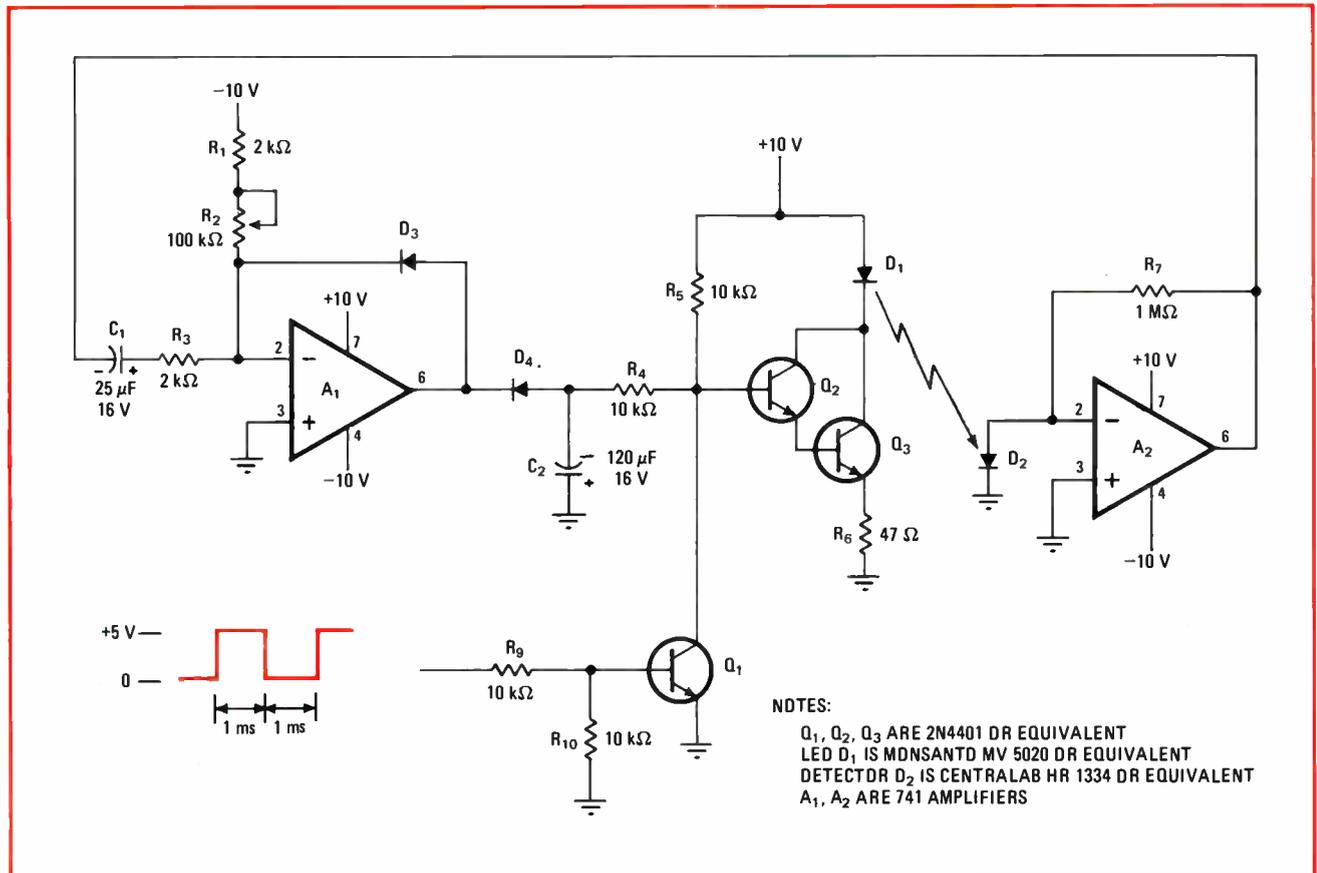
**Steady glow.** Feedback loop senses variations in output of light-emitting diode, which may occur as temperature changes. Photodiode response is almost constant with temperature; it is amplified, and signal controls another amplifier whose output controls LED drive circuit.
