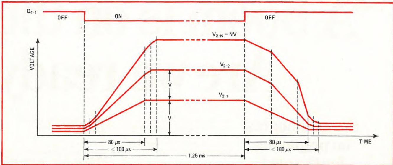
**2. Timing.** The stages start switching sequentially, as diodes  $D_{1-1}, D_{1-2}, \dots$  successively become back-biased, but after all stages are switched, they change voltage levels concurrently. Therefore the rise time is essentially that of a single stage. Similarly, the fall time is essentially independent of the number of stages. The output amplitude is the product of the power-supply voltage and the number of stages.
