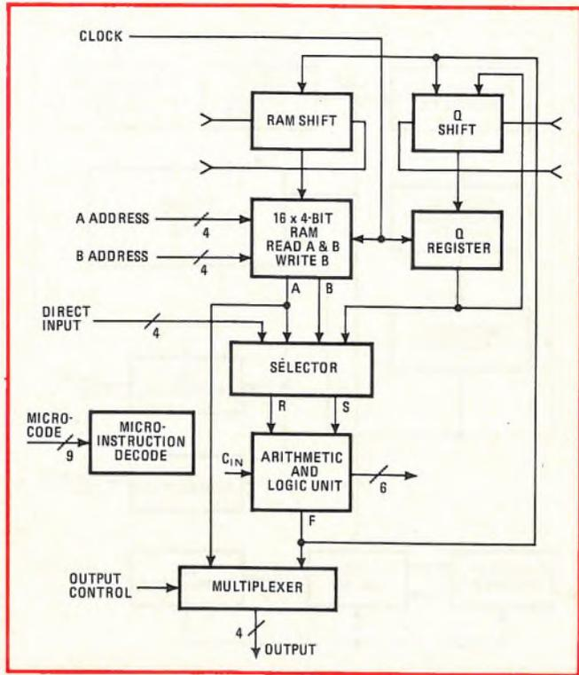
13. Double dealing. AMD's new low-power Schottky TTL processor-slice can handle information 4 bits wide. Entered simultaneously via two input ports and processed simultaneously by the twin RAM ports, this data is handled in sequence on chip by the speedy ALU.
