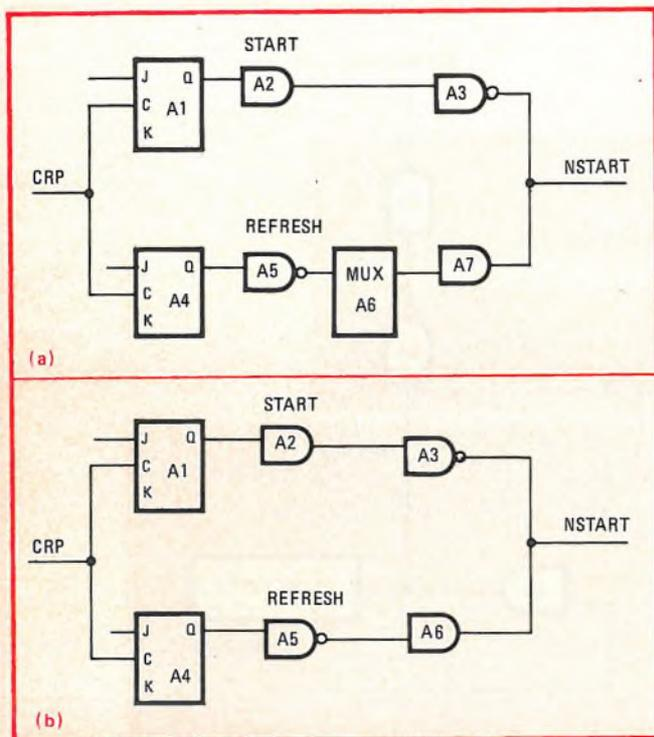
**6. Common reference.** Relative timing is measured from a common reference point (CRP). In 6(a), parallel logic chains lead to the NSTART signal but the multiplexer stage (MUX) adds extra delay tolerance. In 6(b) the multiplexer is replaced by logic gates.
