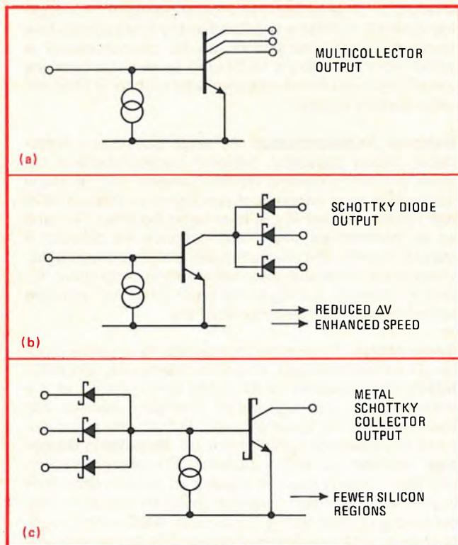
**4. The forms of I<sup>2</sup>L.** Injection logic can be built in three forms: the standard-multicollector I<sup>2</sup>L gate (a), the Schottky-diode output device (b) and its ultimate configuration, a pure metal Schottky collector (c). The last is fastest and smallest and comes from IBM.
