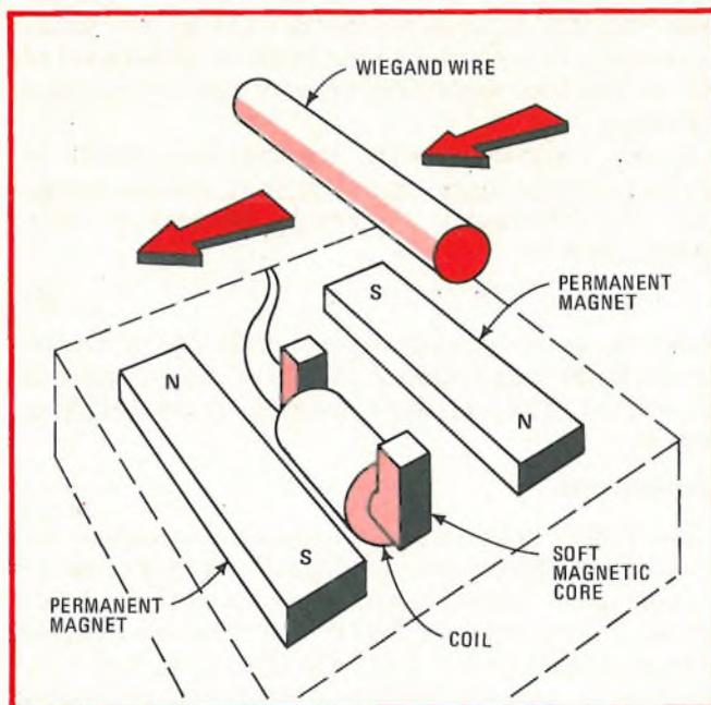
**9. Moving on.** Schematic of a transformer-style read head shows the "switching" magnets used to control the position of the switching signal for maximum sensitivity of the read head as Wiegand-treated wire passes in direction of the arrow.
