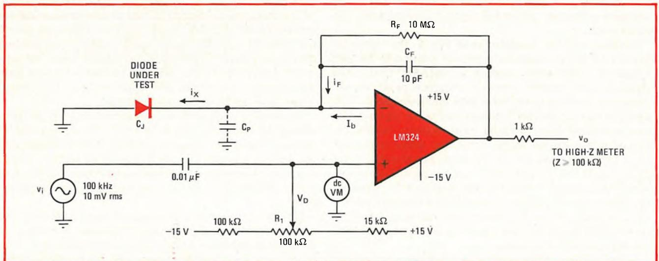
**1. Measuring capacitance.** Junction capacitance of a semiconductor diode is measured as a function of dc-bias voltage in this circuit. Diode is connected to inverting input terminal of LM324 operational amplifier, and dc-bias and ac-test voltages are applied to noninverting input terminal. Low ac test voltage avoids excessive modulation of depletion layer, for accurate measure of small-signal junction capacitance.
