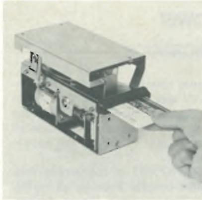
Originally developed for gasoline stations, a magnetic-card reader that can handle even distorted and stained cards has a bit-error ratio of less than  $10^{-6}$ . Maximum recording density is 72 characters. Matsushita Electric Industrial Co. Ltd., 3-1-1 Inazu-cho, Osaka 561, Japan [446]
