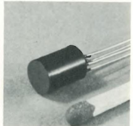
Miniature photocoupler built with a LED and a photoresistor has isolation of 250 V between input and output. An input signal of 10 mW suffices, and the response time is 1 ms. The output circuit can handle up to 80 mW. Segor/Silec, 69 rue de Monceau, 75008 Paris, France [458]
