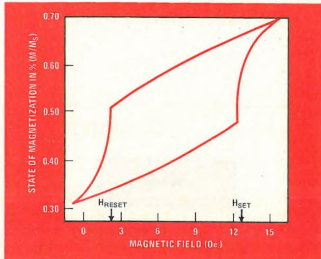
**7. Wire switch.** A key factor in the Wiegand effect is the magnetic loop that provides "set" and "reset" points that are repeatable and depend upon the relative magnetization of shell and core of the wire.
