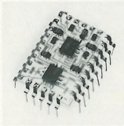
*All three oscilloscopes make wide use of monolithic IC's in order to reduce weight and the number of adjustment points.*
