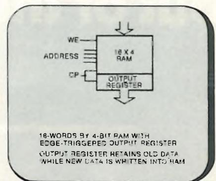
The 9410 64-bit Read/Write Memory is a register-oriented high-speed device organized as 16 words by four bits. An edge-triggered 4-bit output register allows new input data to be written while previous data is held. Three-state outputs are provided for maximum versatility. The 9410 operates at a 10 MHz Microinstruction rate.
