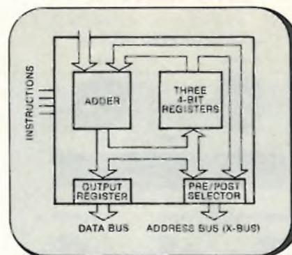
The 9407 Data Access Register (DAR) performs memory address arithmetic for RAM resident stack applications. It contains three 4-bit registers — program counter, stack pointer and operand address — a 4-bit adder, a 3-state address output buffer and a separate output register with 3-state buffers. The DAR performs 16 instructions, and operates at a 10 MHz Microinstruction rate. Samples available August.
