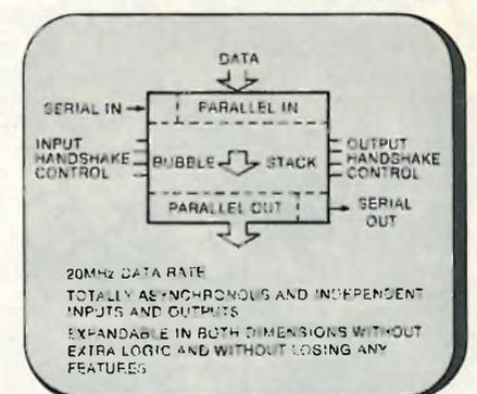
The 9403 FIFO Buffer Memory is a high-speed expandable fall-through type with totally independent and asynchronous inputs and outputs. Organized as a 4-bit wide by 16-word deep "bubble stack," it has four bits parallel and bit-serial data inputs and outputs. Complete "handshake" control signals are provided for unambiguous operation in asynchronous systems. It is intended for disk and high-speed communications applications with data rates of up to 20 MHz.
