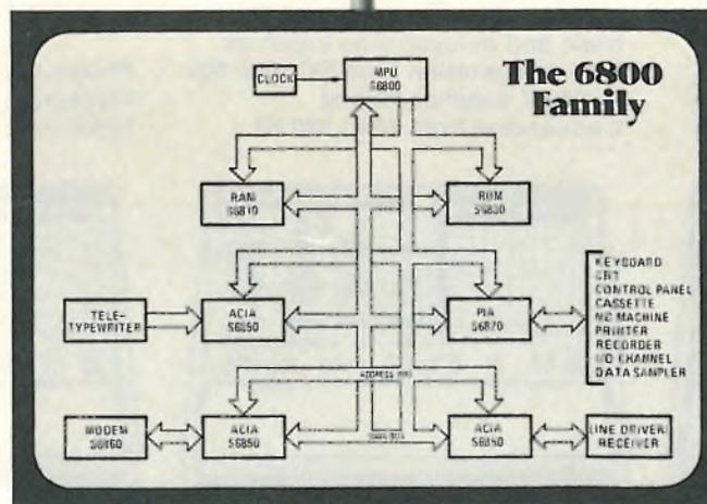
It's less costly because it requires fewer parts. It runs on just one +5V power supply instead of three. It has a more efficient instruction set, which reduces the number of locations needed in memory because of six memory addressing modes. And it needs no TTL to bring it together.
