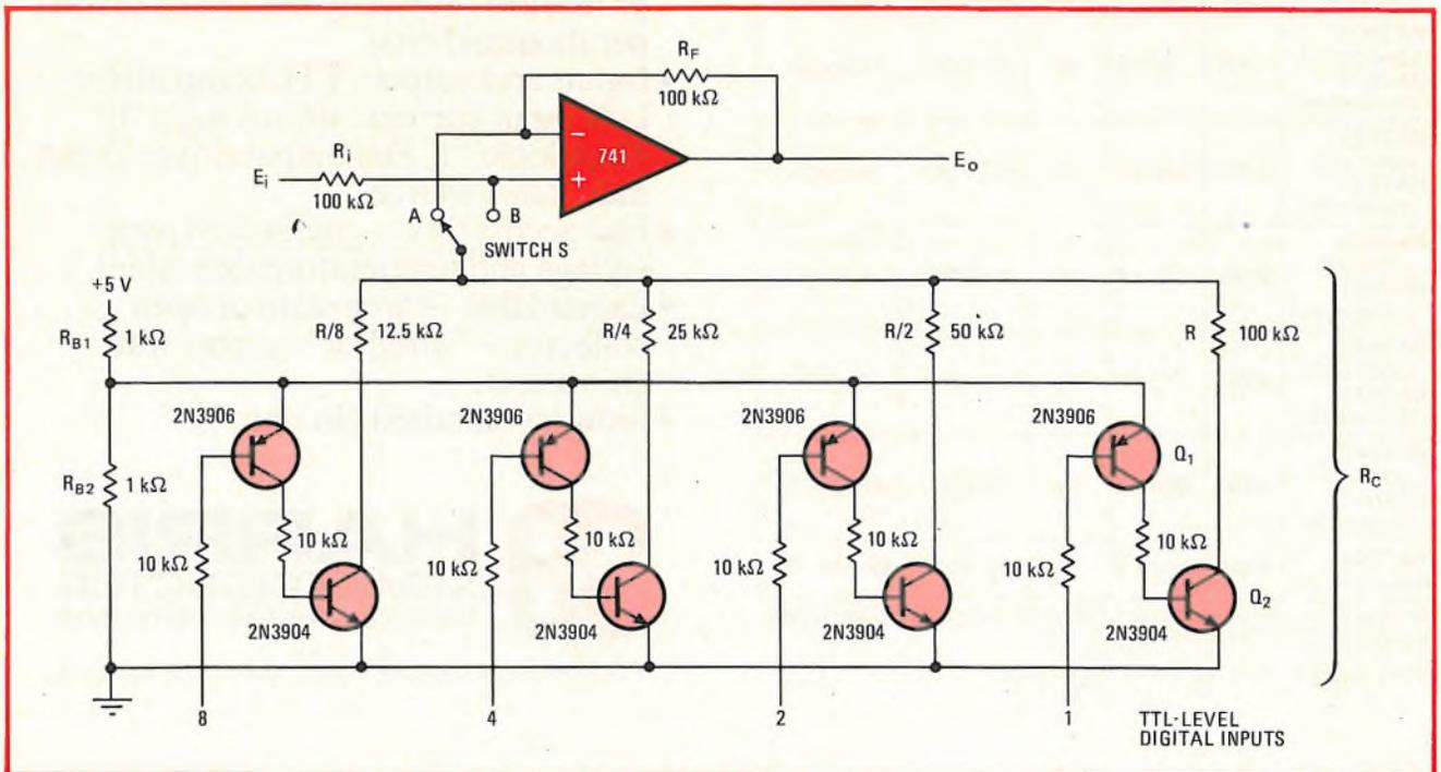
**Programmable gain or attenuation.** The operational-amplifier circuit has a gain of  $G_A = N + 1$  or  $G_B = 1/(N + 1)$ , depending on whether switch S is set to position A or position B. The number N is the value of the negative-logic binary number applied to the digital inputs. If programmable sign-reversal is required, a digitally controlled inverter [Electronics, March 6, p. 85] can be used in tandem with the amplifier.
