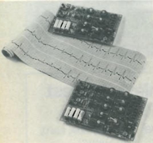
Analog Devices decided that the per-channel cost of these units could be significantly reduced by putting more than one channel into each amplifier package. Since the channels all share a common oscillator, this approach not only saves money but has the added advantage of eliminating beat-frequency noise caused by oscillator mixing.
