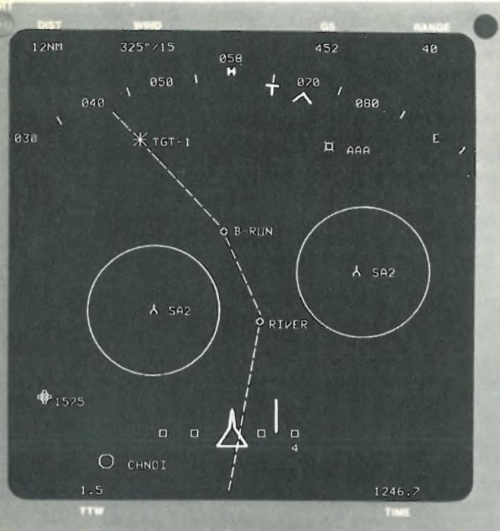
**Digital data.** Computer-generated symbology shown on 6.5-inch-square CRT display in Collins' flight management system includes the aircraft's position (lower center), the flight plan (dashed line), along which are landmarks such as a river and the target, and the location of surface-to-air missiles and their lethal range (big circles) at the aircraft's altitude.
