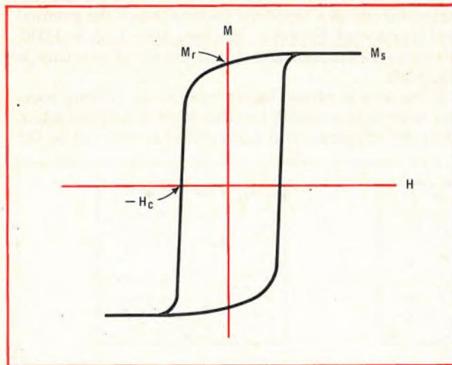
**3. Magnetic switch.** In this plot of a typical hysteresis curve, the coercive field  $H_c$  is the reverse field necessary to bring the magnetization  $M$  to zero; the remanence  $M_r$  is the value of  $M$  at  $H = 0$ ; and the saturation magnetization  $M_s$  is the limiting value of  $M$ .
