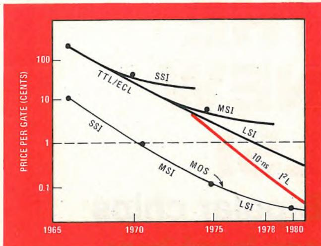
**1. Economical.** Injection logic is the cheapest way of achieving high performance across the board. Using standard bipolar technology,  $I^2L$  gates should break the crucial 1-cent-per-gate level this year and reach the 0.1-cent-per-gate level of MOS in 1980.
