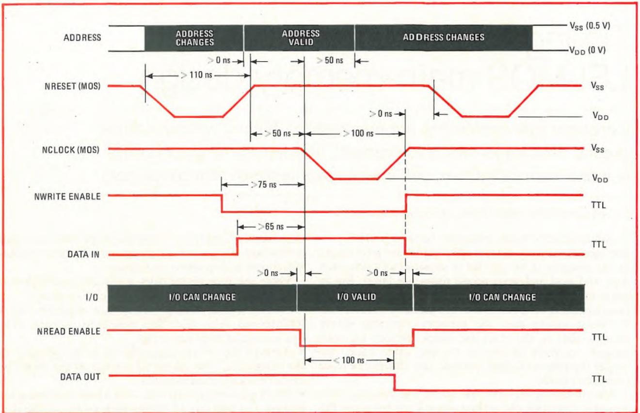
**2. Timing is everything.** For each of the signals to a semiconductor memory, there are basic restrictions on when transitions for address changes, input-output, write and read signals can occur. (Voltage levels are for MOS and TTL devices.)
