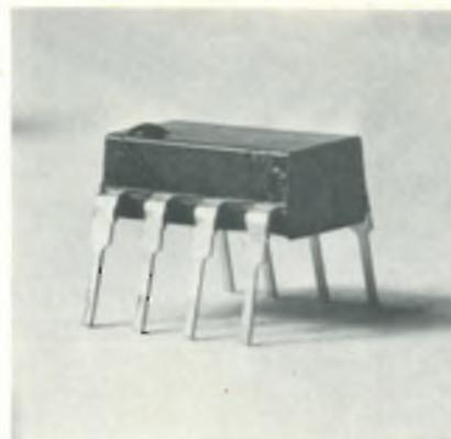
A high-speed opto-isolator, designated the IL-100, transmits data at 5 megabits per second with a common-mode rejection of 50 dB. The IL-100 uses a LED light source and an IC receiver that incorporates a photodiode. Litronix, Hitchin, Herts. SG5 1LW, England [469]
