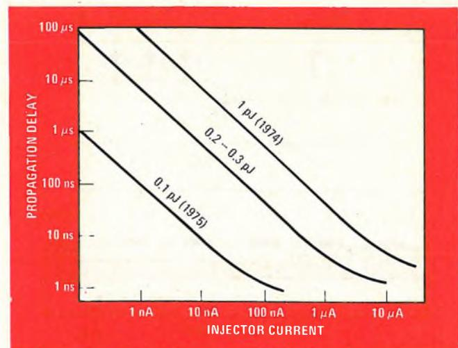
**7. Looking better and better.** In just two years the basic  $I^2L$  process has been improved to the point where 10-ns gates are possible at 100-nA injection current. This is better than TTL performance and signals a new level of programmable processor circuit speed.
