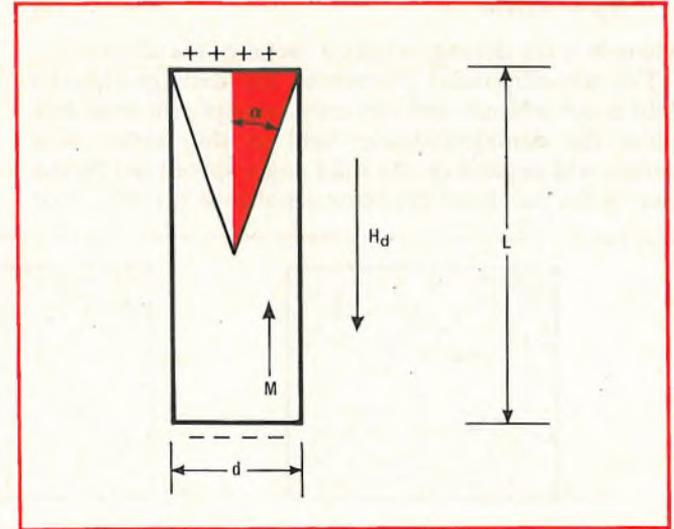
**5. In reverse.** The demagnetization field of a long cylinder (wire) will be proportional to  $d/L$ . This demagnetization field operates in a saturated material when the external magnetization field is removed, which is a key factor in the Wiegand effect.
