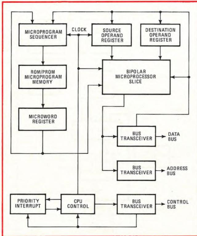
**14. The system.** Beating high system costs is this minimum-package CPU built from 11 of AMD's 2900 family of LSI computing elements. It's expandable to handle 16- or 32-bit-wide words typically required in today's minicomputers and data-processing equipment.
