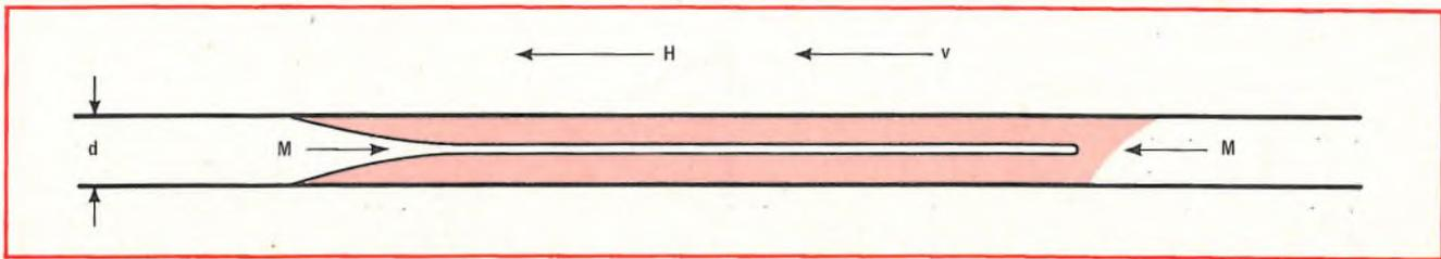
**6. Wire domain.** The approximate shape of the domain formed during the switching process in an inelastically stretched nickel-iron wire travels down the wire at a rate of about  $2 \times 10^5$  centimeters per second. At this velocity, switching times are on the order of  $100 \mu\text{s}$ .
