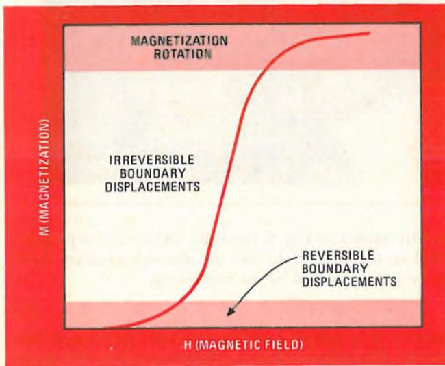
**2. Magnetic boundaries.** A typical magnetization process occurs in three phases: first, a reversible phase in which the domain boundaries move, next an irreversible phase, and finally the domain walls in effect disappear with all the magnetization in one direction.
