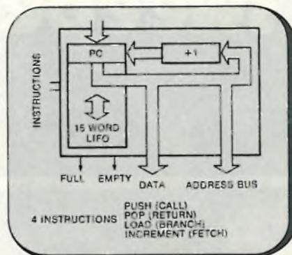
The 9406 16-word by 4-bit "Push Down-Pop Up" Program Stack stores program counter and return addresses for nested subroutines in programmable digital systems. It executes four instructions — Return, Branch, Call, and Fetch as specified by a 2-bit instruction. The 9406 may be expanded to any word length without additional logic and operates at a 10 MHz Microinstruction rate over 16 bits.
