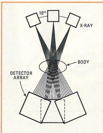
**Scanning.** The X-ray source and the detector array move in an arc around the body, producing 80,000 X-ray absorption values at  $10^\circ$  intervals for each scan of a 13-millimeter-thick cross section. The unit can produce up to eight sections automatically.
