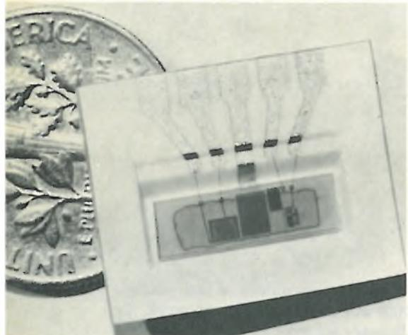
**Less tuning.** Transmitter transducer (left) on Zenith's surface-wave i-f filter is acoustically coupled to receiver transducer (right) through a multistrip coupler.
