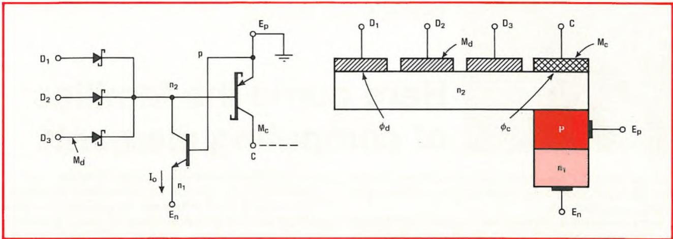
**10. Down the road.** IBM's Wiedmann and Berger have proposed an elegant solution to the Schottky problem—pure metal Schottky collectors—which they say result in minimum-geometry gates much faster than conventional ones. But new processing techniques will be needed.
