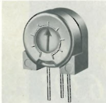
Thin-film trimmer module, the NX-13, has two fixed-resistor branches built in. The device is used primarily for adjustment of operational amplifiers and voltage-regulator integrated circuits. Copal Electronics Co. Ltd., Shiba-nishikubo, Minato-ku, Tokyo 105, Japan [455]
