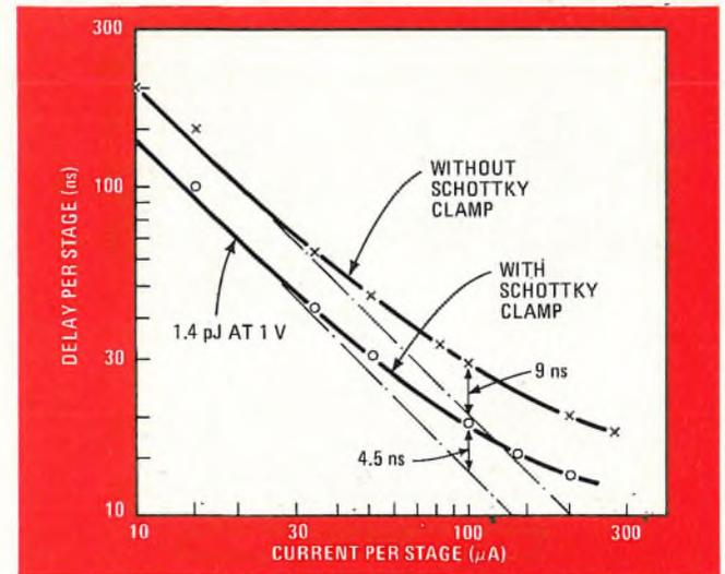
**9. Proof.** When equipped with Schottky clamps, I<sup>2</sup>L gates operate at the 5-nanosecond gate propagation-delay needed for high-performance applications. This speed is to be contrasted with non-Schottky gates' 9-ns operation. (Data courtesy of IBM, Boeblingen.)
