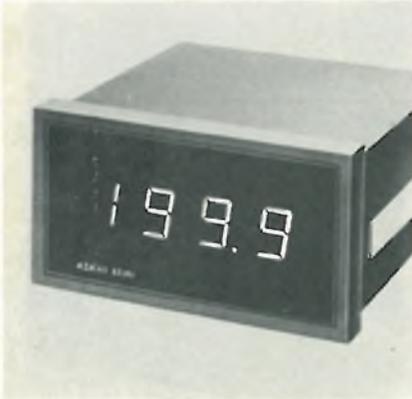
Digital panel meter, model MP-1000, has 0.59-inch-high light-emitting-diode display that can be read at 20 feet. Accuracy is within (0.1% of reading  $\pm 1$  digit). LSI circuits are used extensively. Asahi Keiki Co. Ltd., 1-15-13 Shimomaruko, Ota-ku, Tokyo 144, Japan [443]
