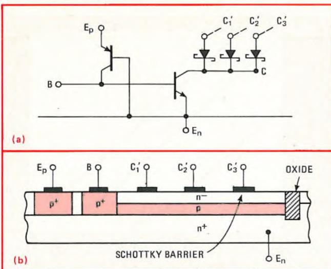
**8. Clamped.** The Schottky clamp in an I<sup>2</sup>L gate reduces logic swings, which in turn reduce gate delays. The clamps can be built in just one additional mask step directly into the p-diffusion wells (b), so that as a result very little space is wasted.
