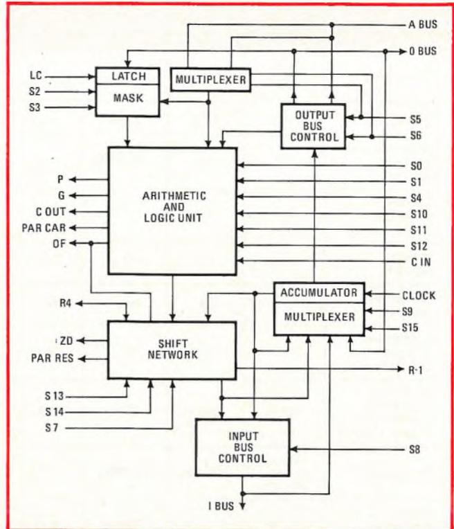
**15. Emulation.** Motorola's 4-bit processor slice is configured like the typical ECL controller. The ALU is driven by a multiplexed latch which loads an accumulator for fast iterative computer operations. It's designed for very fast programmable data-processing duty.
