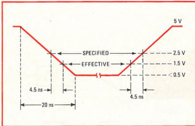
**3. Delay line output.** Rise and fall times at the delay-line outputs depend on the relative position of the tap, and outputs are defined at the 2.5-volt level. Since TTL circuits respond at 1.5-V level, extra delays can occur for taps near the end of the line.
