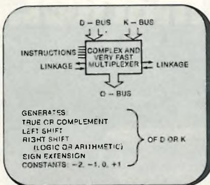
The 9404 Data Path Switch (DPS) is a very fast combinatorial array for closing data path loops around arithmetic logic networks (like the 9405 ALRS). A 5-bit instruction word selects one of the 32 instructions operating on two sets of 4-bit data inputs. Four linkage lines are available for expansion in 4-bit increments. The delay is less than 30ns over 16 bits. Samples available August.
