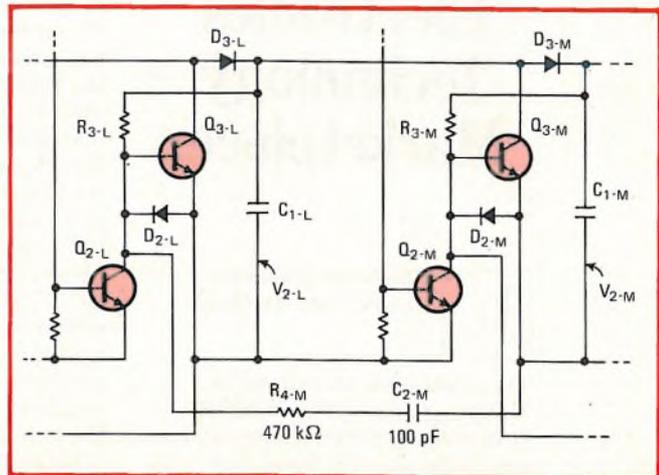
**3. Feedback.** To achieve 400-Hz operation, the circuit in Fig. 1 is modified as shown here.  $R_3$ s provide positive feedback within each stage, and  $R_4$ s and  $C_2$ s provide positive feedback from each stage to the preceding stages. Without the feedback, rise time is about 1 ms; with feedback, rise and fall times are both less than 0.1 ms.
