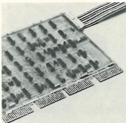
A wire-wrappable module, the MDB-11, is designed for interface applications for the PDP-11 and PDP-8 computers. It will accommodate up to 70 14- to 40-pin dual in-line ICs or sockets. Sintrom Electronics Ltd., 2 Arkwright Rd., Reading, Berkshire RG2 OLS, England [445]
