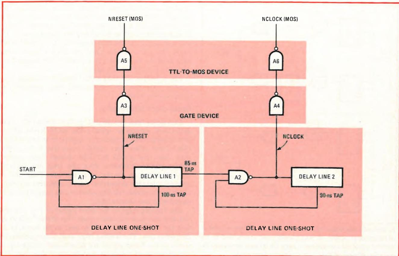
**4. Reset and clock.** Use of two delay lines permits shorter lines, with closer relative timing accuracies. Circuits in the gates and TTL-to-MOS devices which lead to the memory are arranged on the same chips so that their performance tracks closely.
