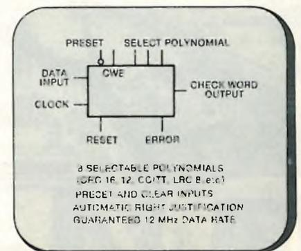
The 9401 Cyclic Redundancy Check Generator/Checker is an advanced tool for implementing the most widely used error-detection scheme in serial digital data handling systems. A 3-bit control input selects eight different generator polynomials, including CRC-16 and CRC-CCITT, as well as their reciprocals (reverse polynomials). Separate Clear and Preset inputs are provided.
