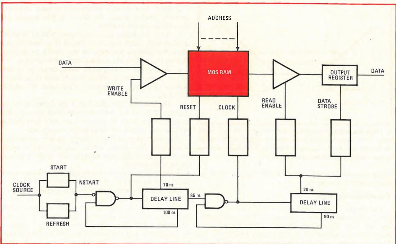
1. **Memory.** A system built around an MOS random-access-memory device can use delay lines to distribute timing signals having close timing accuracies. In the logic chains leading to the memory, gates on the same chips can help equalize time delays.
