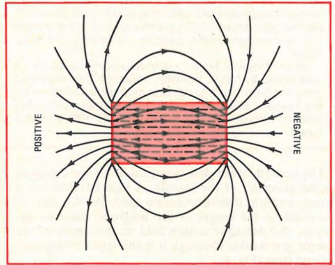
**4. Poles apart.** Magnetic poles, formed on the uniformly magnetized surfaces of a cylinder, establish a magnetic field opposite to the direction of the magnetization. If the external field is removed, the field established by the poles tends to demagnetize the sample.
