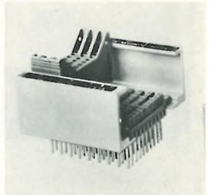
Circuit blocks handle currents to 2 A and test voltages to 2,000 V. The base blocks have 30 connections with wire-wrap terminals. The plug-ins are available with 10, 20, or 30 connections for crimped wires up to 1.5 mm<sup>2</sup> in cross section. Entrelec, rue Leon Blum, 69611 Villeurbanne, France [460]
