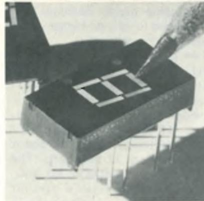
An orange LED display has been added to Monsanto's series of green, red, and yellow displays. The series of readouts, designated MAN 3600, is available in a variety of configurations and is compatible with most circuit requirements. Monsanto Europe S.A., Place Madou 1, B-1030 Brussels, Belgium [448]
