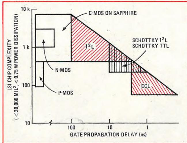
**2. The best for the most.** Of the three approaches to bipolar LSI,  $I^2L$  handles the greatest range of applications—from 100-ns to 1-ns gate propagation-delay times. Schottky TTL and ECL overlap at the fast end, and n-MOS technology takes up the slow jobs.
