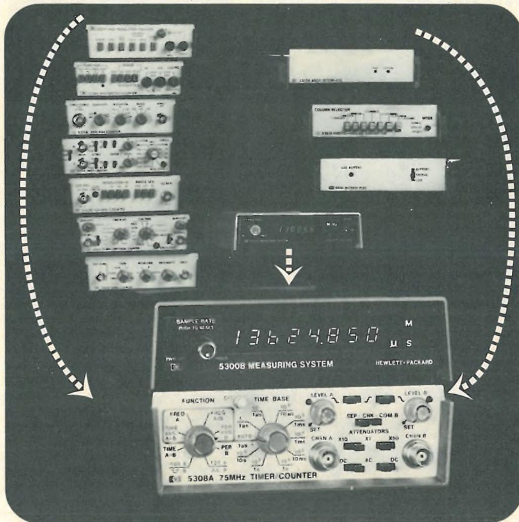
The heart of HP's versatile 5300 Measurement System is a sophisticated mainframe which contains counting circuitry and display. Snap it onto the bottom module you need and it instantly becomes one of eight feature-loaded instruments. The 5300 basic modules include:
