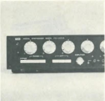
Using a direct-synthesizing system without a phased-lock loop, the model FS-221A generates signals ranging from 0.01 Hz to 200 kHz. Frequency of the signals can be controlled remotely. TOA Electronics Ltd., 307 Suwa-cho, Shinjuku, ku, Tokyo 160, Japan [454]
