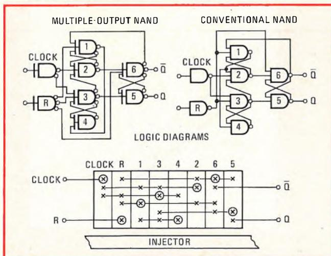
**6. Less wiring.** D-type flip-flop from Bell Labs requires no contacting between cells. This is because logic units in the configuration abut one another adjacent to the injector rail and can therefore be placed automatically in the six available wiring channels.
