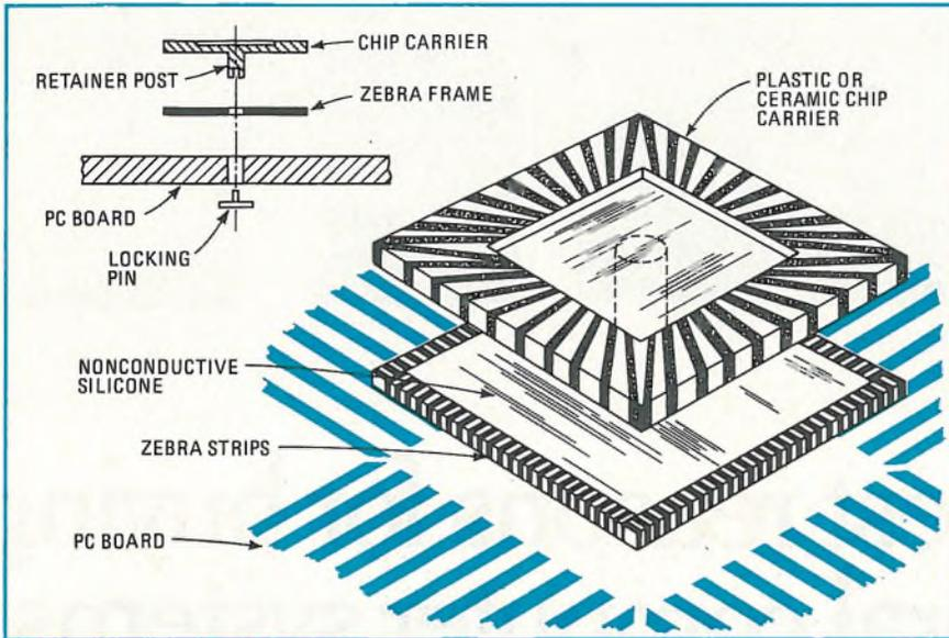
**No solder.** Leadless chip carrier is mounted by Tecknit on a printed-circuit board by pressing its contacts against conductive elastomer Zebra strips. Firm contact to the board is made with the help of a special post and locking pin.
