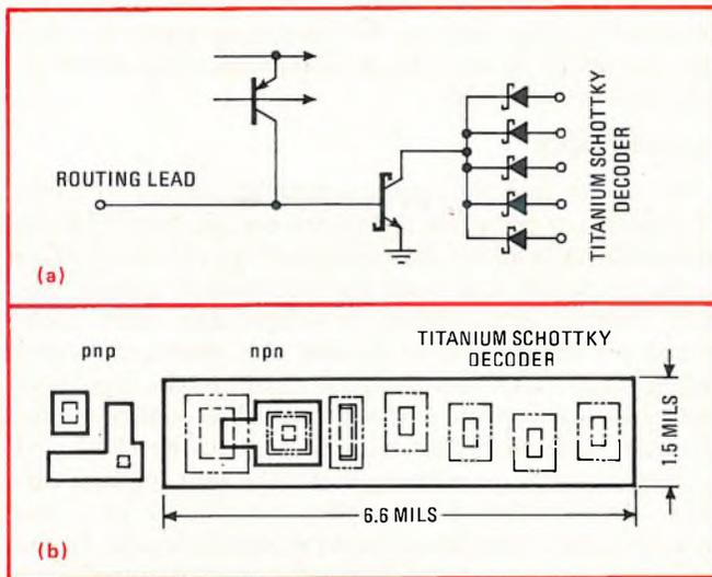
**11. Getting Schottky both ways.** This injection-like logic structure from Motorola uses Schottky diodes to maximum advantage. Routing to the gate is achieved through low forward Schottky diodes, while gate outputs also are Schottky-clamped for extra performance.
