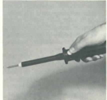
A high-voltage test probe with detachable tips is rated at a maximum working voltage of 30 kilovolts. It is said to be completely safe, since the design ensures thorough earthing and screening of the probe head. Wallis Electronics Ltd., Worthing, Sussex, England [450]
