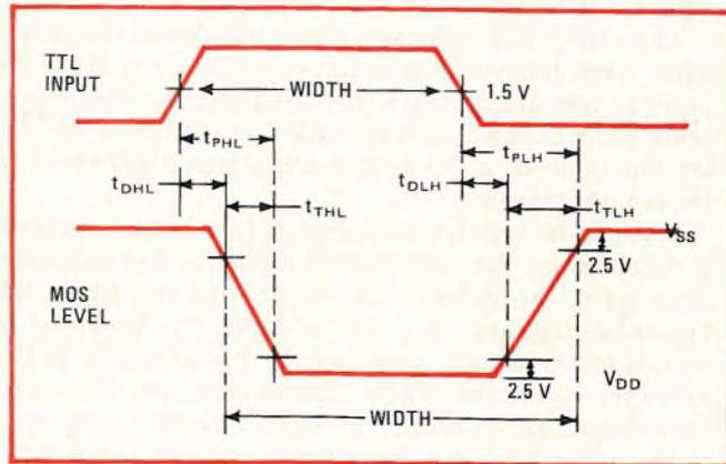
**5. Driving time.** The TTL-to-MOS driver tends to stretch out the trailing edge and the MOS pulse widths are larger than the TTL widths. This fact must be taken into account when calculating the pulse widths of the TTL signals.
