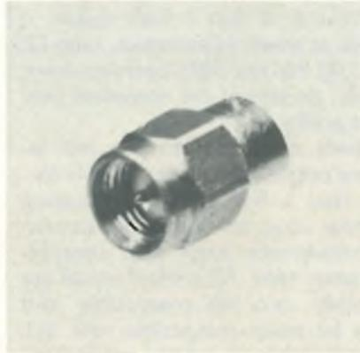
A family of rf miniature coaxial terminations includes laboratory types 12 mm long for dc to 18 GHz, and 9-mm industrial versions for dc to 12.4 GHz. Both types have a maximum VSWR of 1.25 and can handle 1 watt. Radi-all, 101 rue Philibert Hoffmann, 93116 Rosny, s/Bois, France [447]
