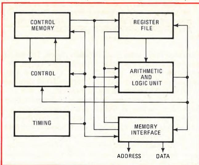
**12. It's standard.** This basic building block configuration characterizes most of today's bit-slice chip configurations. From Motorola, this block of circuits is incorporated into a new ECL slice. Key elements are, of course, the ALU and control memory.
