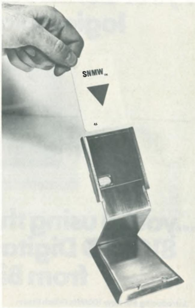
This type of card reader offers several advantages. The wires cannot be altered or "erased" except by destroying the entire card. The detection system requires no electrical power input to the read head and the detection signal is independent of the velocity of the card as it passes the read head.
