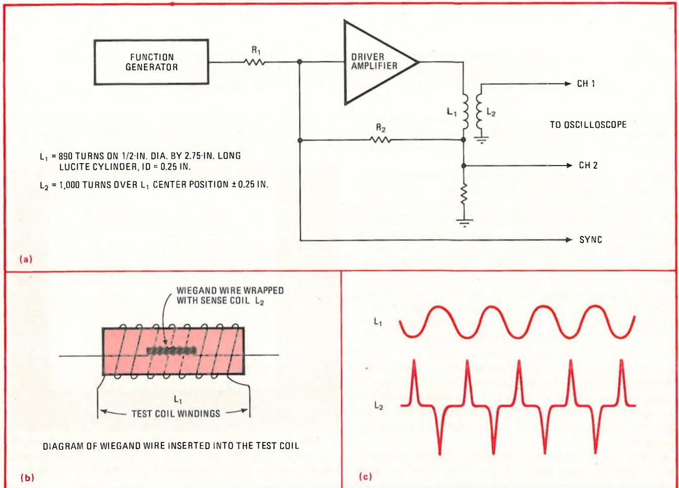
**8. Sensing.** Typical Wiegand-wire test apparatus (a) has a coil arrangement as in (b). Output signal (c) shows oscilloscope trace of waveforms in drive coil  $L_1$  and sense coil  $L_2$ . The means of detecting the signal pulse depends on the particular application, however.
