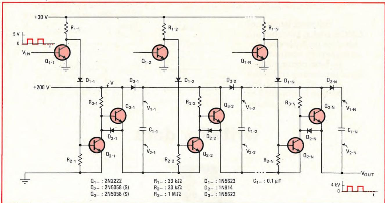
**1. Kilovolt generator.** Square wave of 4 kV at 400 Hz is produced by circuit with 20 low-voltage stages. Each stage includes a capacitor ( $C_1$ ) that acts as a floating power supply for the next stage. The capacitors are charged in parallel and then connected in series. If lower output voltage is desired, input can be applied to  $Q_{1-2}$  or  $Q_{1-3}$  or . . . instead of  $Q_{1-1}$ . (Actual circuit also includes elements shown in Fig. 3.)
