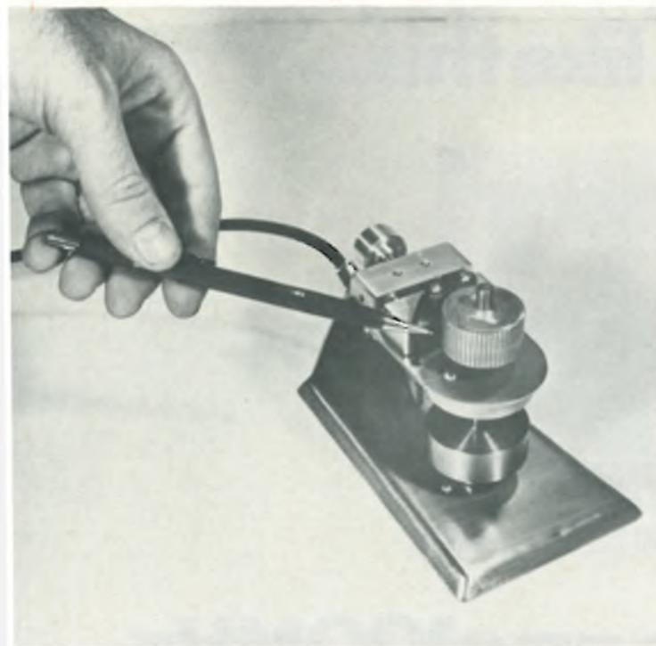
**10. Turning point.** Rotary pulser with Wiegand wires embedded in the rotor could be used for electronic auto ignition since the pulse generated is independent of the velocity of the distributor shaft. As each wire passes the read head a pulse is generated, which could be used to produce, among other things, an ignition spark.
