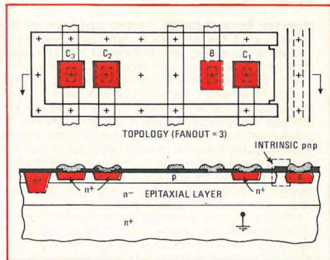
**5. Easy to make.** Schottky I<sup>2</sup>L logic unit from Bell Laboratories is for a fanout of 3. It is fabricated with the aid of a minimum of selective diffusions—p-type for pnp emitters and collectors, n-type for collector contact, and an n<sup>+</sup> emitter diffusion for npn outputs.
