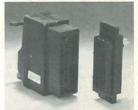
ing 120 or 156 contacts. Mated contact forces of 150 grams minimum are typical, with several thousand mating cycles possible without degradation of performance. Both plug and receptacle halves are modular and permit variations in termination and conductor styles.
