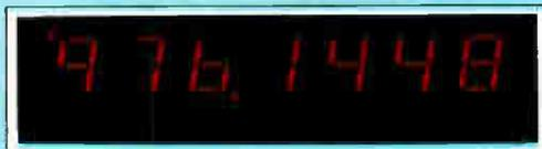
sensitivity is a minimum specification (not a typical) allowing lock-in measurements from even extremely weak signals. The 100 MHz bandwidth means the 5740 handles everything from sub-audio to VHF. Seven, not six digit resolution, means 0.1 Hertz resolution at 1 MHz, 1 part in 10 million in period measurements, with the decimal point always automatically correct.
