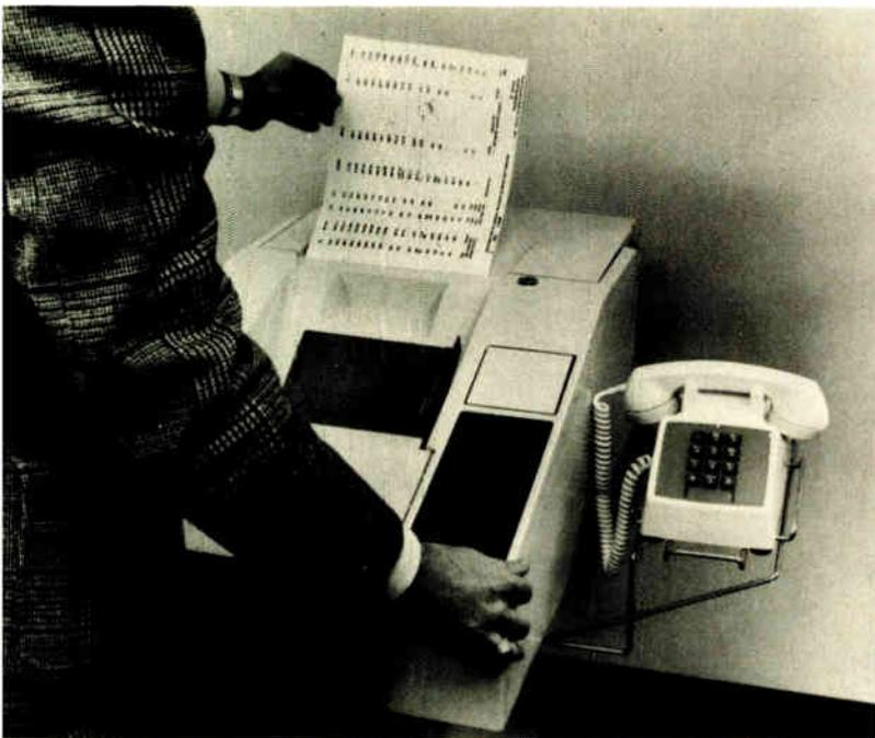
**5. A graphic example.** Xerox Telecopier 200 reads outgoing information and records incoming data with a He-Ne laser at twice the speed of the laserless model. Facsimile equipment is but one of many potential applications in graphics for lasers.
