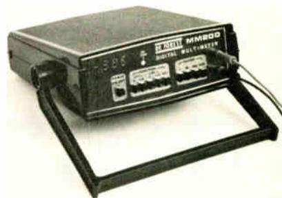
1 to 1,000 volts, ac and dc current with full-scale ranges from 1 to 1,000 milliamperes, and resistance with full-scale ranges from 1 to 10,000 kilohms. Accuracy is within  $\pm(0.5\%$  of reading + 1 digit) on most of the dc voltage and current ranges on ac,  $\pm(1\%$  of reading + 2 digits).
