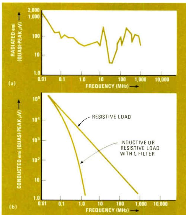
**4. Jagged spectrum.** With electromechanical relays, both contact opening and closure create interference that is radiated directly, as well as being conducted along lead wires, which then act like antennas and also radiate rfi. Radiated interference (a) is highly erratic, especially from 10 to 1,000 MHz. In contrast, conducted interference (b) exhibits a continuous spectrum of noise.
