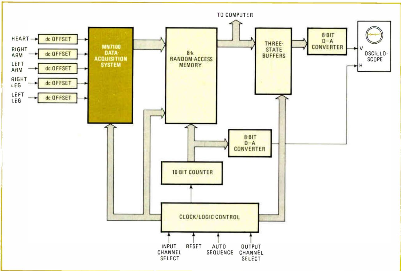
**4. Waveform analysis.** With the MN7100, digital techniques can be used to analyze and display analog waveforms. In this biomedical application, various points of the body are being monitored and displayed on the oscilloscope to ascertain variations in the heart muscles.
