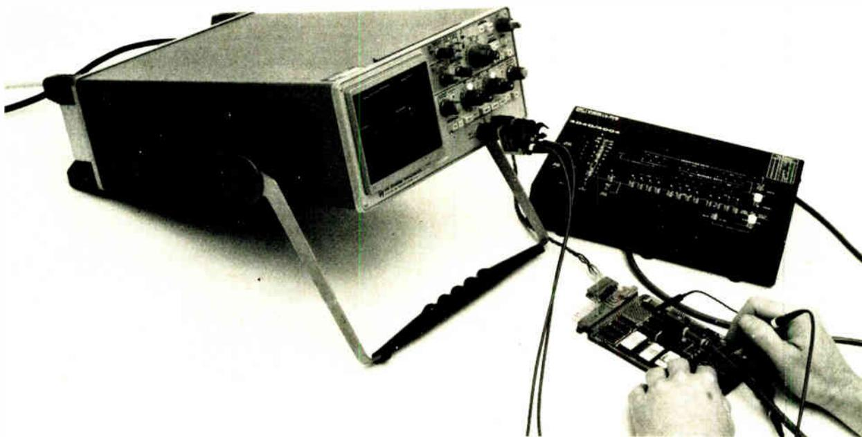
**Debugging.** The final stage in the design of a microprocessor system is to see if the program works as it was designed to. Here, an oscilloscope and a system analyzer are being used to debug a system whose program is in a PROM, equivalent to a circuit breadboard.
