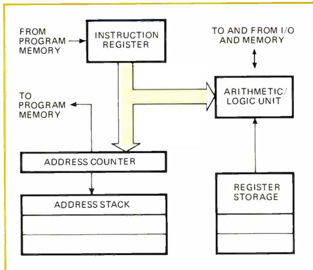
**5. Inside the 4004.** In the Intel 4004 4-bit microprocessor, the address counter accesses the next instruction from memory, and the instruction register then controls the ALU. Read/write memory elements make up the ALU and the register storage cells.
