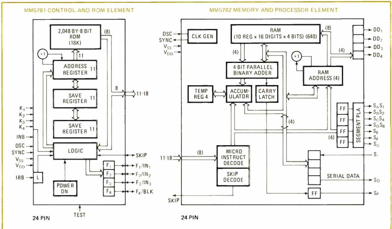
**3. Added power.** Two-chip microcontroller carries more internal ROM and RAM capacity than one-chip versions, making more powerful control systems possible. Program storage and control fit on the MM5781 program chip, with processing and RAM storage on the MM5782.
