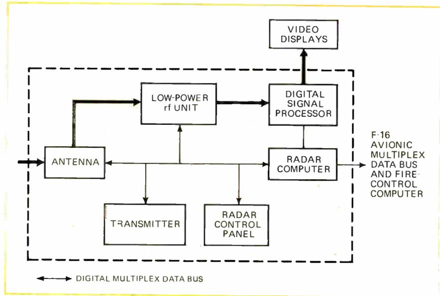
**Replaceables.** Five of the six line-replaceable units in the Westinghouse F-16 radar are interconnected by a digital multiplex bus. The sixth, the digital-signal processor, is connected to the radar computer by a separate high-speed data bus.
