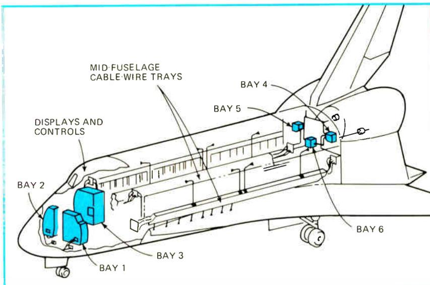
**Packed away.** Cutaway drawing shows locations of six bays containing avionics equipment. Controls, communications, and computer hardware are in forward pressurized crew section
