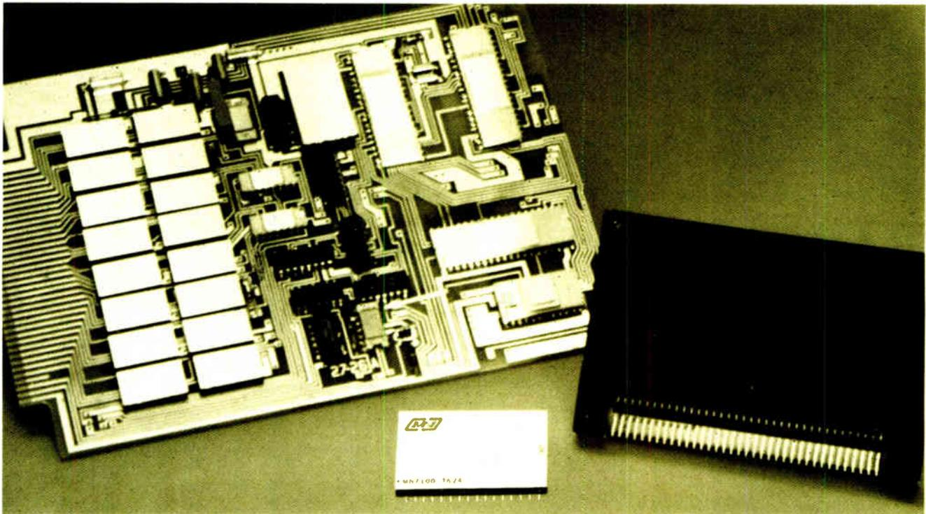
**Size dwindles.** Only a year ago, a multichannel data-acquisition system required an entire pc board. Then 16-channel 12-bit systems became available as hand-sized modules. And now a complete eight-channel 8-bit system has been squeezed into an IC-compatible DIP.
