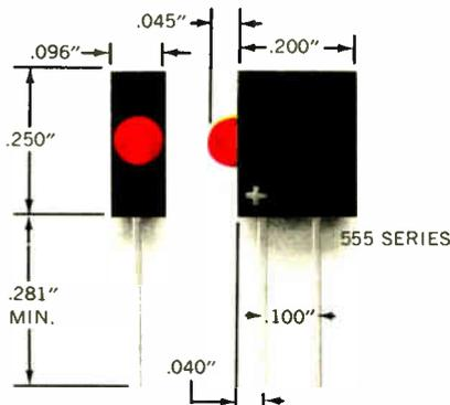
LED logic state fault indicators available in 14 models with voltage ratings from 1.7 to 14. Suitable for dense packaging on printed circuit boards—up to 10 units to the inch—IC compatible. With built-in series resistor. Polarity identified. Low power consumption.
