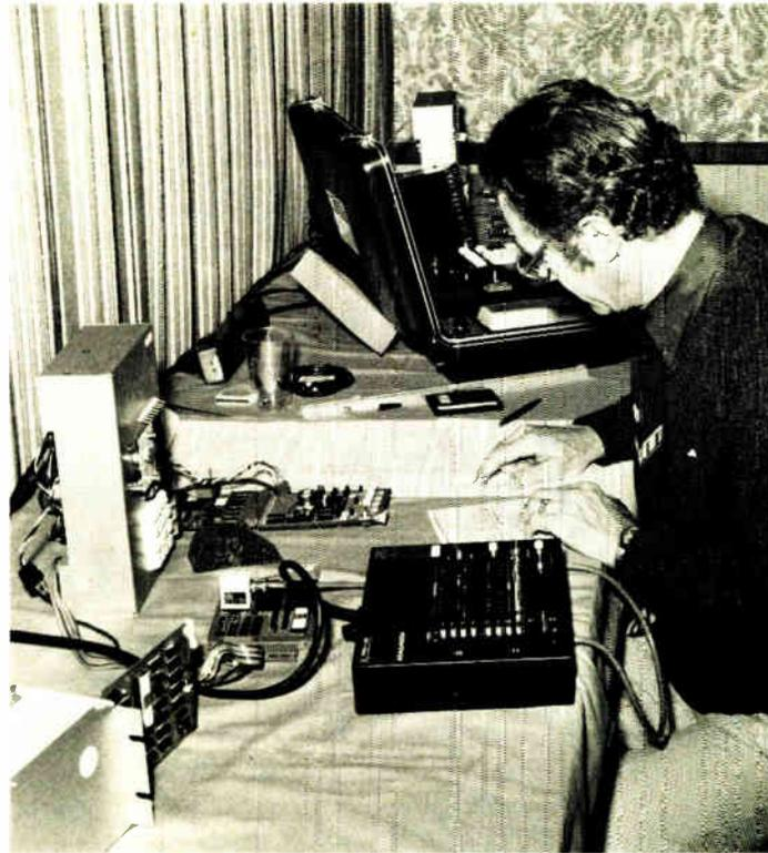
10. **At the bench.** Microprocessor systems—both hardware and software—can be checked out easily once the program has been fully documented, using the formats shown in F.g. 8 and a hardware system analyzer as shown here
