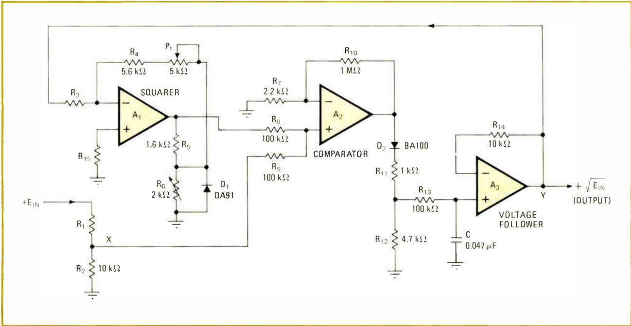
**1. Getting to the root.** Output from three-op-amp circuit is square root of input. Comparator  $A_2$  balances input with square of output to produce the root. Accuracy within 1% is achieved through good square-law characteristic of diode  $D_1$  in feedback loop of squarer  $A_1$ , plus adjustment of scaling and tracking controls  $P_1$  and  $R_6$ . Voltage follower  $A_3$  buffers voltage across capacitor.
