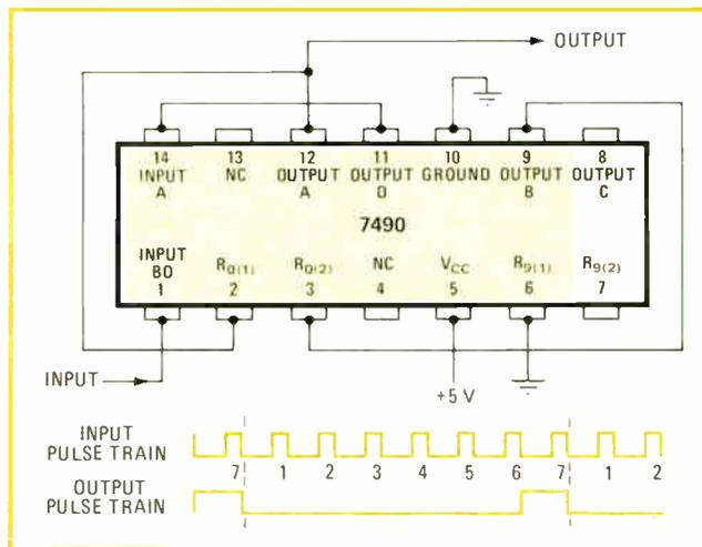
**Divide-by-7 circuit.** A 7490 TTL decade-counter integrated circuit, when connected as shown here, produces one output pulse for every seven input pulses. Because the divide-by-2 stage follows the divide-by-5 stage, the seventh count is a non-BCD code and can be detected by the internal two-input NAND gate to reset the counter. Other connections permit division by any other integer up to 10.
