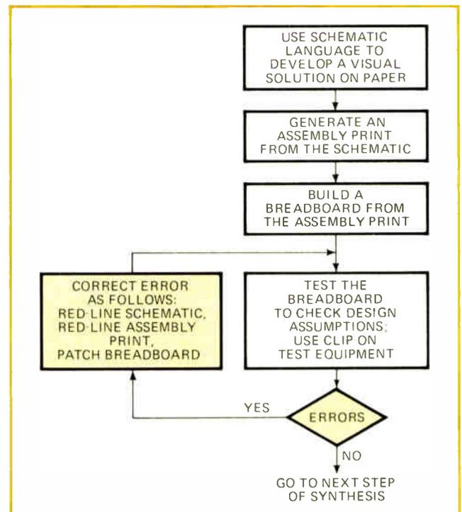
**2. Check it out.** In designing and debugging a hardware module, an engineer typically concentrates on the error-correction stage, in which the schematic and assembly prints are redlined and the breadboard patched to account for the changes.
