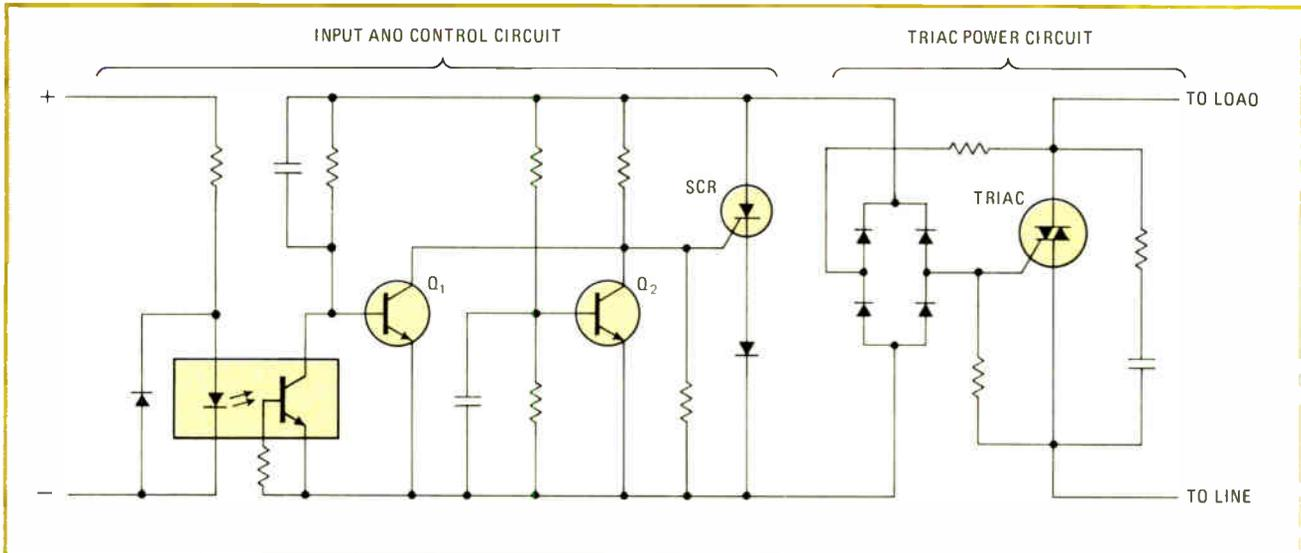
**6. Zero-voltage switch.** Special circuitry in zero-switching solid-state relays delays device turn-on until the driving-voltage sine wave crosses 0. In this Motorola circuit, there is a brief turn-on window between 0 and 5 V when transistor  $Q_1$  is off, permitting the SCR to fire and trigger the triac. As long as  $Q_1$  is on, the gate of the SCR is held at ground potential, thereby preventing it from conducting.
