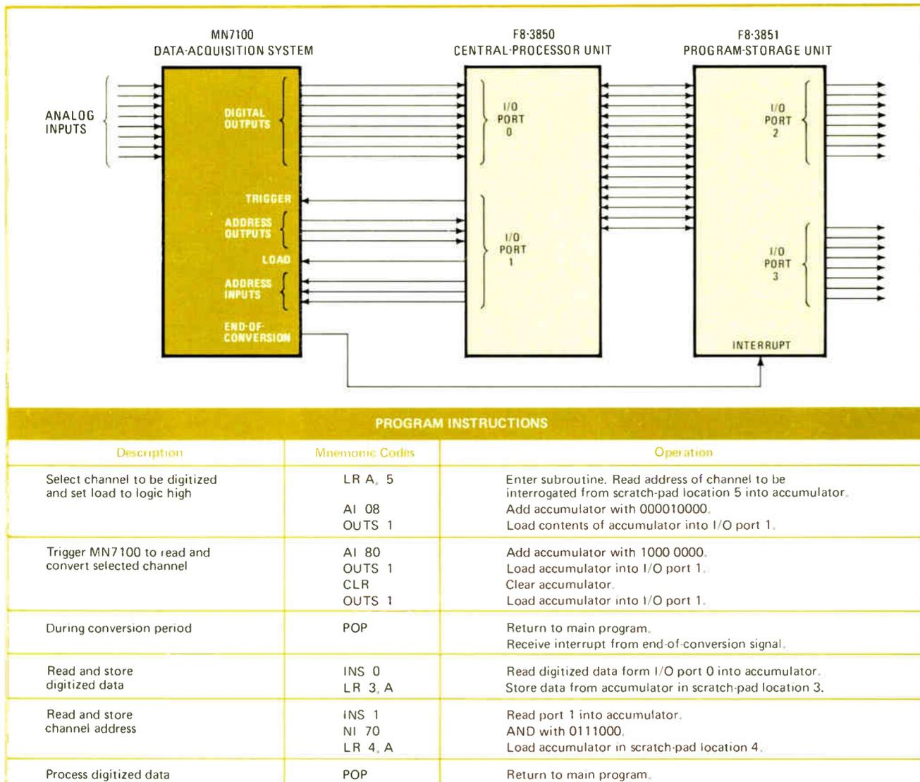
**3. Microprocessor hookup.** Connecting the MN7100 to microprocessor chip sets is easy—especially if the set, like the one here, has a bidirectional I/O port that can be dedicated to a data-acquisition system. Program instructions for the device also are simple
