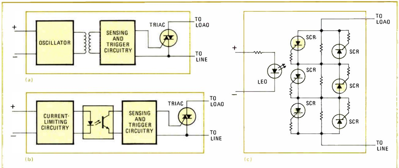
5. **Standard solid state.** Because they don't include optional zero-crossover circuitry, standard solid-state relays are generally about 30% less expensive than their zero-switching counterparts. Here, three versions are shown: transformer-isolated (a) and optically isolated with either a phototransistor (b) or a chain of photo-SCRs (c). The latter configuration is used to obtain very high blocking voltage.
