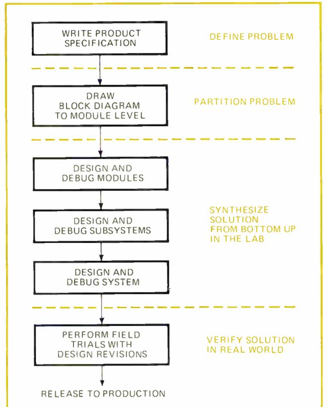
**1. Scientific approach.** When designing hardware, most engineers use a regular approach, working from the original product specification. One of the keys to successful designs is partitioning the problem into easily solved modules and subsystems.
