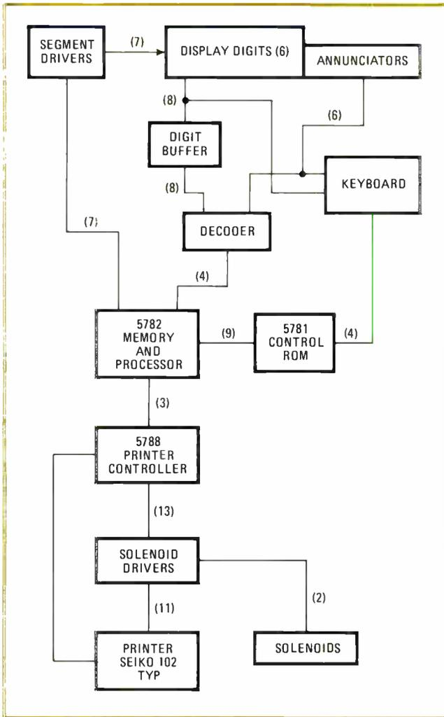
**6. Cashing the chips.** Only nine IC parts are required for an electronic-cash-register system with many desirable features for retail applications. With slight modification, the machine's six-digit LED display can be changed to a high-voltage gas-discharge display.
