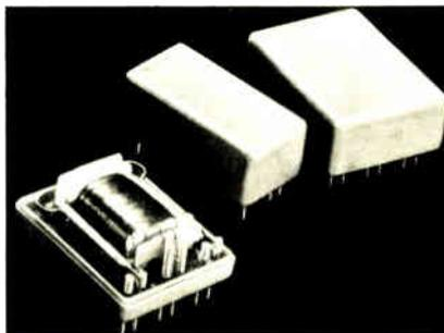
tween boards. Terminal spacing is on a standard 0.1-in. grid. The relays can be wave- or hand-soldered at up to 650°F for a normal soldering time without damage. The spdt version measures 1.105 by 0.605 by 0.437 inches, while the dpdt unit measures 1.105 by 0.905 by 0.437 in.
