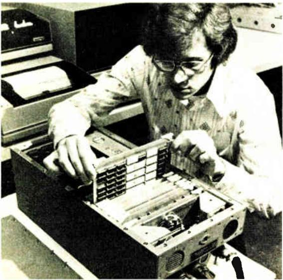
the Westinghouse computers will operate with 16-bit words at speeds of 375,000 operations per second as well as handling 32-bit, 8-bit, or single-bit increments. The DAIS processor and its read-only memory use off-the-shelf, large-scale integrated circuits. The capacity of the core memory is 64,000 16-bit words.
