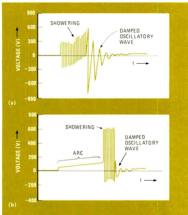
**3. Rfi and contact break.** Unwanted switching spikes are particularly severe when an electromechanical relay switches off an inductive load. The contact voltage breaks up into a series of sharp spikes that eventually damp out. This high-frequency showering takes place even if there is no arcing (a). When arcing does occur, (b), the amplitude of the spikes becomes substantially higher
