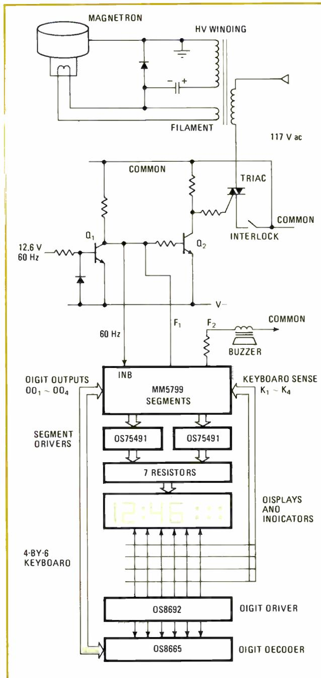
**5. What's cooking?** This microwave-oven controller shows the efficiency of design with a dedicated microcontroller. Relatively few components are needed to achieve, virtually automatically, all the timing and control functions involved in household cooking.
