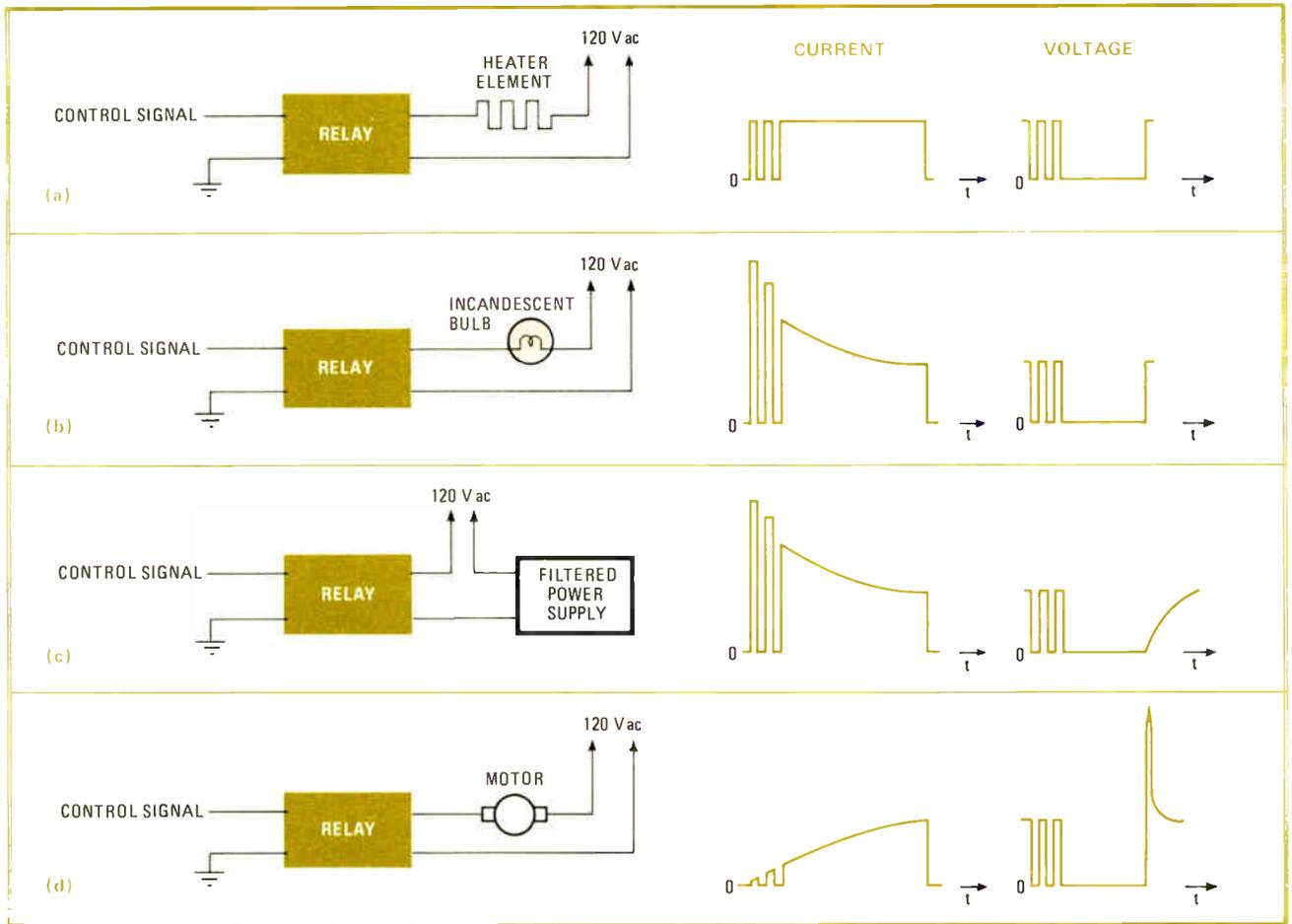
**2. Contact bounce vs load.** In an electromechanical relay, contact bounce occurs when the load is switched on. The extent to which bounce disrupts load current and load voltage depends on the load itself, whether it is a heater element (a), an incandescent bulb (b), a power supply (c), or a motor (d). In the latter case, the largest switching spike is produced upon contact opening, not contact closure.
