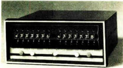
ture is the set of comparison-logic outputs that are available at the rear connector—using gatable, latching, open-collector transistor-transistor logic. This forms a data bus that enables the 8400 series comparators to interface with a central process computer. For additional versatility, the comparison-logic outputs can be multiplexed onto buses with 4, 8, 16, or 24 wires.
