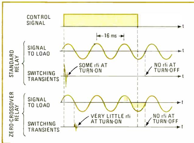
**7. Solid-state comparison.** With or without zero-crossover, solid-state relays generate only a fraction of the rfi produced by electromechanical units. Although zero-crossover versions create less rfi at turn-on than standard models, both types essentially eliminate rfi at turn-off. This is because each employs a thyristor output, and a thyristor is inherently a zero-crossover device for turnoff.
