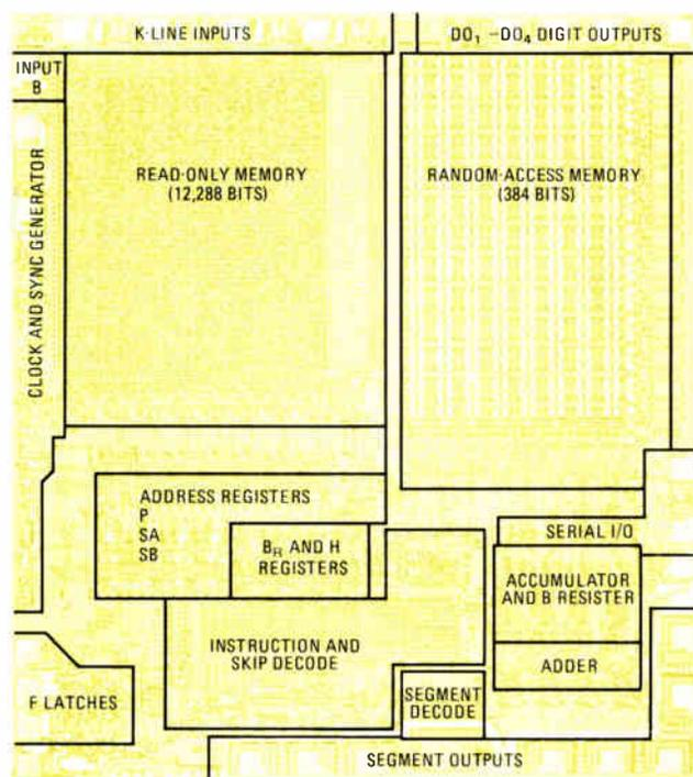
**1. Calculator-derived processor.** Part of a new family of dedicated microcontrollers is the MM5799 programmable calculator chip. Designed for quick-turnaround applications, it contains all system timing, arithmetic and logic, control-ROM, and RAM functions.
