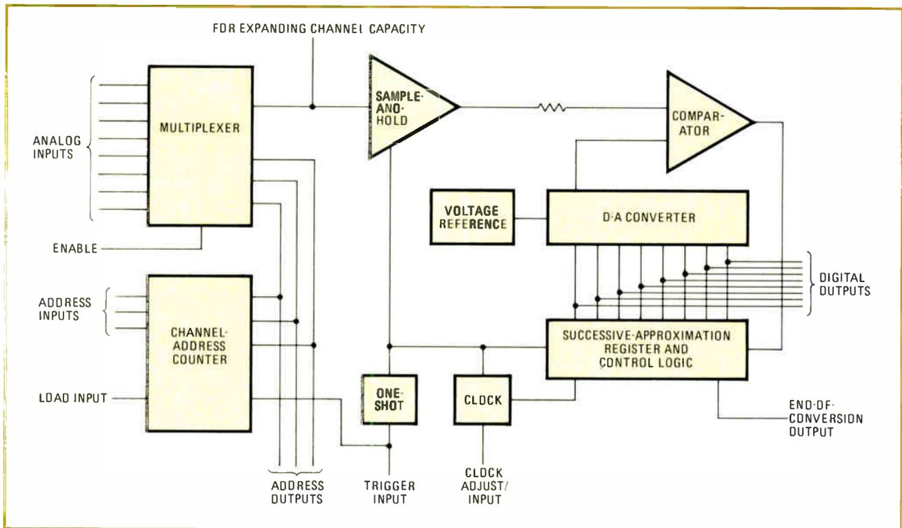
**2. The works.** Circuit operation of the MN7100 is fairly conventional. The desired input channel, selected via the address counter, is fed to the sample-and-hold amplifier by the multiplexer. When the sample-and-hold changes from track to hold mode, the signal is digitized by the a-d converter, which is composed of the d-a converter, the comparator, the voltage reference, and the logic register.
