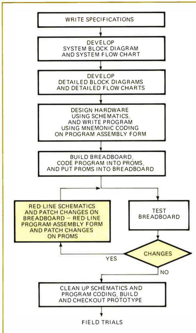
**7. Program design.** The procedure for writing a microprocessor program is similar to that of designing hardware. For every step in hardware design, there is an equivalent step in program organization, so hardware and software elements appear together.
