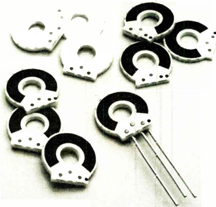
**Before and after.** Photo above shows cermet elements of Bourns model 87/88 semiprecision potentiometer. Elements are shown before (upper left) and after they have been laser-trimmed in a novel production technique
