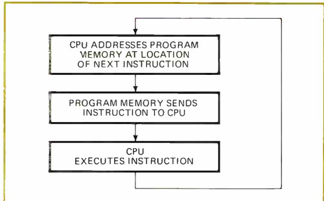
**4. Instruction cycle.** To execute one instruction, a microprocessor typically goes through three fundamental steps—addressing memory, extracting the instruction from memory, and performing the operation. A typical cycle takes about 11 microseconds.
