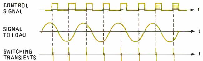
zero-crossover device for turn-off: after the gate signal has been removed, it will not turn off until its anode current has decreased to about 0. From the standpoint of turn-off, there is no difference between a zero-crossover solid-state relay and a standard one.
