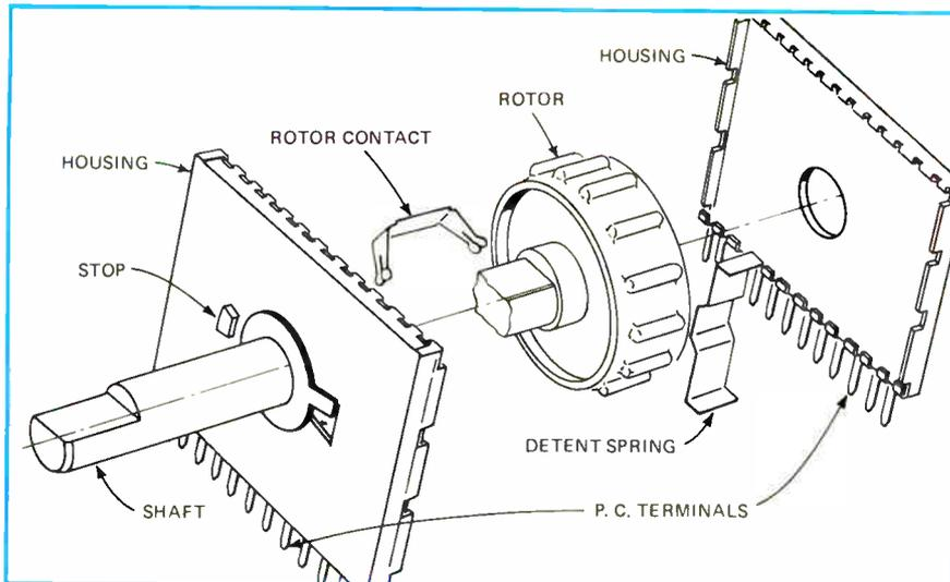
**New style.** Metal matrix, below, contains the contacts, conducting paths and terminals for Oak Industries' rotary switch. Cut to specifications, one matrix is fastened to front housing, a second to the rear housing.
