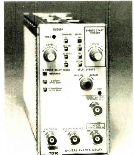
effective memory of the analyzer or delay the action of the memory by a specific number of digital words. In the delay-by-events mode, the 7D10 will count from 1 to 10<sup>7</sup> arbitrary trigger events, periodic or aperiodic, and deliver an output after the preselected count has been reached. In the analog domain, the 7D10 can be used to eliminate jitter or wow in mechanical systems. Price of the plug-in is \$925, and delivery time is 10 weeks.
