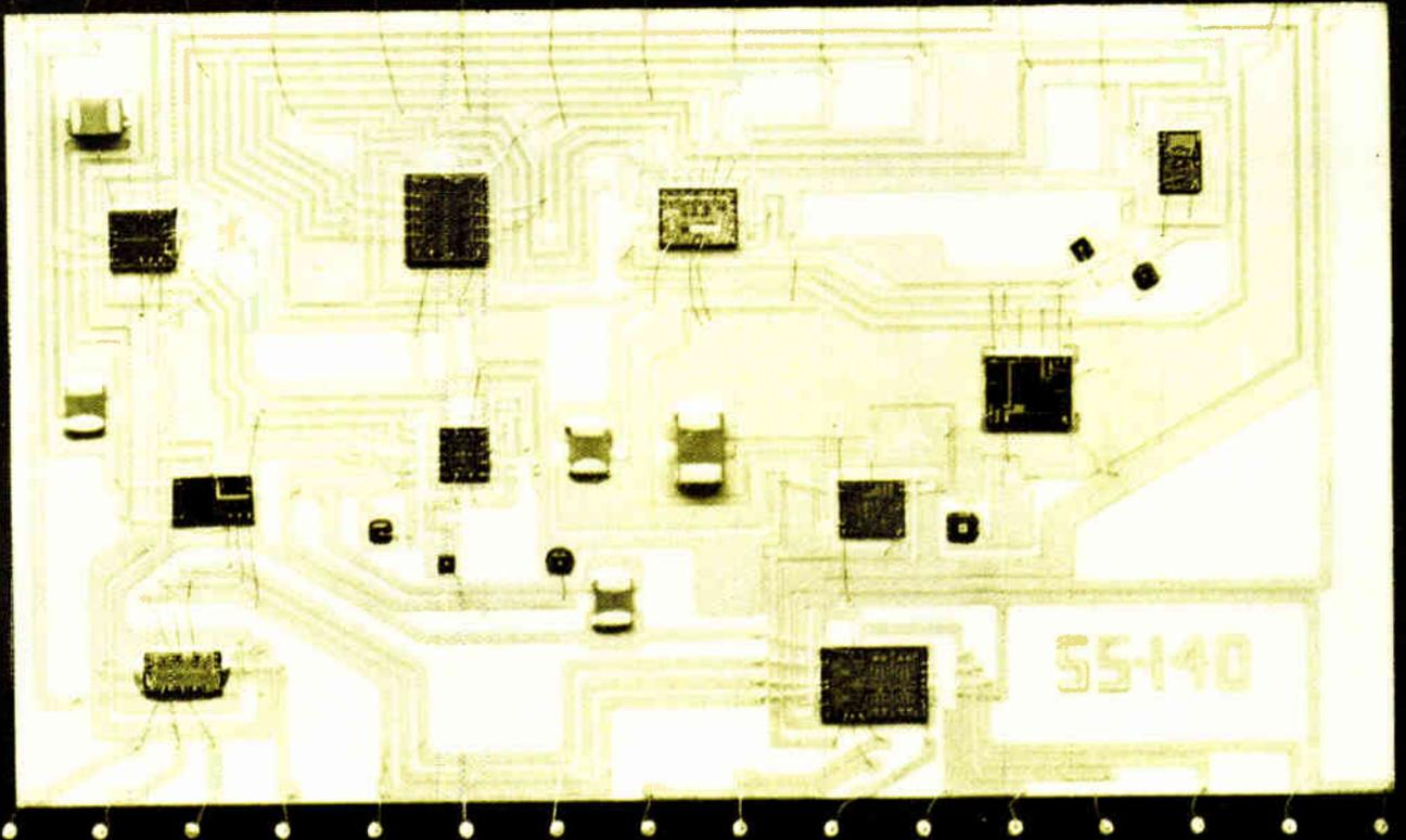
1. **Uncovered.** Inside the 32-pin DIP of the MN7100 data-acquisition system is a 21-chip, thin-film hybrid circuit that can multiplex, sample and digitize eight analog inputs. The device even includes integral clock, control logic, and voltage-reference source.
