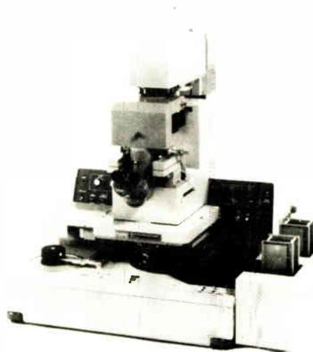
**9. Reduction projection.** Canon's FPA-141 step and repeats a 4:1 mask image onto a resist-covered silicon wafer. The unit can print 0.89- $\mu\text{m}$  lines in positive resists and 1- $\mu\text{m}$  lines in negative resists.
