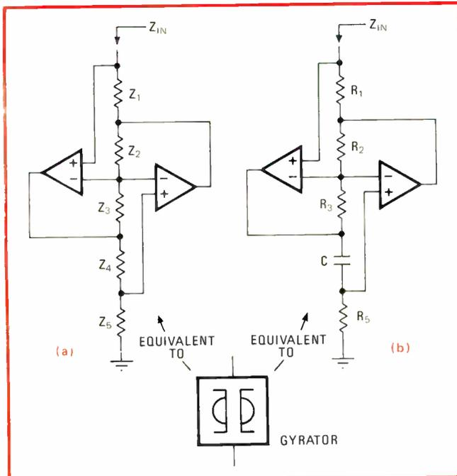
**2. Realistically.** Preferred gyrator realization (a) requires two amplifiers and five impedances. In practical RC implementation (b), impedance  $Z_4$  is a capacitor, and the other impedances are resistors. The gyrator may also be represented by the special symbol shown here.
