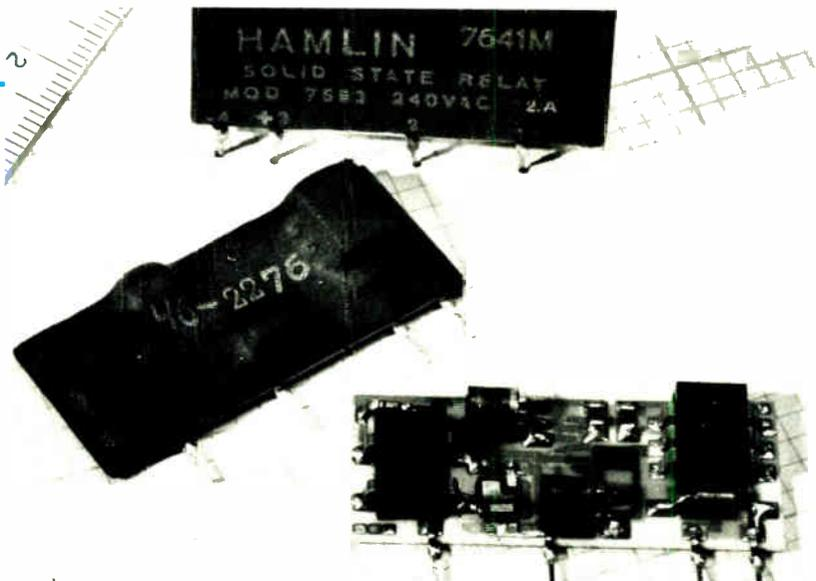
**2. Single in-line.** To build this low-cost relay, Hamlin assembles pretested packaged components on a substrate containing screened resistors and conductors.
