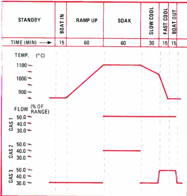
**13. Diffusion.** Time, temperature, and gas flow are controlled in the diffusion process. Note that temperature vs time functions use ramps rather than step functions to maintain process control.
