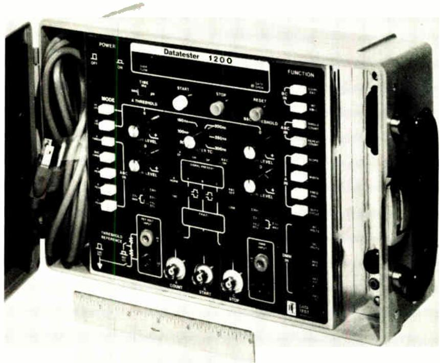
**Helper.** Somewhat bulkier than an attache case, the portable Datatester 1200 multifunction circuit-tester does the job of several separate instruments, including a digital multimeter and a frequency counter and timer. It also counts digital-logic transitions.
