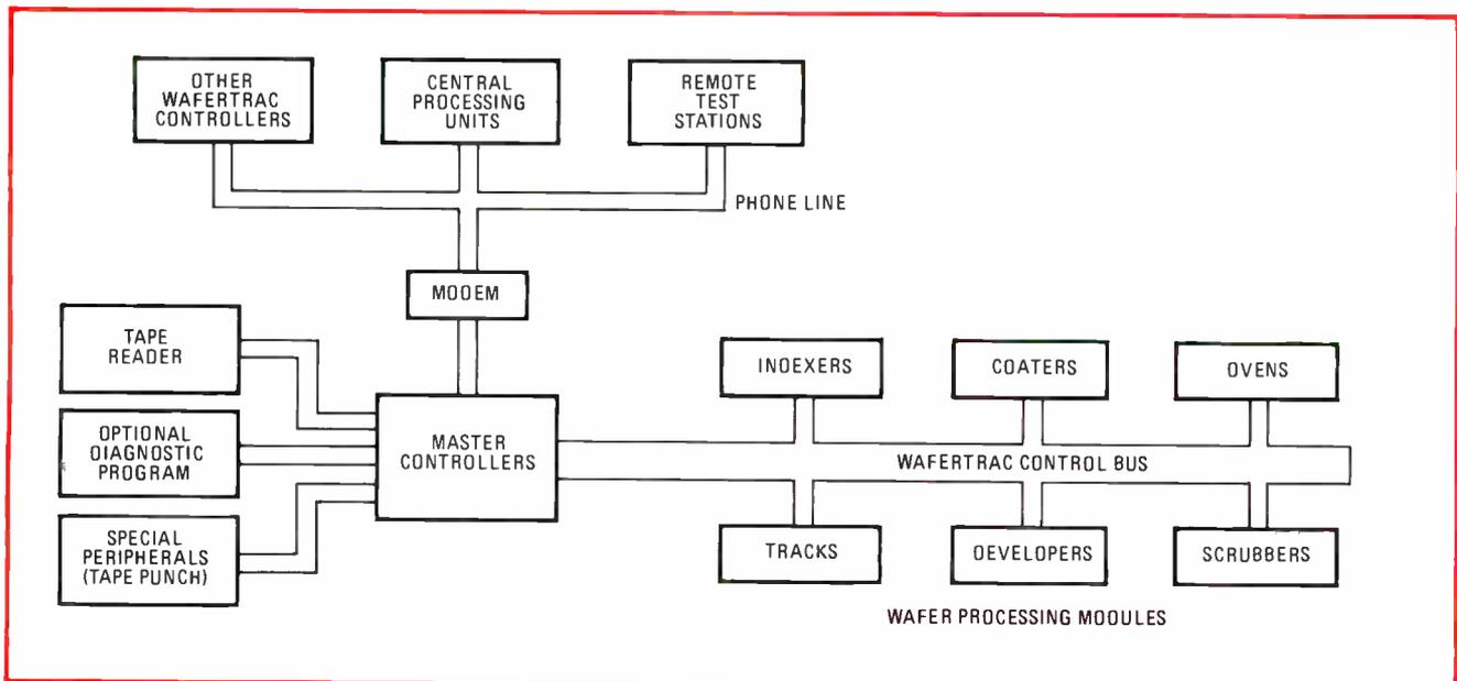
**5. Dial-a-wafer.** The Wafertrac system can be linked over a standard communication bus to other process modules and peripherals. With a modem, the system's microprocessor can communicate over phone lines with a master computer, other Wafertracs, or a remote test station.
