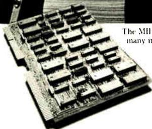
Meet the Plessey MIPROC 16, a 16-bit computer-on-a-card that's faster than any other mini- or micro-computer made.
