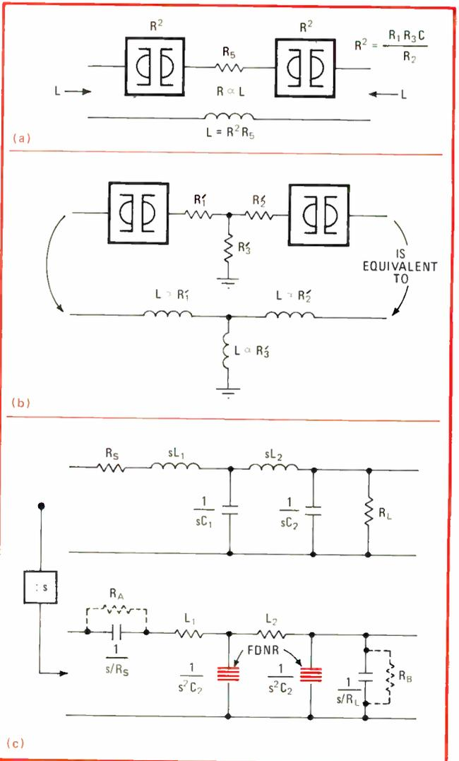
**3. Floating.** Lower terminal of basic gyrator (Fig. 2b) is grounded. To float the circuit, two gyrators may share the same resistor (a), or a network of resistors (b). Floating inductors may also be simulated (c) with functionally dependent negative resistors (FDNRs).
