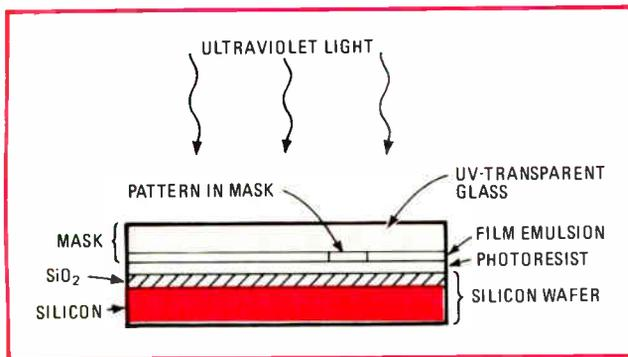
**6. In contact.** Contact printing of IC patterns consists of shining UV light through a chrome or film-emulsion mask that is pressed directly against a resist-coated wafer. Despite the method's deficiencies, it is still the dominant method of IC lithography.
