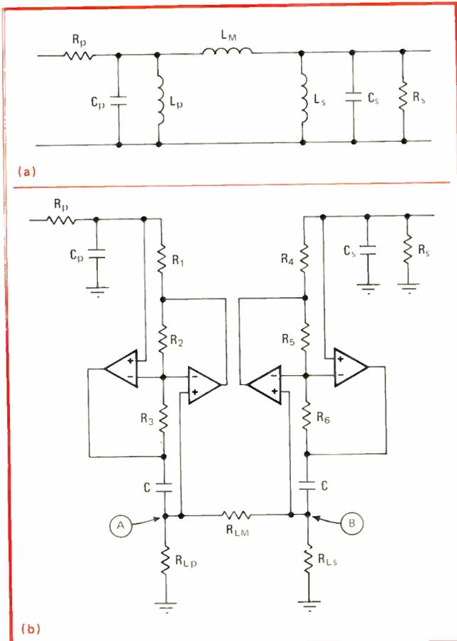
**4. Bandpass filter.** Double-tuned bandpass filter of (a) may be built with two gyrators, as in (b). Sharing resistor  $R_{LM}$ , the grounded gyrators simulate the pi network of inductors in the passive version. All of the amplifiers may be general-purpose devices.
