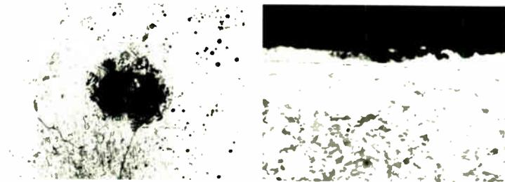
AMP's Materials Research Laboratory pictures of surface oxidation and fretting corrosion on non-lubricated contacts.
