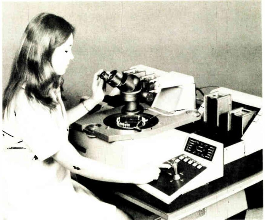
**17. Microprocessor control.** The Electroglas Model 1038 reflects the improvements that IC firms wanted in probers. It is microprocessor-controlled and has a cassette-to-cassette mechanical interface and Z-axis compensation for wafer warpage.
