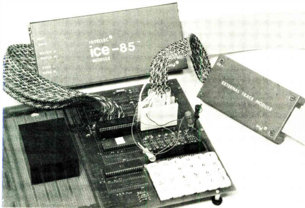
**3. Plug in.** The ICE-85 module has its emulating microprocessor mounted on the cable plug, and 18 trace probes can pick up other signals directly from the prototype circuitry.
