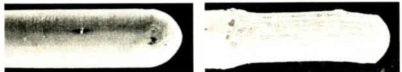
Through the electron microscope, the dramatic improvement AMP Bonded Lubrication makes in contact life and performance is clearly evident.
