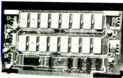
the 8,192-bit memories, the unused sections can be disabled so that a read/write memory can be accommodated within their address space. The board also has provision for a wait state so that it can run in a Z-80 system. Supplied with a full set of integrated-circuit sockets, but without the PROMs, the kit has a small-quantity price of \$85. Delivery is from stock.
