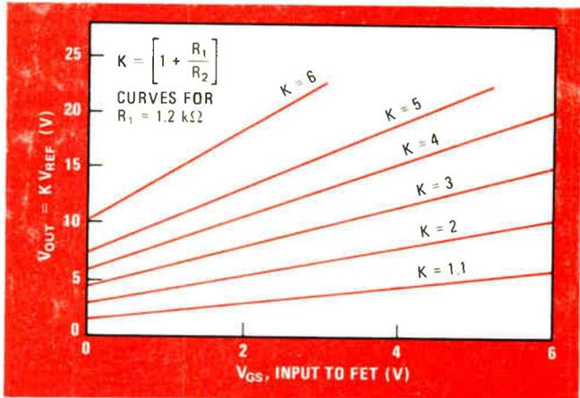
**2. Characteristic equation.** Relationship of scale factor  $K$  to  $V_{out}$ .  $V_{GS}$  is linear as shown by curves. Scale factor is controlled by resistor feedback network at regulator output. FET, used as voltage-controlled resistor, assures output voltage is proportional to  $K$ .
