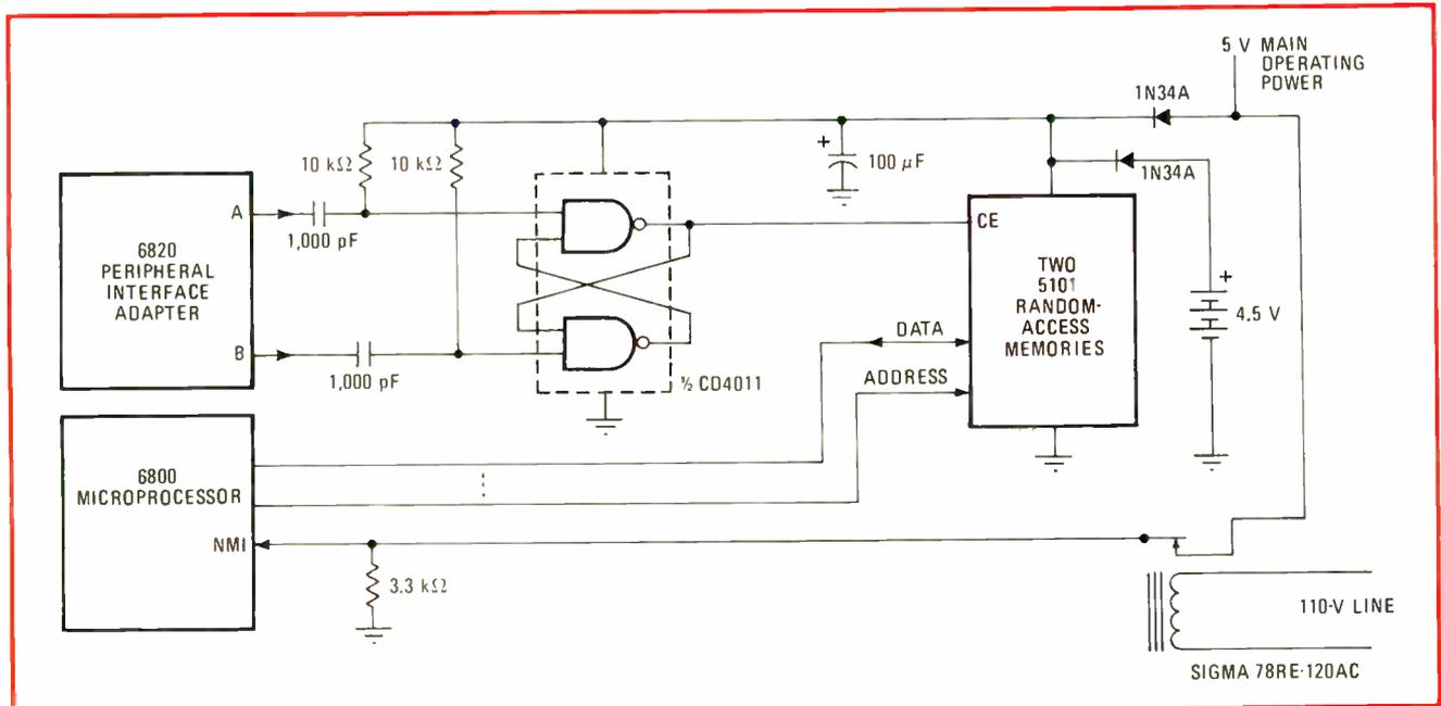
**To the rescue.** Should power to microprocessor or PIA fail, data in their registers is stored in battery-powered RAMs for protection. Control-enable line of RAMs is enabled during normal operation, disabled on power-down to prevent modification of RAM contents.
