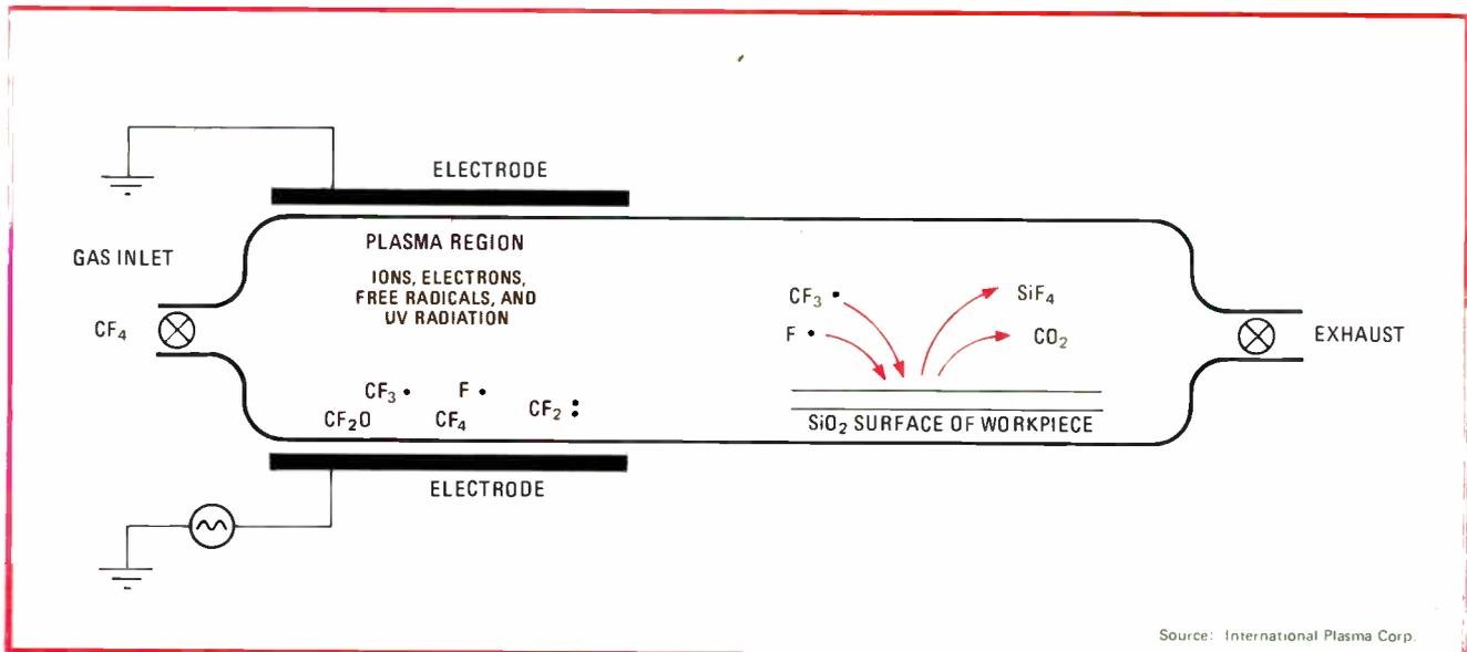
**10. Plasma.** In a plasma reactor during an etching process, plasma is generated in the space between two electrodes. The wafer to be processed lies outside the plasma region, but free radicals survive to reach the wafer and react chemically with the silicon dioxide.
