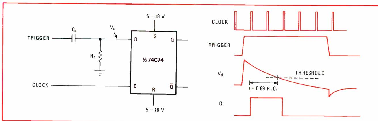
**Monostable controller.** Synchronous multivibrator is formed by differentiator and flip-flop, permitting initialization of clocked system by asynchronous data. Pulse width of multivibrator is determined by time constant of differentiator and clock rate.
