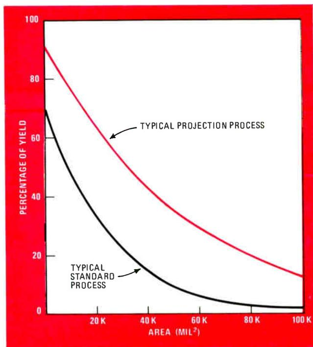
**7. Big chips.** As chip area increases, probe yield goes down. For a usable yield on LSI wafers, many IC firms are switching from contact lithography to projection alignment and printing.
