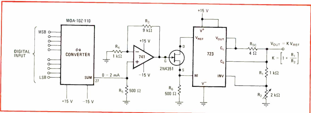
**1. Controlled voltage generator.** Digital-to-analog converter determines output voltage of regulator when FET is used as a voltage-variable resistor. If digital source is computer, specified voltages may be generated for automatic testing of components.
