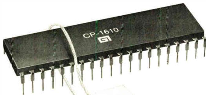
GI has made the unbelievable...believable! You can buy our new powerful CP-1610 single chip 16-bit microprocessor for only \$8.00. Think what that means in terms of your product capabilities and features! Now, for the same price as an 8-bit MPU you can buy all the computing power and designed-in-future of a 16-bit microprocessor.
