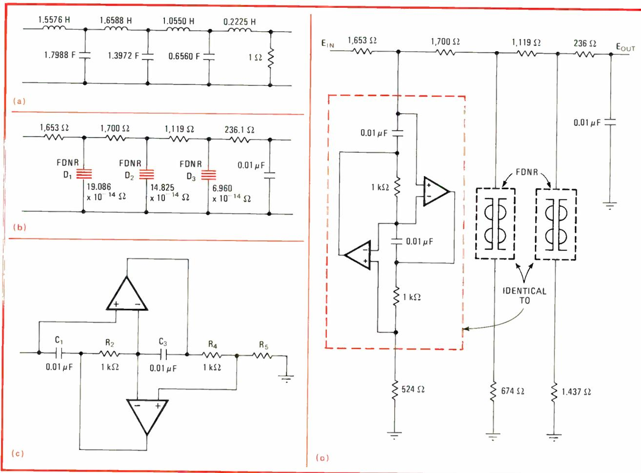
**5. Aliasing filter.** Number of floating inductors in low-pass aliasing filter (a) makes implementation with grounded gyrators difficult. Instead, FDNRs may be used (b), each of which requires two capacitors (c). The final circuit (d) employs only three of these FDNRs.
