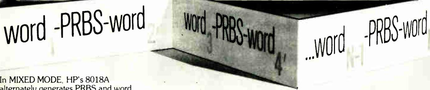
In MIXED MODE, HP's 8018A alternately generates PRBS and word information, simulating preamble-data message-postamble patterns.
