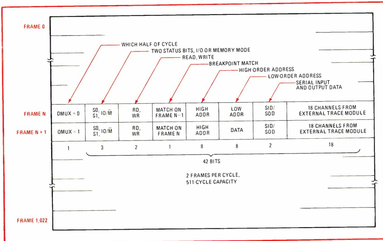
**4. Trace memory.** For logic analysis, the ICE-85 trace memory holds 1,023 frames of 42 bits each. Since the 8085 works on the basis of two frames per cycle, with low-order addresses and data multiplexed in alternate frames, the memory can store up to 511 machine cycles.
