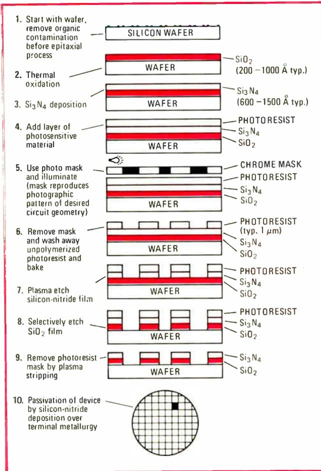
**11. Plasma processes.** A typical process for a silicon wafer shows that plasma processes may be applied for wafer cleaning, oxide etching, resist stripping, and silicon-nitride deposition (passivation).
