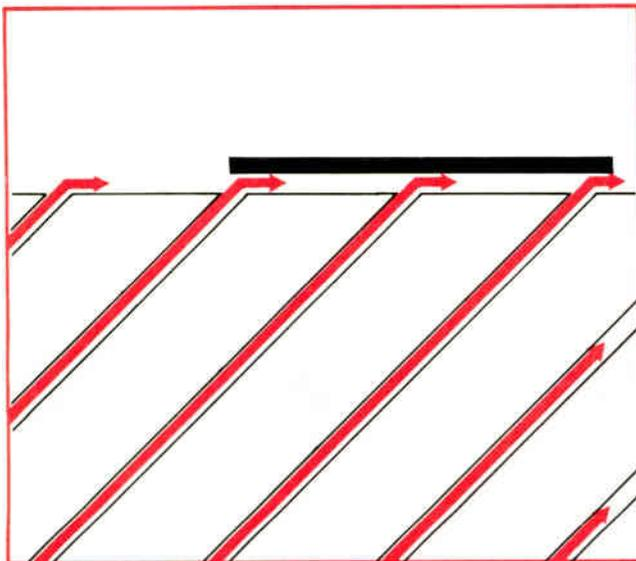
**2. Jet transport.** In GCA's Wafertrac, an air transport system gives gentle touchless wafer handling. The mechanism provides a rolling vortex of air that surrounds, moves, and supports the wafer.
