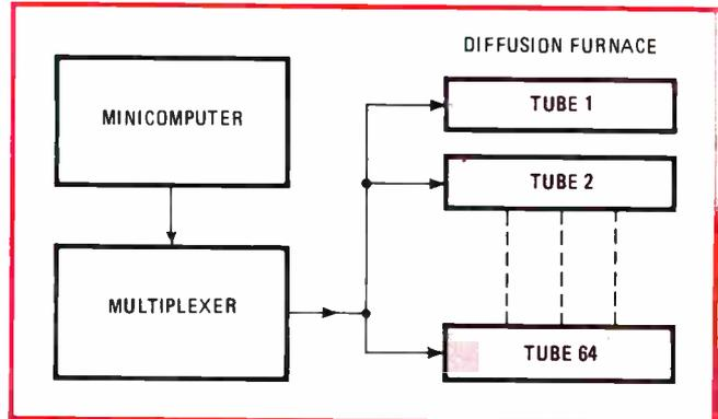
**14. Minicomputer control.** One of the first approaches to automating multiple diffusion tubes was to let a minicomputer with a multiplexer act as the master controller. However, failure of either of these components disables all the diffusion tubes.
