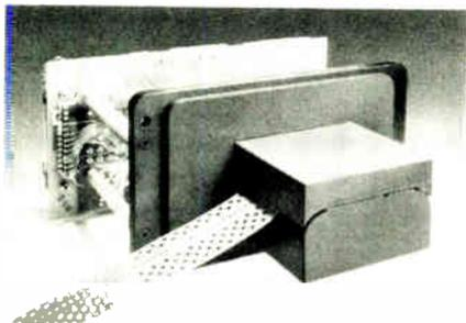
skewed or otherwise imperfect tape. The head, which is made of a highly wear-resistant material, will not accumulate static charges—another way in which it tends to lower the reader's error rate.
