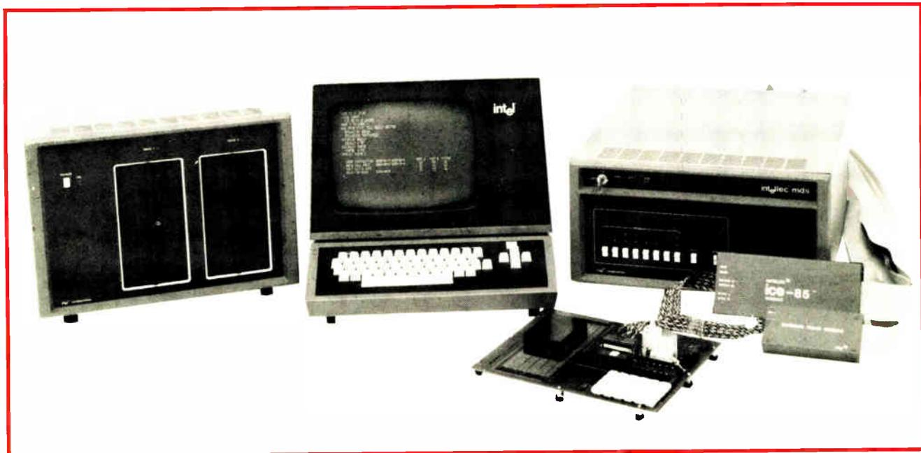
in the signal cable. Previous emulators, typified by the ICE-80 developed for the 8080A, can operate only up to about a 2-megahertz clock rate, whereas the ICE-85 emulation module can run at the 8085's 3-MHz rate or even at higher speeds.
