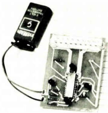
**Game guts.** TI board in Parker's sub chase game holds microprocessor, resistors, discrete LEDs and, under lenses at top, segmented LEDs. Wires go to keyboard.
