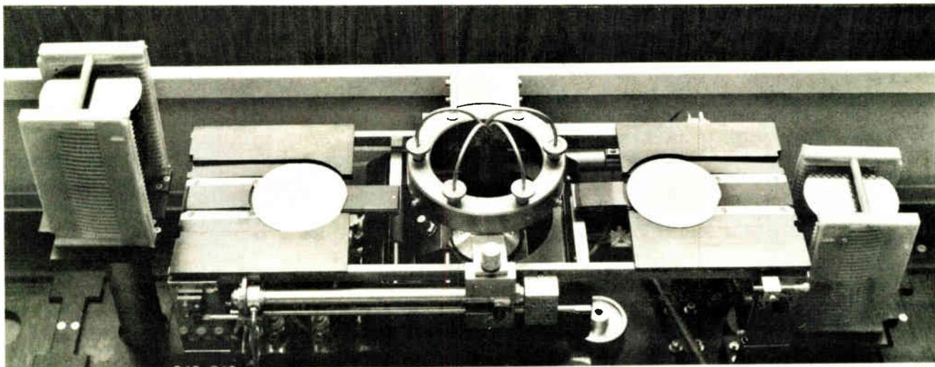
**3. Untouched by human hands.** Pneumatically driven teflon supports transport wafers in Macronetic's in-line wafer-processing equipment. Wafers move from the left cassette to the transport, through a scrubber, to the right transport, and back to a cassette.
