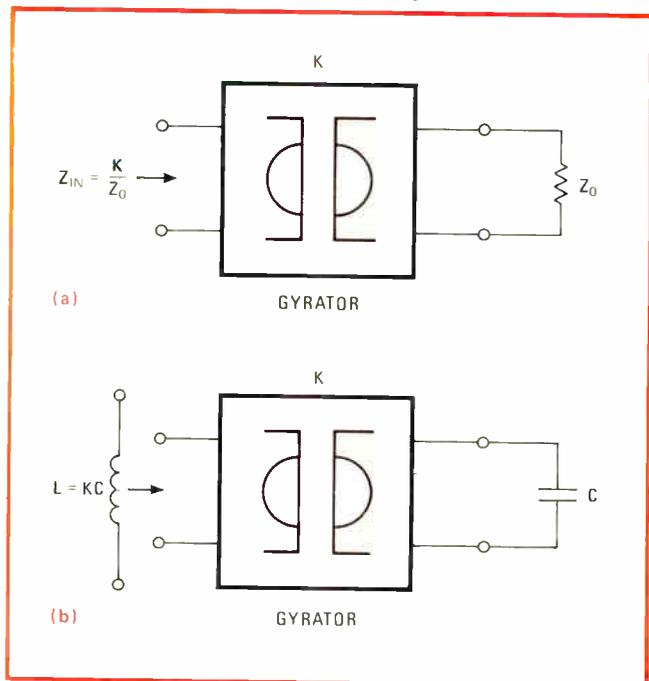
**1. Ideally.** Coupled LC filters simulated with gyrators have characteristics approaching the ideal. In effect, the gyrator is a lossless two-port circuit (a) that inverts a load impedance. With a capacitive load impedance, the circuit (b) simulates a high-quality inductor.
