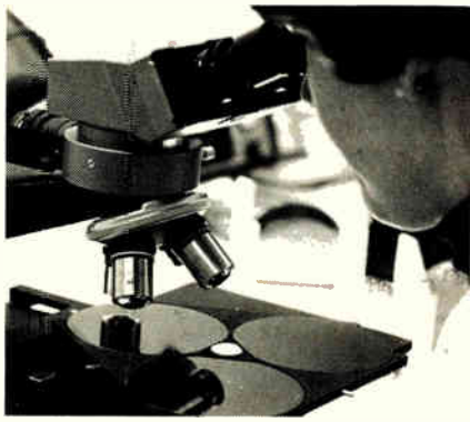
A good look. Frances McLaughlin inspects 4-inch wafers at National Semiconductor plant in Greenock, Scotland, before the masking-etch step.
