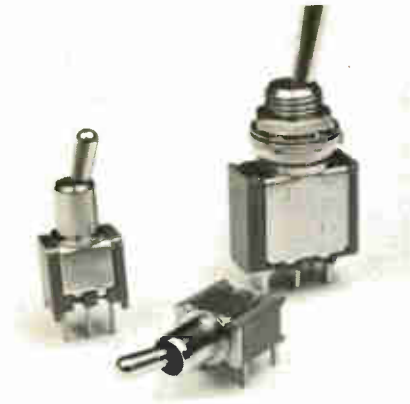
Subminiature single- and double-pole toggle switches, with right-angle or standard lugs, for printed-circuit boards are designed for low-level 0.4 VA maximum, 20 V dc or ac. Minimum level is 100 \mu V. They feature self-extinguishing blue diallylphthalate bodies. APEM, BP 1, 82300, Caussade, France[458]
