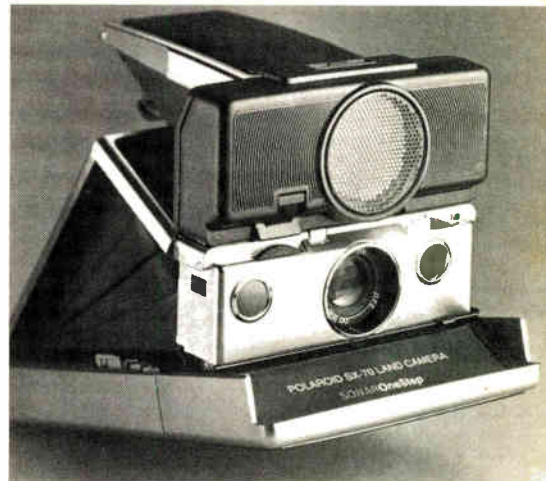
Ranger. Sound waves created by electrostatic transducer helps new camera find range. Motor focuses lens according to time for sound to hit target and return.
