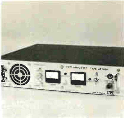
A traveling-wave amplifier, type AF 161P, is designed to be incorporated into ground-based microwave-landing systems in the 5.00-to-5.25-GHz frequency band and fits into 19-in. racks. ITT Components Group, Electron Device Product Group, Brixham Road, Paignton, Devon, England[457]
