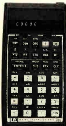
**HP-33E. Programmable Scientific.** 49 program lines of fully merged key codes. Editing, control, and full range conditional keys, plus 8 user memories.
