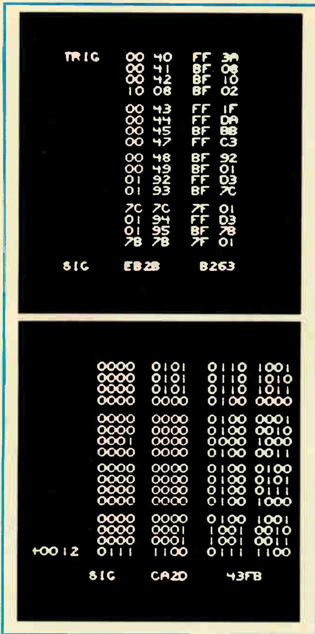
**3. Identifying data.** The data in the model 532 main memory can be displayed in the form of 16-word pages on a scope in hexadecimal (top) or binary (bottom), along with the identifying signatures.
