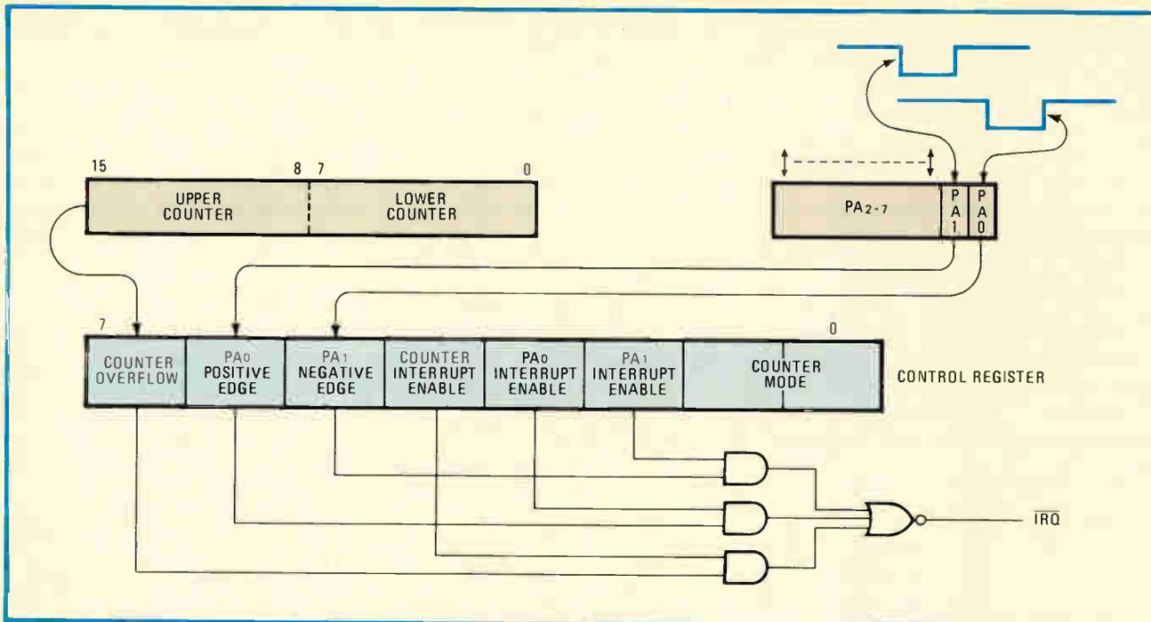
**5. Interrupts.** The  $\overline{IRQ}$  interrupt request originates from three sources that are each software-maskable: the rising edge at pin  $PA_0$ , the falling edge at  $PA_1$ , and counter overflow. The other interrupt,  $\overline{NMI}$ , is non-maskable and is used for critical events such as power failure.
