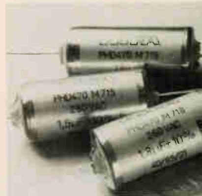
Metalized polypropylene capacitor PHD 470 can be used for many ac applications, particularly in motor circuits and for coupling. Its range is from 1.5 to 3.0  $\mu\text{F}$ , and its tolerance is  $\pm 10\%$ . It operates at 260 V ac at 50 Hz. RIFA, Fack, S-161 11 Bromma, Sweden [462]
