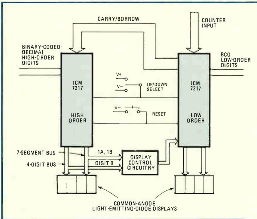
**Up-down eight-digit counter.** When two 7217 four-digit devices are used in tandem, the low-order stage's carry/borrow bit becomes the high-order stage's input.
