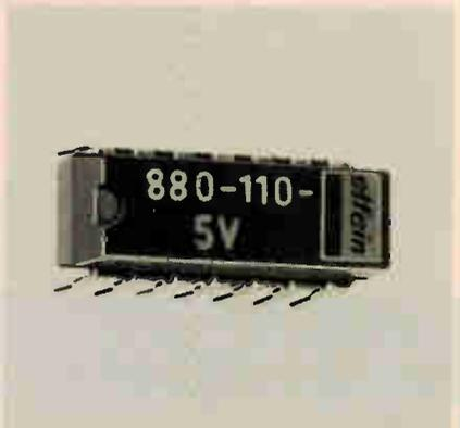
Featuring bounce-free mercury contacts, dual in-line reed relay Q43 handles 300 mA and 28 V at a 10-W switching power. Transfer resistance is 100 m $\Omega$ ; maximum deviation, 10 m $\Omega$ . Life is between  $5 \times 10^6$  and  $5 \times 10^7$  operations. Elfein GmbH, 6 Frankfurt, Wienerstr. 120, West Germany [458]
