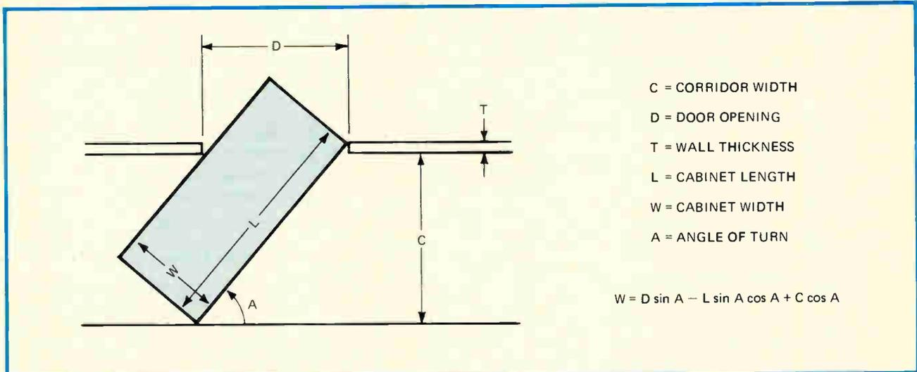
**Tight fit.** HP-25 program finds the largest equipment-cabinet width, W, that just allows it to pass through door opening. Calculation stops when the maximum value of W is found or when it is determined that the cabinet corner just clears the wall.
