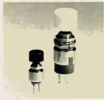
The 9100 momentary push button is 6.5 mm in diameter and 17.5 mm in overall length. Its contact resistance is less than 30 mΩ and its insulation resistance is greater than 1,000 MΩ measured at 500 V. It has a life of 300,000 operations. APEM, B. P. 1, 82300 Caussade, France [450]
