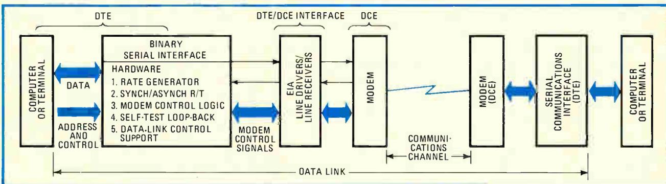
**1. Linkage.** Modems, serial communications interface, and communications channel are all part of basic data-communications link. Data-link controls are needed only for the link, not for the computer or its peripherals. The modem can also be a data-service unit for Dataphone digital service, a line driver and line receiver (modem eliminator), or an interface with a satellite or microwave channel.
