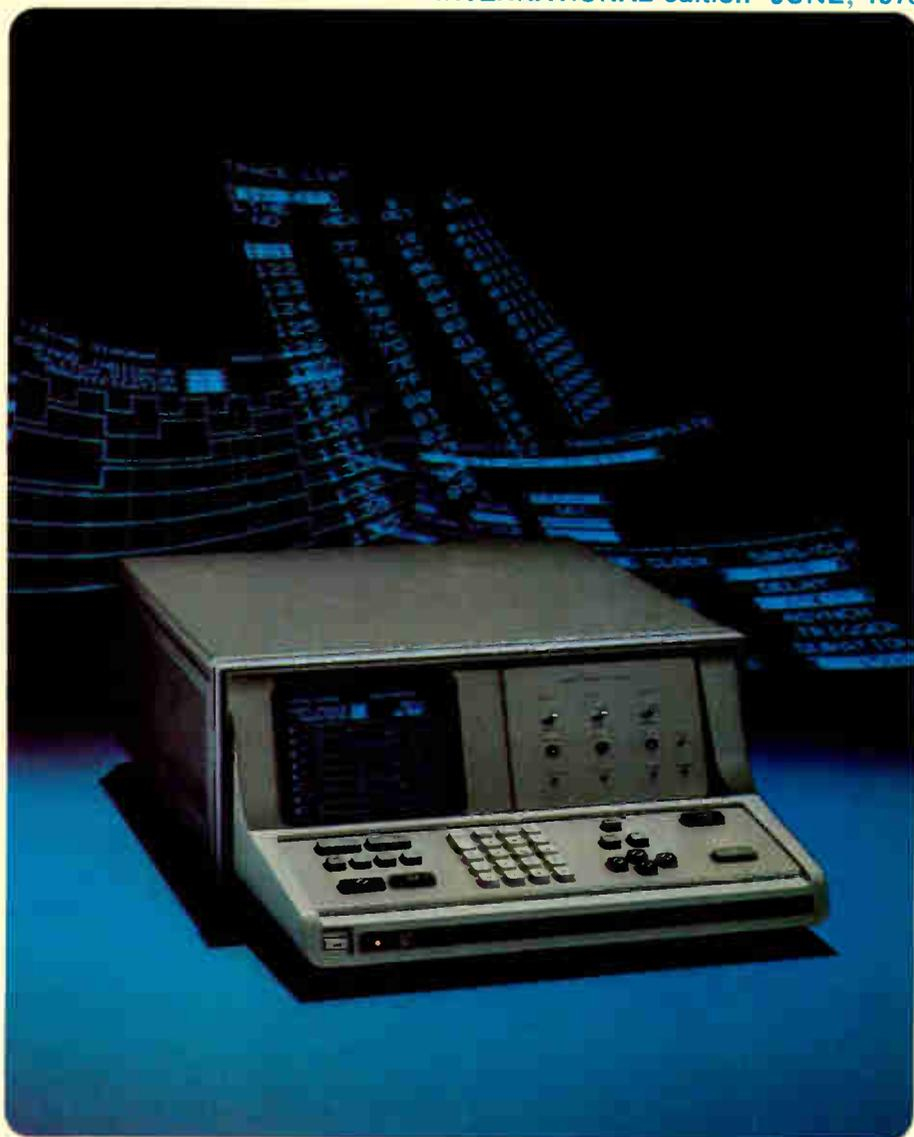
Simultaneous state, timing, and interactive measurements, plus glitch triggering make this logic analyzer a powerful tool for both hardware and software designers. Simple keyboard entries to pin-point areas of interest in system activity also save development and debugging time of synchronous and asynchronous digital systems.
