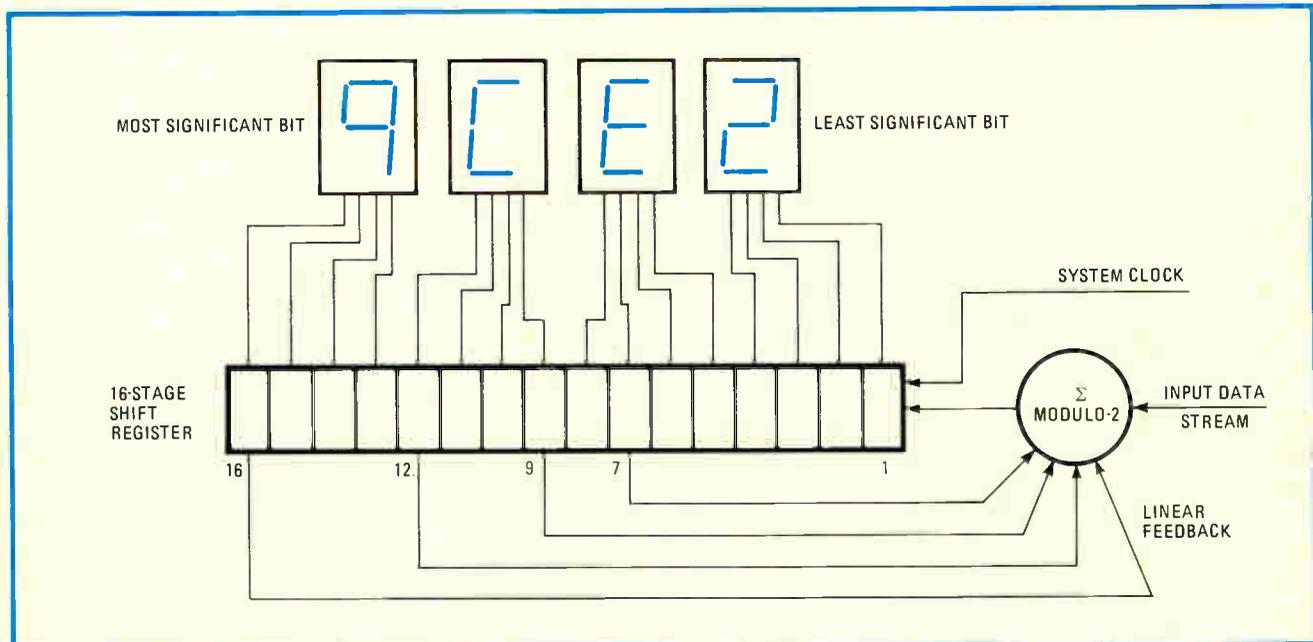
**2. Watching digits.** In the basic signature analyzer, a single-channel probe catches a pulse train unique to the node under examination. Passing this train through a linear feedback register gives an identifying signature that can be compared with that of a known-good node.
