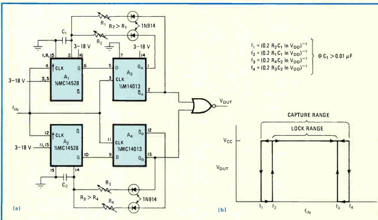
**Within limits.** Circuit (a) detects whether input signal is within user-set frequency range  $f_2$ – $f_3$  (b). Flip-flops enable selectable hysteresis so that circuit, once locked, will not change state until  $f_{in}$  moves below  $f_1$  or moves above  $f_4$ . Lock and capture ranges are controlled by  $R_1$ – $R_4$ . Hysteresis eliminates jitter that would normally occur at output if  $f_{in}$  were near  $f_2$ 's or  $f_3$ 's edges.
