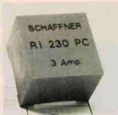
The RI-200 series of compact chokes is designed to suppress radio-frequency interference for thyristors and triacs. They are vacuum-molded in polyurethane for protection against moisture and are suitable for printed-circuit-board mounting. Schaffner, CH-4708 Luterbach, Switzerland [461]
