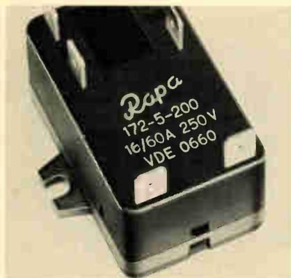
Designed for consumer and industrial applications, power relay 172 operates with ac or dc. It handles about 3,500 VA at a maximum continuous current of 16 A. Two working contacts are spaced 3 mm apart. Rausch & Pausch, 8672 Selb, P. O. Box 1540, West Germany [451]
