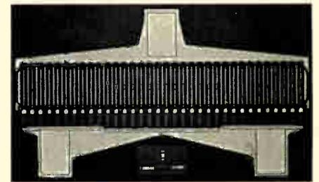
Internal matching at input enables broad bandwidth designs with this 34-finger ballasted transistor.
