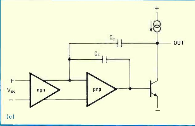
To simplify biasing in a standard bipolar op amp, a current mirror makes the conversion from a differential to a single-ended stage at the output of the first stage. But this approach does not work with a JFET differential input stage. Such a bipolar current mirror would yield much too large an input offset voltage when the JFET was biased for maximum slew rate. The low transconductance of this transistor actually causes the input to exceed the offset voltage of the mirror.
