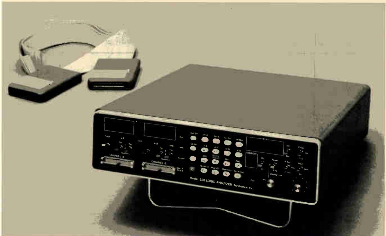
**Fast service.** Combining the best of two analyzer worlds, the model 532 captures 250 32-bit words of logic-state data and automatically computes and displays two associated signatures that identify faults in the microprocessor-based system under test.
