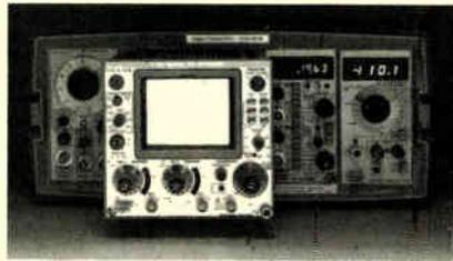
beam modulation input—both of which are also in the rear—this allows interconnection with other TM 500 plug-in modules, such as pulse generators, function generators, digital and universal counters, digital multimeters, a logic analyzer, and others. With the SC 503, users should be able to assemble measurement systems that are well suited for medical or biophysical applications, as well as for a variety of electromechanical measurements.
