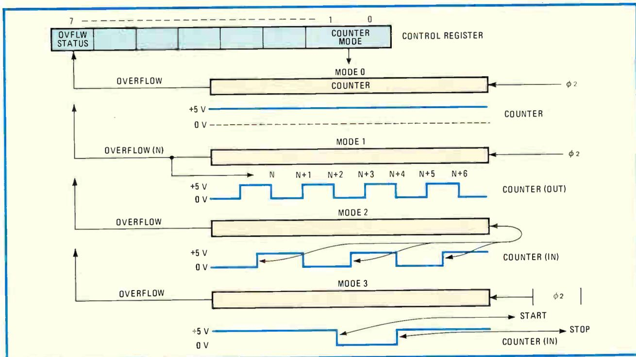
**4. The counter.** The four-mode counter is programmed by 2 bits in the control register. Modes 0 and 1 are both free-running, the latter toggling the CNTR pin on overflow. Mode 2 counts down with each rising edge on CNTR, and in mode 3 CNTR gates the countdown.
