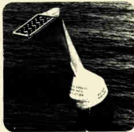
**Solar energy** is used to re-charge the storage battery aboard each of the forty survey buoys currently performing a marine study in the Indian Ocean. Continuously monitored data is automatically transmitted from each buoy every hundred minutes via the Nimbus-Six satellite. The study is being carried out by the Commonwealth Scientific and Industrial Research Organisation (CSIRO). Philips supplied the solar collector panels.
