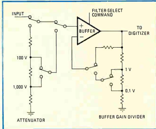
**4. Stable elements.** The accuracy of the 6000 depends on the design of the input attenuator and the stability of the isolating buffer amplifier, which also contains a selectable filter to combat noise.
