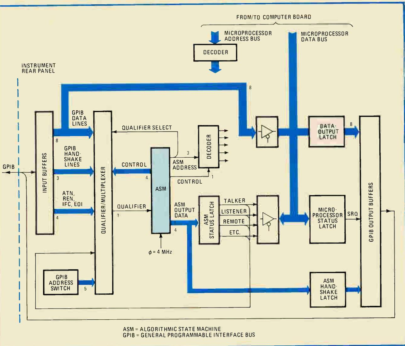
5. Interface board. A self-contained IEEE-488 interface board is controlled by an algorithmic state machine. The board operates independently of the microprocessor. A BCD interface that occupies the same address space is also available.
