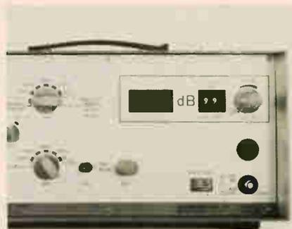
Semiautomatic attenuation tester DT-1 feeds a 1-kHz sine-wave noise signal into the line and then measures noise level with its built-in level meter. Automatic range selection of results simplifies operation. Felten & Guillaume, 5 Cologne 80, P. O. Box 805001, West Germany [460]
