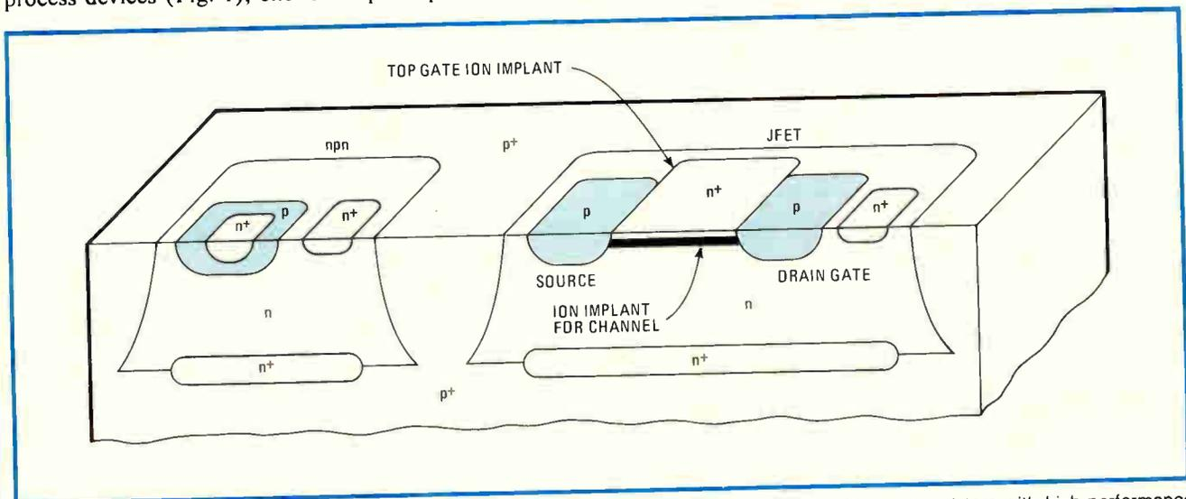
**1. Basic structure.** Because of ion implantation, bi-FET circuits can combine high-performance bipolar transistors with high-performance matched JFETs. One implant creates the p channel between source and drain contacts, another the gate region over this channel.
