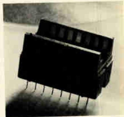
The TSN integrated-circuit socket will permit high-density mounting on pc boards for increased burn-in oven production. It measures 12.53 mm wide, accommodating a 16-pin unit. Astralux Dynamics Ltd., Brightlingsea, Colchester, Essex, CO7 0SW, England [464]
