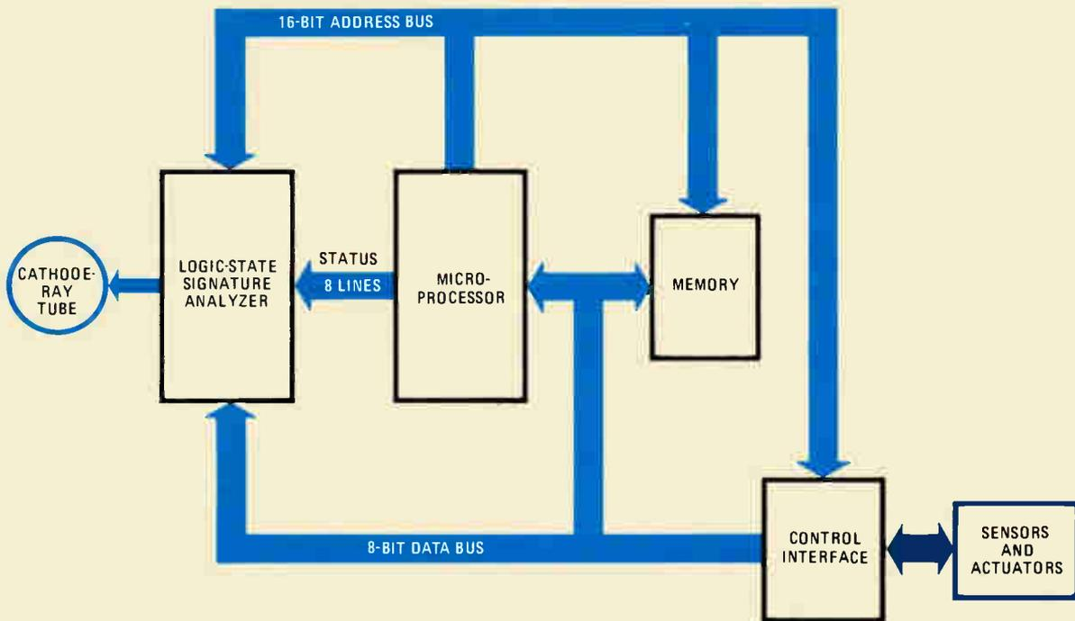
**4. Checking a controller.** In monitoring the performance of a microprocessor-based industrial controller, the 532 is first used with the product operating under laboratory conditions. Then it looks for signature changes as the environmental conditions are varied.
