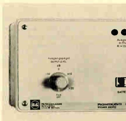
Speech-noise generator model RGS-1, for speech simulation on telephone channels, produces a quasi-random noise signal using MOS shift registers. An active RC filter performs a spectral evaluation. Felten & Guillaume, 5 Cologne 80, P. O. Box 805001, West Germany [452]
