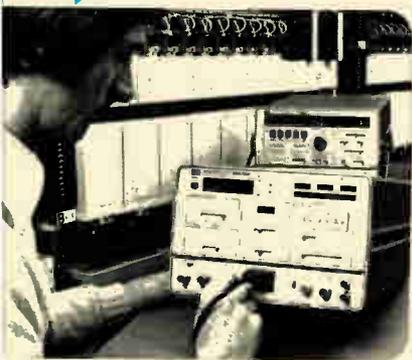
Hewlett-Packard's new 3771A performs troubleshooting measurements to CCITT standards on high speed data transmission lines. When used with the existing HP 3770B Telephone Analyzer, shown in background, they provide a complete, portable data line test system.
