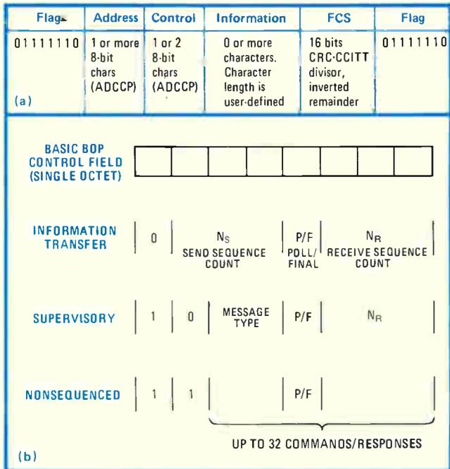
**3. Frame format.** With a BOP, only one frame format (a) is necessary. Each station attached to the link searches for the flag sequence and for an address sequence. For multipoint links, each station must detect a flag immediately followed by its address to activate the receiver. The heart of the BOP message is the control field (b). It determines message type and send/receive sequence counts.
