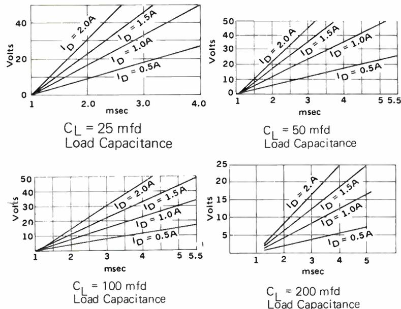
$I_D$  = Difference between programmed current and constant load current.
