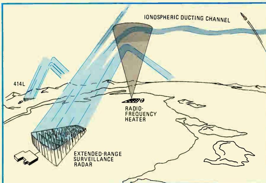
**Long-distance radar.** The tunneling or ducting effect in the ionosphere could provide a means of using long-range radar signals injected into the duct via rf "heaters."
