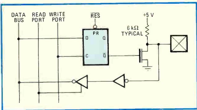
**3. No direction.** The bidirectional input/output lines require no direction register. Normally written to 1, an input is overridden by a 0, which latches the D-type flip-flop driving the transistor low. The 6-kilohm pull-up resistor can be omitted with a mask option.
