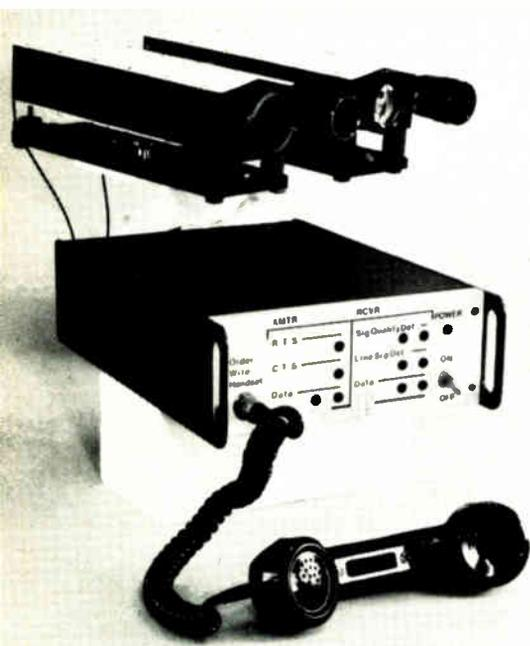
**Many uses.** A GaAs laser unit, designed for secure data transmission over fiber-optic cables, is serving as a line-of-sight teletypewriter link. It also can carry voice traffic.
