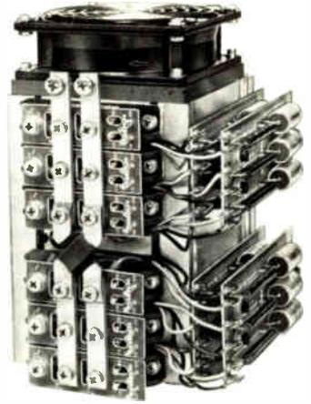
The SEMIPACKS are available as components or integrated in a completed assembly. The unit shown above is a quad drive circuit employing 6 SEMIPACK. Our engineers will design a custom assembly to meet your specific need.
