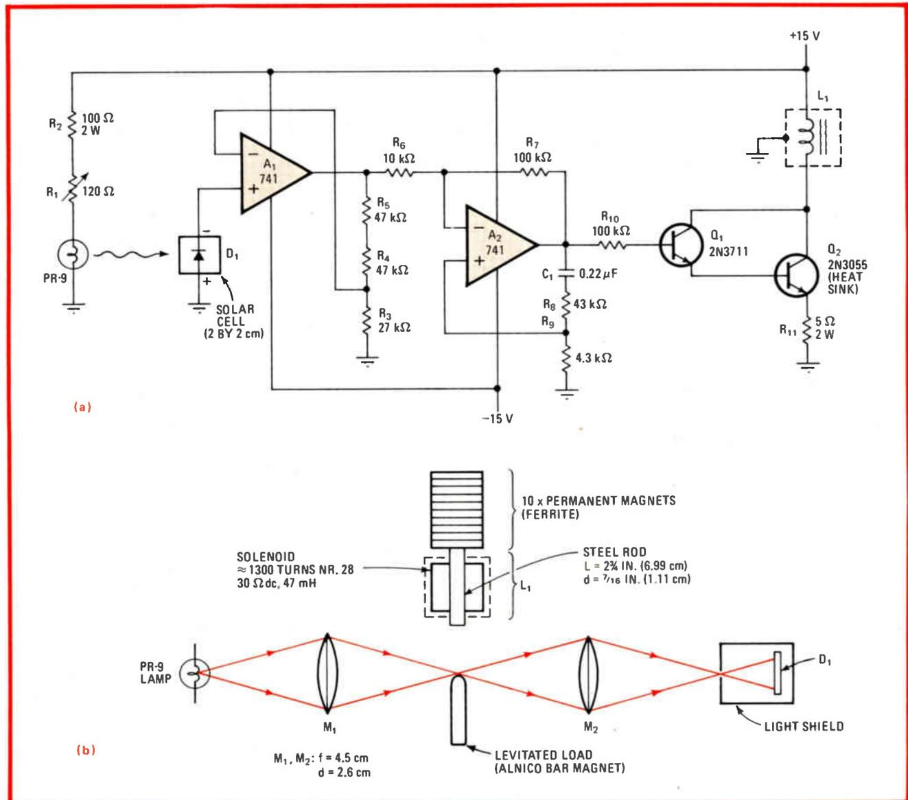
**Rising rotors.** Levitator circuit (a) suspends 1-in. steel spheres up to 2 1/2 millimeters off reference surface. Optical arrangement (b) sets object distance. Details of levitation coil construction are outlined. Permanent magnets set ultimate levitation range.
