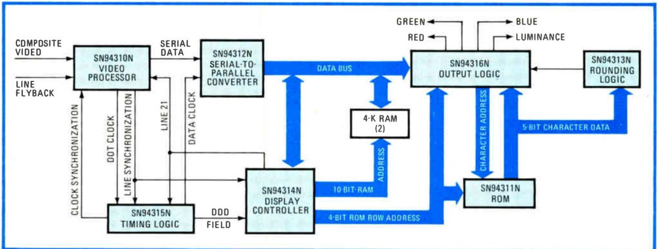
**Six chips.** Texas Instruments has developed a six-chip set that turns digitally transmitted codes into subtitles not otherwise visible on the TV screen. There also is a random-access memory that temporarily stores the data necessary for character generation by the ROM.
