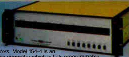
**Pulse Generators.** Model 154-4 is an automatic pulse generator which is fully programmable with its IEEE-488 interface and the Model 3520 Controller. Model 154-4 provides a repetition rate of 10 Hz to 50 MHz, pulse delay and width from 10 ns to 10 ms, and outputs of 0.5 to 10 V within a -10 to +10 volt window. An exceptionally versatile instrument for the systems user.
