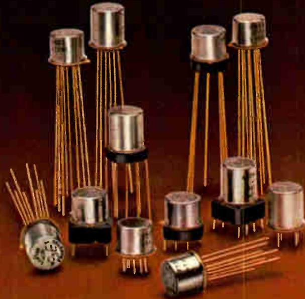
When we originally developed the TO-5 relay, it was designed to meet the stringent size, weight, and power drain requirements of military aerospace and avionics applications. It met them so much better than anything else on the market that it soon became the industry standard, and spawned a whole family of descendants.
