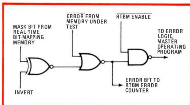
**3. Error-processing logic.** NAND gate at right hides error signal when RTBM is enabled so that pattern processor keeps running. To count bit errors, 1s from masked catch RAM are inverted and combined with 0s in place of error signal from memory under test.
