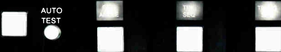
**Auto Test.** Initiate this automatic routine and the Model 101 tells you if it's correctly calibrated. If not, the control panel display identifies the required adjustments.
