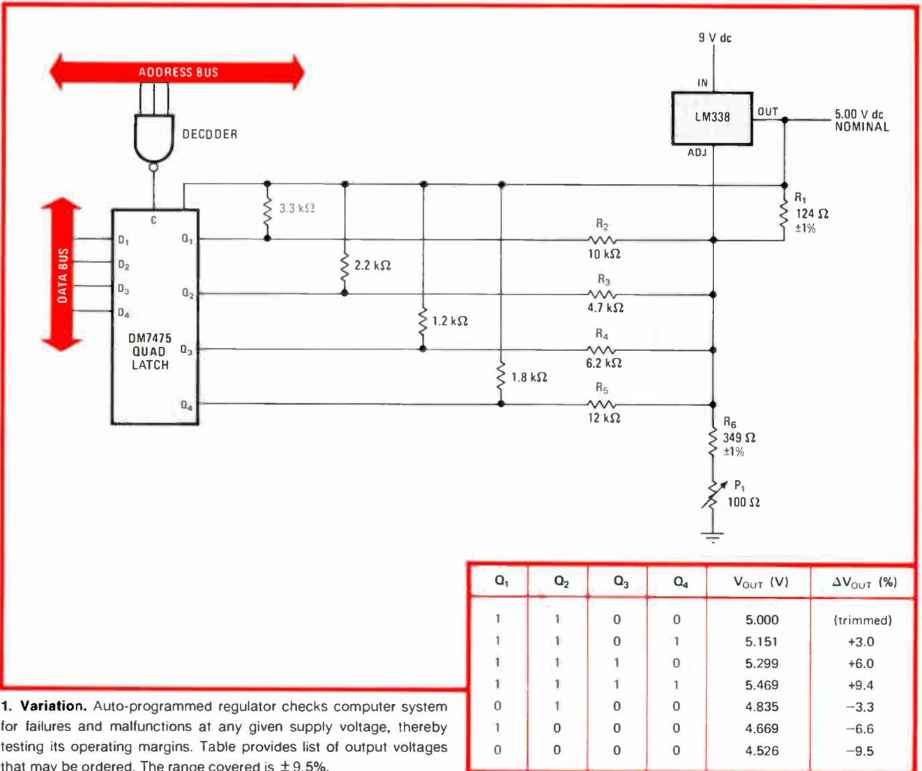
**1. Variation.** Auto-programmed regulator checks computer system for failures and malfunctions at any given supply voltage, thereby testing its operating margins. Table provides list of output voltages that may be ordered. The range covered is  $\pm 9.5\%$ .
