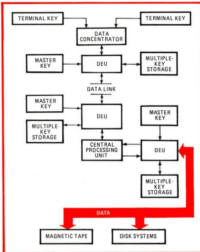
**6. Computer safety.** Three DEUs are needed for this system, which consists of remote terminals, a CPU, and magnetic memories. A separate key may be specified for each reel of tape or disk.
