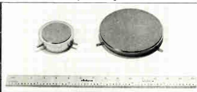
Systems for MBE growth over one and two inch wafers
