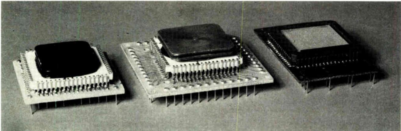
4. DIP-like chip-carriers. An adapter that makes a chip-carrier with leads on 50-mil centers look to the printed-circuit board like a DIP with leads on 100-mil centers can simplify the problem of designing boards for mixed arrays of SSI chips in DIPs and LSI chips in carriers.
