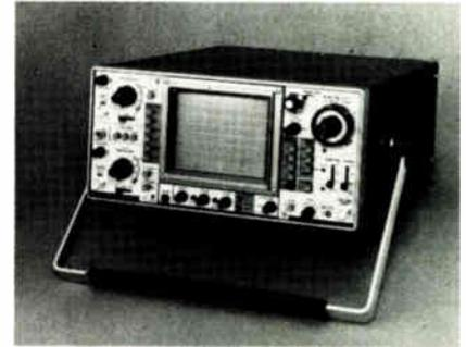
fier increases this sensitivity to 1 mv/cm. A signal-out port on one channel permits the scope to be used as a preamplifier for other instruments. It also allows cascading of the two vertical amplifiers for increased sensitivity.
