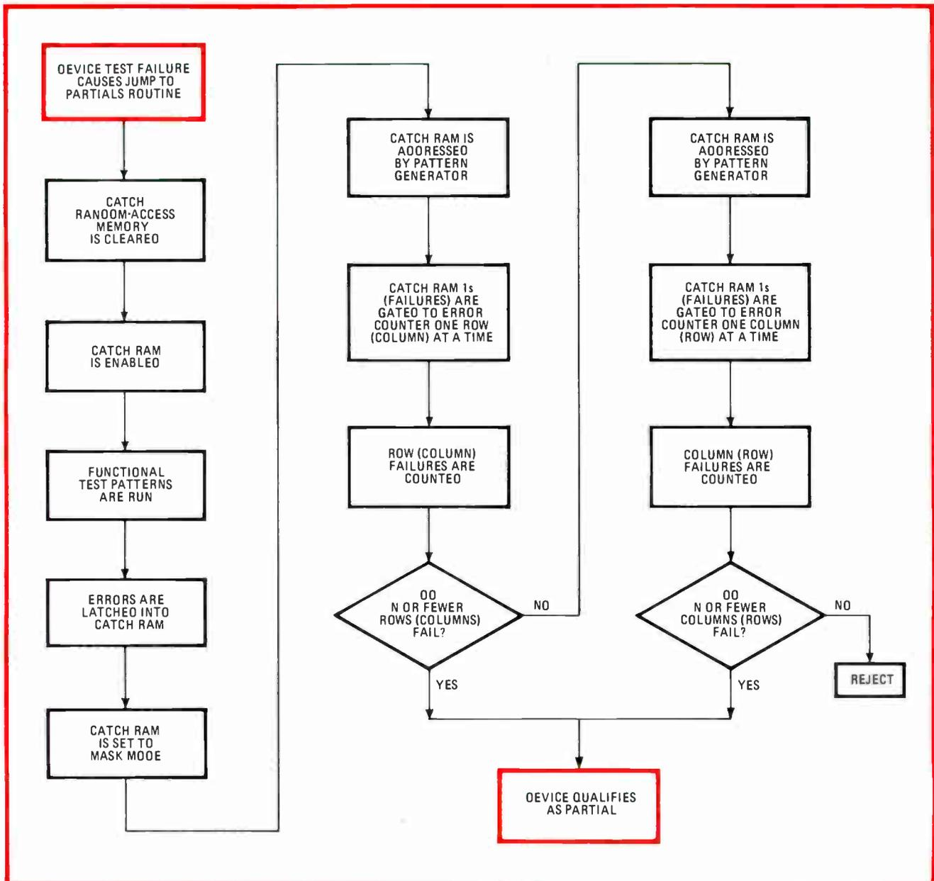
**4. Complete partial test.** Partial testing program is linked to device test routine so that when a failure occurs during normal testing the partial test is called automatically. Clearing the catch RAM and checking its contents by row and/or column adds very little to total wafer test time.
