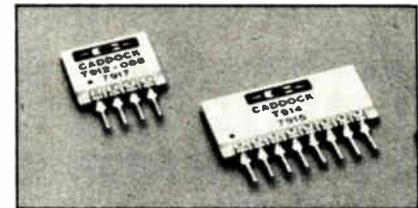
**Caddock's Type T912 and T914 Precision Resistor Networks.**
