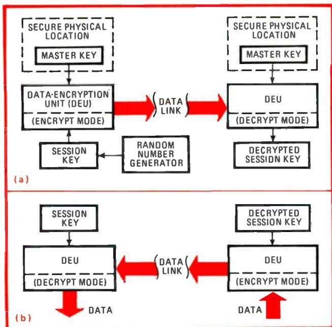
**5. Pick a key.** The S6894-2 can be used in the master-key (a) or the session-key (b) mode. Two new commands are required for two-key operation. These are included in software.
