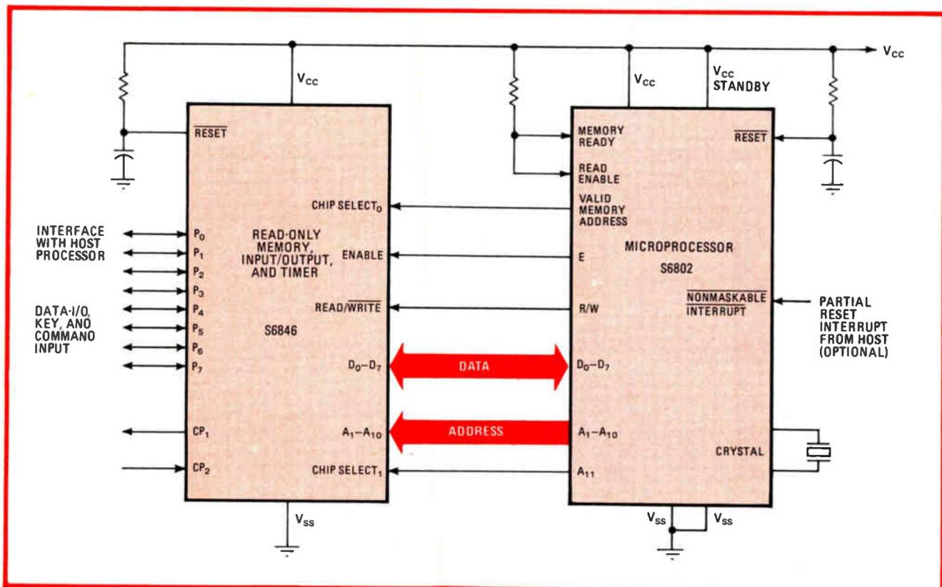
**1. Encryption brothers.** American Microsystems' S6894, a two-chip data-encryption and -decryption unit, contains an S6802 microprocessor and an S6846 read-only memory that also has I/O and a timer. Models handling data rates of up to 11,500 bits per second are available.
