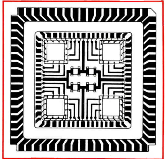
**6. Eye to the future.** A four-chip hybrid on a simple one-layer substrate not only is an immediately cost-effective package for SSI chips that lets all leads be directly wired to the board, but can also be replaced by one gate-array chip later without board redesign.
