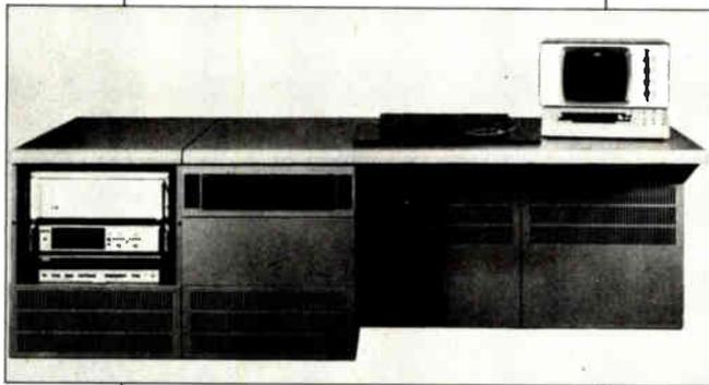
In addition to its super system speed, Series 70 offers faster, more accurate fault isolation. It features multiphase clocks, which let you program timing increments with 20 ns resolution. And its new dynamic current measurement technique lets you track bus-related faults at full system speed.
