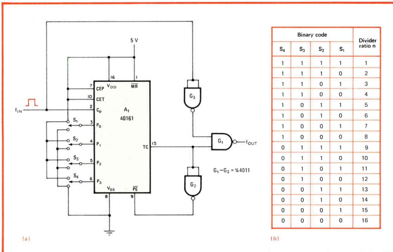
**Binary breakup.** Single counter and three gates simplify design of variable-modulo divider (a). Binary switches  $S_1$ - $S_4$  set counter to  $16 - n$ , where  $n$  is desired divider ratio (b). Output of gate  $G_1$  is a pulse with a frequency equal to  $f_{out} = f_{in}/n$ , for  $1 \leq n \leq 16$ .
