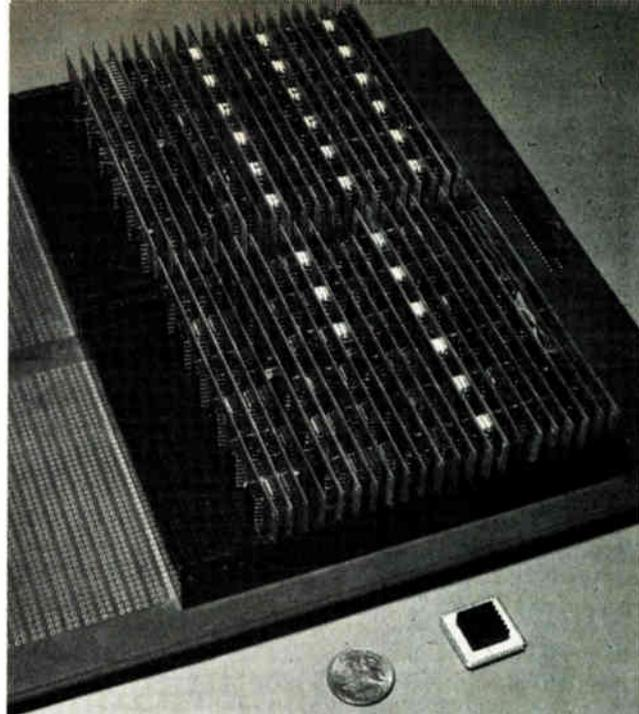
**3. Large is small.** The large-scale integrated circuit in the foreground is equivalent to the 220 small-scale integrated circuits in dual in-line packages behind it. A practical system average of 150 SSI chips replaced by one LSI chip can be achieved without much difficulty.
