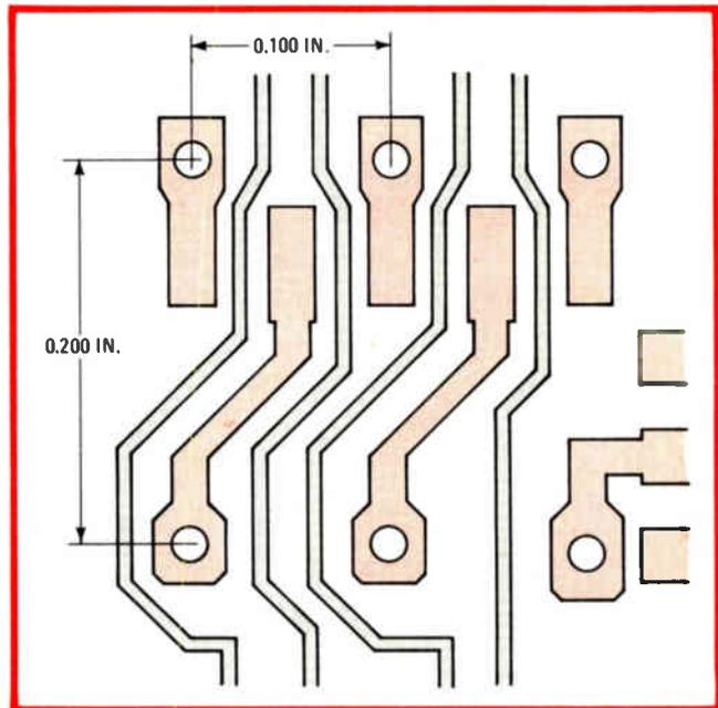
**8. Room at the pad layer.** Staggering the chip-carrier with respect to the via grid allows printed wiring to be put on the same layer with the 50-mil-spaced carrier pads, saving an internal layer. Four-layer boards with 68-lead carriers have been fabricated with this scheme.
