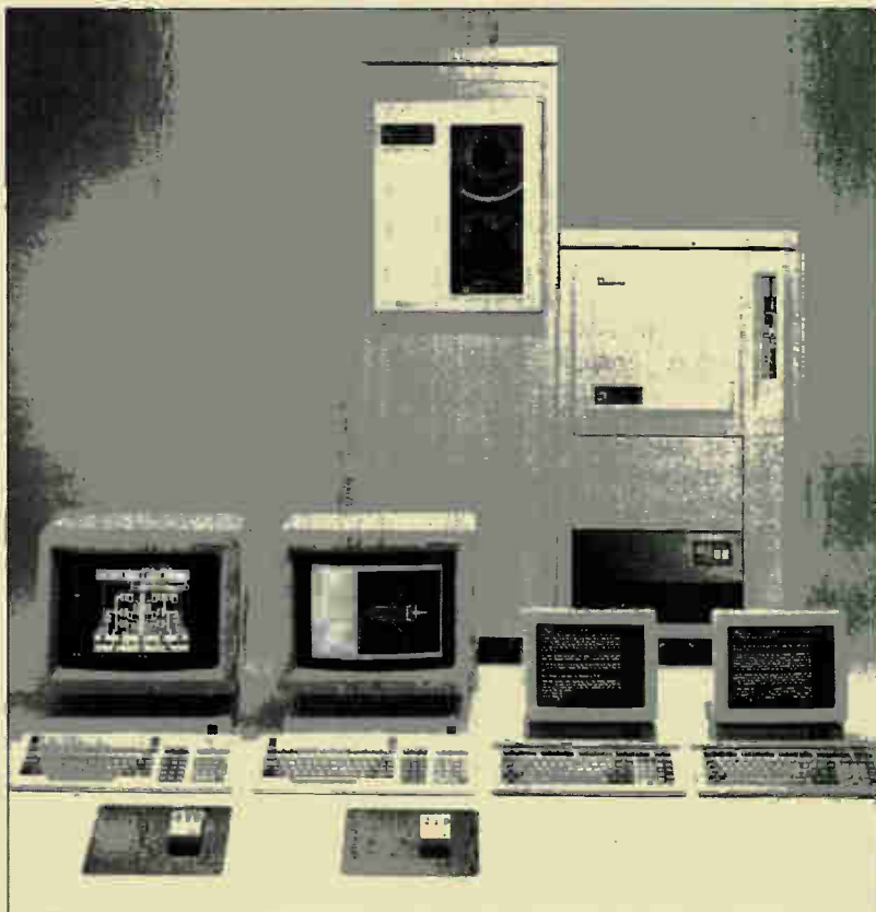
6. MULTIMICRO. The Masscomp MC5700 is a multiprocessor 68020-based midrange computer for scientific, laboratory, and engineering applications.
