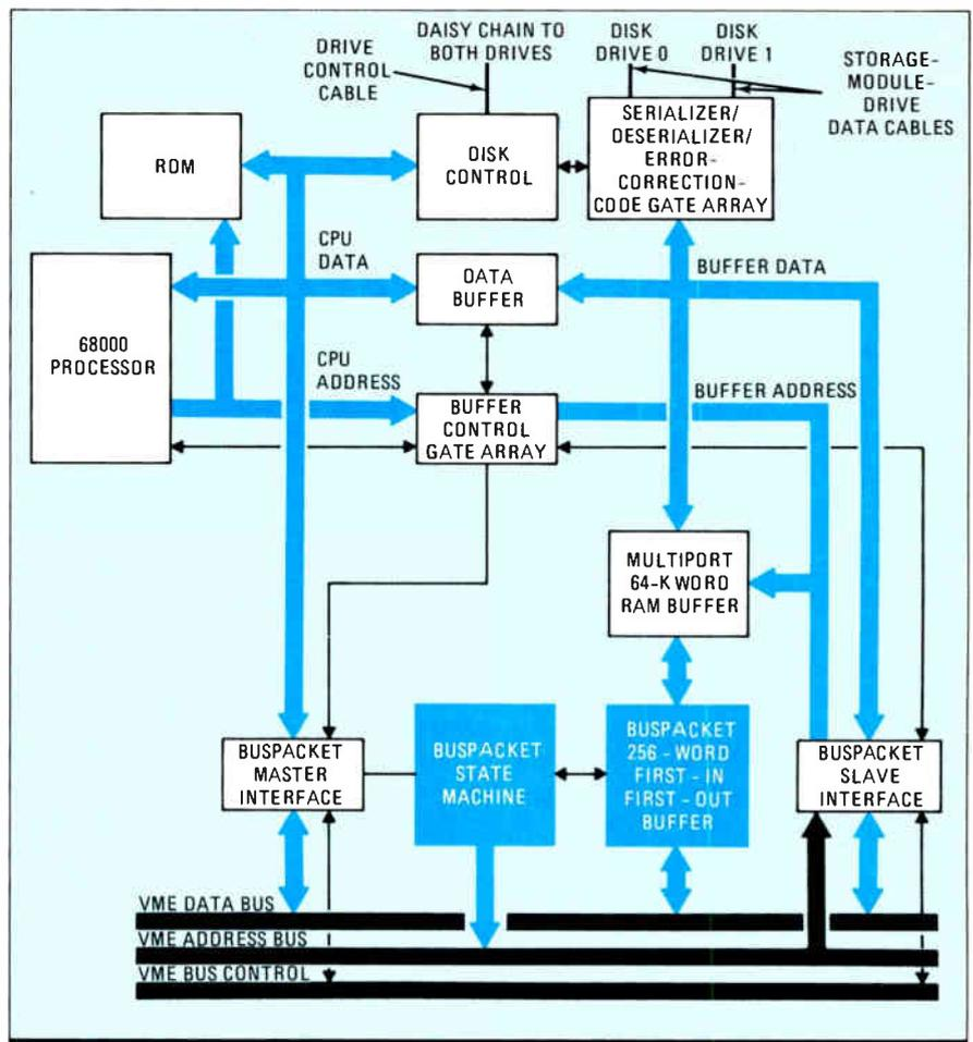
**2. NEW PARTS.** A first-in first-out buffer for assembling packets plus a delay-line state machine dramatically upgrade the performance of this SMD disk controller.
