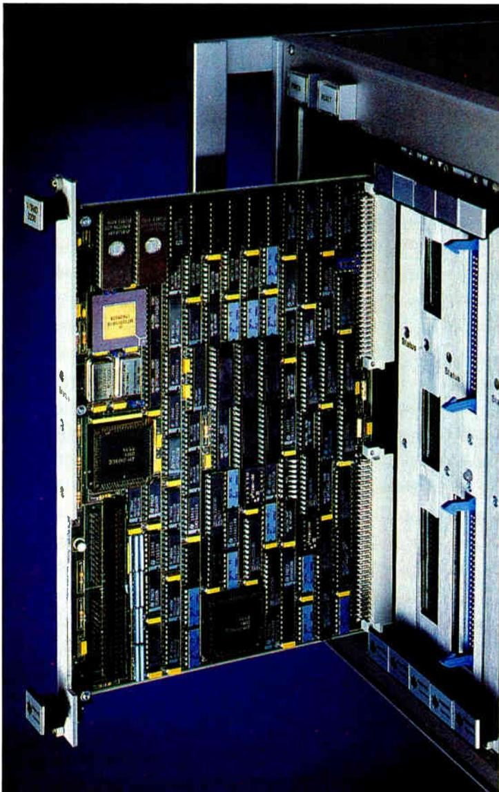
**1. SPEEDY.** Interphase's V/SMD 3200H controller uses the BUSpacket to send data between disk drives and the VMEbus at more than 30 megabytes/s.
