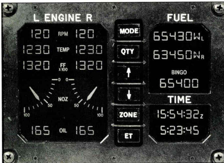
**7. DUAL LCD.** This complex dual LCD for integrated fuel and engine control necessitates use of an SMT driver board and two special elastomeric connectors.
