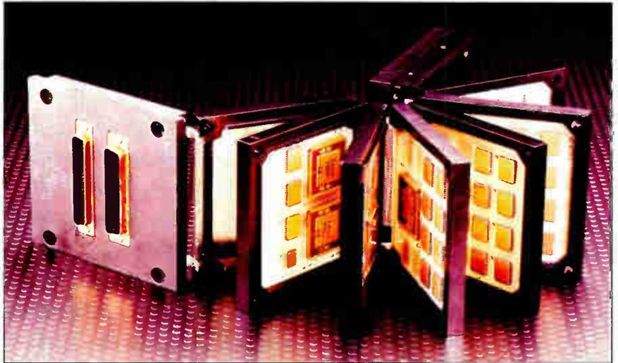
**RAD HARD.** Control Data Corp.'s Spacecraft Control Processor, with its 2- $\mu\text{m}$  CMOS/SOS technology, will be ready two years before machines based on 1.25- $\mu\text{m}$  VHSIC chips.
