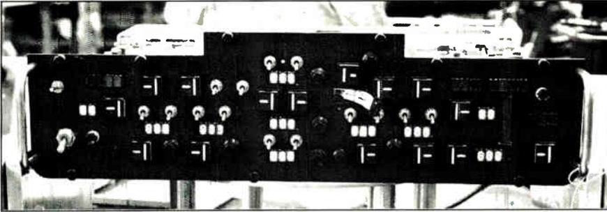
**5. FUEL MANAGEMENT.** Gull Inc.'s Interface Fuel Management Panel for the KC-135 achieves its high packaging density with a combination of rigid, flexible, and rigid-flex boards.
