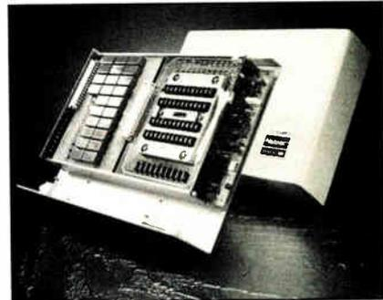
over 100 channels/s. The module features complete on-board signal processing and can measure a variety of inputs with up to 0.03% accuracy without any preconditioning.
