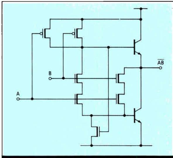
**3. BiMOS CELL.** In a BiMOS internal array, a basic macrocell can be configured either as a two-input CMOS NAND gate or as a one-input bipolar NAND gate.
