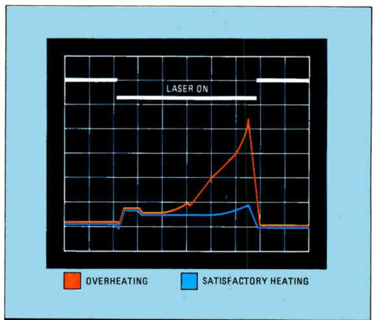
**1. TIME BASED.** The infrared signatures of solder joints with identical laser exposure times show overheating in one. The cause is insufficient solder.
