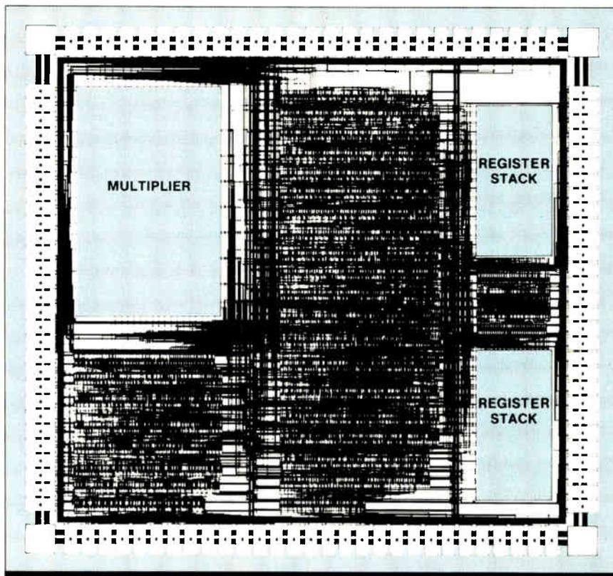
**FAST.** Happi software placed and routed three macro and 1,500 standard cells in 97 min.
