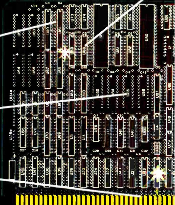
Multiwire Division's electroplated circuit board construction provides surface features for surface-mount components as well as traditional through-hole-mount components. Our experience in new package types encompasses both leaded and leadless devices with pin pitches of 18 mils or more, pin grid arrays and discrete surface-mount components.
