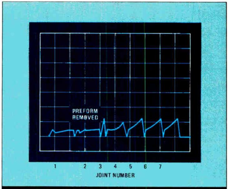
**3. THERMALLY MONITORED.** The monitoring of seven identical joints revealed the probability of excess solder in the first and second joint and the absence of solder in the third.
