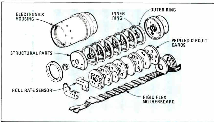
**4. SHOCK MOUNTED.** The Copperhead's guidance package consists of annular pc boards plugged into a rigid-flexible printed-circuit motherboard.
