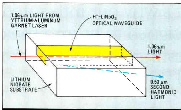
**HALF AS MUCH.** Matsushita has built a second-harmonic generator that halves the wavelength of near-infrared laser light.
