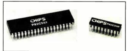
The 82C551 features collision detection. Its built-in jabber function detects transmissions over 65 ms, then ignores that line until the transmission ceases, which helps to isolate faulty nodes from the rest of the network. It has a diagnostic loop-back for fault detection and isolation.
