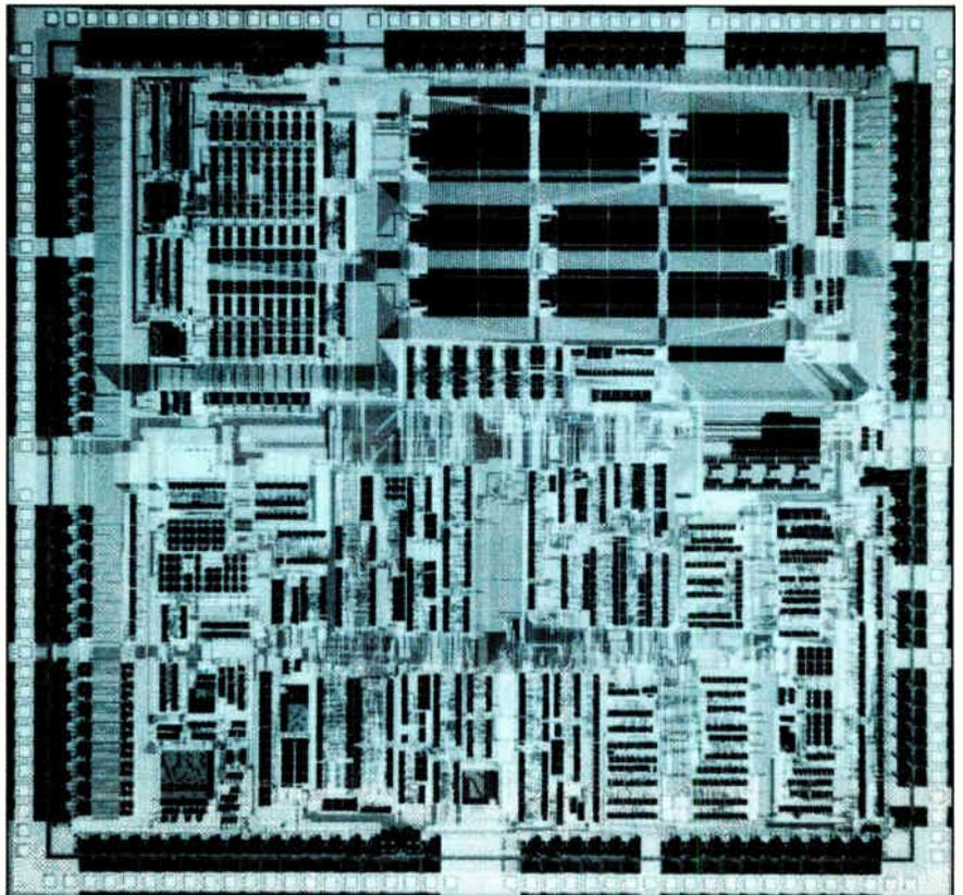
**SPEEDY DELIVERY.** Intel's message passing coprocessor handles all the tasks that are necessary to send message packets at maximum speed among modules on a Multibus II.
