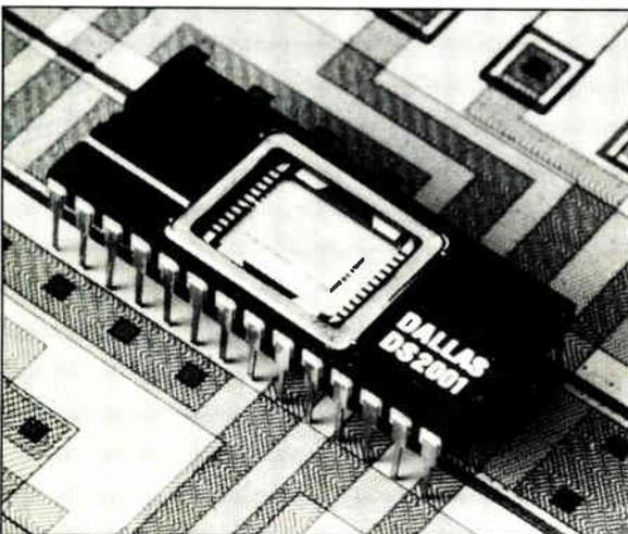
**PARITY BIT.** Dallas Semiconductor's dense FIFO is organized as 2-K by 9 bits for parity checking.
