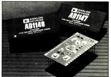
$\mu$ s. Data may be loaded into the AD1147's input latches from 8- and 16-bit buses. The analog output range can be set for either voltage or current.
