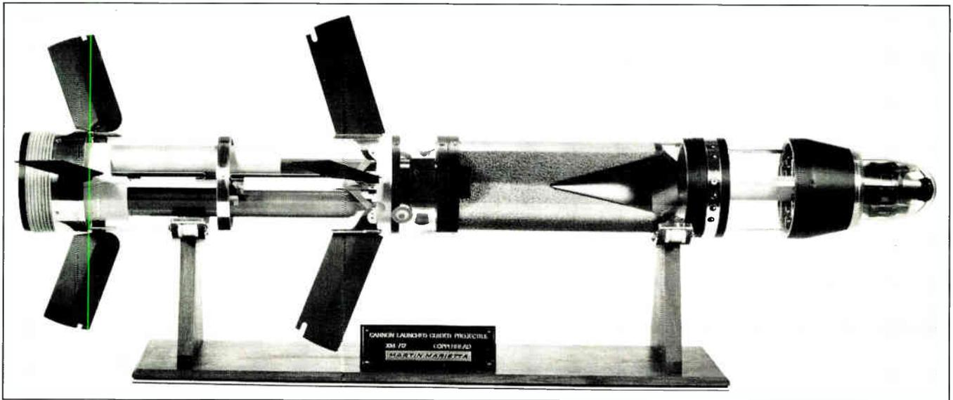
**3. COPPERHEAD.** The cannon-launched Copperhead is designed to endure a 13.5-ms 9,000-g force.
