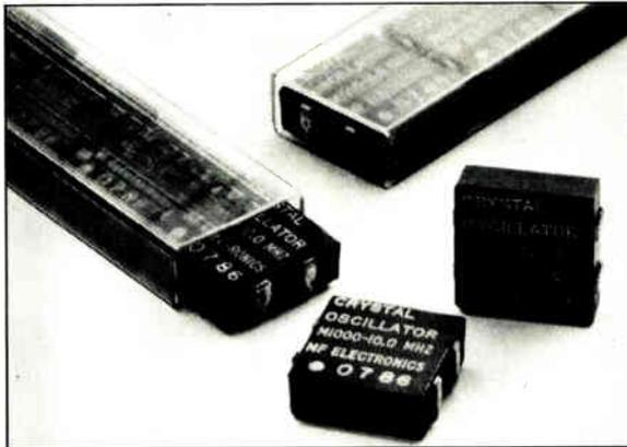
**NO DAMAGE.** MF's crystal oscillator comes in plastic J-leaded packages for safe handling by pick-and-place machines.
