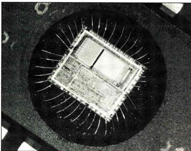
**OPENER.** To expose a chip and one or both ends of the bonded wires (above) to allow fault analysis with a microscope or microprobes, Gfeller's Jetty acid stream system (right) can etch away a plastic package.
