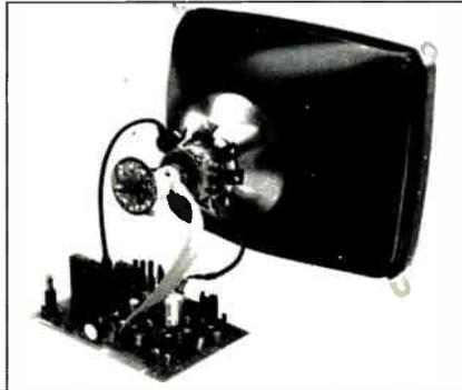
110° CRTs. It accepts either Schottky TTL or emitter-coupled-logic video signal inputs with full gray-scale display and requires a 24-V input. The 300MDX is available now.
