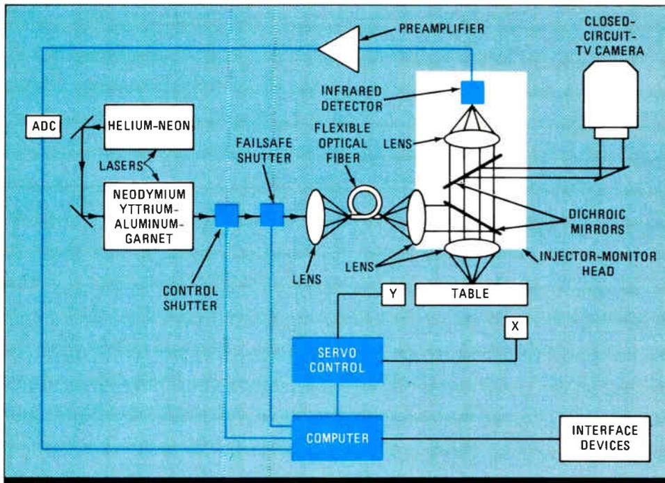
**2. SIGNING OFF.** In Vanzetti's laser soldering system, an IR detector senses the optimal joint temperature to trigger the laser's shutter when the solder becomes liquefied.
