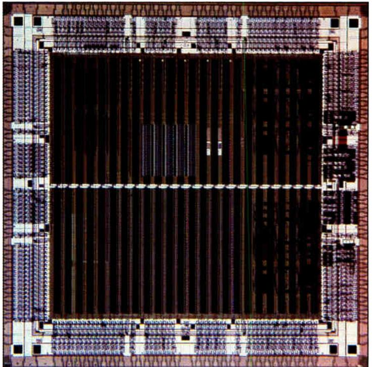
**1. BIPOLAR-CMOS.** Motorola's 2- $\mu\text{m}$  process with n-wells and silicided gates, drains, and sources merges CMOS and bipolar.
