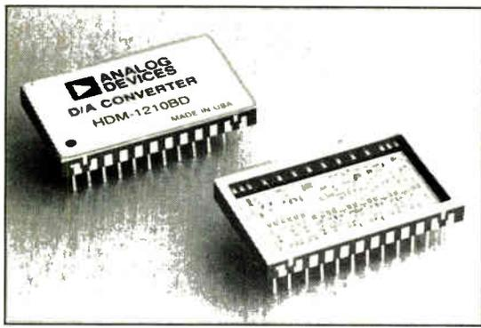
**VOLTAGE TOO.** Analog Devices' 85-ns multiplying DAC has a current output but can be set to put out a voltage.
