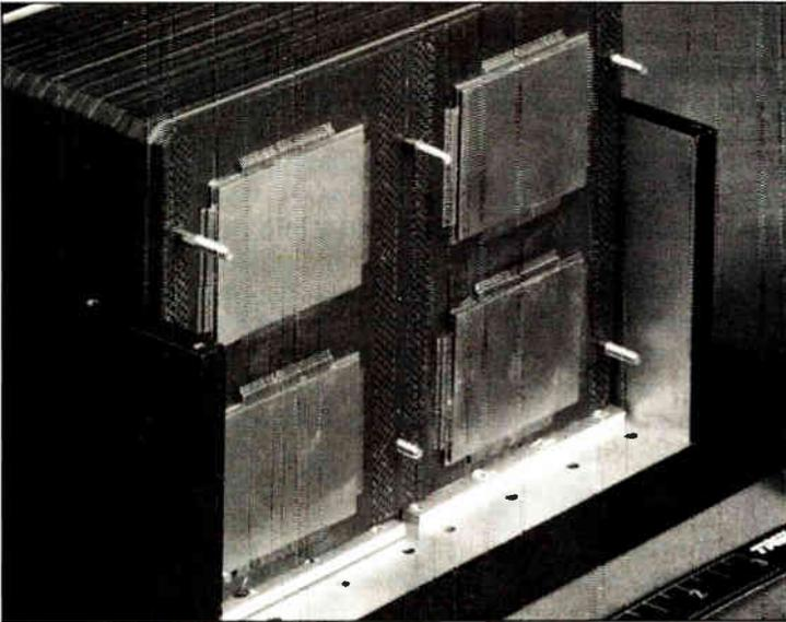
**3. MOCKUP.** The cards in a VHSIC Phase 2 signal processor show the packages used for the superchips under development.
