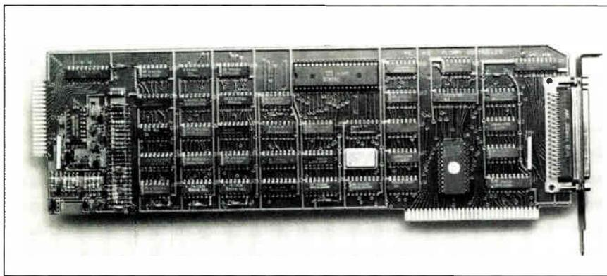
**MIXING.** With Drivemaster, 360-K-byte and 1.2-megabyte drives can be mixed in systems.
