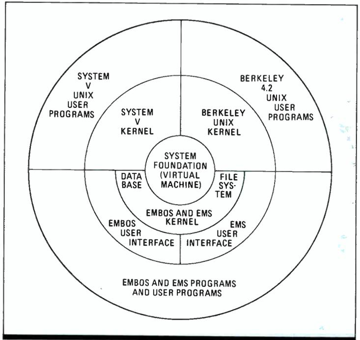
**2. EASY ADDITION.** The compartmentalized structure of the System 6400 lets Elxsi add EMS functions at all levels while leaving existing Embos and Unix functions virtually intact.
