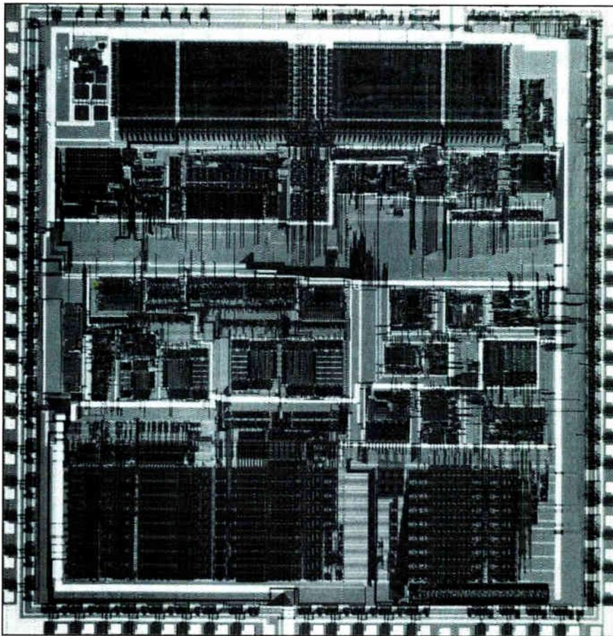
**2. SPEEDUP.** Motorola boosted the speed of its MC68020 to 25 MHz using a 1.5- $\mu$ m HCMOS manufacturing process and a single metal layer with polysilicide.
