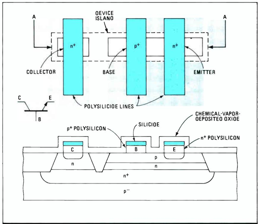
**3. BUFFER.** A chemically deposited oxide covers an Aspect-fabricated npn transistor's polysilicide interconnection material and isolates the emitter, base, and collector from the metal layer that will be formed over the oxide.
