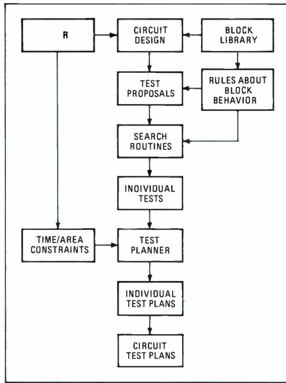
**BRITISH BUNDLE.** From England's GEC Research, Loops suggests circuits to be built in to provide self-test.
