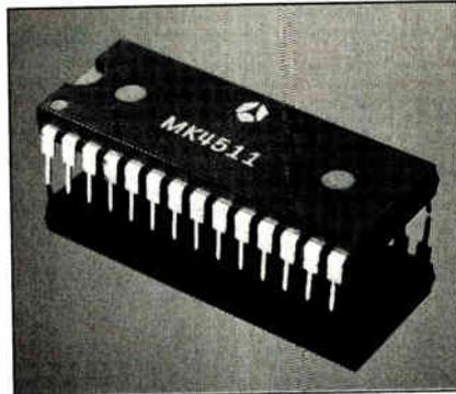
**SMART.** Mostek enters the SRAM market with a chip that has on-board control circuitry.
