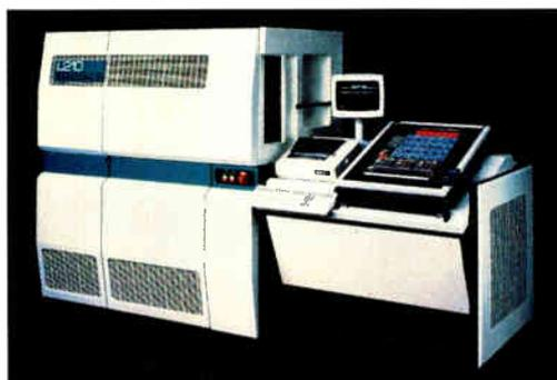
The L210i is Teradyne's first board tester for VLSI in-circuit testing, and in-circuit tester budgets.
