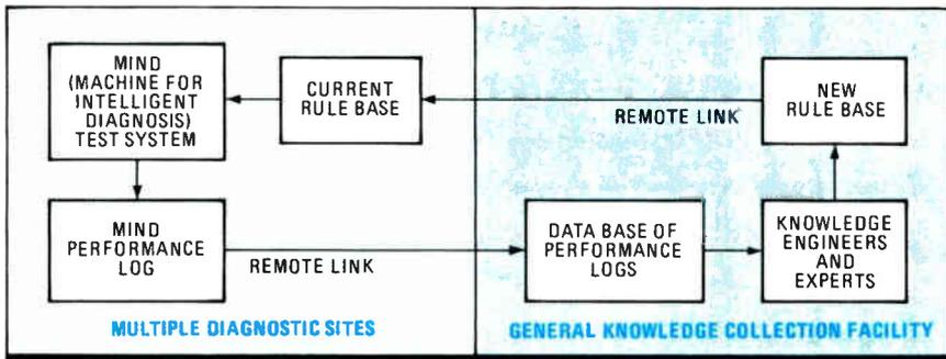
**KNOWLEDGE COLLECTOR.** Teradyne's central facility collects data from all its MIND VLSI test systems in the field. The information then is used to update the field installations.
