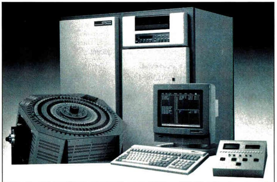
**1. COMPACT TESTER.** Though it includes all the circuitry needed to test 256-pin ASICs, the STS 8256 system is completely contained in two 19-in. racks.
