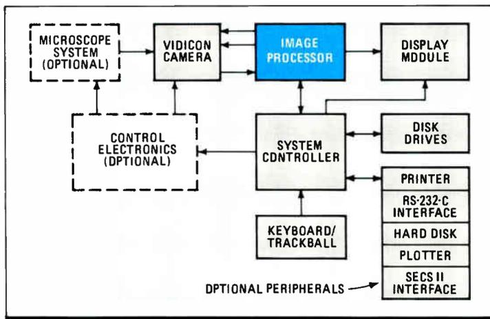
**1. DIGITAL MICROSCOPY.** Digital signal processing and software let an Accuvision system make submicron measurements with an optical microscope.
