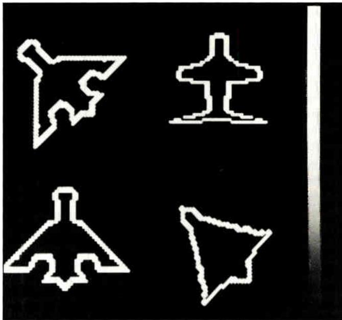
**WHICH PLANE?** Sandia system picks out the two images on the left as matching the target image, despite their rotations; the others are rejected.
