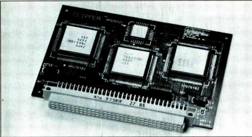
**1. CLIPPER CHIPS.** Fairchild's three-chip Clipper 32-bit microprocessor module is being introduced in a 40-MHz version featuring a top execution speed of 6.5 mips.
