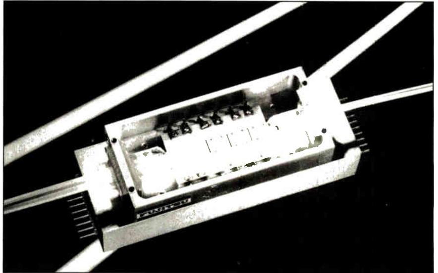
Fujitsu is bringing out a waveguide three-channel optical matrix switch.
