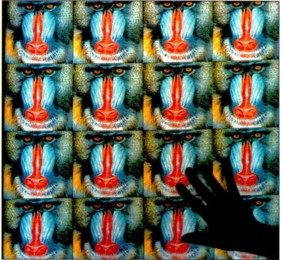
**2. PIXELS GALORE.** It takes lots of pixels (2,048 by 2,048) to produce 16 images at 512-by-512 resolution each. The Metheus Omega 3720 controller does it.
