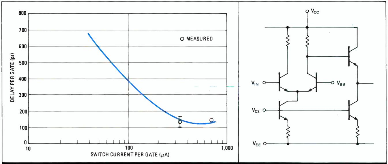
**4. FAST SWITCH.** An Aspect gate (right) will still switch at subnanosecond speeds, even though power varies.
