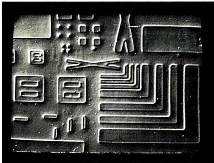
**3. SHEARED EFFECT.** In shearing, two identical images are displaced by several pixels, producing a 3-d-like image.
