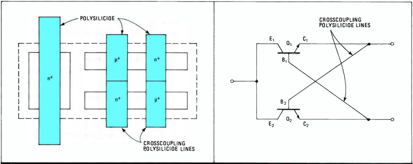
**2. DUAL-PURPOSE.** Fairchild Semiconductor's Aspect process is based on the concept of contactless transistors. The polysilicide lines that interconnect common transistor nodes also serve as part of the transistor's base, collector, and emitter.
