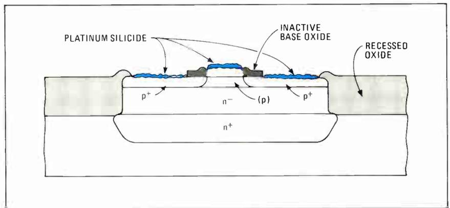
**NOT TO WORRY.** TRW's process for CML-based circuits has an emitter-base structure that is designed to minimize the boron-channeling problems that occur in both bipolar and MOS VLSI.
