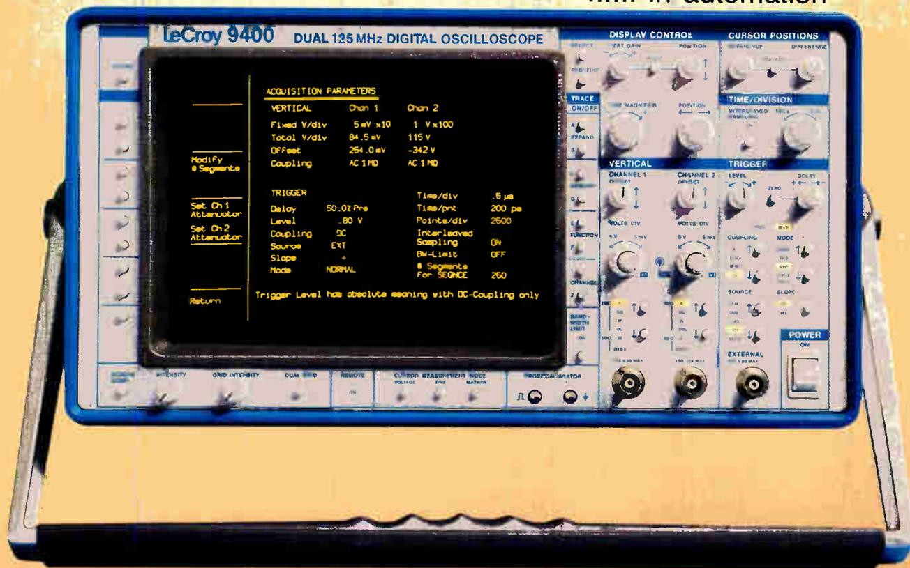
**125 MHz BW; 100 MS/s ADCs; 5 GS/s Interleaved Sampling; 128 k Waveform Memory;  $\pm 1\%$  Accuracy; Summation and Continuous Averaging; Arithmetic Processing; Fully Programmable.**
