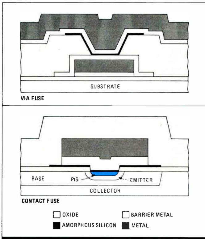
**NO TRENCH.** TI turns to scalable antifuse technology using amorphous silicon for high-density bipolar PROMs without trench isolation.
