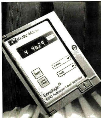
bin. Advanced electronics in each ITU measure this time and analyze all echoes, filter out extraneous noise, and convert the time values to material-level information.
