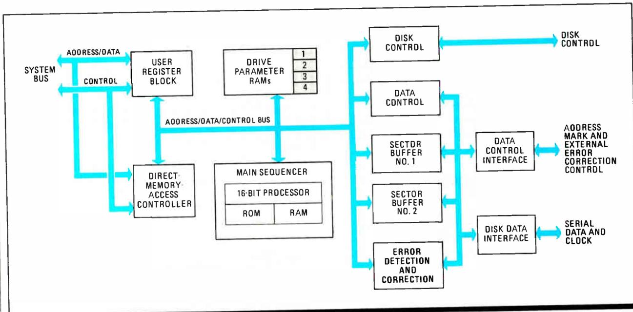
**OUTSIDE HELP.** In addition to its three error-correcting procedures, the Am9850A can go off chip if necessary.
