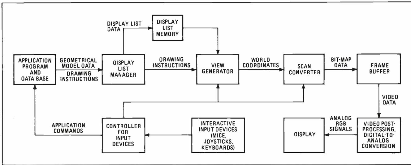
**1. ASSEMBLY LINE.** A typical graphics subsystem has several processing steps, beginning at an application program and ending with the display, that act like an assembly line to produce a picture. The user closes the loop between the display and input devices.
