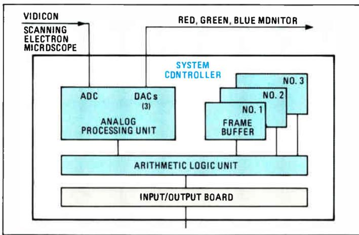
**2. FRAMED.** The digital image processor with a fast analog processing unit and up to three frame buffers digitizes, stores, and averages object images.
