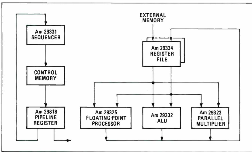
**1. THREE BUSES.** AMD's 32-bit Am29300 family uses external registers and is linked by three 32-bit buses using a flow-through architecture.
