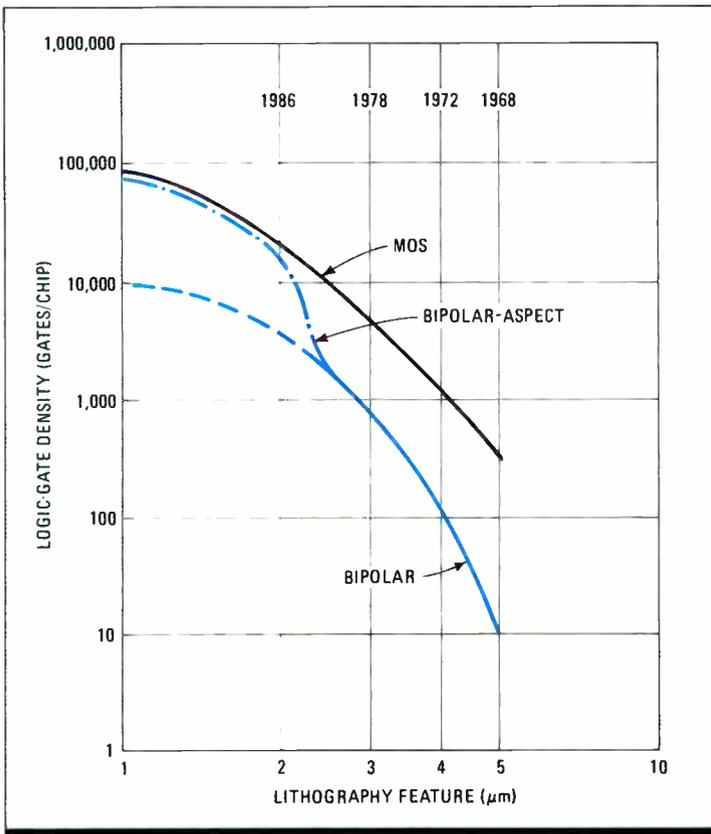
**1. ONE BETTER.** Bipolar ICs fabricated in the Aspect process will match the density of MOS devices and surpass them in speed.
