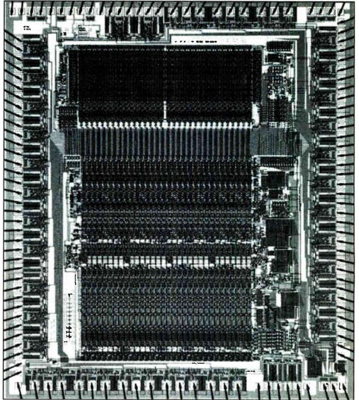
**4. NUMBER CRUNCHER.** Weitek's entry in the 32-bit building-block race is the WTL7137, a 32-bit integer processor with the on-chip functions needed in numeric and controller applications.
