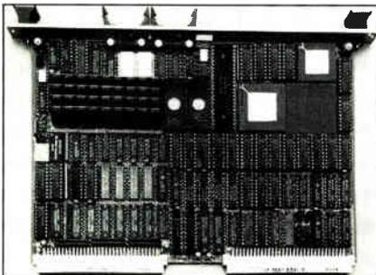
megabytes of dual-access RAM with parity, up to 128-K bytes of EPROM, 128-K bytes of static RAM for user functions, and a single RS-232-C serial port.
