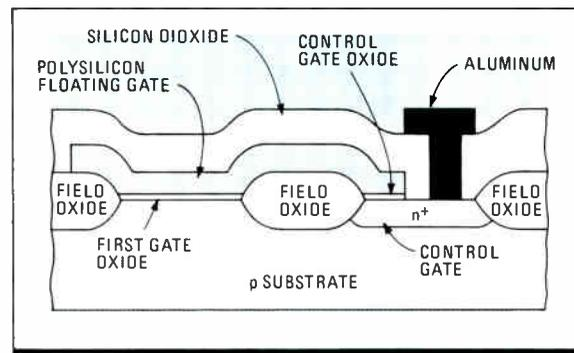
**SINGLE POLY.** Toshiba's EPROM cell laterally isolates the control gate from the cell transistor physically and electrically.
