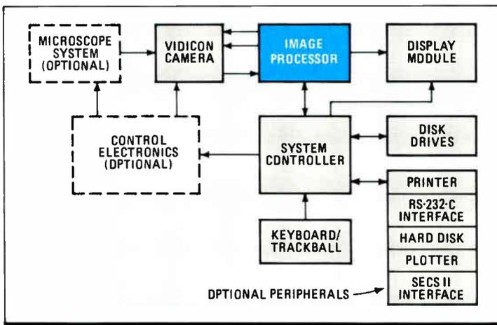
**1. DIGITAL MICROSCOPY.** Digital signal processing and software let an Accuvision system make submicron measurements with an optical microscope.
