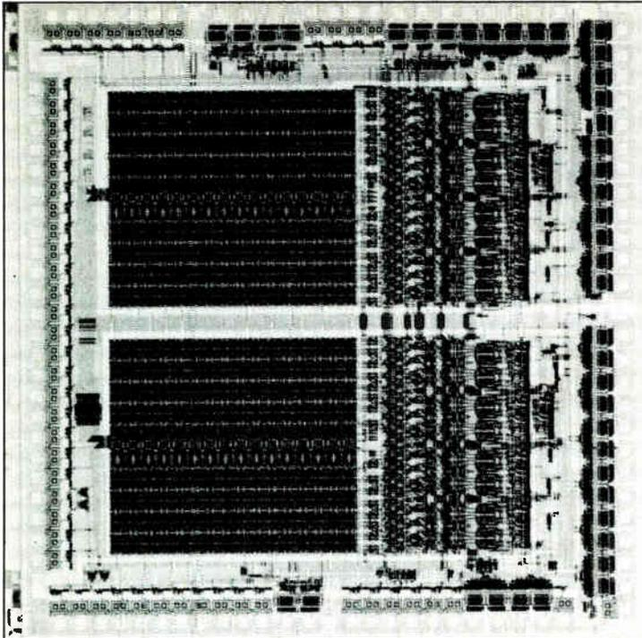
**3. 2901-COMPATIBLE.** WaferScale's WS59032 contains 32 registers, eight 4-bit 2901-type ALUs, and carry-lookahead logic. It is microcode-compatible with the 2900 family.
