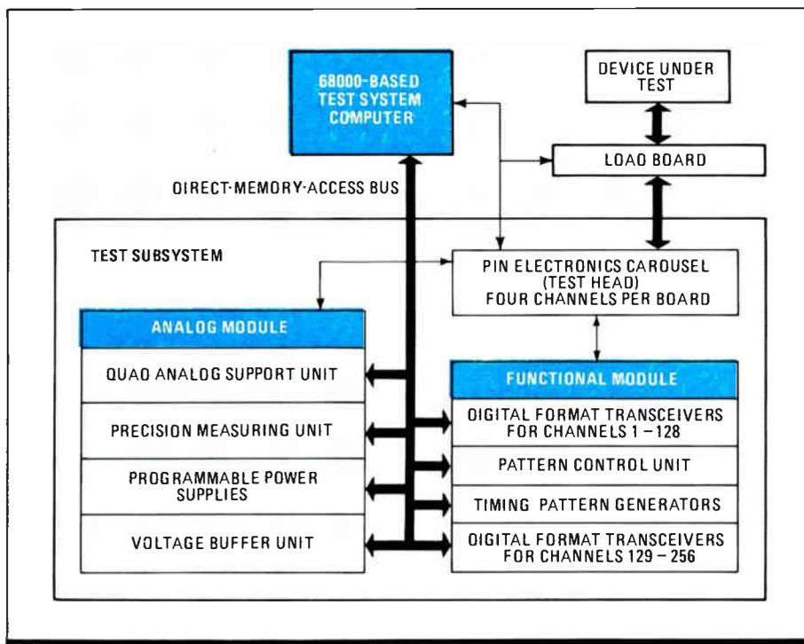
**2. FAST LINKS.** A DMA bus links the system computer to the analog and functional test modules. High-speed cables connect the two modules to the test head.
