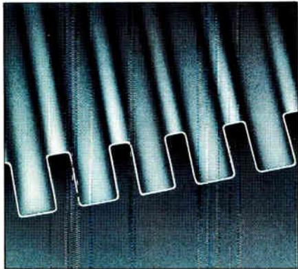
EBR-9 resist profile—0.25 $\mu$ m line and 1.0 $\mu$ m thickness
