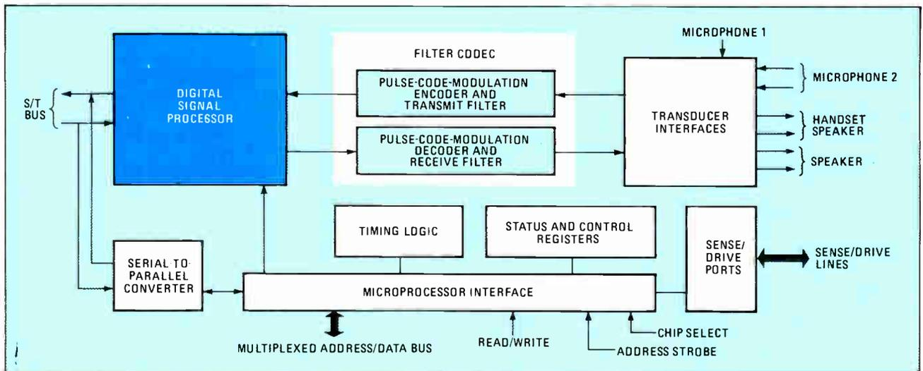
**WORKHORSE.** Mitel's DSP executes three programs, including the DTMF generator that produces audio signals from the telephone's keypad.
