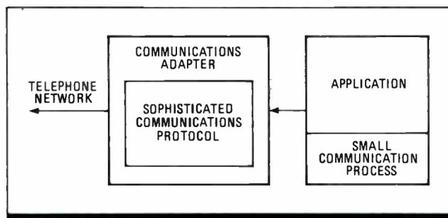
**... AND WITH JUST-PC.** Sophisticated communications functions are provided by the adapter without imposing a large load on the system.
