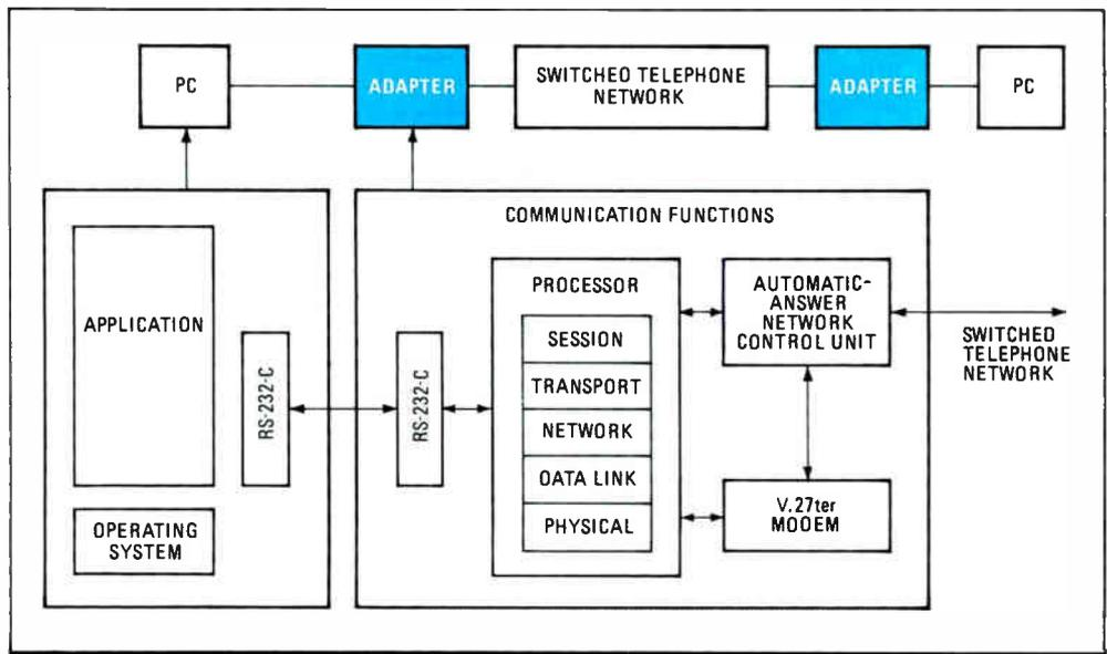
**SIMPLE.** Computer, seeing JUST-PC adapter as a communication function, sends through RS-232-C port.
