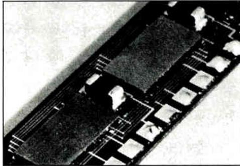
applications requiring three to nine chips. The multichip substrate can be built into another package or used as a subassembly.
