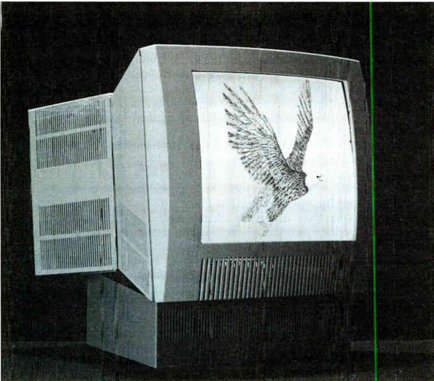
**LOTS OF DOTS.** Megascan Technology's new monochrome display, at 300 dots/in. (4,096 by 3,278 pixels), offers the highest resolution available in a conventional CRT.
