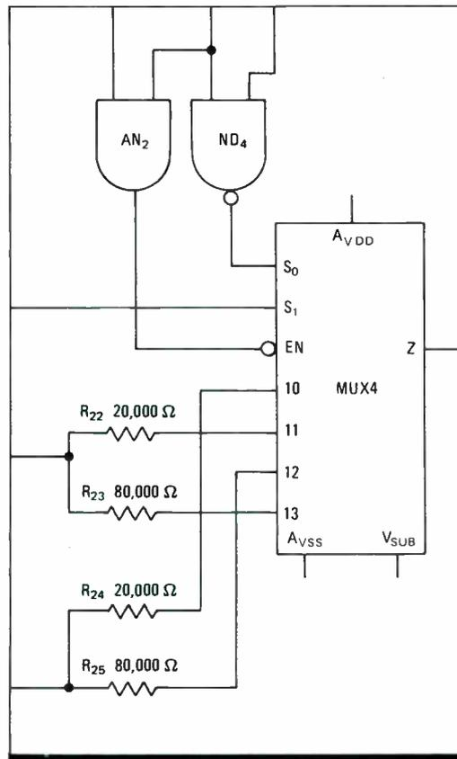
**2. CHECKING BOTH.** An analog multiplexer contains both analog and digital input pins, which the Sierra simulator can easily simulate concurrently.
