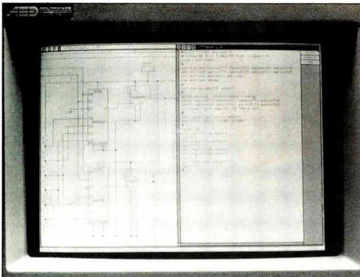
**1. ALL TOGETHER.** Sierra Semiconductor's analog behavioral models simulate both analog and digital functions at the same time.
