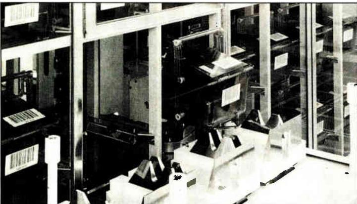
**CLASS 5.** At TI's Class 5 semiconductor processing facility in Dallas, automated guided vehicles reduce human contact with the processed silicon wafers.
