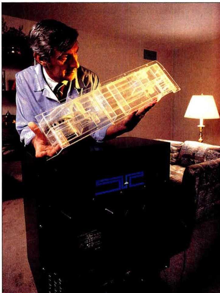
**HIGH FIDELITY.** Audio waveguide technology developed by Amar Bose brings better sound to a Zenith digital TV.
