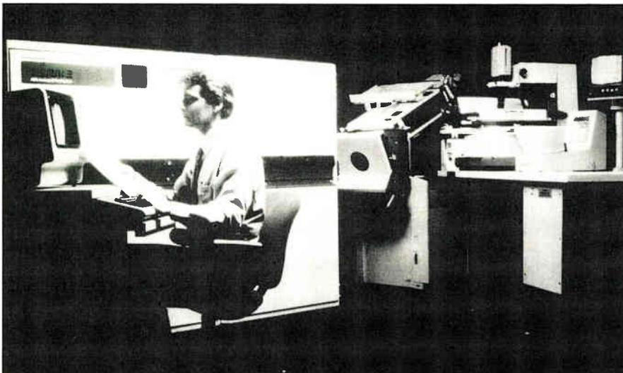
**PRECURSOR.** Architecture of Teradyne's A370 analog VLSI tester anticipates one-pass analog and digital testing of mixed-function chips.
