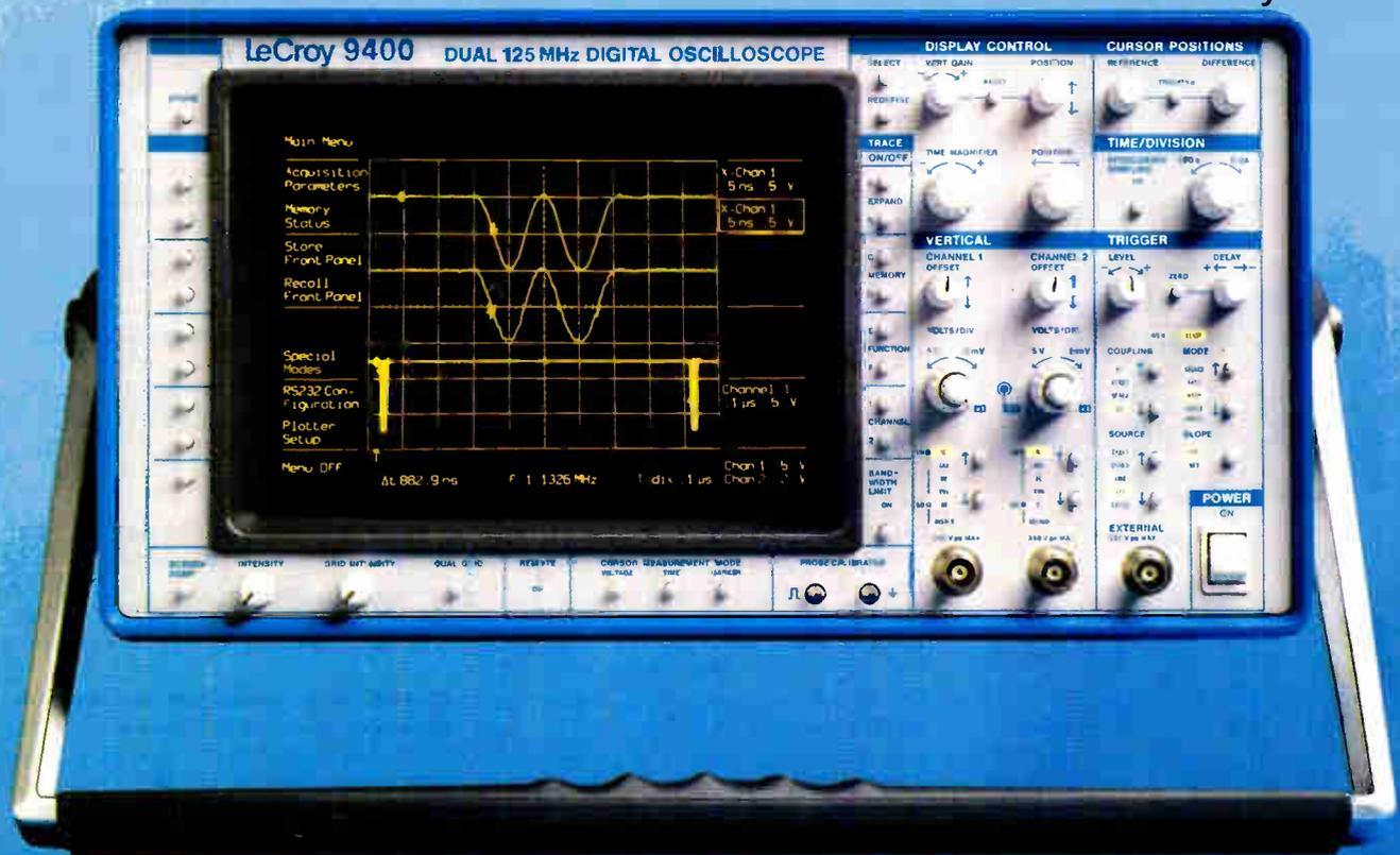
**125 MHz BW; 100 MS/s ADCs; 5 GS/s Interleaved Sampling; 128 k Waveform Memory;  $\pm 1\%$  Accuracy; Summation and Continuous Averaging; Arithmetic Processing; Fully Programmable.**
