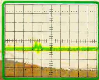
**New KYNAR® Piezo Film is a unique polymer transducer with a dynamic range of  $10^{-3}$  to  $10^6$  psi and a broad-band frequency response from DC to GHz.**
