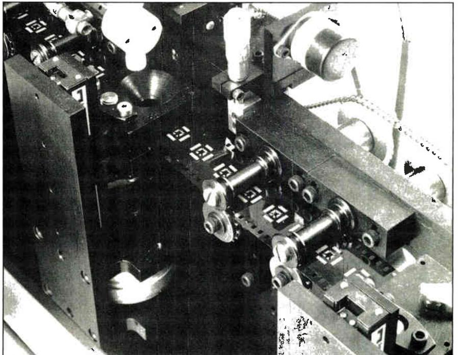
**MESA PAK.** Mesa Technology uses this machine for reel-to-reel encapsulation of TAB-bonded devices. Encapsulation prevents edge shorting and fatigue stress on the bonded device.
