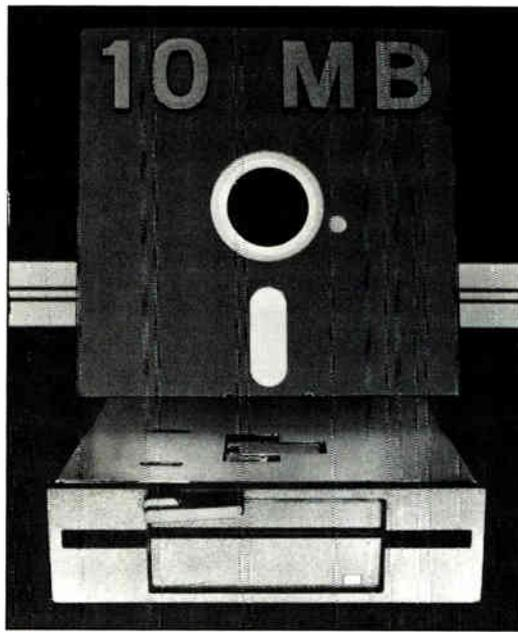
**SPEEDY.** Konica drive spins at 600 rpm—twice the speed of a conventional floppy—and has 5 times the tracks.
