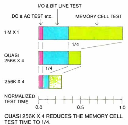
page mode, CAS-before -RAS refresh, and sophisticated test circuitry. NEC have integrated a 4-bit wide test mode that cuts total testing time by up to half. This keeps testing costs down, but maintains a high level of product reliability – essential factors in volume production of large capacity memory chips.
