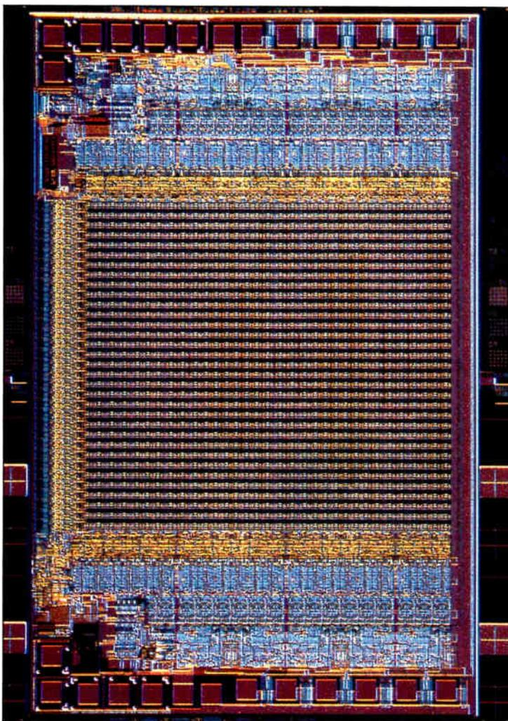
**ERASABLE ASIC.** By eliminating AND/OR gates in its 78C800 IC, Excel in effect creates erasable application-specific ICs—Erasics.
