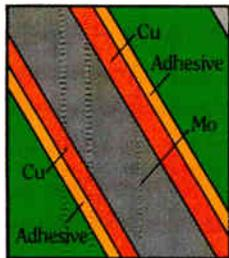
The best way to take the heat off: incorporate a copper-clad molybdenum metal core in the PC board. One, this unique material solves the problem of thermal mismatch with its ultra-low coefficient of expansion. Two, it serves as an integral heat sink. And, three, it significantly increases the rigidity of the board, preventing solder-joint failure due to flexing, warping or twisting.
