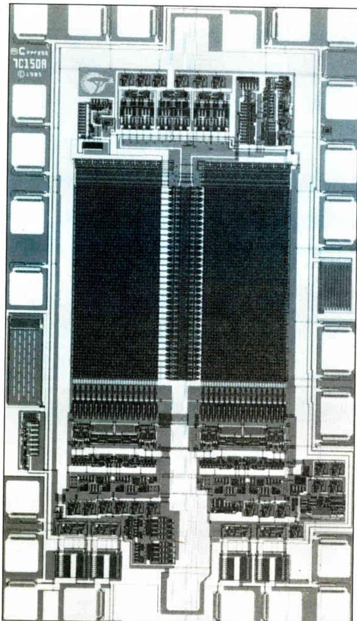
**FAST ACCESS.** The Cypress Semiconductor 1-K and 4-K CMOS SRAMS have access times from 10 to 15 ns.
