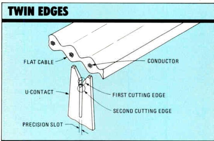
4. The U-shaped contacts on Fujitsu's FCN series of insulation-displacement connectors have two cutting edges for quick and reliable mass termination.
