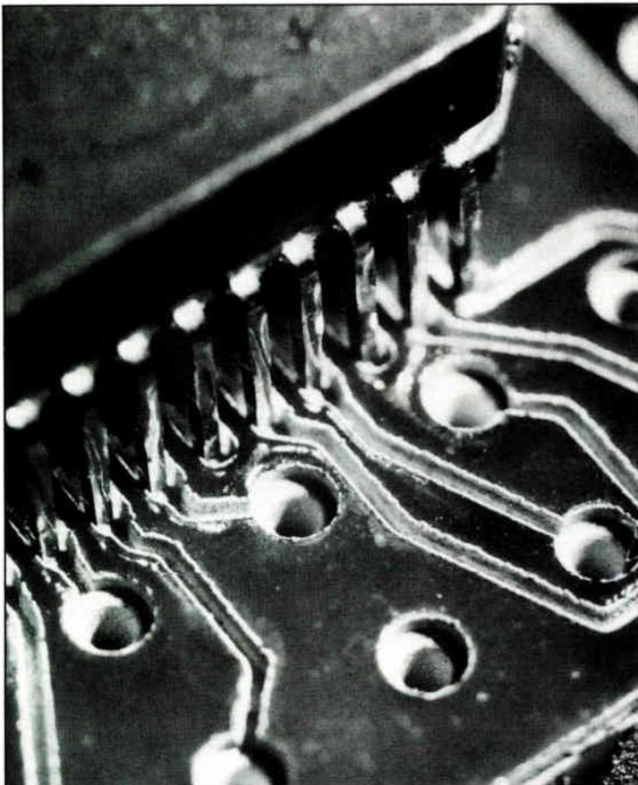
2. Fine pitch leads can be accurately self-aligned in the grooved traces, allowing surface-mounted components to be wave soldered.
