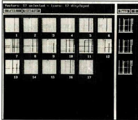
Window with a sequence of 17 images shows logic state of a device corresponding to each test vector.
