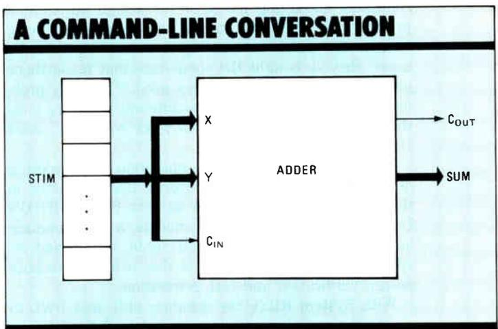
**2. One language serves both design and fault simulation.** Here, a conversation builds a fault file for an adder.
