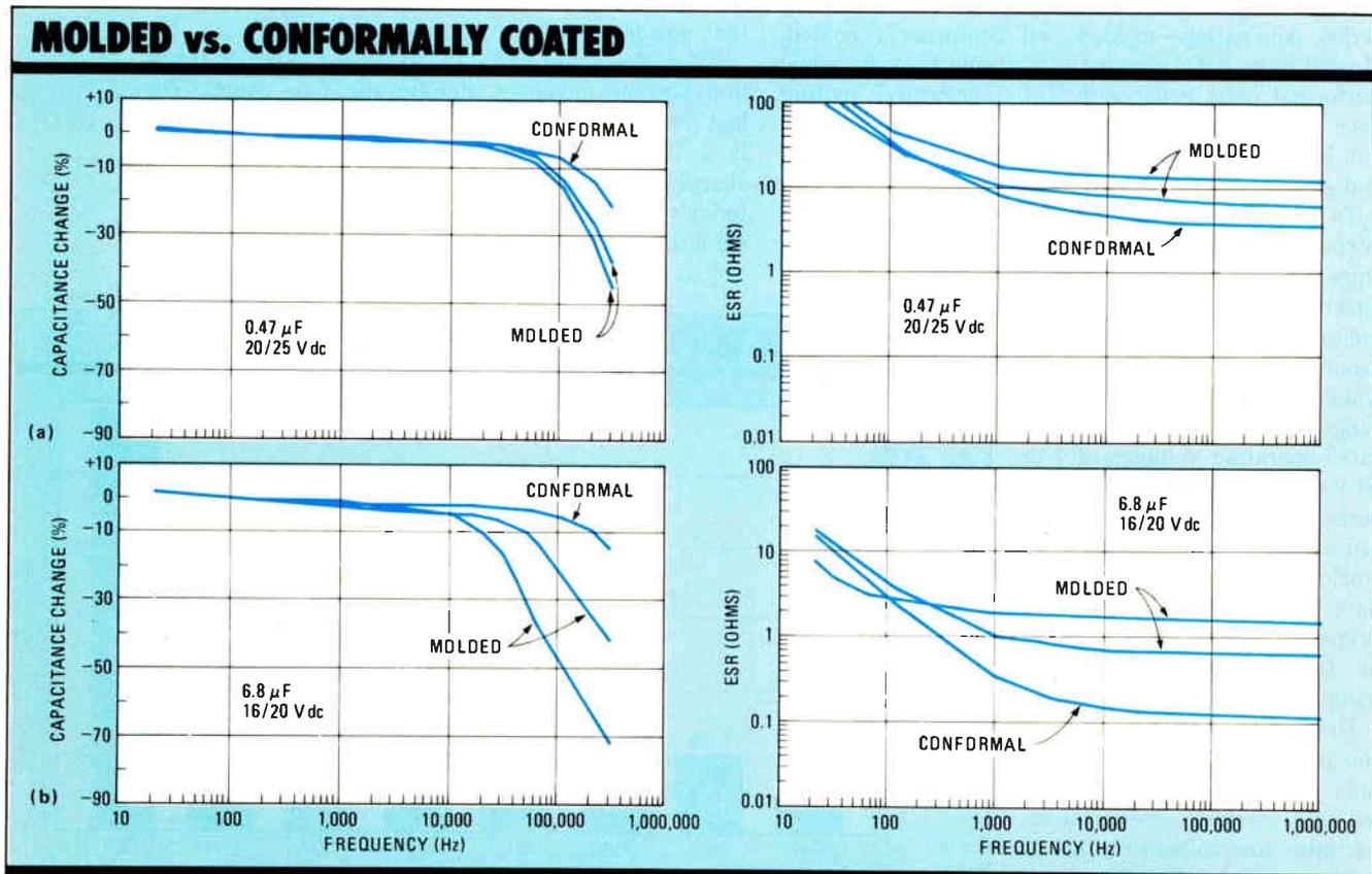
1. Conformally coated chips perform with less capacitance loss and lower ESR beyond 50 kHz for both low values (a) and moderate values (b).
