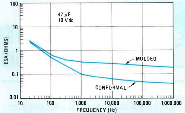
2. Application-specific tantalum chip capacitors can be optimized for a particular task, like switching power supplies.
