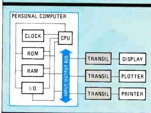
In a typical application, SGS-Thomson's Transil arrays protect the peripheral devices of a personal computer.
