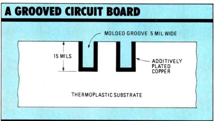
1. Dimensional Circuits' circuit-board technology is based on grooved traces molded into a thermoplastic substrate and then metalplated.
