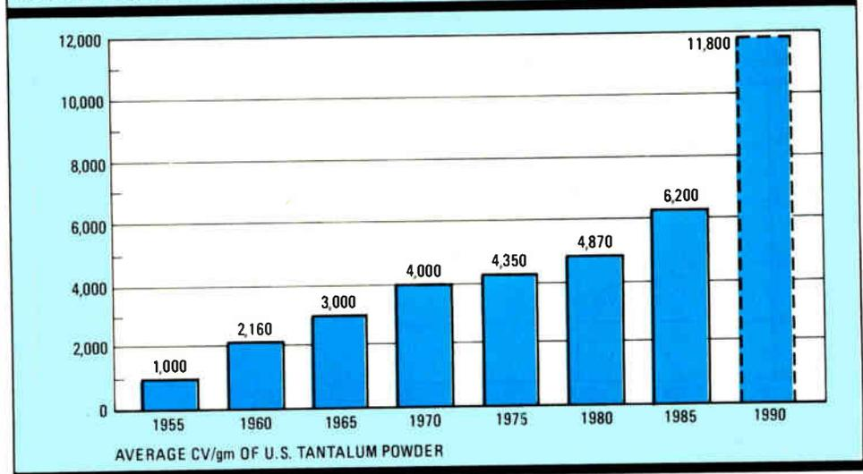
15,000 CV/gm. Current workhorse powders are typically in the range of 6,000 to 12,000 CV/gm and have average particle sizes of 4 to 5  $\mu\text{m}$ . Even now, some powders offer as much as 18,000 to 23,000 CV/gm. However, there is usually a substantial time lag from the point when a new high-CV/gm powder becomes available in volume until capacitor manufacturers are able to adapt their processes to make satisfactory capacitors with it.
