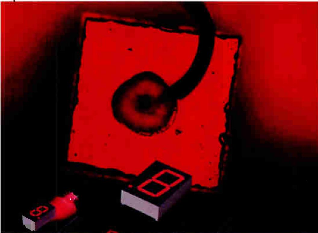
Increase the brightness of the LED's you design into your equipment by as much as 300% with HP's new red AlGaAs products. The price? Only 25% more than our standard high-efficiency red devices.
