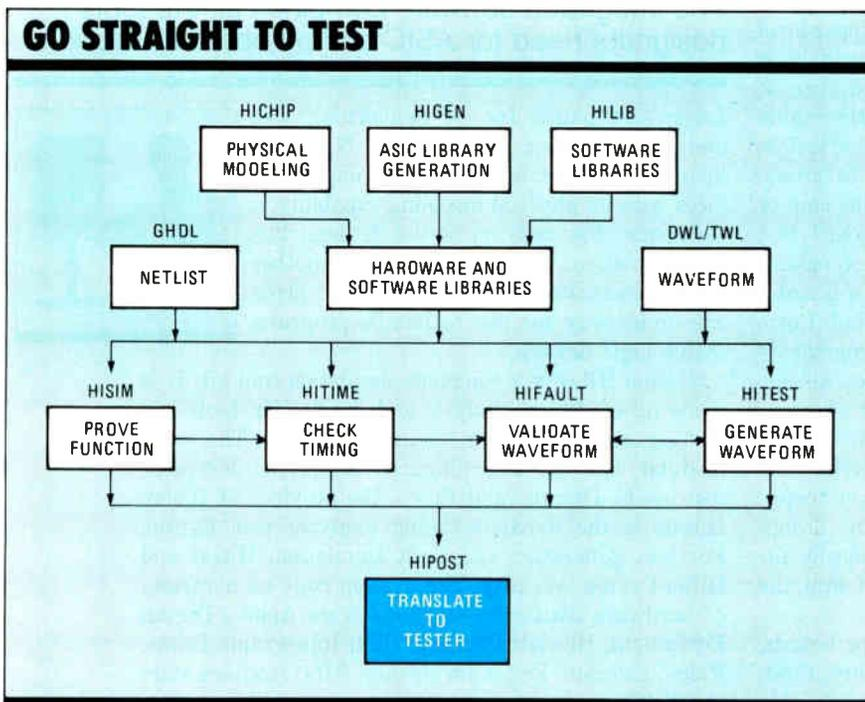
**System HILO** saves time because design vectors no longer need translation before entering the test environment, and because engineers do not have to write more test vectors.
