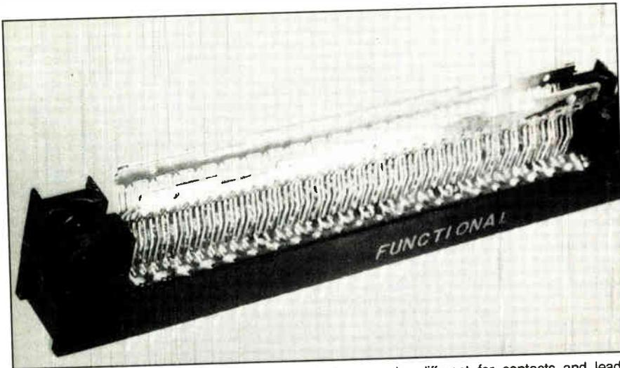
**2. Material finishes** and form factors can be different for contacts and lead-termination combs because they are manufactured separately, then welded together.
