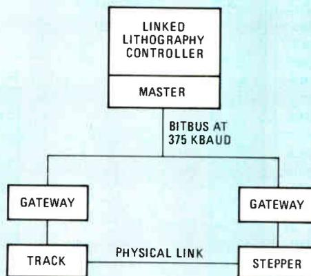
The linked-lithography controller is based on an IBM PC linked to equipment via a communications network.
