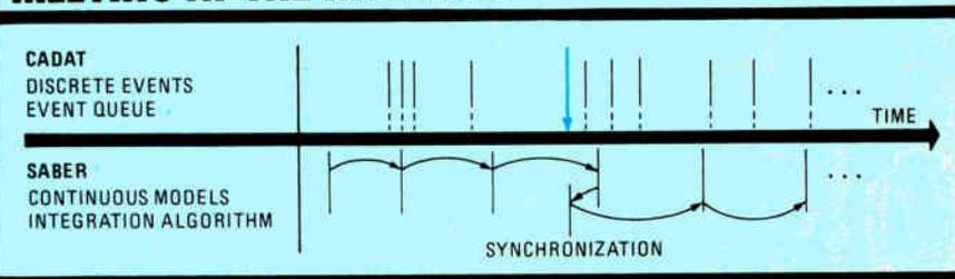
1. The Calaveras algorithm synchronizes Cadat's event-driven simulation (above the line of the interface) with Saber's matrix solution (below the line).
