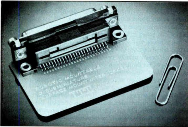
3. The subminiature-D connector now comes in surface-mount styles like this ITT Cannon unit, with up to 25 contacts.
