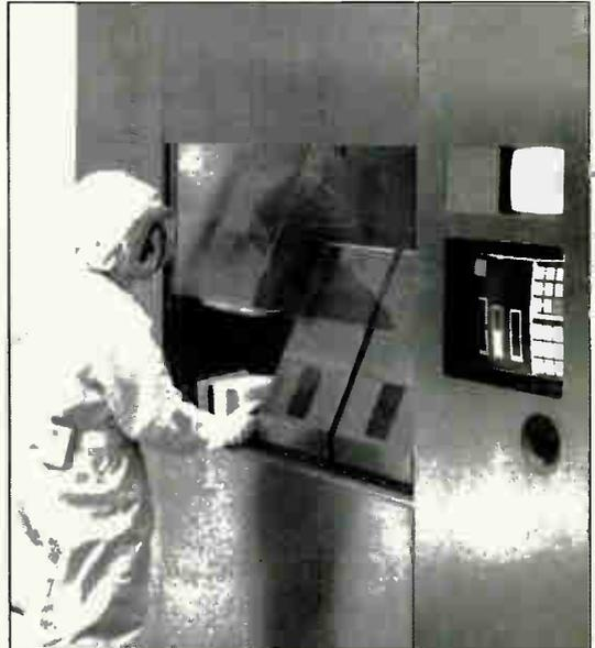
Extrion 1000 holds 13 200-mm wafers, 18 150-mm wafers, 22 125-mm wafers, or 27 100-mm wafers.
