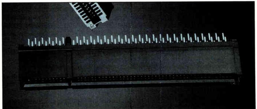
1. These card-edge 50-mil connectors from AMP offer up to 91 dual contacts, which top off a plating of nickel and palladium with a flashing of gold.
