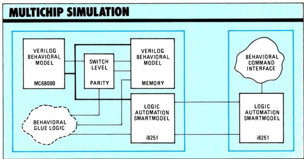
1. Simulation of multichip models containing various logic circuits and memories, as well as processors like the Motorola 68000, is crucial for today's more complex designs.
