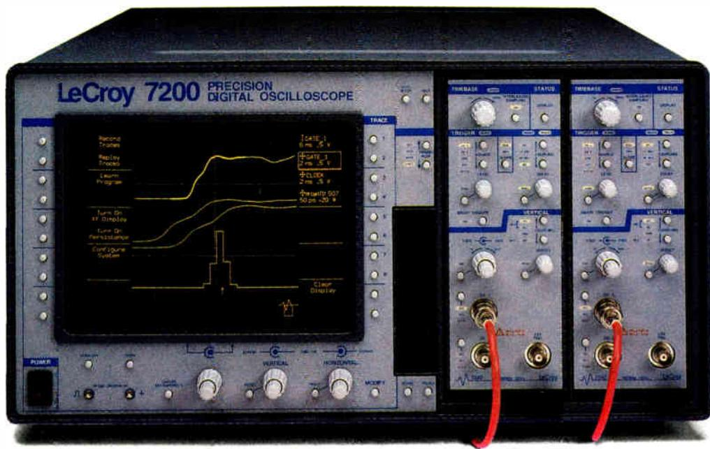
Now get real-time sampling at up to 2 gigasamples/second using 8-bit ADCs on each channel. The 7200 is the digital oscilloscope with an analog personality – simply easy to use. Display your data in seconds instead of hours via instant auto-setups and built-in help.
