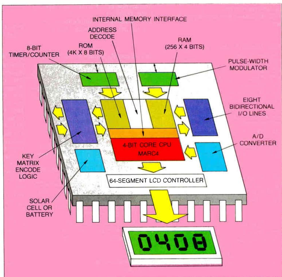
**MARC4 holds a CPU, program and data memory, I/O ports, and such peripherals as LCD drivers; a system can be configured on a single chip.**
