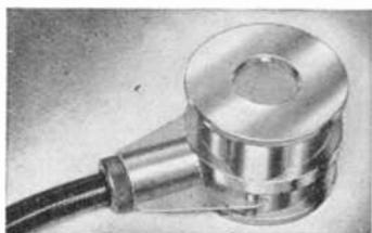
*Transducer Head. The generating crystal is air-backed to give maximum ultrasonic output. Special rear connections to crystal eliminate corona discharge at high R.F. potentials. Siastic rubber sealing rings can be supplied, enabling the transducer to be immersed in liquids up to 150°C. temperature.*
