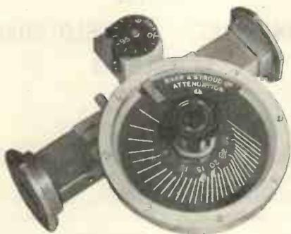
incorporates a unique means of compensation of the scale reading to correct the variation with frequency in attenuation characteristic of the metallised vane within the guide. There is no need to refer to calibration data and errors due to incorrect setting up are virtually impossible.
