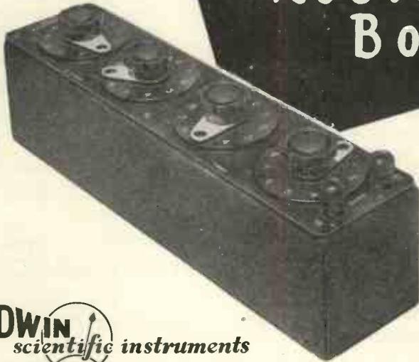
4, 5 and 6-dial. Ranges 0.1 ohm to 111,111 ohms. Accuracy  $\pm 0.1\%$ . Maximum loading 10 watts per dial. Non-inductive for mains and audio frequencies: metal cased. Write for Leaflet No. E.113.
