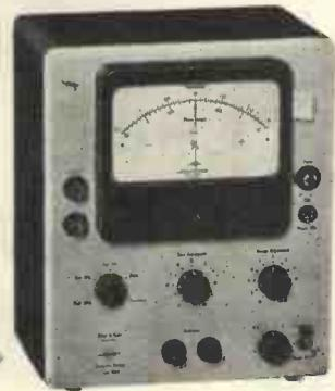
The accuracy is better than 0.03% for indication round the zero point and better than 3% for full scale indication of impedance or phase angle deviations.
