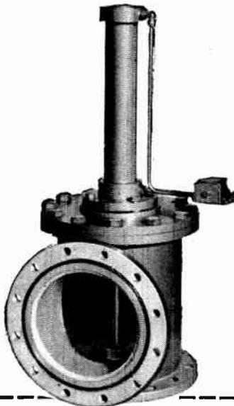
The Stokes Model 217 High Vacuum Poppel Valve features a quick-acting positive air cylinder and is absolutely leak-free. Fully opening valve design provides maximum conductance. Disc and body are corrosion-resistant plated... actuating stem is chrome plated... flanges are standard. 4-, 6-, 10-, 16-, 24-, 30-, and 36-inch sizes.
