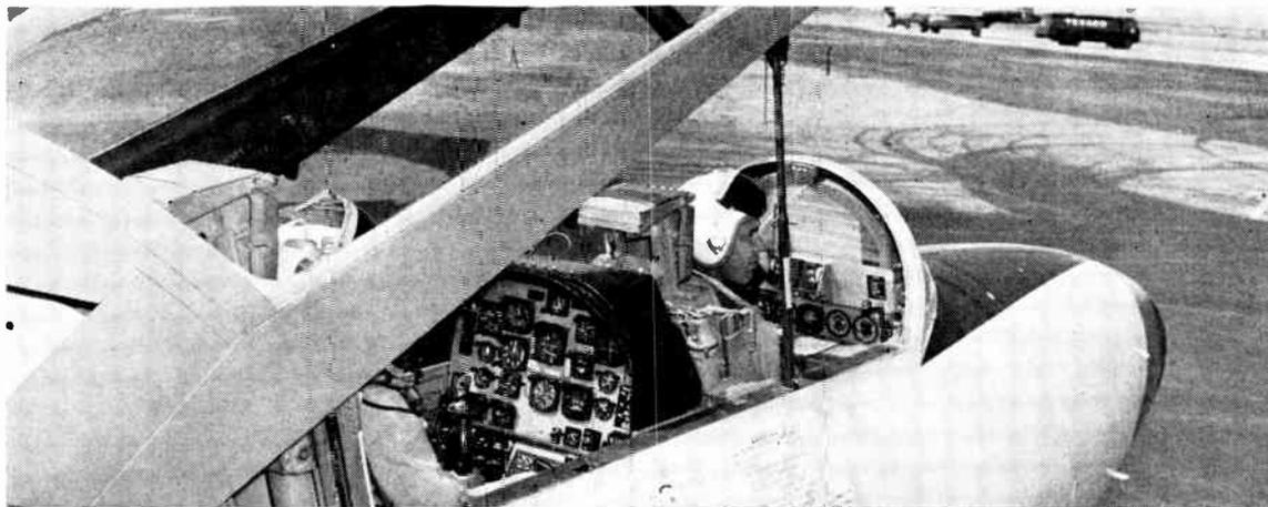
Pilots of the future will not need to read maze of flight instruments, shown in rear cockpit, because of new flight data presentation display shown in front cockpit
