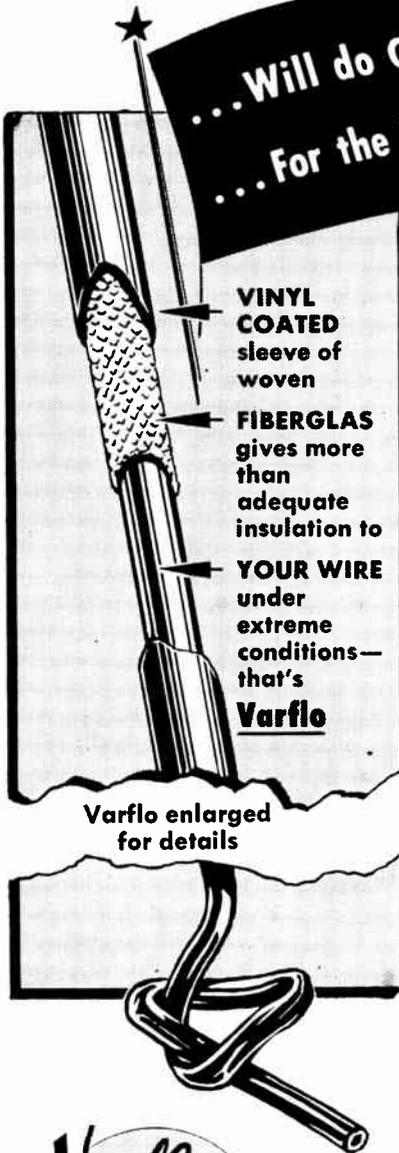
**VINYL COATED sleeve of woven FIBERGLAS gives more than adequate insulation to YOUR WIRE under extreme conditions—that's Varflo**
