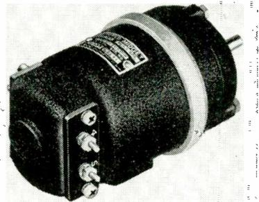
"FB" FRAME, 2-1/4" x 4". DC—as wound field and permanent-magnet field motors and generators, and servo motors. AC—as universal motors, and permanent-magnet generators, one, two, or three phase. Also in shorter length; as capacitor start and run, two and four pole AC motors. As induction type to 1/200 HP at 3400 RPM; as synchronous type to 1/500 HP at 3600 RPM.
