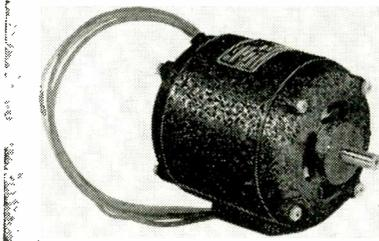
ALP FRAME, 3-3/8" x 4-5/16", capacitor start and run, two and four pole AC motors, internal fan cooled. As induction type to 1/20 HP at 3400 RPM; as synchronous type to 1/40 HP at 3600 RPM.
