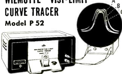
For rapid alignment of I.F. coils of frequencies from 85 kc to 11 mc. Operator adjusts test trace (B) to fall between traces of limit coils (A and C), set up to production specifications. Defective coils immediately detected. All error is eliminated as circuit changes or line voltage variations affect all three traces equally.
