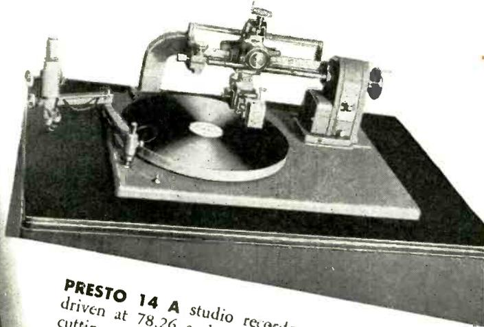
**PRESTO 14 A** studio recorder, directly gear driven at 78.26 and 33.3 r.p.m., selection 10 cutting pitches 88-136 lines per inch, designed to cut vertical or lateral masters or instantaneous recordings.
