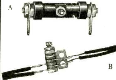
"Coprox" rectifiers by Bradley feature gold-coated positive contact pellets to combat aging. Specially designed terminals and pre-soldering of lead wires prevent overheating during assembly.
