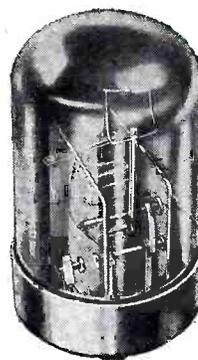
The accelerometer is a newly developed electronic tube useful in measuring linear acceleration. Operating range — 1 to 100 g's.
