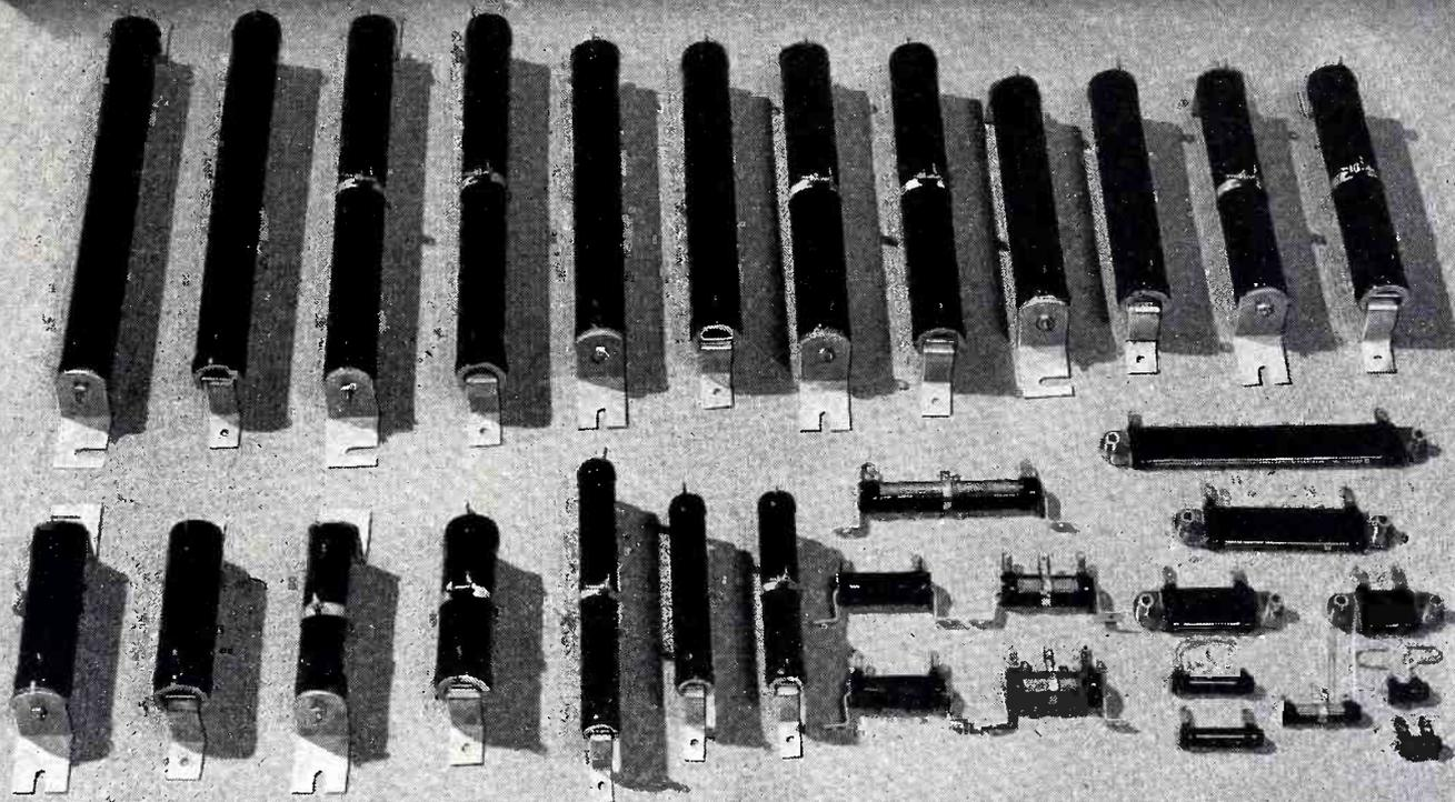
I-T-E POWER WIRE WOUND RESISTORS are made in a wide variety of types, sizes and ratings with mountings and terminals as specified. They have silver soldered connections, are locked and insulated with blue-black Vitreous enamel for fast heat-dissipation, and are held to close tolerances to meet critical conditions of atmosphere and usage. Ratings range from 5 to 215 watts in fixed and adjustable types and from 30 to 75 watts in oval types.
