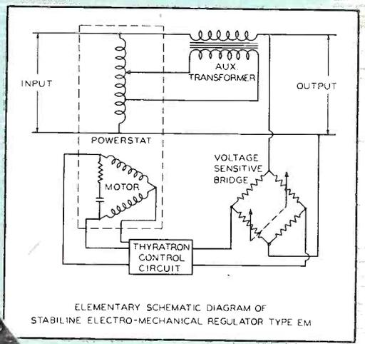
ELEMENTARY SCHEMATIC DIAGRAM OF STABILINE ELECTRO-MECHANICAL REGULATOR TYPE EM
