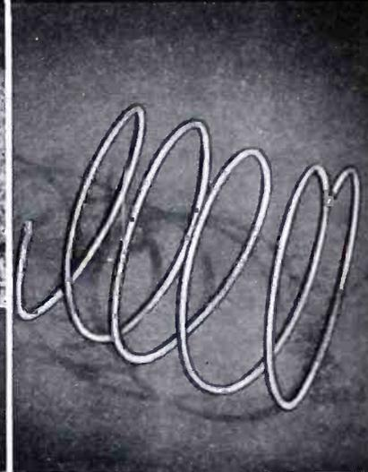
A solid or stranded conductor over which has been extruded a homogeneous vinylite plastic sheathing.
