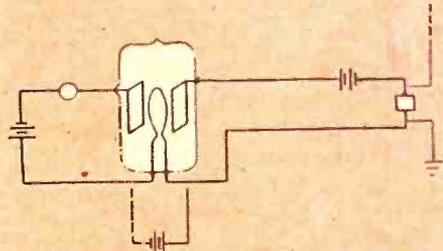
An illustration from deForest U. S. patent No. 841,387 showing a control element adjacent to the cathode but on the opposite side from the anode
