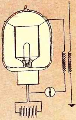
Fleming patented the use of Edison's tube as a detector for wireless signals. Drawing taken from his U. S. patent No. 803,684
