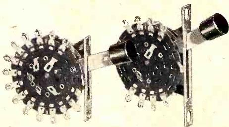
**LEVER ACTION SWITCHES** are particularly designed for intercommunication, centralized radio, sound distribution, public address and test equipment. Positive indexing available in two, three and four positions. Return spring action available in two and three positions. Both types have appropriate circuit combinations. Refer Notes A and B.
