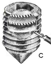
(C) Knurling of this "Unbrako" Socket Set Screw swages the threads and makes it a most excellent Self-Locker—for use where the points such as: flat, dog, cone and oval do not lend themselves to knurling. Sizes from #4 to 1-1/2" in diam-
