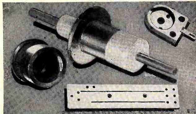
**INSERTS**—May be made of any common metal that can withstand temperatures of about 1200° F and that has a coefficient of thermal expansion of the order of 100 to 175 x 10<sup>-7</sup> per degree C. Included are cold rolled steel, copper, nickel, aluminum, Monel, Inconel, etc.
