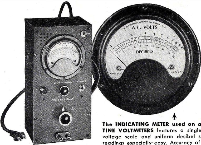
The **INDICATING METER** used on all **BALLANTINE VOLTMETERS** features a single logarithmic voltage scale and uniform decibel scale. Makes readings especially easy. Accuracy of indication is 2% at any point on the scale.
