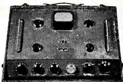
**The 90-A Portable Recording Amplifier** unit incorporates the following: three channel mixing preamp. and line input—response: NAB, 78 rpm, and flat (30-15,000 cps)—high and low frequency equalizers—outputs for one or two turntables or a line.
