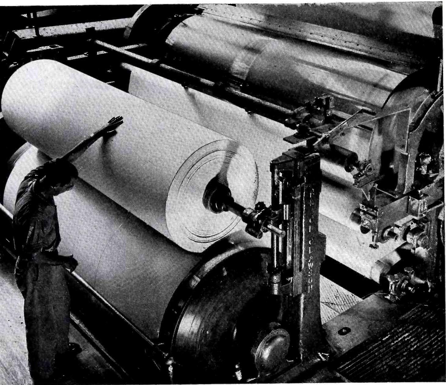
Our specialty is the manufacture of insulating papers for condensers, coils, transformers, or other insulating purposes...in thicknesses ranging from .0002" to .004".
