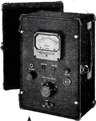
**MODEL 302 ELECTRONIC VOLTMETER.** This Sensitive Electronic Voltmeter is portable and operates from light-weight batteries contained within carrying case. Reads AC voltages from 1 millivolt to 100 volts over frequency range of 5 cycles to 150,000 cycles. Accuracy 2% at any point on scale. Can be used as highly stable amplifier. Input impedance  $\frac{1}{2}$  megohm. Uses standard Eveready or Burgess batteries. Battery life over 150 hours.
