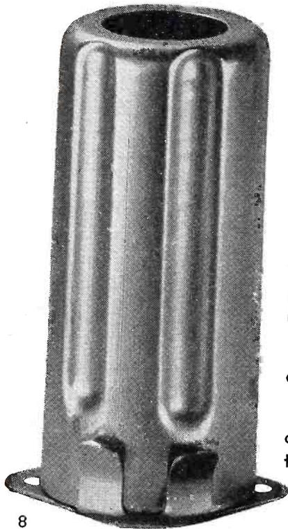
The shield is sized so that three of the flutes make a slide fit with the tube, supporting it throughout its length. A hardened and tempered spring steel clip locates the shield and holds the tube firmly in place.
