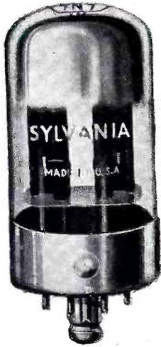
In Sylvania Lock-In receiving tubes, the contact pins are sealed into the glass bottom, thus eliminating the need for soldered connections. No top cap connections are used — a feature which contributes to compactness. Many Lock-In types are especially suitable for UHF applications, because of their low lead inductances, low interelectrode capacitances and low dielectric losses.
