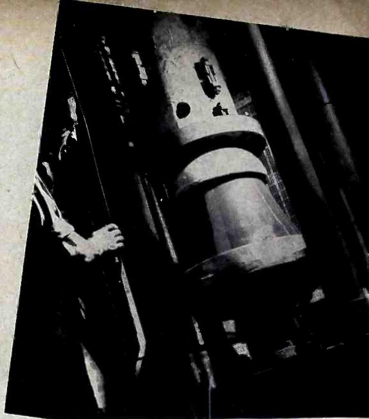
*"A million pounds on a teacup." This Lapp compression cone is a supporting insulator for a guyed-mast radiator. With a wall thickness of 2½ inches of porcelain, it is proof-tested at 1,500,000-lb. loading. The unit withstood 3,000,000 lbs. on design test.*
