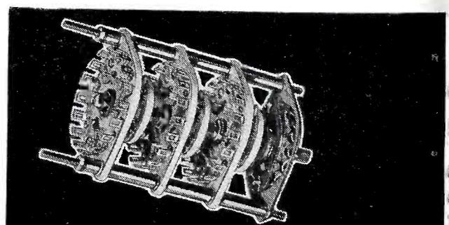
Specially designed for transmitters, power supply converters, X-ray equipment, etc., CRL medium-duty Power Switch gives efficient performance up to 20 megacycles. Minimum life operation of 25,000 cycles without failure.
