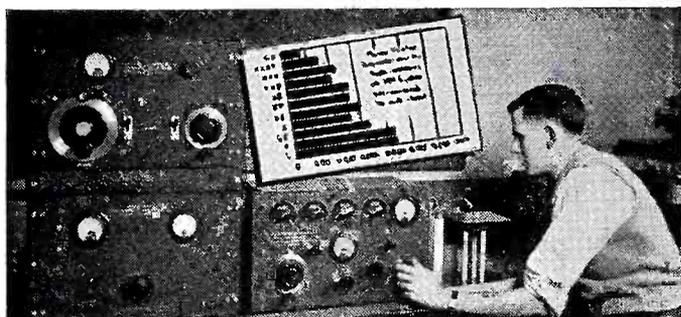
**Power Factor Test on Standard Dilecto Grades**—The standard test method is called the Resonant Circuit Resistance Variation Method. Measurements are at  $10^6$  cycles per second. Equipment for this test consists of a stable high frequency generator, a vacuum tube voltmeter, decade resistors, and a Standard Precision Type Variable Air Condenser.
