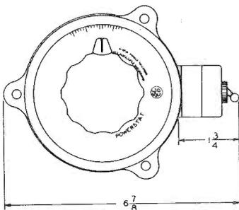
NOTE: WITH 2 AND 3 GANGED UNITS TERMINALS ONLY ARE PROVIDED. EXTENSION CORD, OUTLET RECEPTACLE, SWITCH, AND FUSE ARE NOT FURNISHED.
