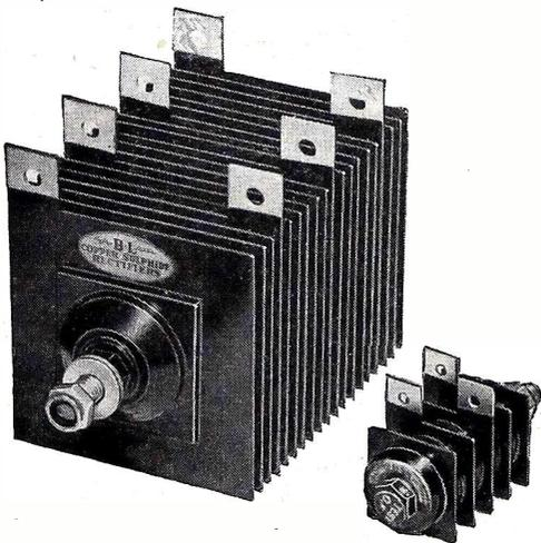
(Large Stack) Copper Sulphide. Three phase bridge, fan cooled. Output rating 100 amperes, 7 $\frac{1}{2}$  volts DC. Size over all 8" x 4 $\frac{1}{4}$ " x 3 $\frac{1}{2}$ ".
