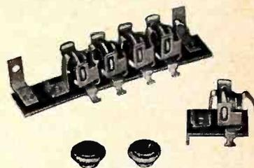
**GRID BIAS CELLS**, an exclusive patented Mallory product, are especially designed to provide dependable and constant grid bias potential in radio receivers, high gain voltage amplifiers, AVC circuits, hearing aids and many electronic applications employing Class A amplification. Individual cells and appropriate holders are available to accommodate one to four cells in series. Refer Notes A and B.
