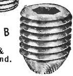
(B) The knurled cup point of this "Unbrako" Socket Set Screw makes it a Self-Locker—the point digs-in and stays dug—regardless of the most chattering vibration. Yet, it can be backed-out with a wrench and used over and over again. Sizes from #4 to 1-1/2" in diameter.
