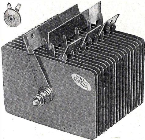
(Large Stack) Selenium Rectifier. Three phase bridge, fan cooled. Output rating 100 amperes, 14 volts DC. Size over all 7 $\frac{3}{4}$ " x 5 $\frac{1}{2}$ " x 6".
