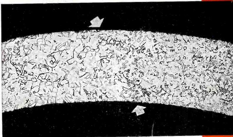
*Photomicrograph of transverse section of WELDRAWN\* stainless tubing showing \*complete recrystallization in weld area.*
