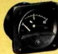
**SMALL PANEL . . .** These general-purpose panel instruments are particularly suitable for use in radio and communications equipment where accuracy and quality are required and space is at a premium. D-c, r-f, and a-f instruments operate on the permanent-magnet, moving-coil principle; alternating-current (a-c) instruments, on the moving-iron principle. 1 1/2 in. and 2 1/2 in. instruments find wide usage where minimum frontal dimensions and depth behind the panel are essential requirements.
