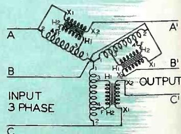
TYPICAL MANUALLY OPERATED THREE PHASE LINE CORRECTOR POWERSTAT TYPE LC CONNECTION 11
