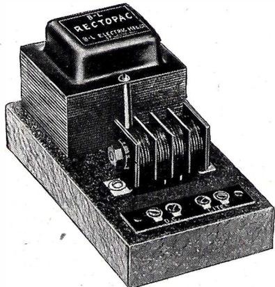
◀ B-L "RECTOPAC". Copper Sulphide Rectifier assembly. Output rating 10 amperes, 10 volts DC. Operates from 115 volts 50-60 cycles AC. Size 7 $\frac{1}{8}$ " x 4" x 4".
