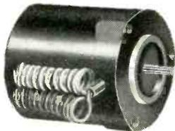
**GEARED INDUCTION MOTORS**—miniature 2-phase servo motors with gear reducer. Desirable motor features: Maximum torque at stall with low wattage input and high torque/inertia ratio. Gear reducer conservatively rated at 25 oz/in. Maximum torque with gear ratios from 5:1 to 75,000:1 available.
