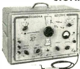
To meet FM and AM service requirements, here's Sylvania's new Signal Generator Type 216! With it you can align the rf and if sections of all FM and AM receivers, adjust all types of FM and TV discriminators, and make overall receiver checks. Its high level output and
