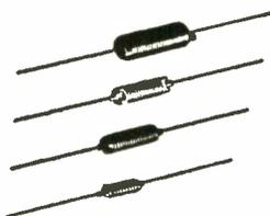
Single-layer wound on low power factor steatite or molded plastic cores. Seven stock sizes cover range 3 to 520 mc. Two units rated 600 ma; all others 1000 ma.
