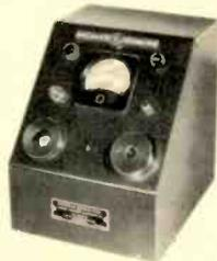
An extremely high-quality, self-balancing electrostatic potentiometer. A standard 3-inch meter provides direct measurement in two ranges—50 and 250 mr for rapid, accurate reading of "pencil" type pocket ionization chambers.
