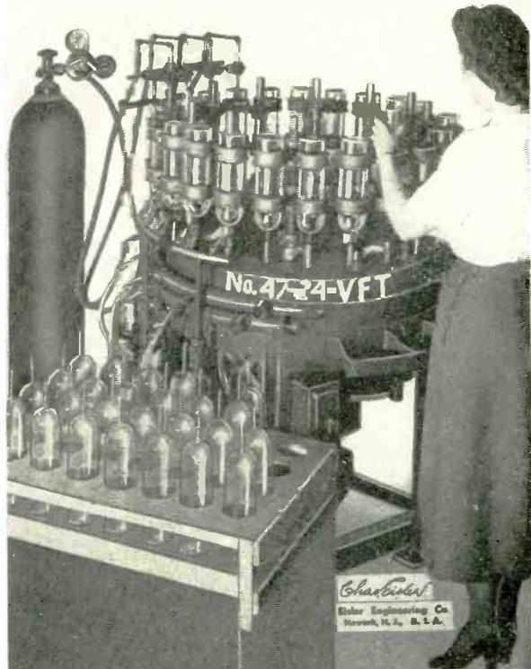
Automatic Piercing and tubulating machine for vacuum flasks.
