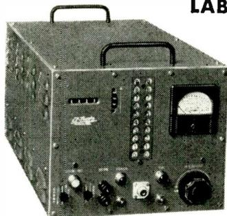
A completely modern unit, designed to speed up laboratory counting. Direct reading scale quickly indicates total count. No extra computing. Total count on 100 scale up to 999,999 or 9,999,999 on 1000 scale before recycling.
