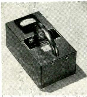
A portable Alpha meter in which alpha radiation is measured by means of an air ionization chamber, and a vacuum tube amplifier circuit which operates an indicating meter—light, compact, and unusually stable.
