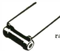
Resistors are wire wound on a ceramic core, rigidly held in place, insulated, and protected by vitreous enamel. Even winding dissipates heat rapidly —prevents hot spots. Many types, in ratings from 5 to 200 watts.
