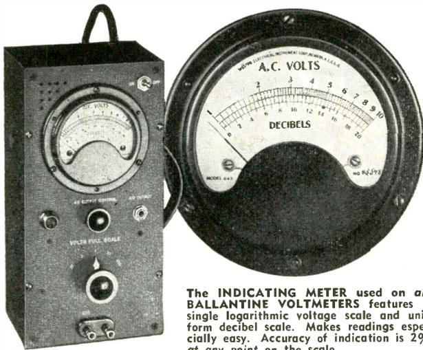
The INDICATING METER used on all BALLANTINE VOLTMETERS features a single logarithmic voltage scale and uniform decibel scale. Makes readings especially easy. Accuracy of indication is 2% at any point on the scale.
