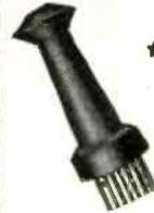
★ Star Miniature Socket Wiring Plugs for accurate alignment of miniature socket contacts during wiring. Precision cast of zinc base alloy—pins of stainless steel. #JE-9 (9 pin); #JE-10 (7 pin).
