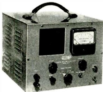
A practical time and cost saving accessory. When connected to the oscilloscope of such scalars as El-tronics models LS64, LS256, LS100, LS1000, CGM3B or the equal it becomes an integral part of the scalar, saving the expense of a complete counting rate meter.
