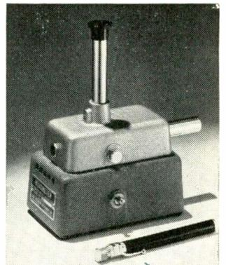
The Minometer provides a prescription for computing daily, the amount of radiation exposure. It consists of a small compact string electrometer and an ionization chamber designed in the shape of a fountain pen to be carried conveniently in a coat pocket. The chamber value is 0.2 r full scale when checked against the calibrated scale in the electrometer.
