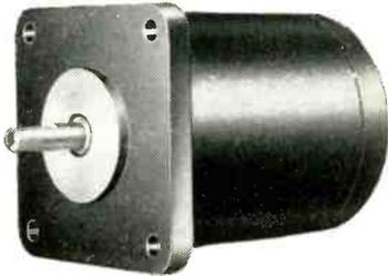
**MOTOR DRIVEN INDUCTION GENERATORS**—combination of a 2-phase, high-torque, low-inertia induction motor and an induction generator. Used as a fast reversing servo motor. Available with maximum stall torques of 1.0 (unit shown) to 6.7 (other units) oz/in.
