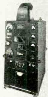
**2 KW AMPLIFIER—Class C RF Amplifier. Range: 1-25 Mc's.**
