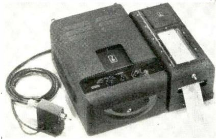
Used with Brush Magnetic Direct Inking Oscillograph and BL-306 Pickup Head, measures small displacements within the range of .000010 in. to .015 in. Utilizing a carrier type displacement sensitive pickup, produces immediate records of absolute values. The
