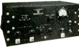
Model TAA-16 is designed for use with square-law-detector probes and slotted wave-guides in determination of standing-wave voltage ratio. Operating frequencies 500 to 5000 cycles, wide band or highly selective. Full-scale readings with less than 15  $\mu$ -volts at input with wide band, 10  $\mu$ -volts with selective operation.
