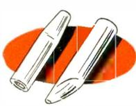
resistance welding electrodes.
