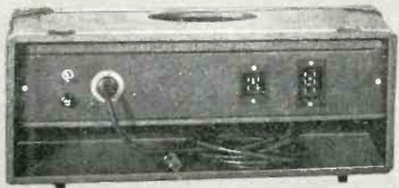
PORTABLE TAPE RECORDER 900-P . . . Complete in two easily portable cases. Includes three heads for superior performance, three microphone channels in amplifier, Weston type V. U. meter, 2-speed single motor drive. New, and the finest recorder of its type available anywhere.
