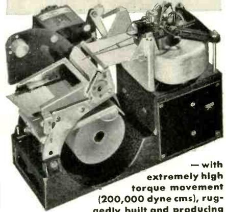
— with extremely high torque movement (200,000 dyne cms), ruggedly built and producing clear, permanent records.
