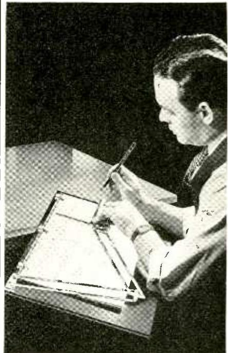
and paper clamps, all in one, and the size is about the same as a brief case. The entire drafting mechanism is precision engineered of non-reflecting metal. Angles from 0 to 360° are available.
