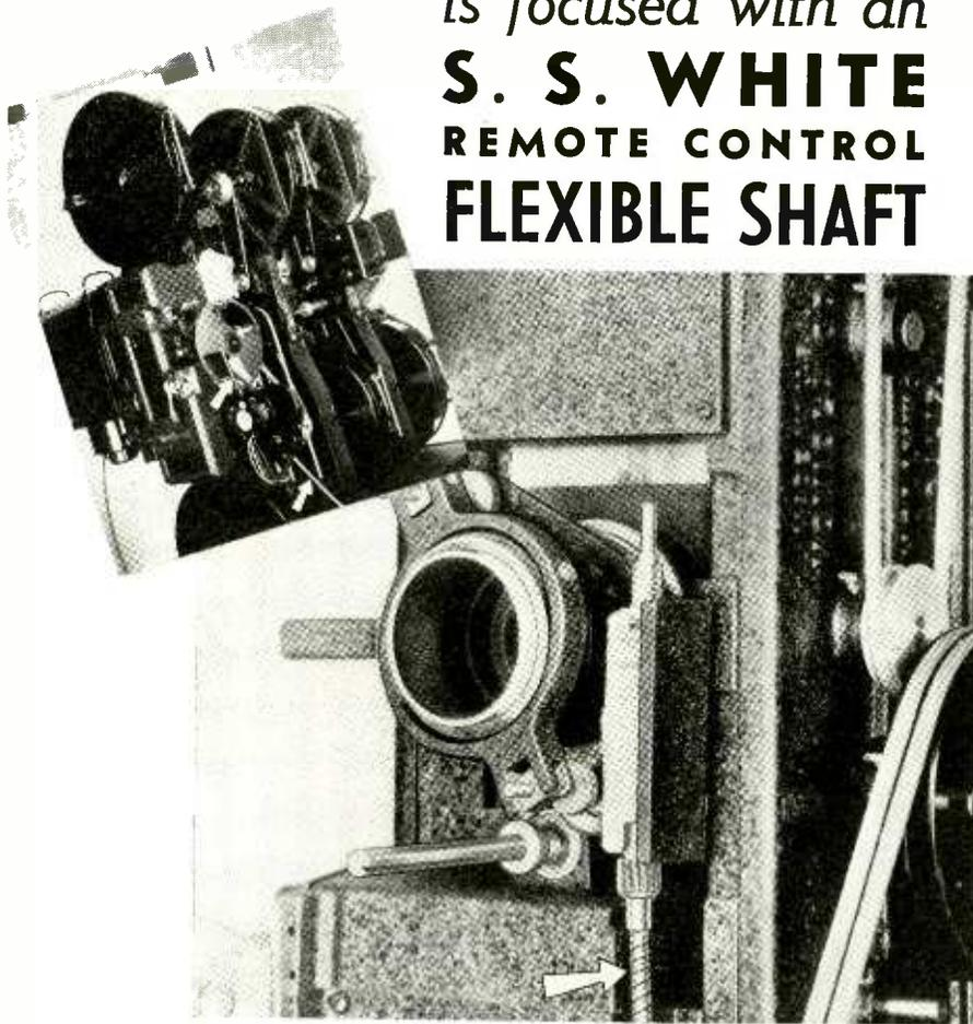
**This** projector is one of eight in the studios of Walt Disney, equipped with S. S. WHITE Flexible Shafts for focusing. The shafts are of the type specially developed by S. S. WHITE for remote control.
