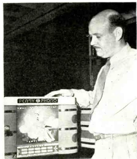
Dr. Gordon K. Woodward, Los Angeles physician, recently developed this automatic phonograph which sells tunes to the public at a rate of a penny a tune, instead of the customary nickel now required. The device was made practical through the development of a new type of record which is 16 inches in diameter and contains 10 separate songs on each side. Each side of the record contains more than one hour of tunes
