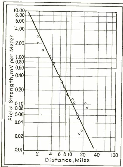
Fig. 2—Field strength vs distance for three meter waves plotted on logarithmic coordinates
