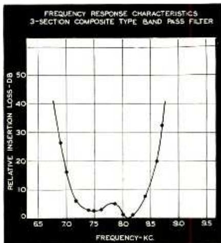
Fig. 9—Response characteristic of three-section bandpass filter used in circuit in Fig. 8
