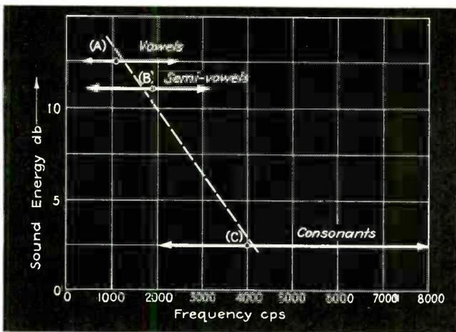
Fig. 1—The relationship between the frequency components and the corresponding power levels associated with various speech sounds, on which Mr. Csepely's scheme is based
