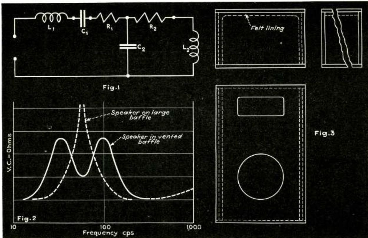
Fig. 1—Equivalent electrical circuit of the mechanical operation of the speaker diaphragm in the vented enclosure. Fig. 2—Impedance-frequency characteristic of the vented
