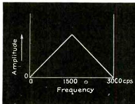
Fig. 5—Frequency response characteristic of the output when oscillator frequency varies continuously
