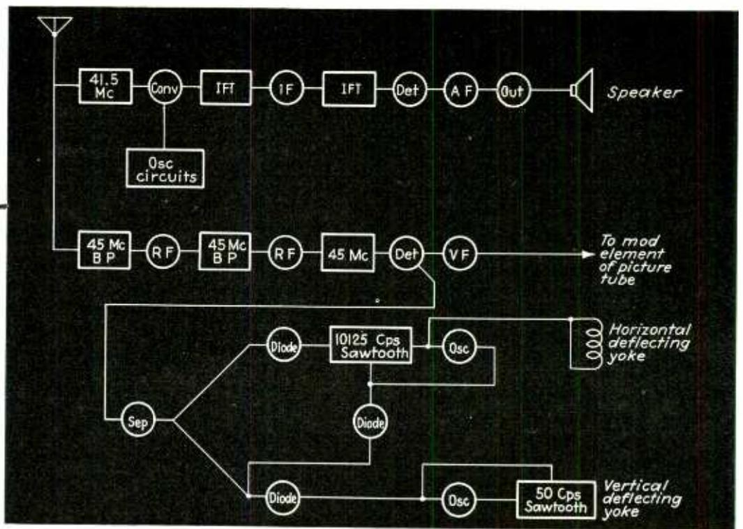
followed by a flatly tuned i-f transformer, double wound, feeding a pentode i-f amplifier and thence through a further double wound i-f transformer to the diode of a conventional double diode-triode circuit, resistance coupled to an output pentode. Avc was provided on the i-f stage only. The separate power-pack chassis was equipped with a single, half-wave high-voltage rectifier and with a pair of parallel-connected low-voltage rectifier tubes.
