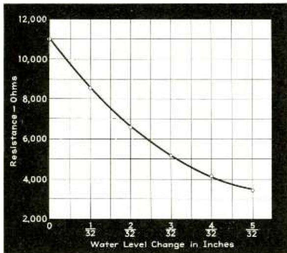
Fig. 5—Curve showing the change in resistance  $R_2$  as the pointer is immersed in the water
