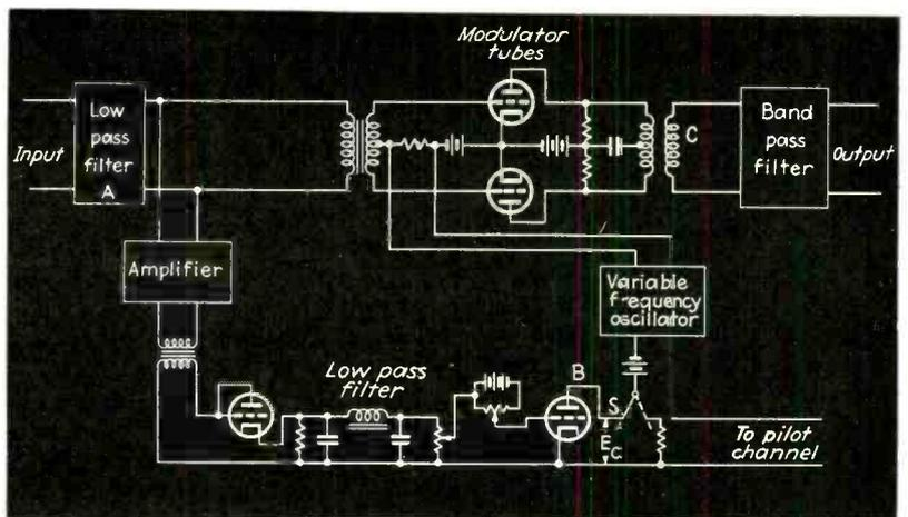
Fig. 2—Practical means of shifting the sideband components from instant to instant so that they fall within the channel limits for use at the transmitter
