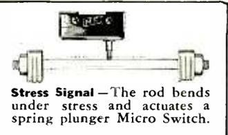
**Stress Signal**—The rod bends under stress and actuates a spring plunger Micro Switch.
