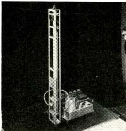
Reverberation device which uses a spring for sound transmission
