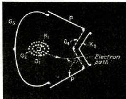
Fig. 3—High mutual conductance tube which makes use of secondary emission and permits the high gain necessary in television receivers
