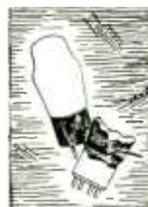
**VACUUM TUBES:** Films formed with “dag” colloidal graphite discourage secondary and undesirable primary emission emanating from vacuum tube elements. Electrostatic shielding may also be accomplished.
