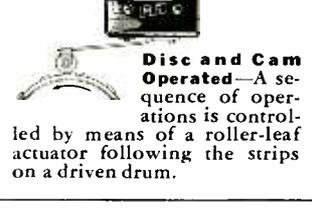
**Disc and Cam Operated**—A sequence of operations is controlled by means of a roller-leaf actuator following the strips on a driven drum.
