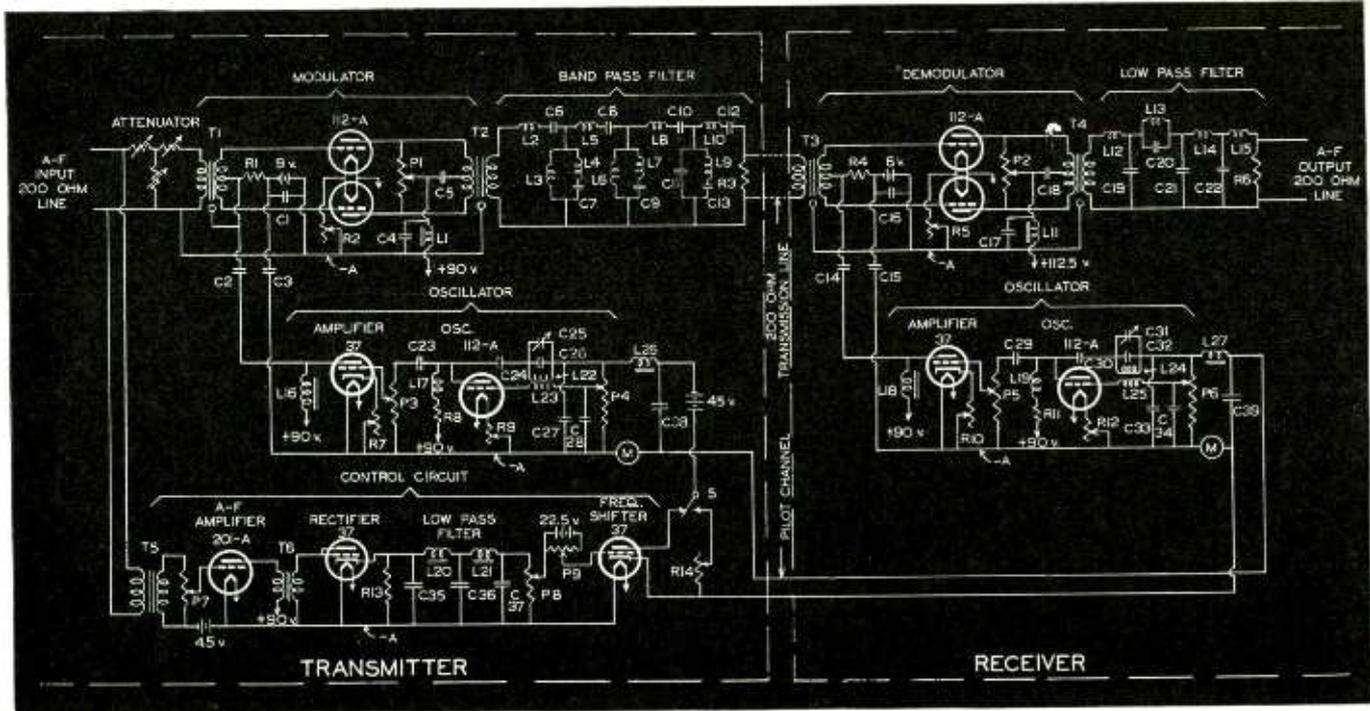
Fig. 8—Complete circuit diagram of experimental narrow-band set-up
