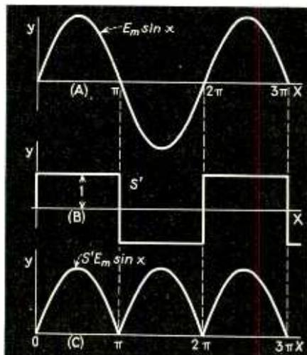
Fig. 2—Typical voltage curves of the full wave rectifier
