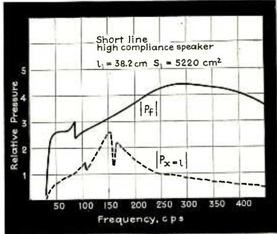
Fig. 12—Observed pressure at front and back of acoustic line using a high compliance speaker
