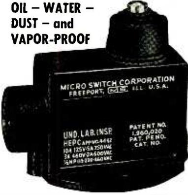
Here is the new Water-Oil-Dust and Vapor Proof Micro Switch for non-hazardous locations. Genuine Neoprene seals and gaskets are used. Strong field wiring terminals accept No. 14 solid wire. The die cast housing is rugged—and standard 1/2" conduit hub makes installation handy. Ask for Bulletin No. 5.
