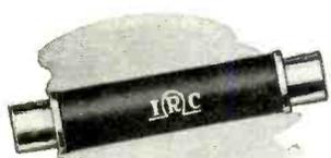
**"C" COATING**... Developed especially for the most severe conditions such as met on shipboard, tropical countries, intensely humid climates, etc. Withstands the standard U. S. Navy hot and cold salt water immersion cycling tests. Temperature rise and wattages are the same as for the IRC Type "A" Coating.
