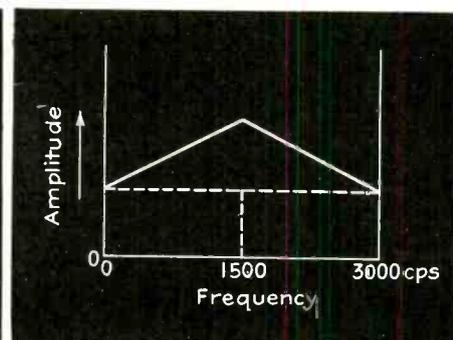
Fig. 6—Characteristic when oscillator frequency remains constant one third of the time
