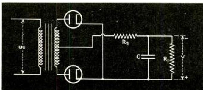
Fig. 7—A typical rectifier power supply.  $R_1$  is the load and  $C$  and  $R_2$  make up filter
