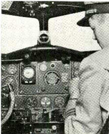
Position of flight-ray indicator on airplane instrument board. The indications coordinate as many as four instruments simultaneously, doing so without confusing the pilot
