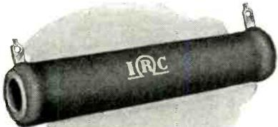
**"B" COATING**... The ideal coat for relatively low-range, high-temperature requirements where wire sizes are sufficiently large to assure dependability. Admirably suited for general normal atmospheric requirements. Ratings based on 250° C. rise from a 30° ambient in free air.
