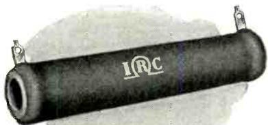
**"B" COATING**... The ideal coat for relatively low-range, high-temperature requirements where wire sizes are sufficiently large to assure dependability. Admirably suited for general normal atmospheric requirements. Ratings based on 250° C. rise from a 30° ambient in free air.
