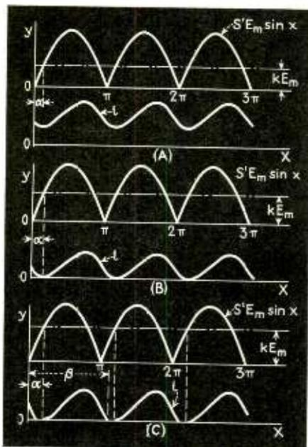
Fig. 4—Voltage and current curves of the rectifier shown in Fig. 3 for the condition of no current cutoff
