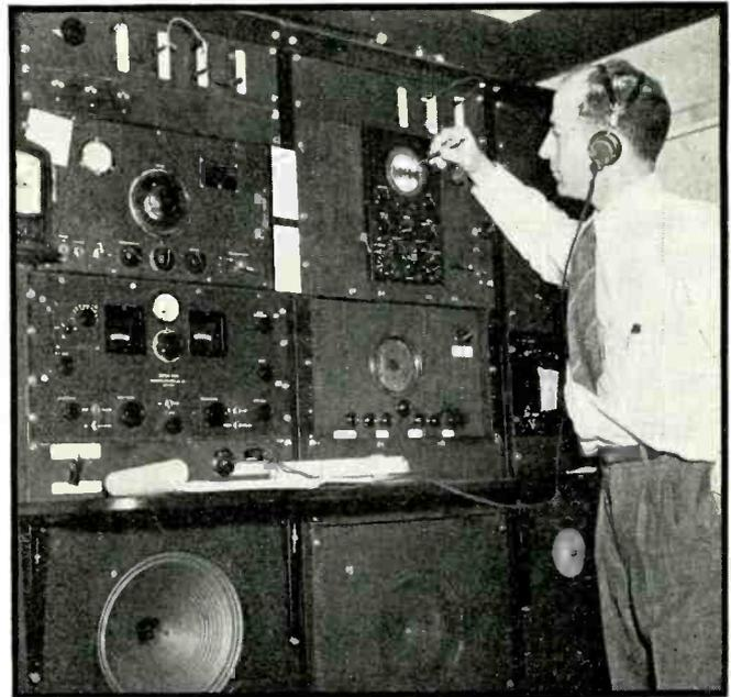
Percentage modulation and other aspects of the modulation envelope are monitored on a cathode ray oscilloscope, fed from any of several calibrated communication receivers. James Homsy, inspector in charge of the station, is shown on the job
