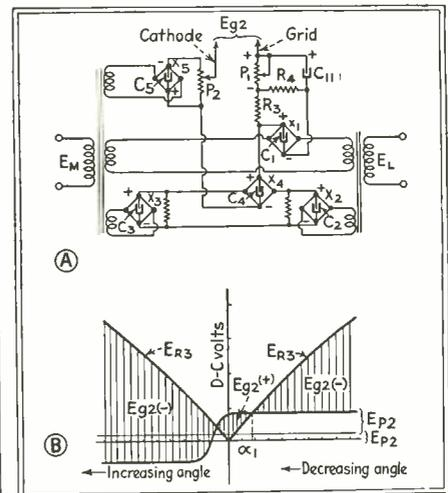
Fig. 3—Grid control circuit for the tube  $T_2$  and the grid control voltage phase difference characteristics
