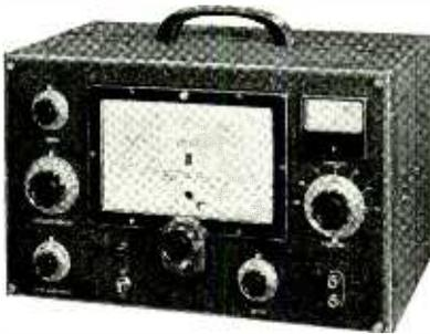
The model CR-6-A beat frequency standard signal generator supplies a reliable signal of known potential and frequency over the wide ranges of from 10 micro volts to 100 volts any where in the range from 10 cycles per second to 50 kilocycles per second.
