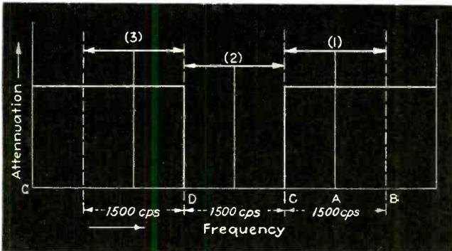
Fig. 3—Characteristic of an ideal 1500-cps bandpass filter, showing how a region 4500 cps wide may be shifted into the pass region
