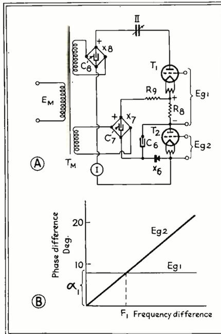
Fig. 1—Electronic interlocking circuit for generator synchronization and its grid control voltage requirements
