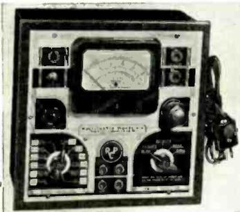
The system of A.C. measurements, employed in this Model assures higher accuracy, greater ruggedness, and far greater sensitivity than is obtainable with the copper oxide rectifier method. Meter movements are approximately 450 microamperes for full scale deflection. Meter protected by instrument fuse and double double fuse.
