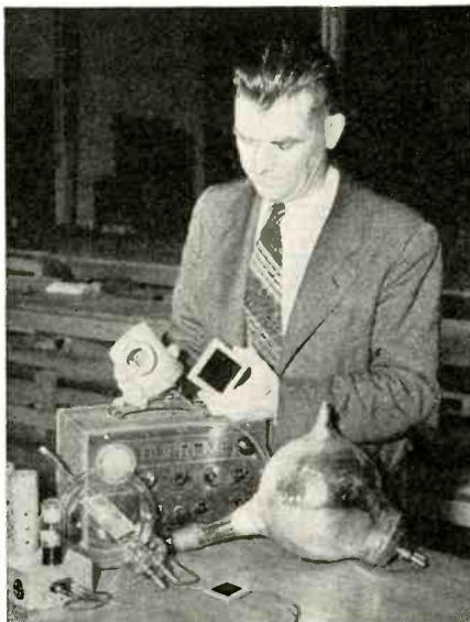
Guy Ball, exhibiting a newly invented instrument which, it is claimed, will enable aircraft pilots to see through fog. The device operates as a miniature television system to provide a picture of the terrain below the plane, on the screen of a cathode ray tube. Demonstrations have been given showing the effectiveness of the device to "see through" infrared filters, but field tests under actual operation are still to be made
