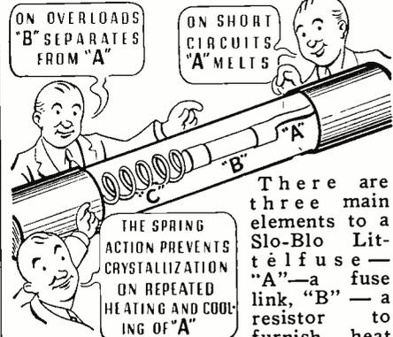
There are three main elements to a Slo-Blo Littelfuse—“A”—a fuse link, “B”—a resistor to furnish heat inertia, and “C” a spring for tension. This Slo-Blo Littelfuse protects equipment having high inductive or capacitive surges. It gives extra value to intermittent duty circuits where frequent cycles of operation would crystallize and break a simple fuse element.
