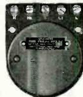
**Time Delay Relays (Model 613)** Compensated bi-metal operation... single or double circuit... provides time delay of 15 seconds to 1 minute between initial impulse and operation... handles up to 25 watts at 110-volts output.
