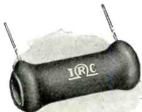
**"A" COATING**... An organic cement coating designed for domestic, medium- and high-range applications where low cost and good protection from abnormal humidities are required. Has a temperature rise limitation of 130 degrees C. from 30 degrees C. ambient in free air.
