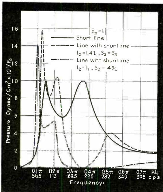
Fig. 5—Computed pressure curves for an acoustic line, and an acoustic line with a shunt line
