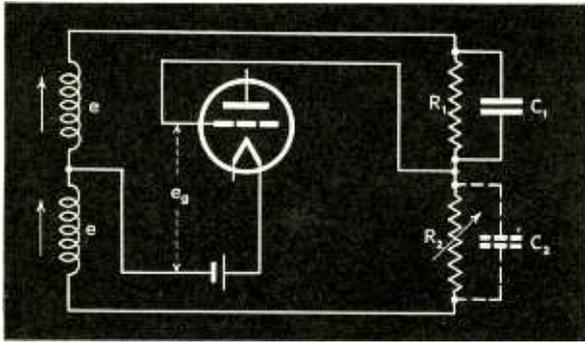
Fig. 3—The operation of the indicator depends upon the balance or unbalance between  $R_1$  and  $R_2$ .
