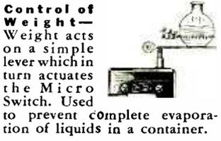
**Control of Weight**—Weight acts on a simple lever which in turn actuates the Micro Switch. Used to prevent complete evaporation of liquids in a container.
