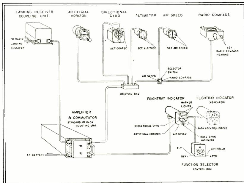
The "Flight-Ray" aircraft instrument indicator, which applies the readings of four instruments simultaneously to the face of a cathode-ray tube
