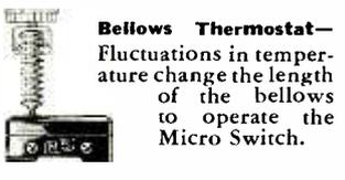
**Bellows Thermostat**—Fluctuations in temperature change the length of the bellows to operate the Micro Switch.
