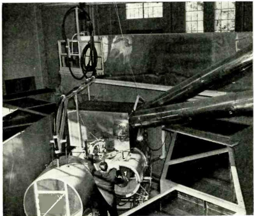
A view of the huge 220 ton cyclotron at the William H. Crocker Radiation Laboratory of the University of California. The vats of water surrounding the machine are for radiation protection for the workers. The tubes above lead from the oscillator
