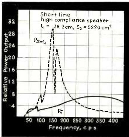
Fig. 10—Observed power output at front and back of acoustic line (Fig. 1) using a high compliance speaker
