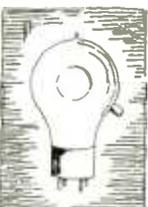
**PHOTOELECTRIC CELLS:** Graphite surfaced electrodes absorb free alkalis and alkaline metals in photoelectric cells. No selenides result when the “dag” product is used in the selenium types.
