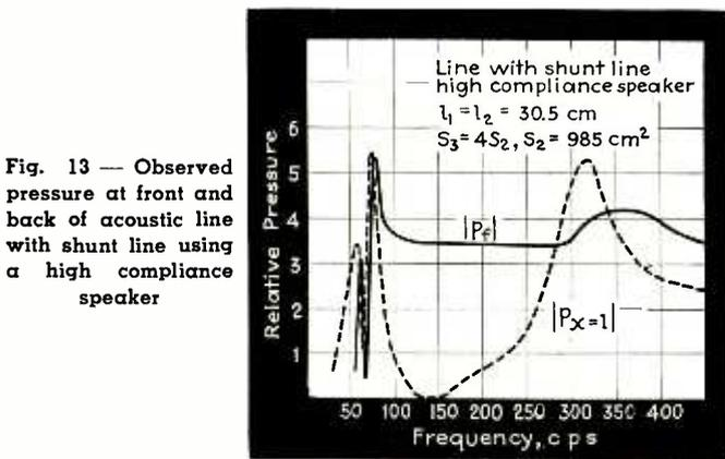
Fig. 13 — Observed pressure at front and back of acoustic line with shunt line using a high compliance speaker
