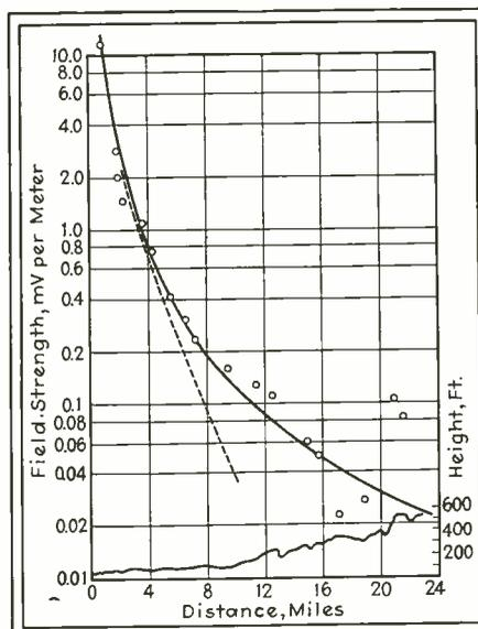
Fig. 1—Field strength vs distance for three meter waves. The wavy line is the contour of the land between the transmitter and receiver
