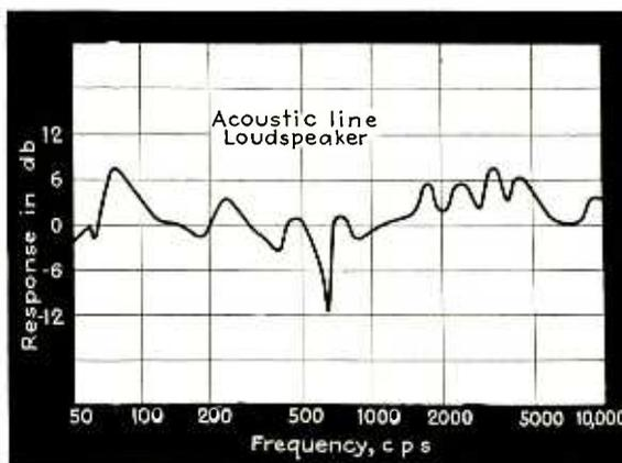
Fig. 14 — Frequency characteristic of the acoustic line loudspeaker
