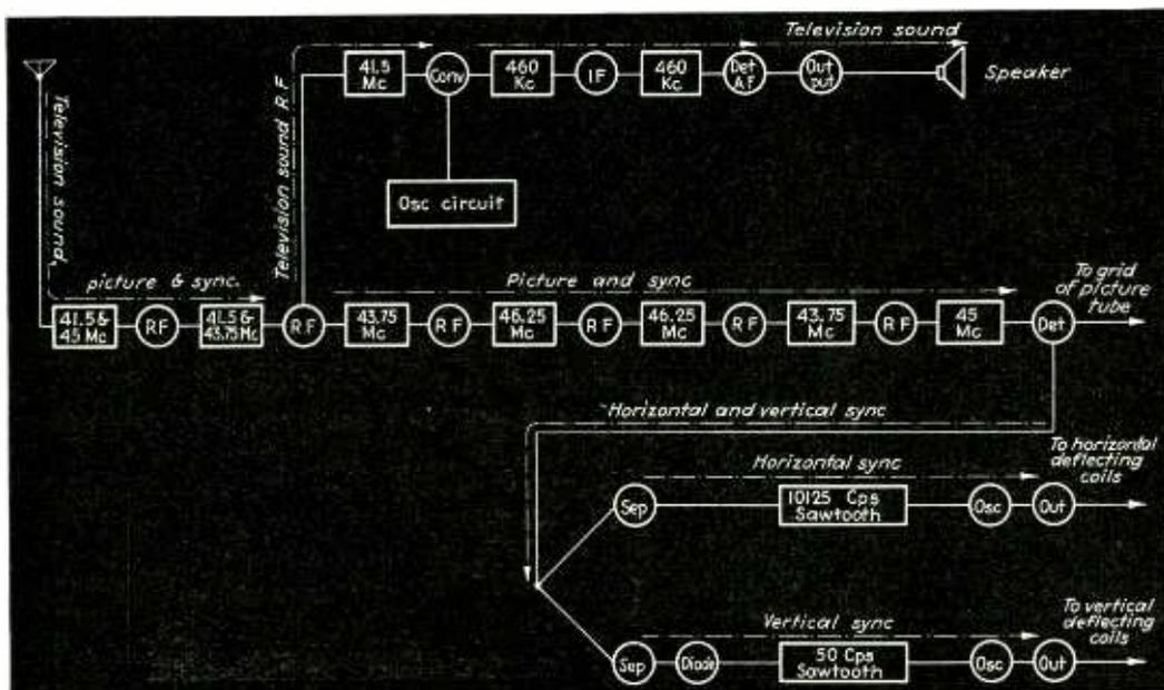
Fig. 1—Block diagram of an early British television receiver. Four chasses were used plus a metal container for the picture tube
