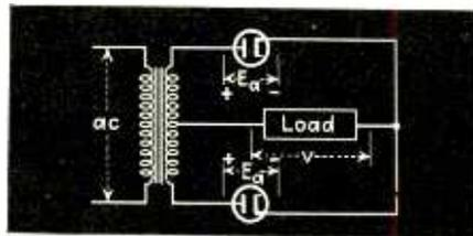
Fig. 1—Circuit diagram of typical full wave rectifier
