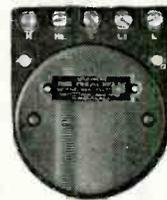
**Time Delay Relays (Model 613)** Compensated bi-metal operation... single or double circuit... provides time delay of 15 seconds to 1 minute between initial impulse and operation... handles up to 25 watts at 110-volts output.
