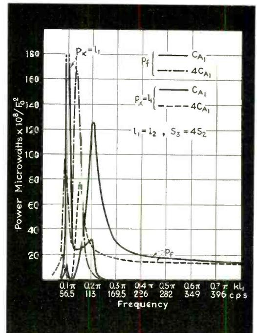
Fig. 7—Computed power output at front and back of the line with shunt line for two values of speaker compliance
