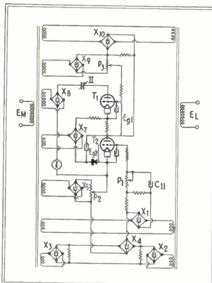
Fig. 4—Circuit diagram for the complete electronic synchronizer for power generators
