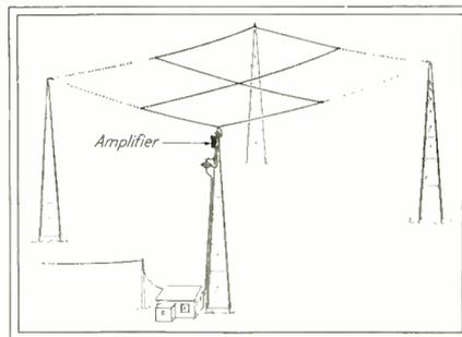
Rhombic receiving antenna and relay amplifier (on tower)
