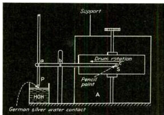
Fig. 7—As the water level changes the frame A also changes causing a deviation in the curve being drawn on the rotating drum
