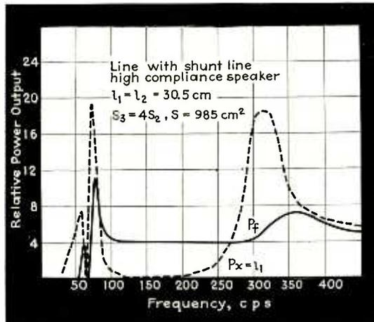
Fig. 11—Observed power output at front and back of acoustic line with shunt line using a high compliance speaker
