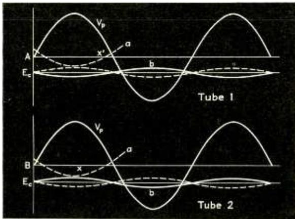
Fig. 4—Curves of the voltages which are applied to the thyatron rectifier
