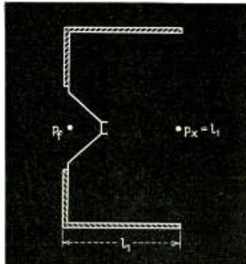
Fig. 1—Sound chamber of a conventional radio cabinet
