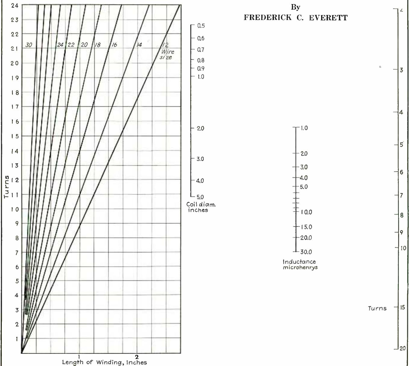
Charts in various forms have been available for the design of short-wave inductances, but there has been nothing to insure that the highest possible Q had been obtained in the design. By utilizing the information produced by Pollack<sup>1</sup> it has been possible to make the entire computation without "cut and try."
