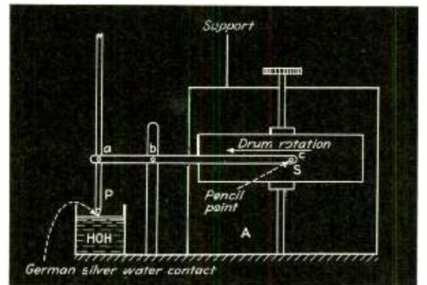
Fig. 7—As the water level changes the frame A also changes causing a deviation in the curve being drawn on the rotating drum
