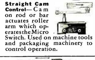
**Straight Cam Control**—Cam on rod or bar actuates roller arm which operates the Micro Switch. Used on machine tools and packaging machinery to control operation.
