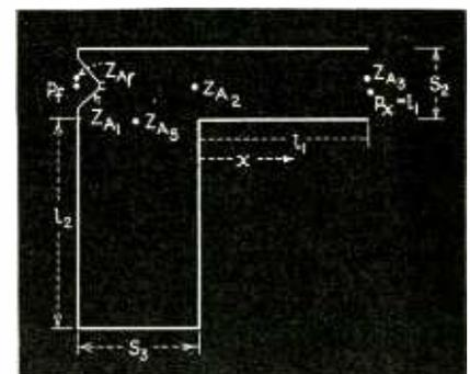
Fig. 3—Above, diagram of an acoustic line with a shunt line
