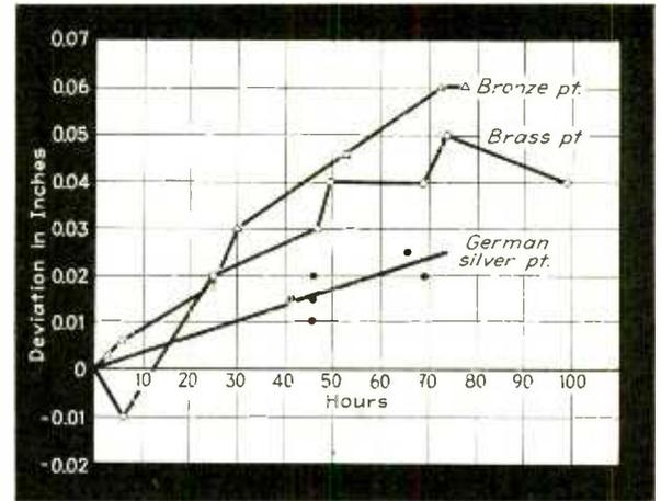
Fig. 6—Curves showing the variation in indication due to the use of different metals for the pointer
