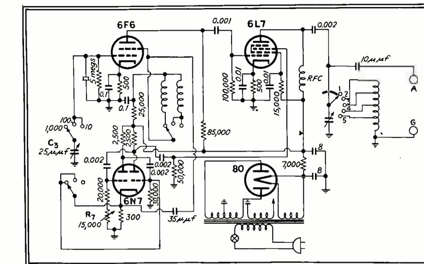
Circuit diagram of the Hallicrafters crystal controlled frequency standard which provides signal of a wide variety of frequencies and is easily calibrated
