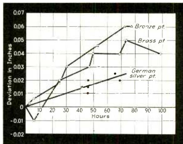
Fig. 6—Curves showing the variation in indication due to the use of different metals for the pointer
