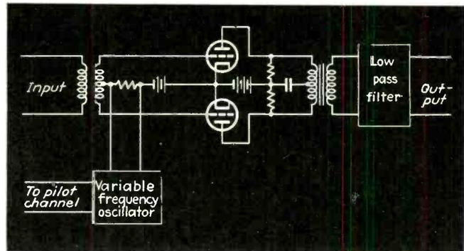
Fig. 4—The receiving end of the narrow-band system. The pilot channel controls a variable oscillator which reverses the shift introduced at the transmitter
