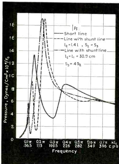
Fig. 6—Computed curves of the pressure at the speaker for an acoustic line, and a line with a shunt line
