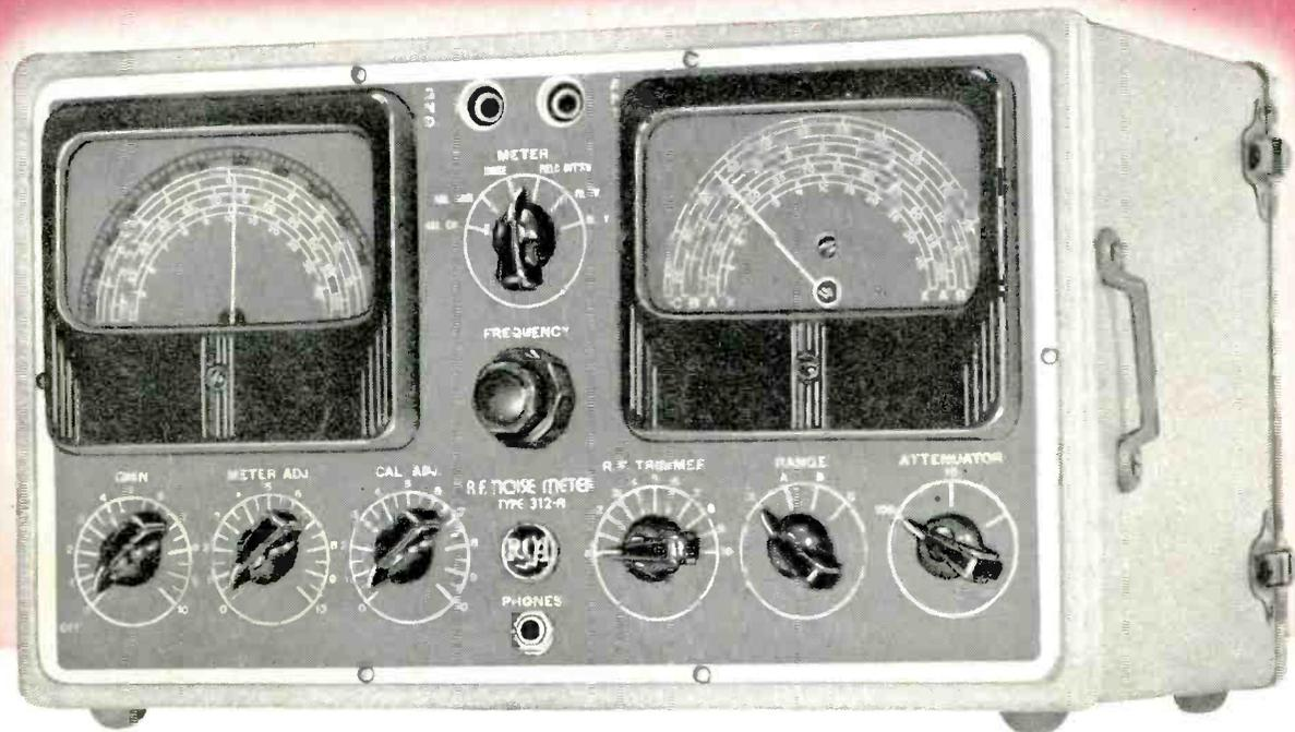
**T**HE NEW RCA 312-A Noise Meter answers a need for a meter to measure radio interference felt by utility companies, manufacturers of electrical appliances, and broadcast stations. It is a flexible instrument designed in accordance with the recommendations of the Joint Committee of the Edison Electric Institute, the Radio Manufacturers Association, and the National Electrical Manufacturers Association.
