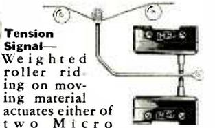
**Tension Signal**—Weighted roller riding on moving material actuates either of two Micro Switches to indicate tension on material.
