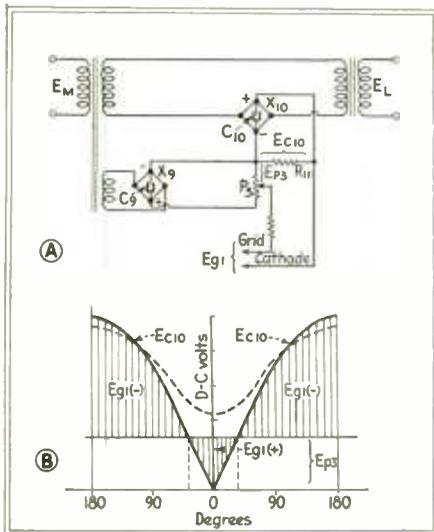
Fig. 2—Grid control circuit for tube  $T_1$  and the grid voltage phase difference characteristics
