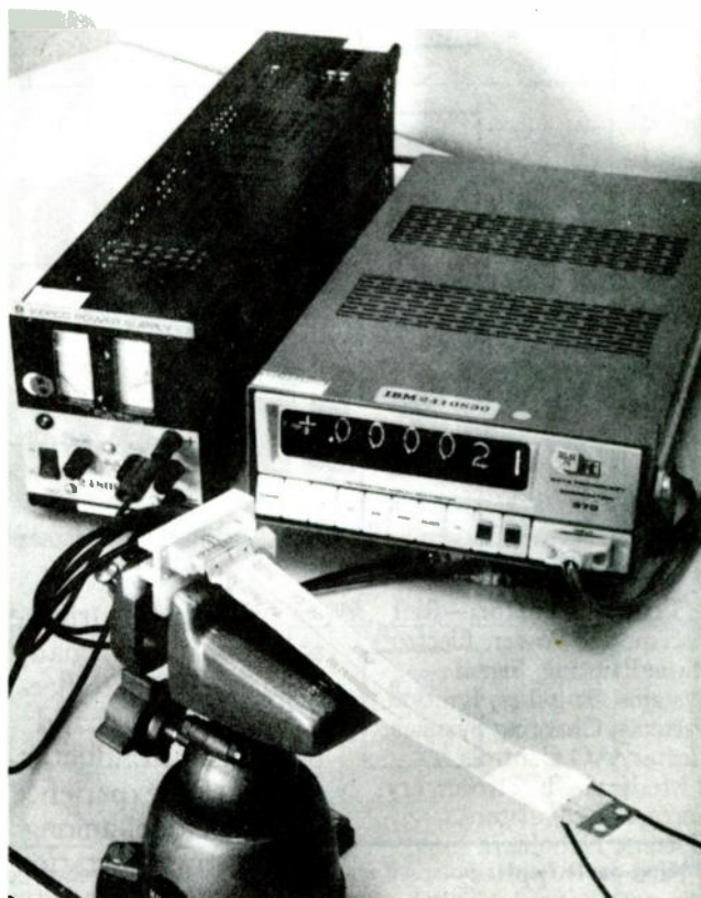
1. Test arrangement. Measurement tests joint between bus and connector. Soldered assembly, in jig, is shown close up in Fig. 4.
