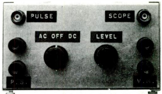
2. All packed up and ready to go. Complete electronic load circuit, including the 9-volt battery that powers it, is housed in a standard 3-by-2-by-5/4-inch aluminum box. Connectors can be seen.
