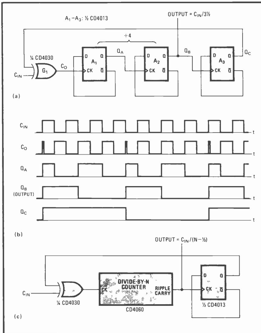
**Half-integer divider.** Divide-by- $3\frac{1}{2}$  counter is divide-by-4 circuit modified by flip-flop  $A_3$  and exclusive-OR gate  $G_1$  (a). Timing diagram details operation (b). Method may be extended to form a divide-by- $(N - 1/2)$  counter by replacing flip-flops  $A_1$  and  $A_2$  by ripple-carry, divide-by- $N$  counter (c).
