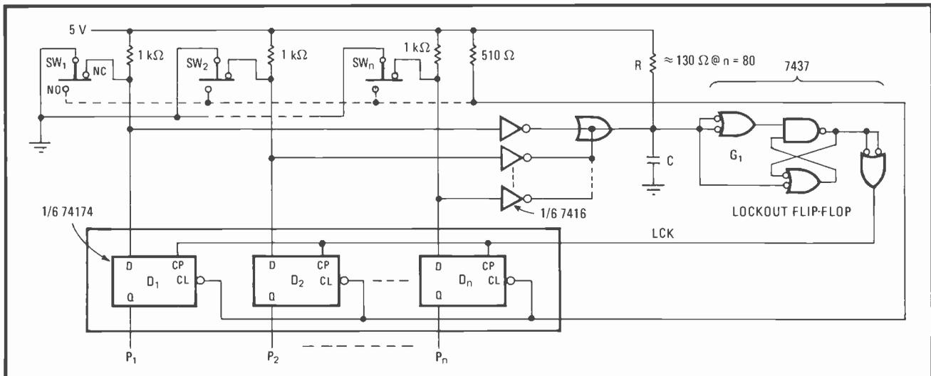
**Simplification.** Momentary-contact priority encoder uses about one fifth the number of chips of previous design. Circuit responds to first command received by switches and locks out all subsequent commands, thus forming a first-come, first-served switch.
