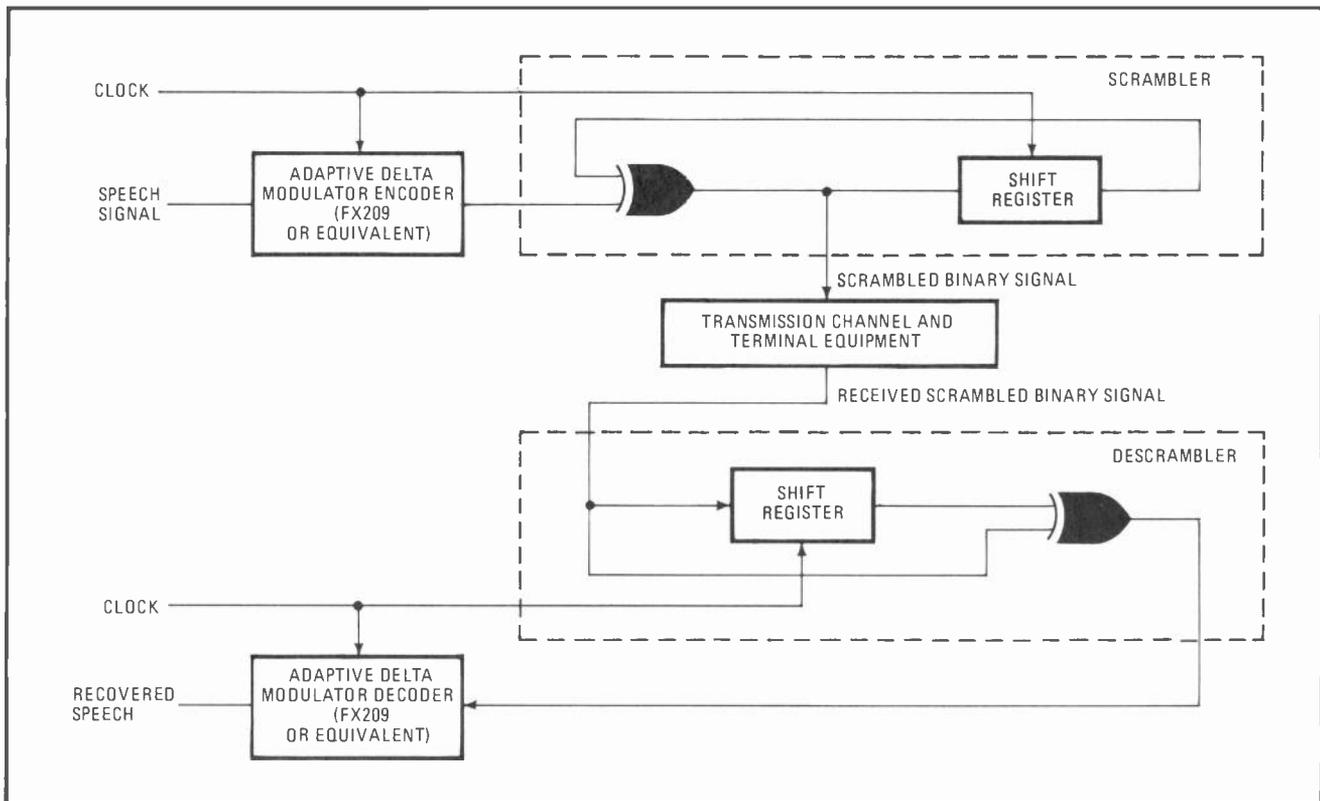
**11. Scrambling speech.** Clocking a shift register along with an adaptive delta modulation encoder and adding an exclusive-OR gate provides a scrambled binary signal, which can be first unscrambled and then decoded by a similar setup at the receiving end of the link.
