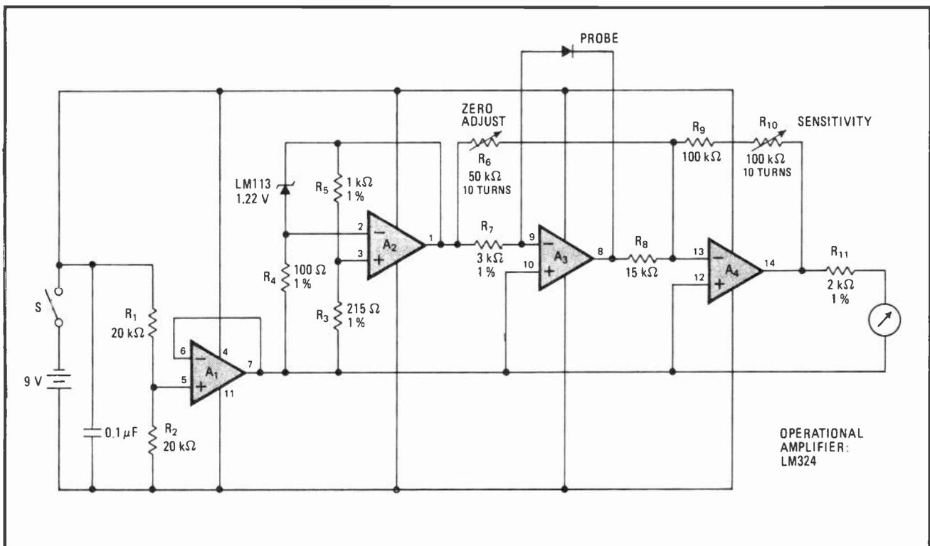
**Precision thermometer.** Accuracy is limited primarily by ammeter readability. Thermometer is sensitive enough for medical applications where temperature variations are small. LM113 can be replaced by two silicon diodes in series for less demanding applications.
