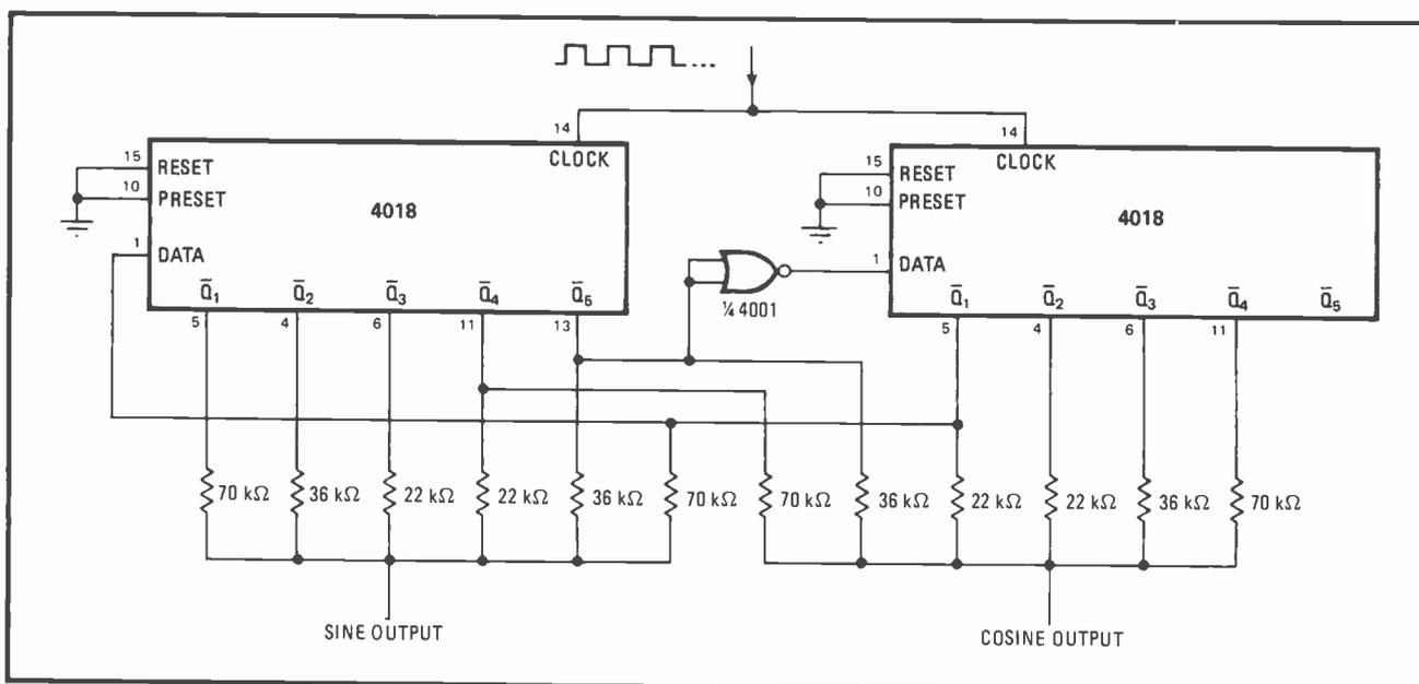
**Digitized waves.** Frequency dividers and weighted resistor network generate sine and cosine waveforms. The 4018 counters divide input frequency by 12. First counter provides 12-bit approximation of sine function. Second device lags by 90°, producing cosine waveform.
