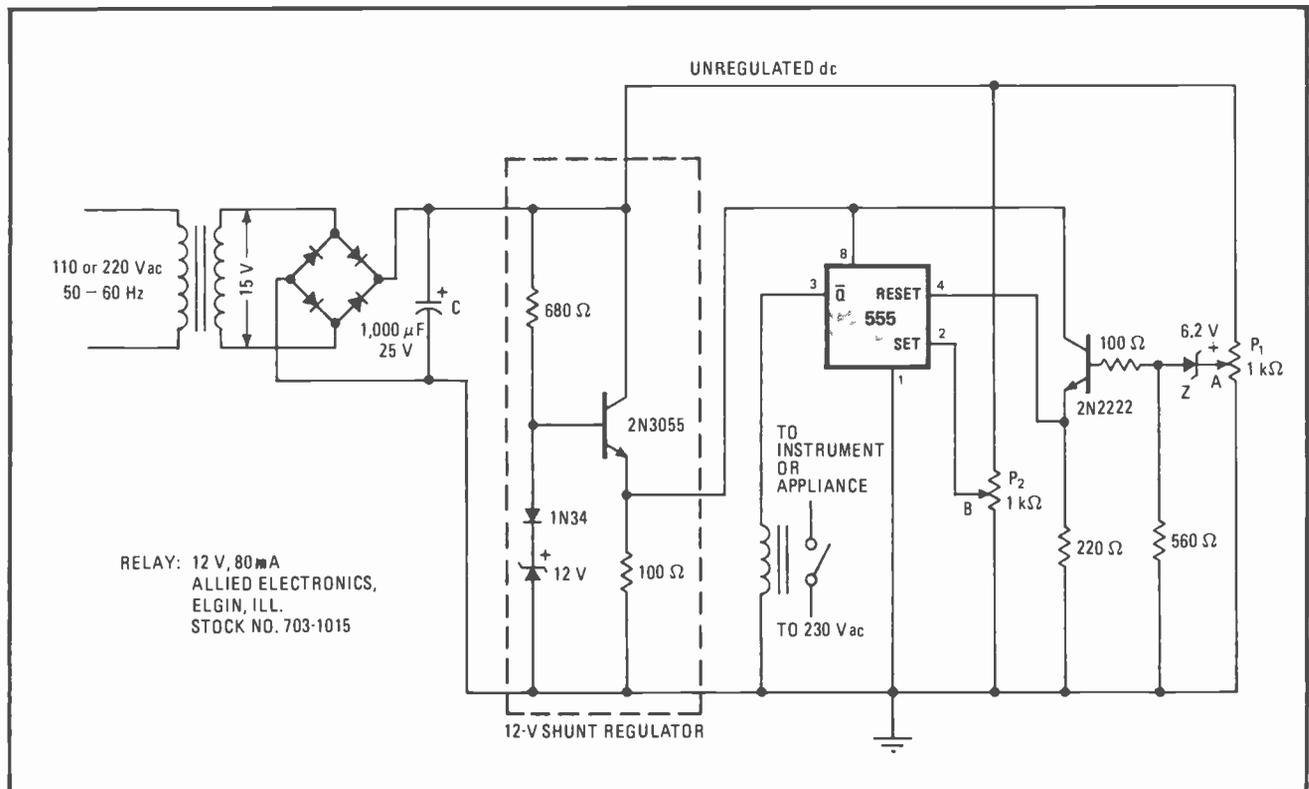
**Line-voltage monitor.** 555 timer circuit senses if ac line voltage is above or below set limits, then de-energizes line relay if necessary, removing power from equipment. Simple circuit uses set-control potentiometers P<sub>1</sub> and P<sub>2</sub> to monitor unregulated dc voltage, whose value is directly proportional to the ac line voltage. Timer and 2N2222 transistor require the regulated power source.
