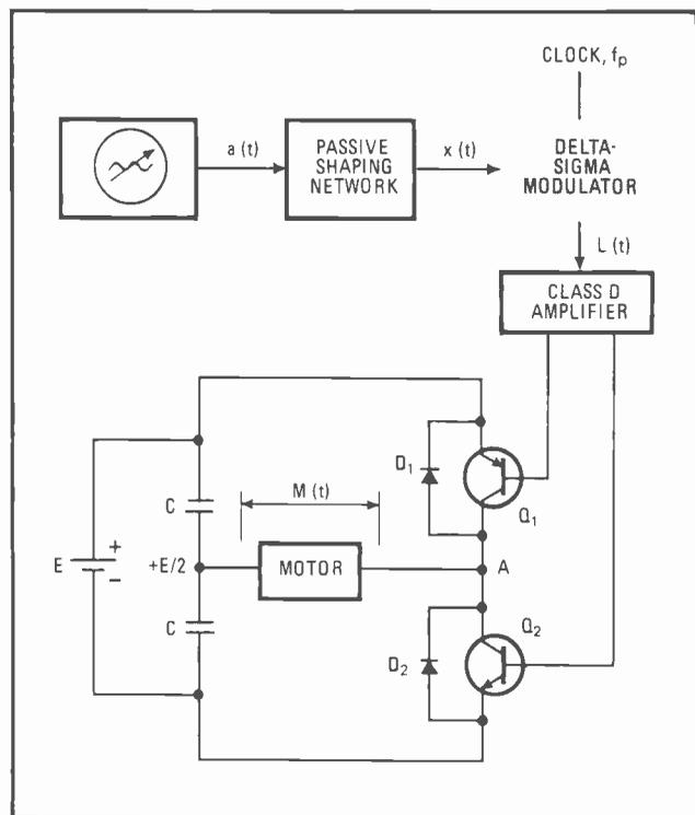
**10. Remote control.** There is an advantage in using a delta-sigma modulator for the remote control of an induction motor—the speed-torque characteristics of the motor can be easily controlled even when it is separated from the controller by a noisy channel.
