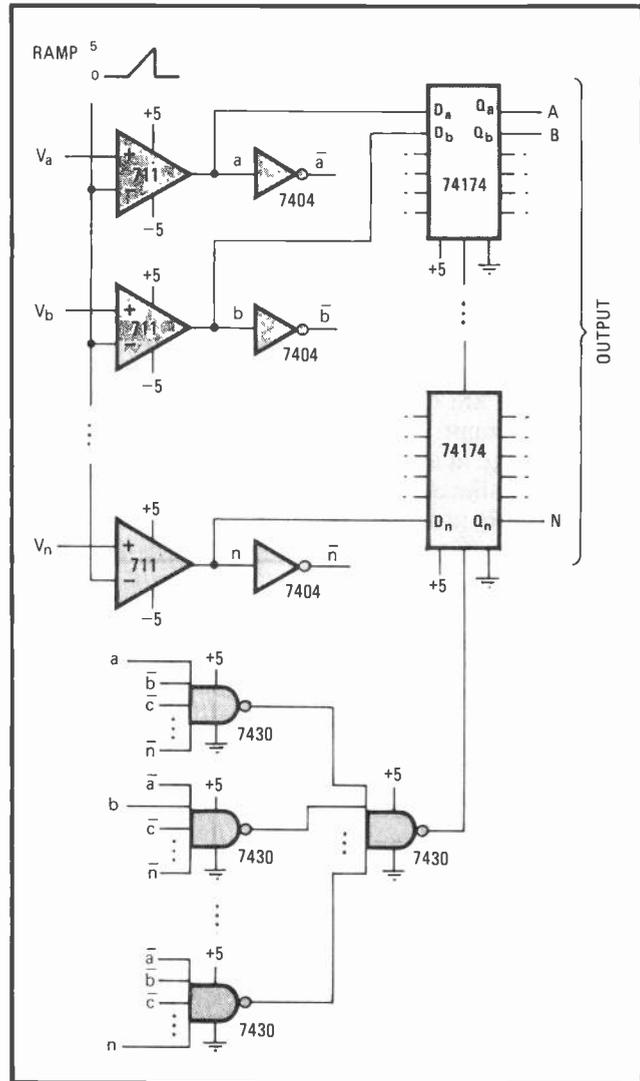
**Maximum-voltage detector.** Relative maximum of sample set  $V_1 - V_n$  is determined by ramp generator and logic circuit. Sample voltages drive all comparators high if values lie above the minimum ramp voltage. Logic detects lone op amp remaining high during the ramp sweep and clocks that state to its D flip-flop.
