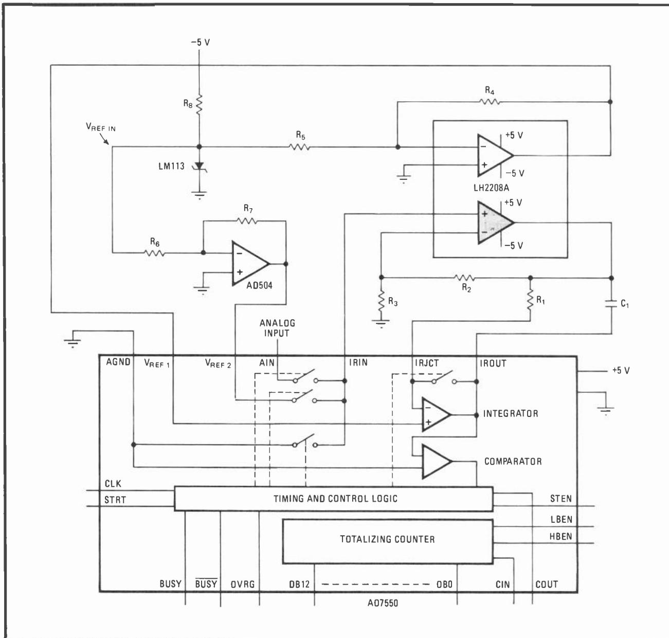
**1. Improved performance.** AD7550 accurately measures even microvolt-level analog voltages if op-amp buffer is placed in converter's integrator and error compensation loop. Converter views offsets as just another error that has been introduced in integrator loop.
