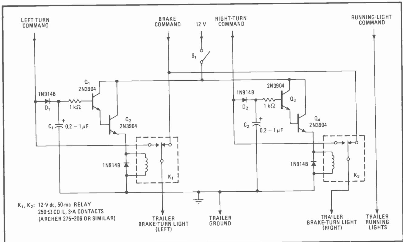
**Auto-to-trailer interface.** Relays multiplex brake and turn commands onto common bus line, permit control of brake-turn lights on trailer. Darlington amplifiers provide high command-line isolation and sufficient drive for the relays.
