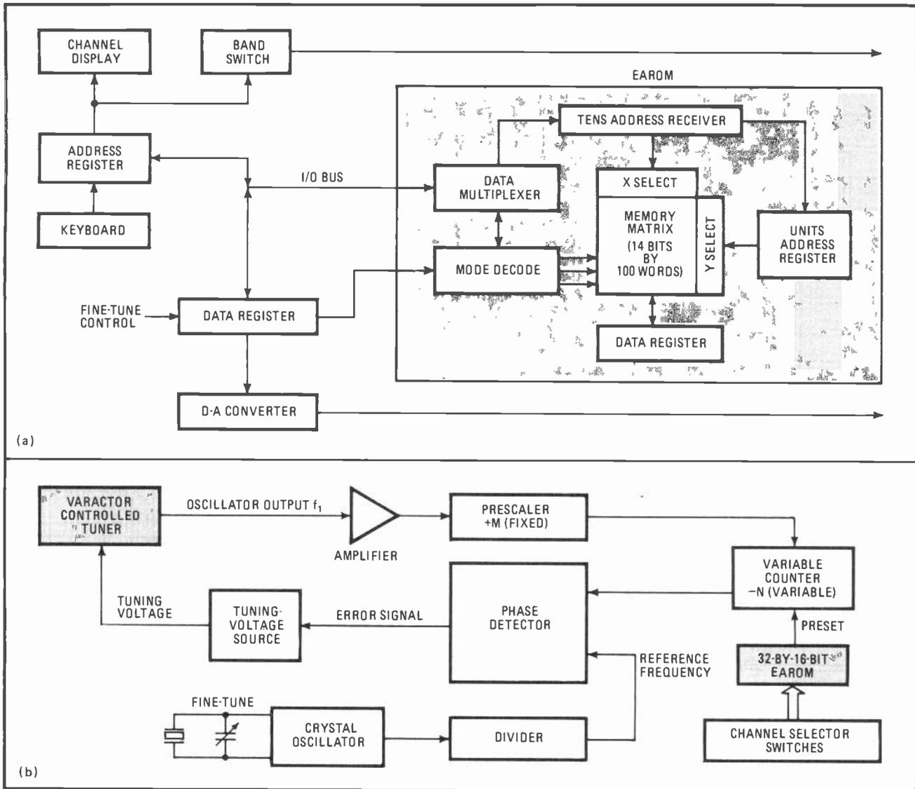
**8. Tuning a television set.** In varactor tuning (a), the electrically alterable ROM stores digital information that goes to a digital-to-analog converter to provide the proper bias to the varactor. In phase-locked-loop systems (b), the alterable ROM stores the proper division information for the various desired channels by controlling the count ratio of the variable counts.
