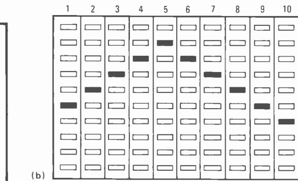
**2. Display.** Comparators, NAND gates, and transistors drive bar displays as each is strobed in succession (a). Amplitude of Y-axis signal determines which of 10 LEDs in each display is illuminated during sweep. Typical sine wave is displayed on 100-dot matrix (b).
