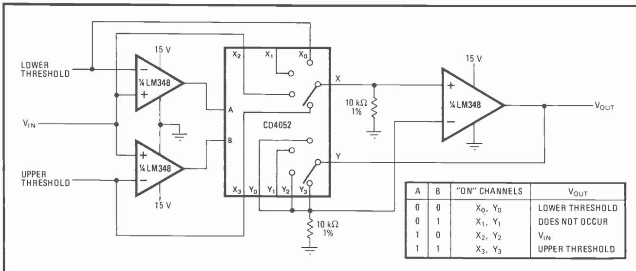
**Dual-threshold clamper** State of comparators driving analog multiplexer ports A and B determines which of three inputs appears at V. Circuit response is linear between threshold limits. Truth table describes circuit function.
