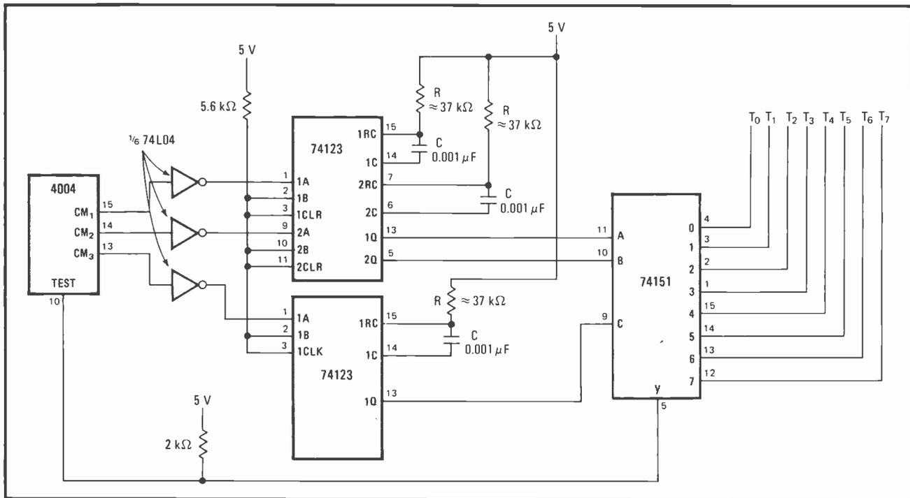
**Expanded test capacity.** Multiplexed test lines increase usefulness of 4-bit 4004 microprocessor. Selection of test lines  $T_0$ – $T_7$  is accomplished by software. One-shots are retriggerable, transform processor's pulse output to true logic signal for selecting multiplexer lines.
