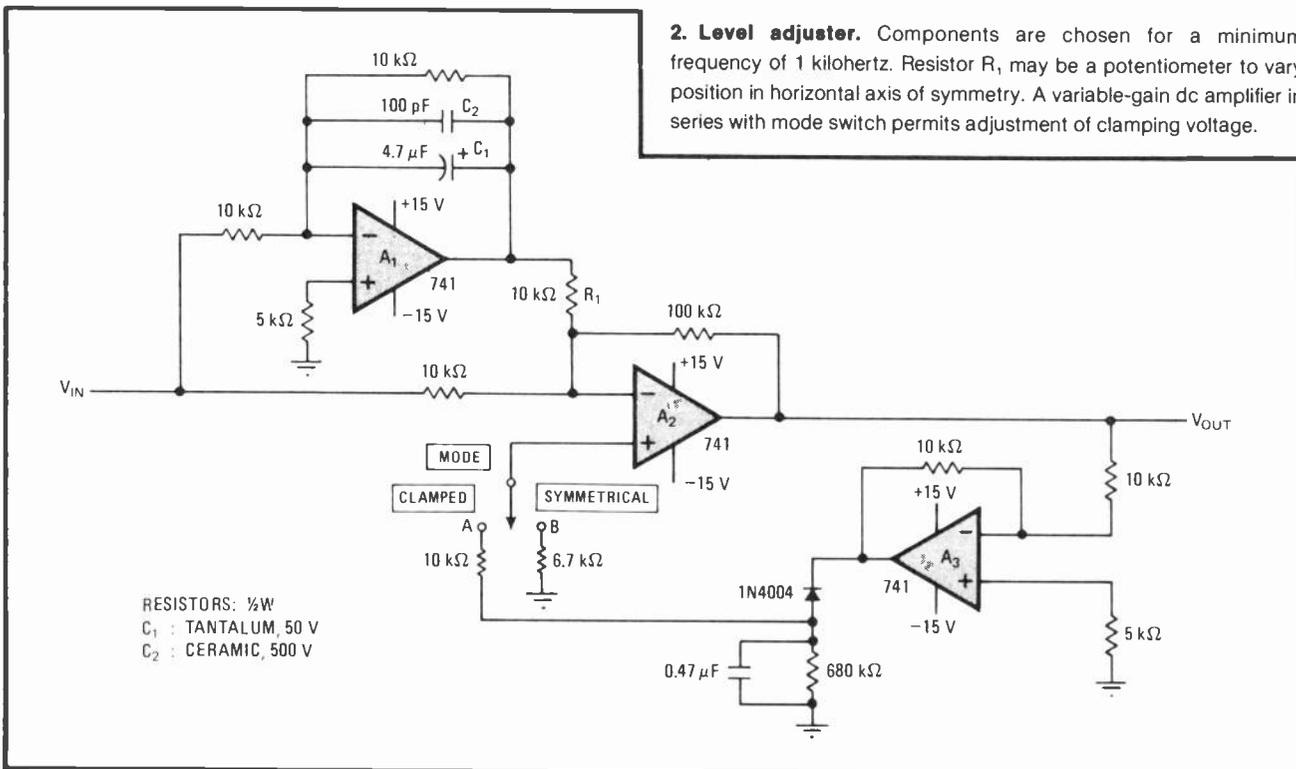
$A_3$  is symmetrical about 0. The polarity of the output voltage depends on the orientation of the diode—for the direction shown, it is positive-going.
