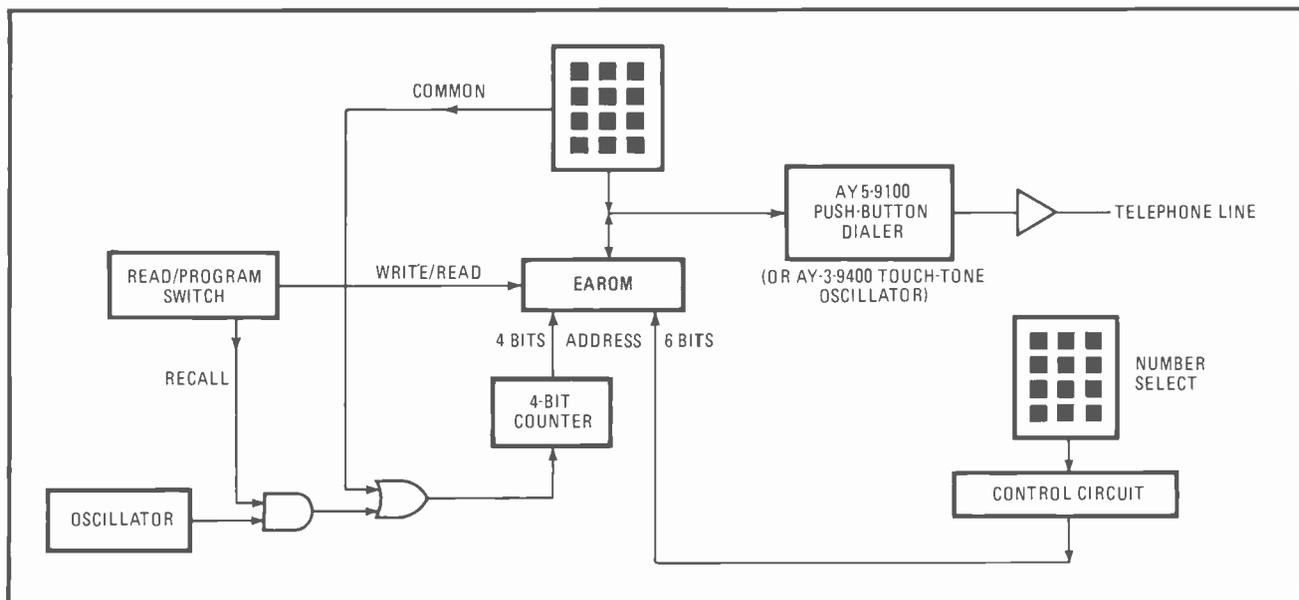
**9. Dialing.** An electrically alterable ROM in a repertory dialing system stores telephone numbers, which are then automatically supplied to the dialing mechanism when requested by the user. This 4,096-bit memory provides enough data to handle 64 16-digit numbers.
