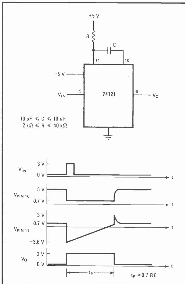
**1. Standard configuration.** TTL circuits alone cannot control the duty cycle of a one-shot directly because negative voltage is generated at timing port during normal operation. Reduction of this voltage to low level permits adjustment of pulse width.
