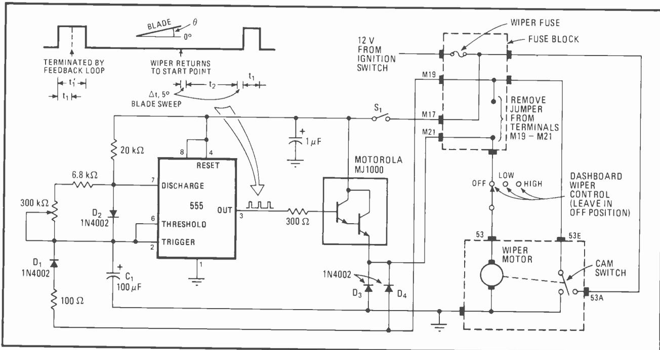
**1. Wipe-rate selection.** Control over the time between sweeps in negative-ground windshield wiper systems is done by the 555 and a synchronous feedback loop. Delay time can be varied from 0 to 22 seconds. Synchronizing the feedback to the wiper blades' position ensures that sweep rate will be independent of variations in wiper speed. Terminal block notations are for Volkswagen Rabbit.
