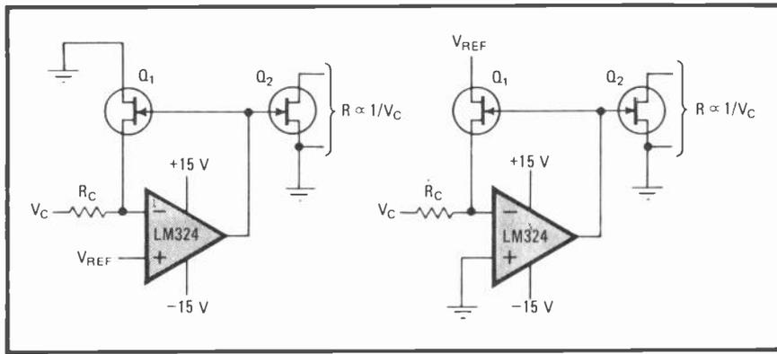
**1. Voltage-controlled resistance.** Unused half of FET  $Q_2$  can function as voltage-controlled resistor in external circuits.  $R_{ds}$  is inversely proportional to control voltage in both circuits.  $V_c$  values are negative for n-channel FETs, positive for p-channel FETs.
