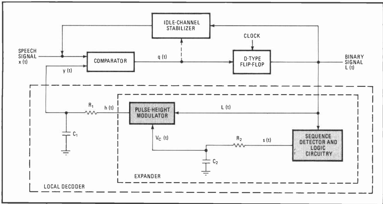
**7. Improving s/n ratio.** A continuously variable slope delta (CVSD) encoder may be viewed as a collection of linear delta modulator encoders having different, but fixed, step sizes that between them provide a near peak signal-to-noise ratio over a wide dynamic range.
