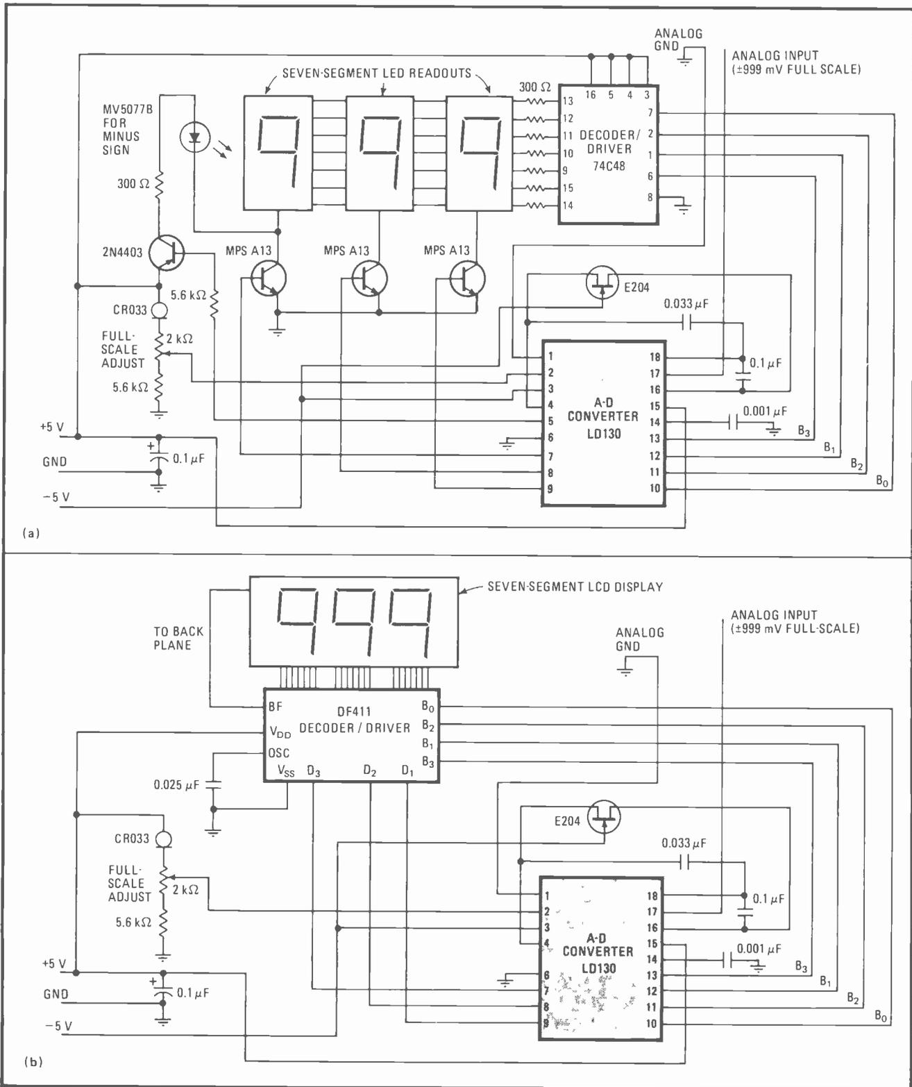
**3. Choice of display.** With the appropriate decoder/driver, the single-chip LD130 quantized-feedback converter can interface with either a light-emitting-diode display (a) or a liquid-crystal display (b) to form a three-digit panel meter capable of measuring to  $\pm 999$  mV.
