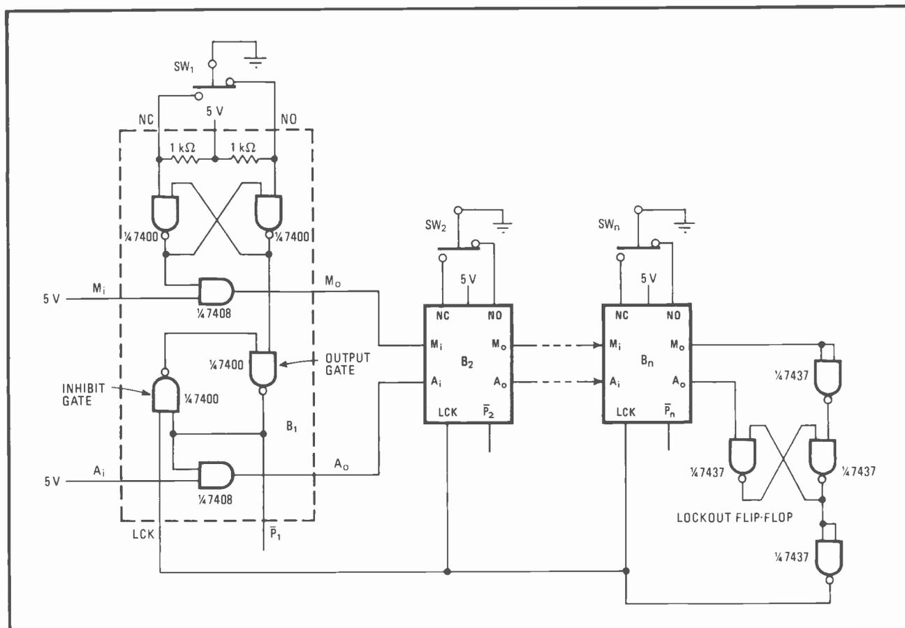
**Priority encoding.** First switch to close captures its output buffer. Circuit disables all other buffer output lines by generating a lockout (LCK) signal. Release of switch or switches automatically resets circuit. The truth table of the switch array is illustrated.
