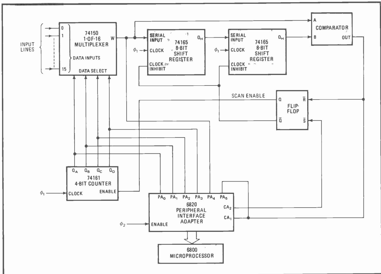
**Smart controller.** Sixteen lines are multiplexed to microprocessor, which performs input update only when notified of a state change on any line. The 6820 peripheral interface adapter is programmed to generate interrupt on negative transition of CA<sub>1</sub>, which in turn generates negative-going CA<sub>2</sub> to advance counter by one. For eight input lines, an eight-input multiplexer and just one shift register would be used.
