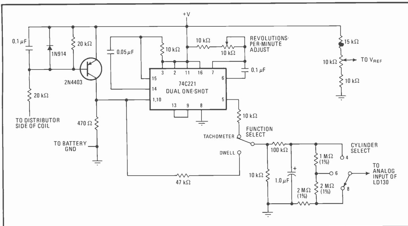
**4. Build it.** Hooking up this circuit up to the LD130 converter enables the device to measure engine revolutions per minute or the dwell time between point closures, depending on the position of the function switch. The circuit operates from a single positive supply.
