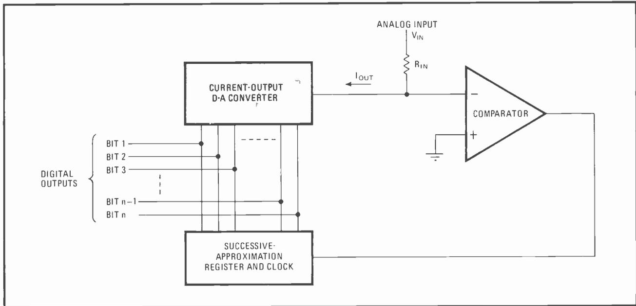
**3. A-d converter.** All of the relationships that apply to the drift errors in a d-a converter also hold for a successive-approximation a-d converter, since this component includes a current-output d-a converter as one of its circuit blocks, as shown here.
