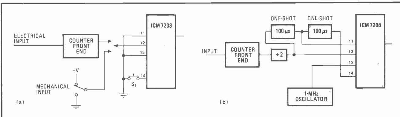
**2. Easily adaptable.** A slight modification to the input circuit makes it absolutely versatile. The circuit can be configured to monitor the number of electrical or mechanical events (a) or as a period counter (b) for measuring input cycle duration or the time between events.
