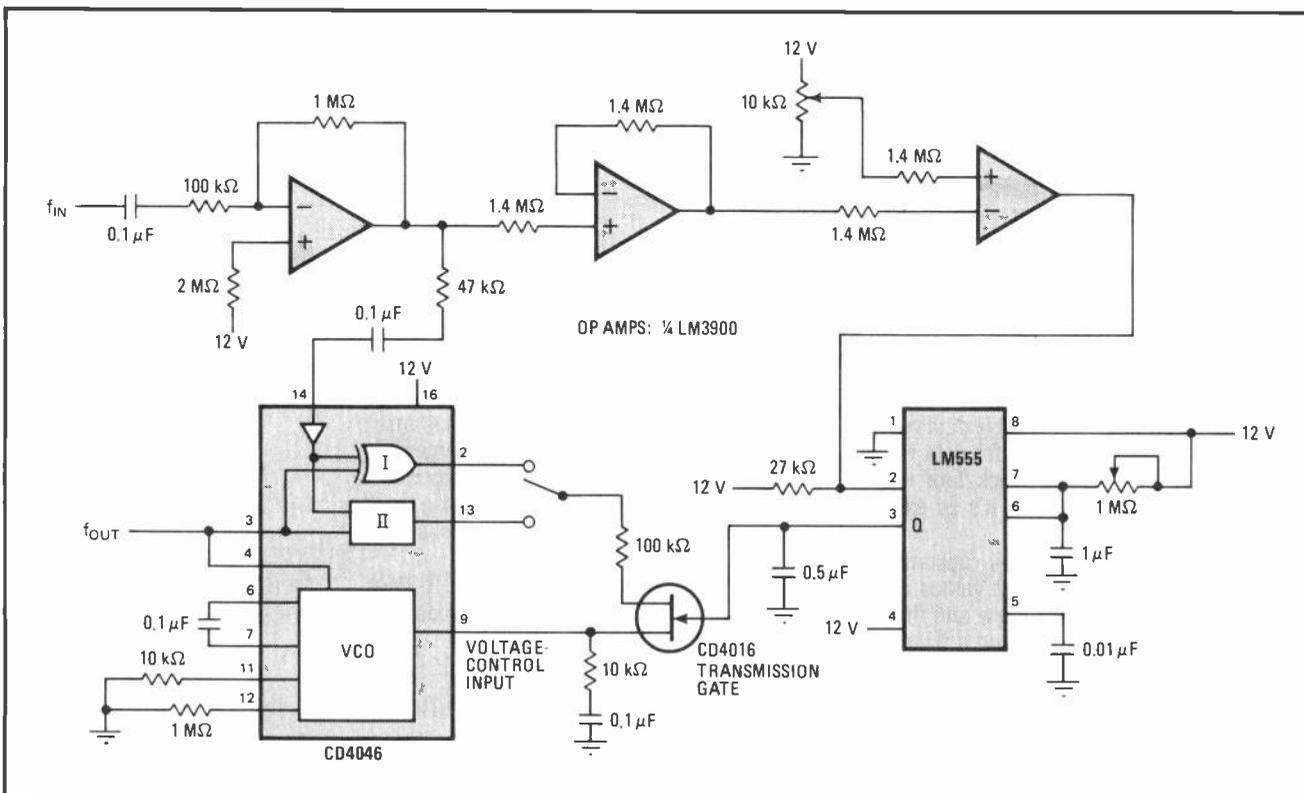
**Self-gated sample-and-hold.** Input-signal burst closes feedback loop in PLL, locks it to incoming frequency. Removal of input opens loop but causes no change in VCO frequency because of RC network, which stores unchanging voltage to drive oscillator.
