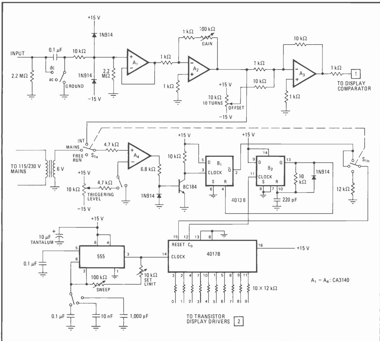
**1. Signal, timing, and logic.** Driver circuits for scope's LED bar displays are straightforward. Input circuit can process ac or dc signals and has variable Y-axis gain control. A<sub>1</sub> - A<sub>3</sub> is input-signal path. A<sub>4</sub>, B<sub>1</sub>, and B<sub>2</sub> provide sync for 555 clock generator and 4017 counter, which strobes bar displays. Circuit has internal, free-run, or power-line triggering option. Maximum sweep rate with 555 is 10 kHz.
