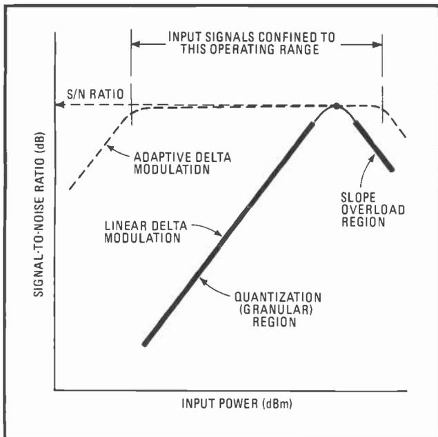
**4. Signals and noise.** The ratio is relatively constant in an adaptive delta modulation system, but in a linear delta modulation system it depends on signal level. At low input power, quantization noise predominates; a steeply sloping input produces slope overload noise.
