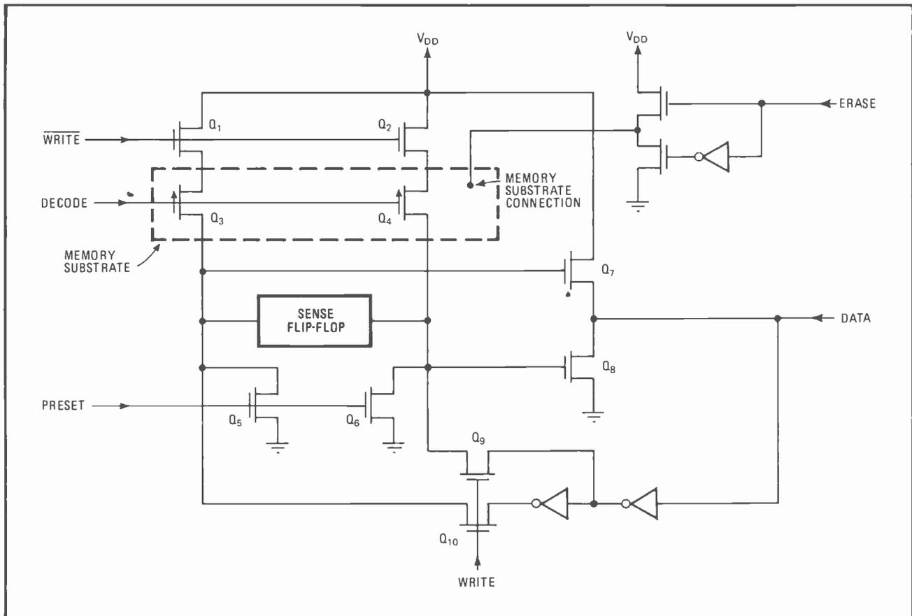
**4. Two transistors.** The flip-flop of this two-transistor cell detects whether an addressed memory location is in the low-threshold or in the high-threshold state over a range of voltages. The same circuitry also writes bits into the memory cell and erases them.
