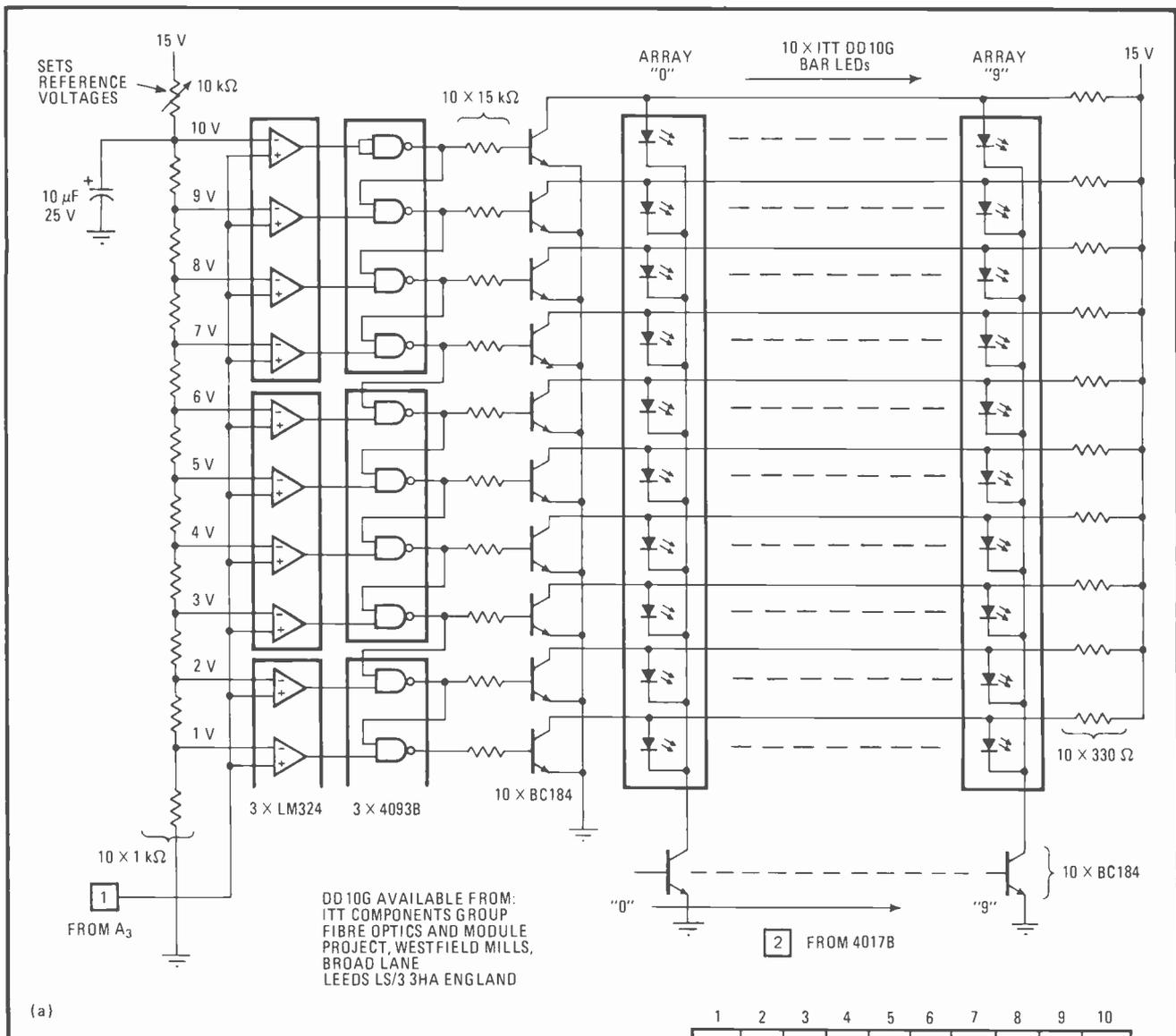
either. During any sweep, the 4017 Johnson counter steps at a rate controlled by the 555 timer and strobes each bar display in turn.  $A_4$ ,  $B_1$ , and  $B_2$  synchronize the counter's location to the sweep rate.
