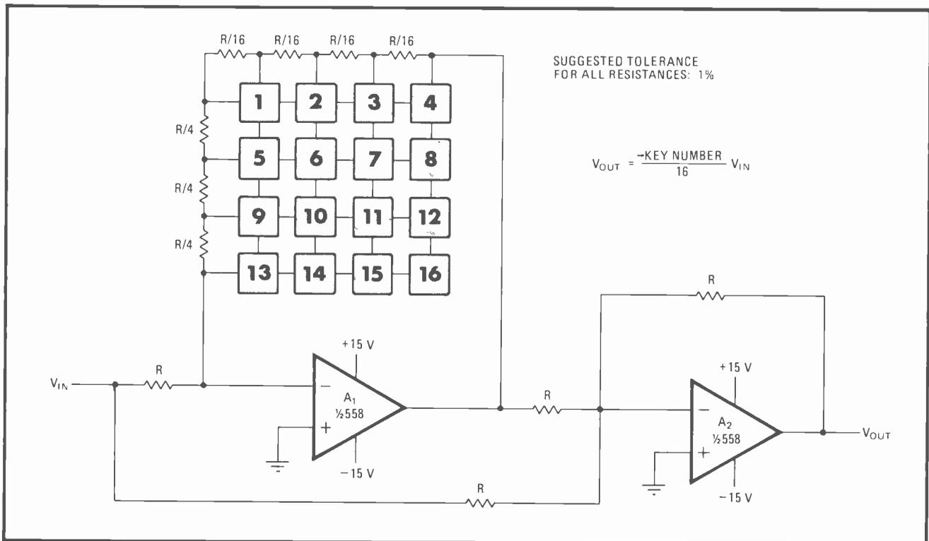
**Digital control** A standard keyboard and a few precision resistors in op amp's feedback circuit generate an output voltage proportional to the number on the key depressed. Circuit applications vary from component testing to analog-voltage control of computer systems.
