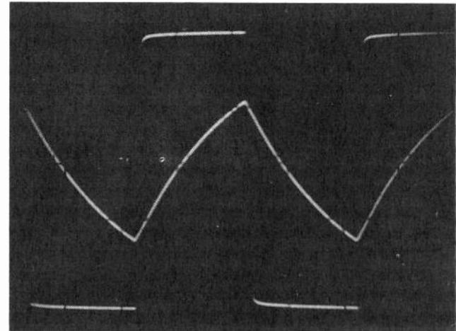
**2. Square-wave response.** Square-wave output is result of circuit's use of a short as well as a long time constant. If filter uses only long time constant, overfiltered triangular waveform results. Full square-wave output yields higher signal-to-noise ratio.
