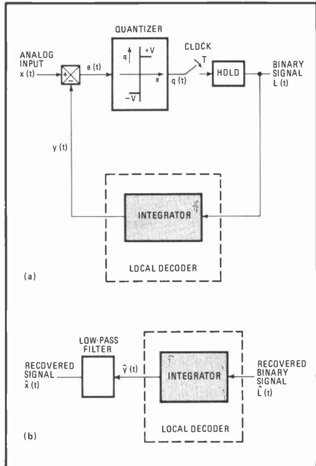
**2. Linear delta modulation system.** The encoder (shown at top) comprises a subtractor circuit, quantizer, sampling circuit, holding circuit, and local decoder, which is essentially an integrator. The decoder (bottom) needs only a local decoder and low-pass filter.
