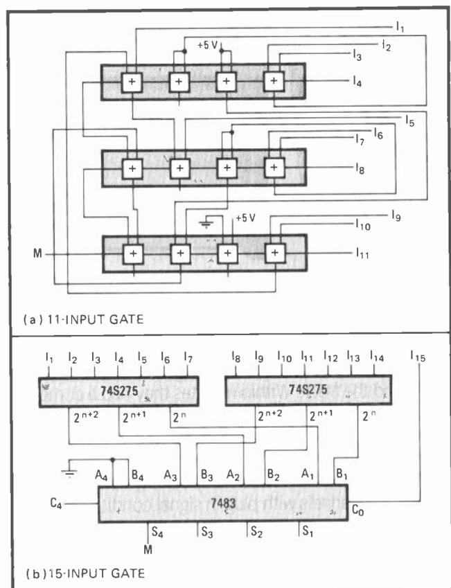
advantageous to search for devices with characteristics similar to the adder and use them to reduce wiring and design headaches—and, in many cases, to minimize chip count. In Fig. 2b, a 15-input gate is implemented using two 74S275 “Wallace trees” and a full adder; the 74S275 provides the function of four adders without the external wiring. When connected to the external adder, space and cost are minimized.
