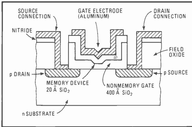
**3. What the three gates do.** This three-gate structure allows the MNOS memory designer the optimum tradeoff between storage-gate thickness and nonstorage-gate thickness. Here a 20-angstrom-thick silicon-dioxide layer in the center of the channel allows charge to tunnel from the memory's substrate to the oxide-nitride interface when a high enough voltage is applied to the gate.
