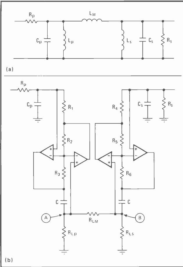
**4. Bandpass filter.** Double-tuned bandpass filter of (a) may be built with two gyrators, as in (b). Sharing resistor  $R_{LM}$ , the grounded gyrators simulate the pi network of inductors in the passive version. All of the amplifiers may be general-purpose devices.
