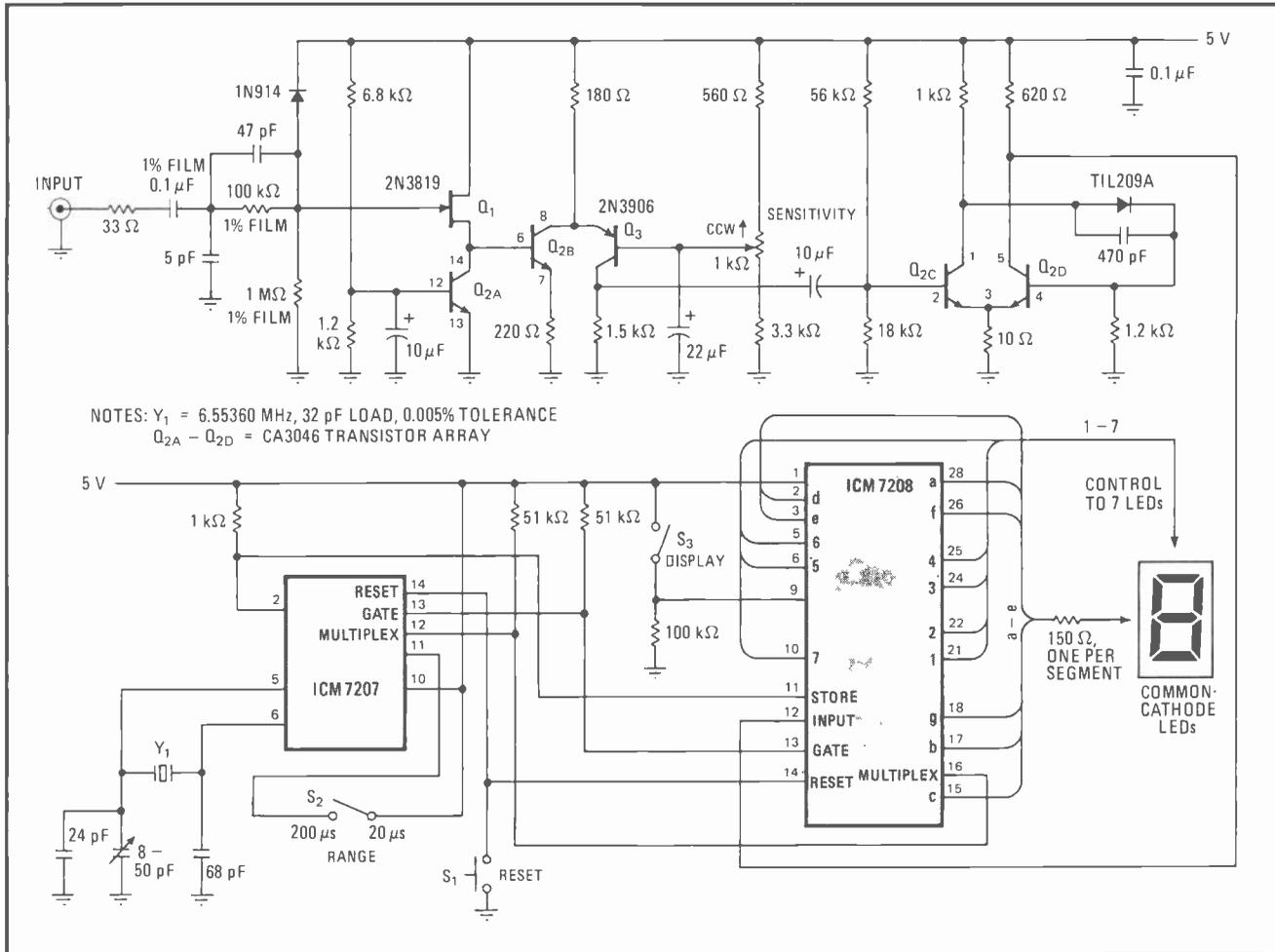
**1. Frequency counter.** A well-designed front end and two LSI circuits permit realization of a high-performance, low-cost frequency counter. The counter's frequency response is 5 MHz, but can be expanded to 30 MHz. Total cost is \$50, half that of competitive units.
