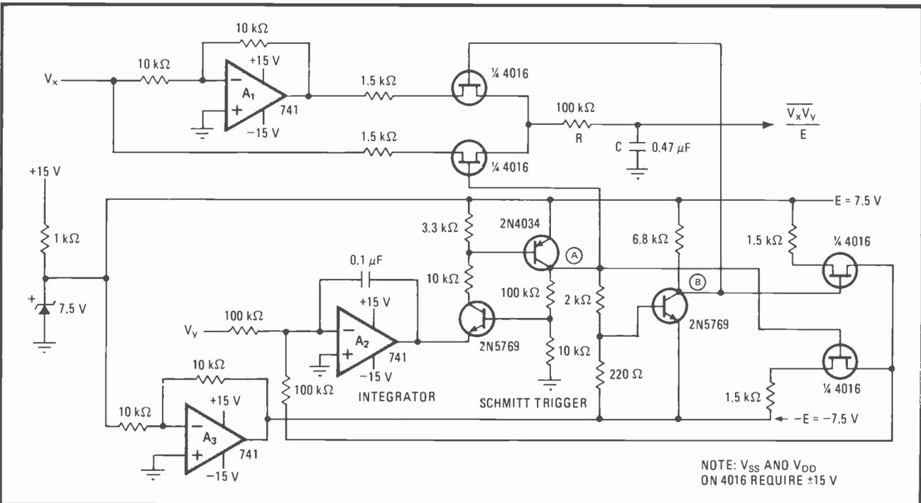
**2. Multiplier.** Building the circuit from the block diagram shown in Fig. 1 is straightforward.  $A_1$  is inverting, unity-gain amplifier.  $A_2$  serves as integrator. Three transistors form standard Schmitt trigger. Four transmission gates provide a practical switching circuit arrangement for  $\pm E$ ,  $\pm V_x$ . Inverting operational amplifier  $A_3$  ensures that  $+E$  is equal in magnitude to  $-E$ .
