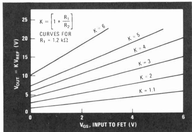
**2. Characteristic equation.** Relationship of scale factor  $K$  to  $V_{out}$ .  $V_{GS}$  is linear as shown by curves. Scale factor is controlled by resistor feedback network at regulator output. FET, used as voltage-controlled resistor, assures output voltage is proportional to  $K$ .
