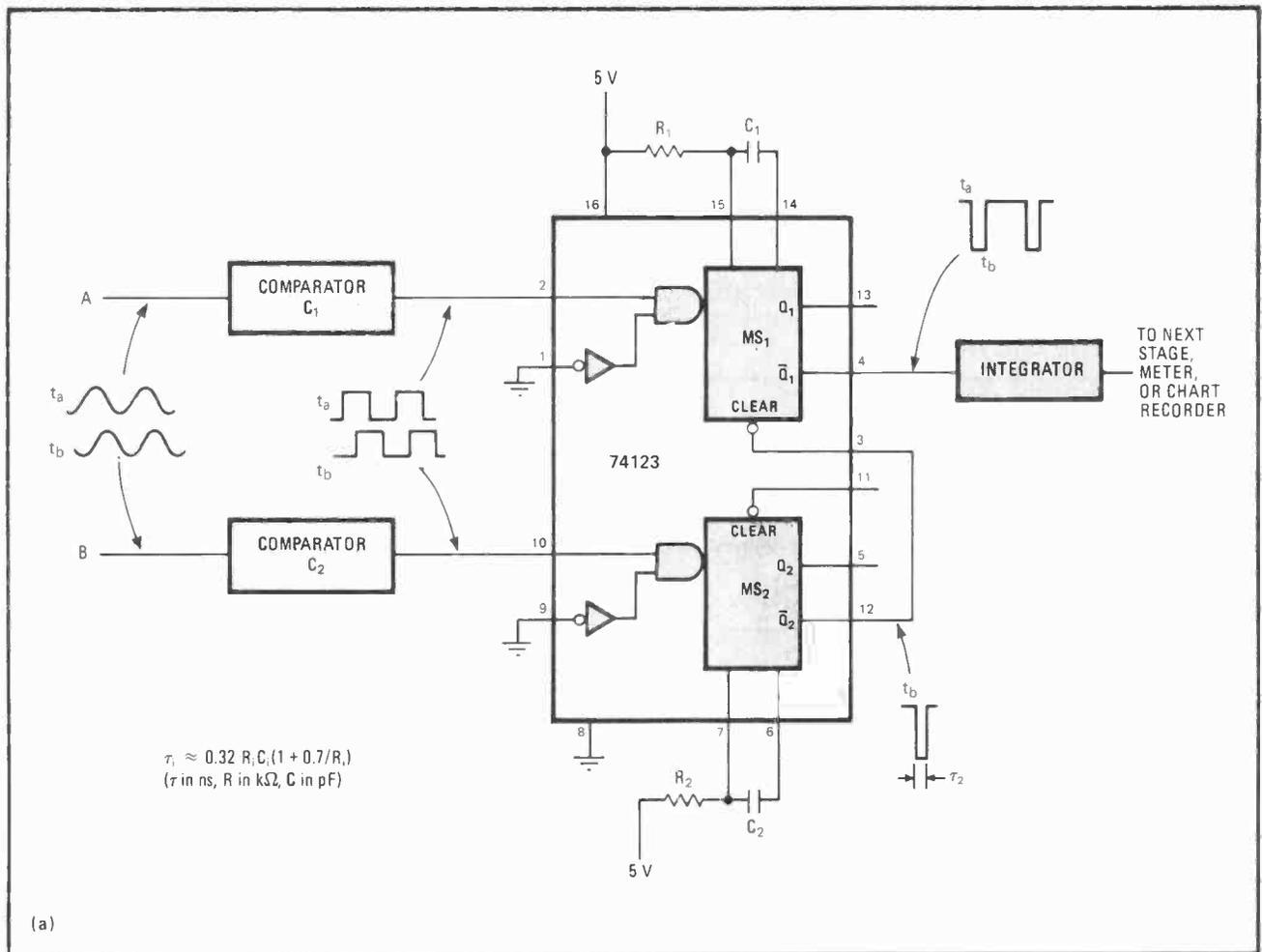
**360° phase detector.** Dual one-shot and integrator yield unambiguous voltage and slope output combination for changing phase-lead or phase-lag angles (a). Output from integrator increases when B leads A, decreases when A leads B(b).
