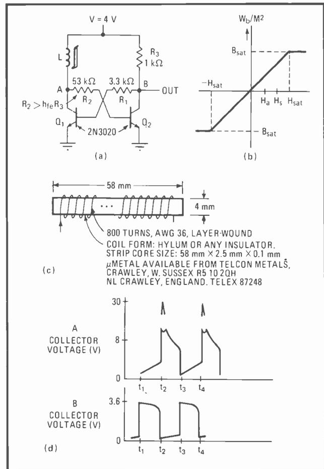
**Field sensitive.** Saturable core reactor enables oscillator to detect change in any magnetic field whose flux lines cut reactor windings (a). Oscillator frequency is determined by the core saturation time (b). Inductor is made of  $\mu$  metal, insulated core form, and 800 turns of high-gauge wire (c). Timing diagram details operation (d).
