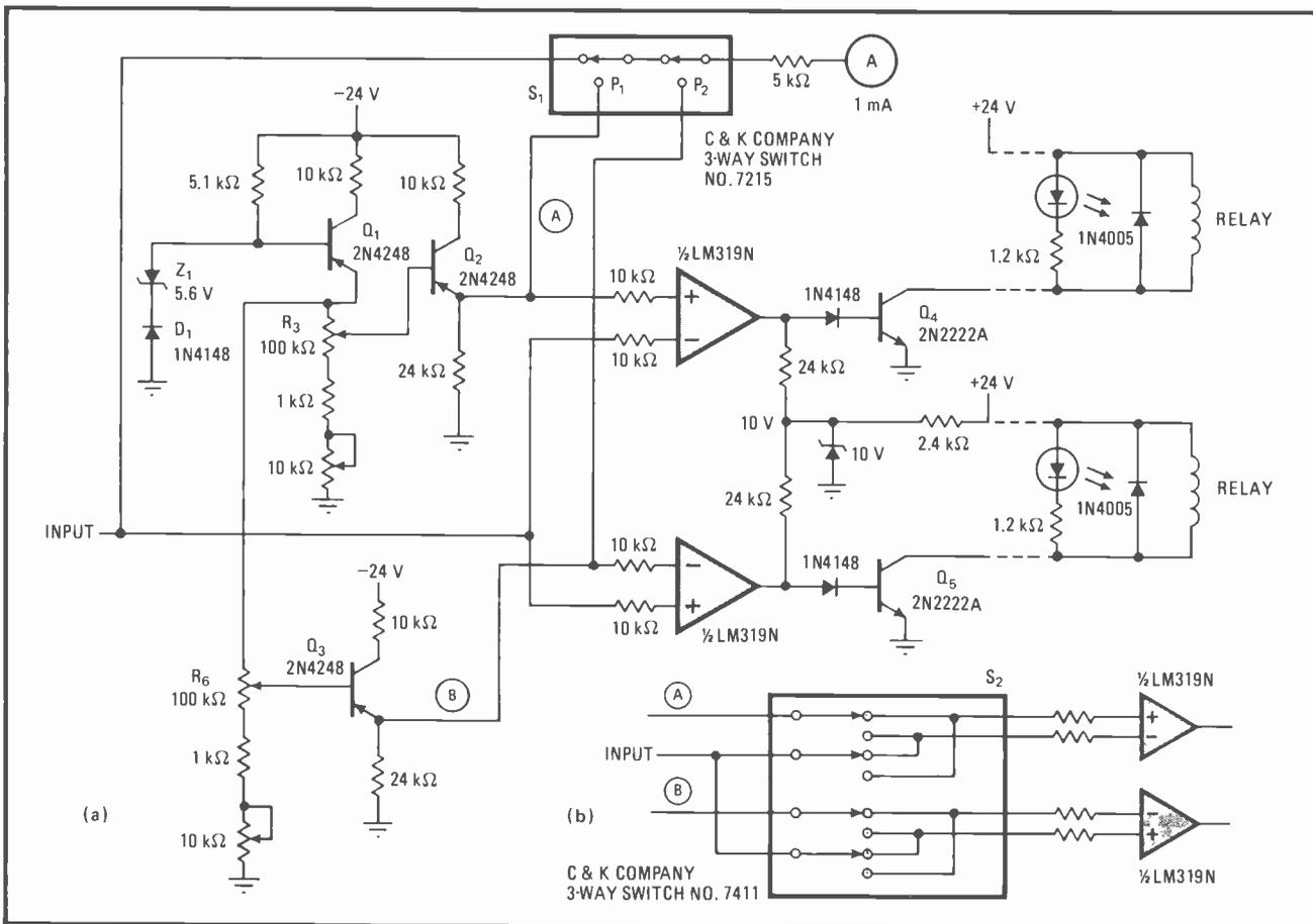
**Mechanical to electrical conversion.** Implementation of dual-set-point meter using standard meter and comparator circuits (a) is low-cost and reliable. When a three-way switch is added to circuit (b), double high and low set points can be set.
