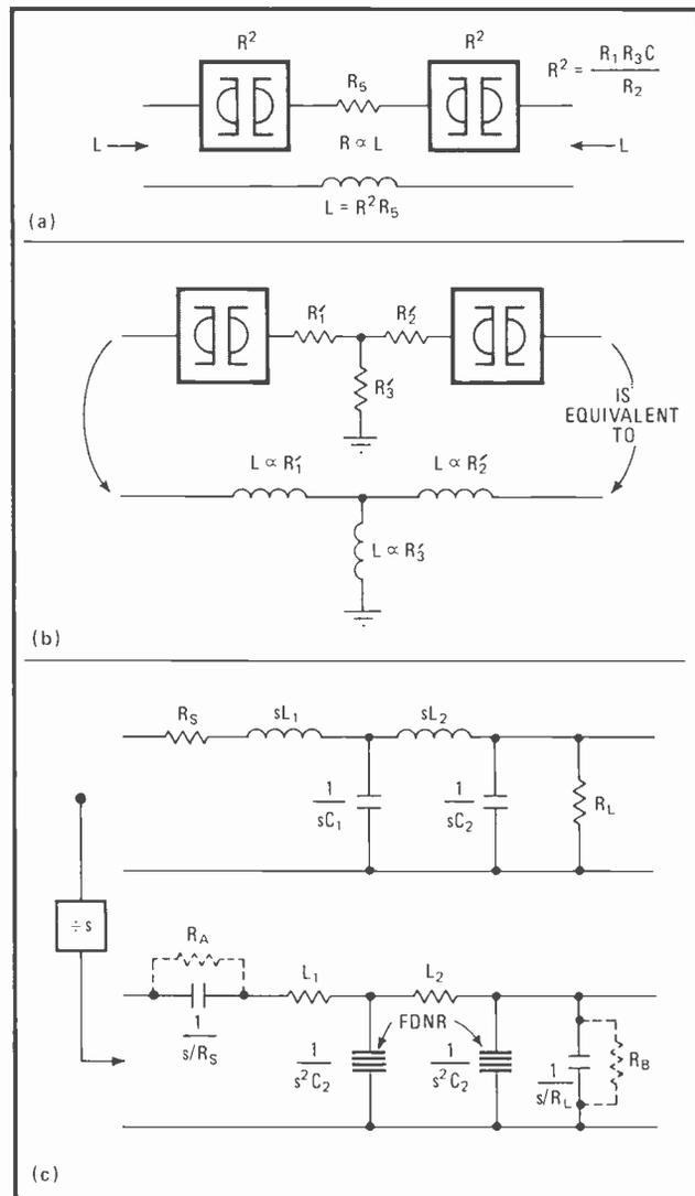
**3. Floating.** Lower terminal of basic gyrator (Fig. 2b) is grounded. To float the circuit, two gyrators may share the same resistor (a), or a network of resistors (b). Floating inductors may also be simulated (c) with functionally dependent negative resistors (FDNRs).
