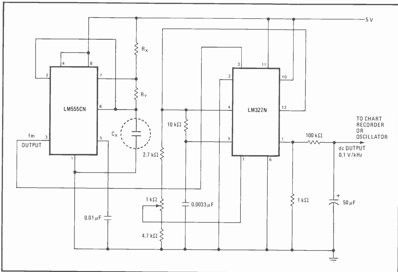
**Transducer-to-recorder interface.** Two timers determine transducer capacitance, perform capacitance-to-voltage conversion for chart recorder, while isolating transducer from output-circuit loading. Transducer placed in timing network of 555 astable multivibrator determines its frequency. LM322 one-shot, which should have a much shorter period than the multivibrator, transforms frequency into voltage
