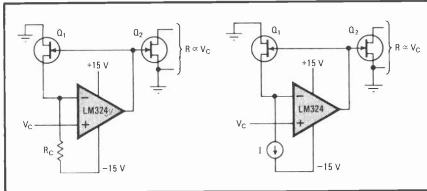
**2. Direct proportional control.**  $R_{ds}$  varies linearly with  $V_c$  in both circuits. If  $V_c$  exceeds  $V_{ref}$  or breakdown voltages of FET in either figure, a resistor should be inserted between output of operational amplifier and gate of FET to prevent burnout.
