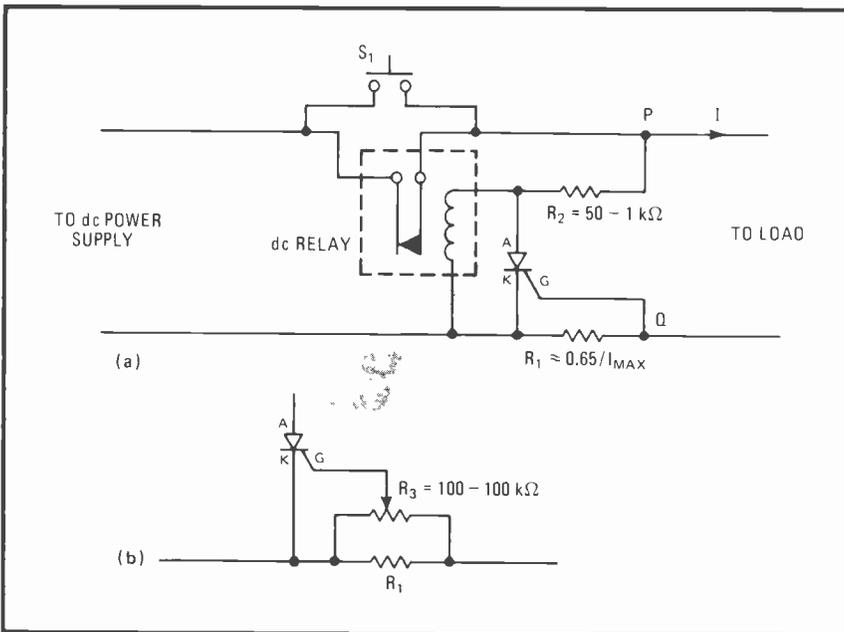
voltage across points PQ will be equal to the nominal supply voltage, and the normal operating voltage will appear across the relay winding. The relay and resistor  $R_2$  are selected according to the dc supply voltage used and the relay's rated coil voltage, respectively.
