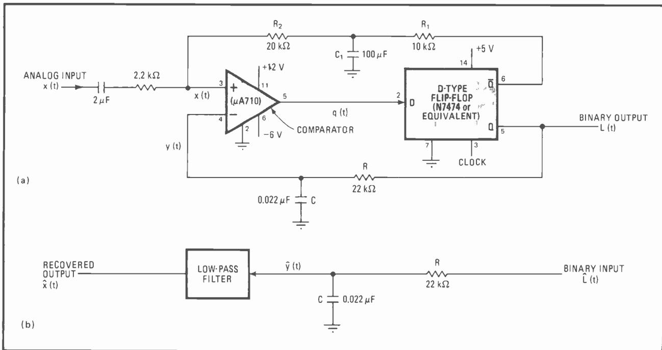
**5. Linear delta modulation.** A comparator, D-type flip-flop, and a resistor-capacitor integrator are all that is needed for a low-speed linear delta modulation encoder. The delta modulation decoder requires only a simple RC integrator and a low-pass filter.
