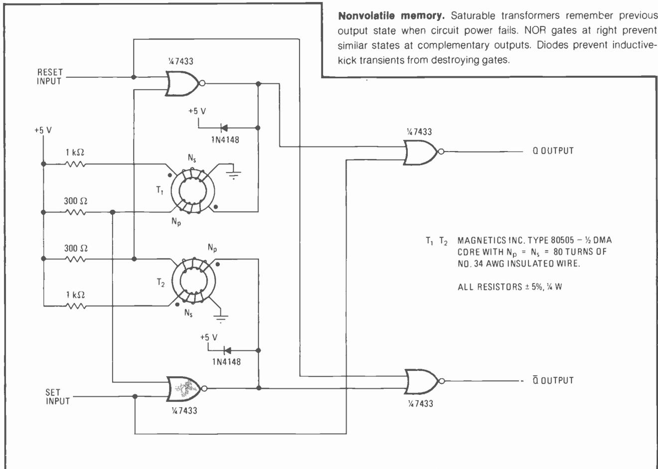
65  $\mu$ s. Should power fail during operation, the power-supply fall time must be much less than 35  $\mu$ s; otherwise, the latch may lose its contents. The same rise-time constraints accompany power-up.
