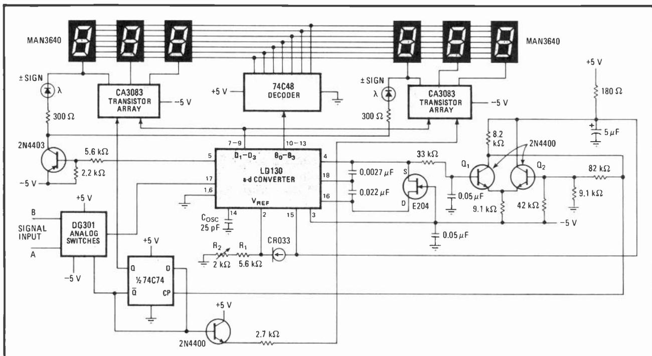
**Two voltmeters in one.** If the input signals can be sampled at rates of 60 times per second or greater, they can be measured, then observed simultaneously at acceptable flicker rates. Key to circuit operation is use of fast-sampling analog-to-digital converter.
