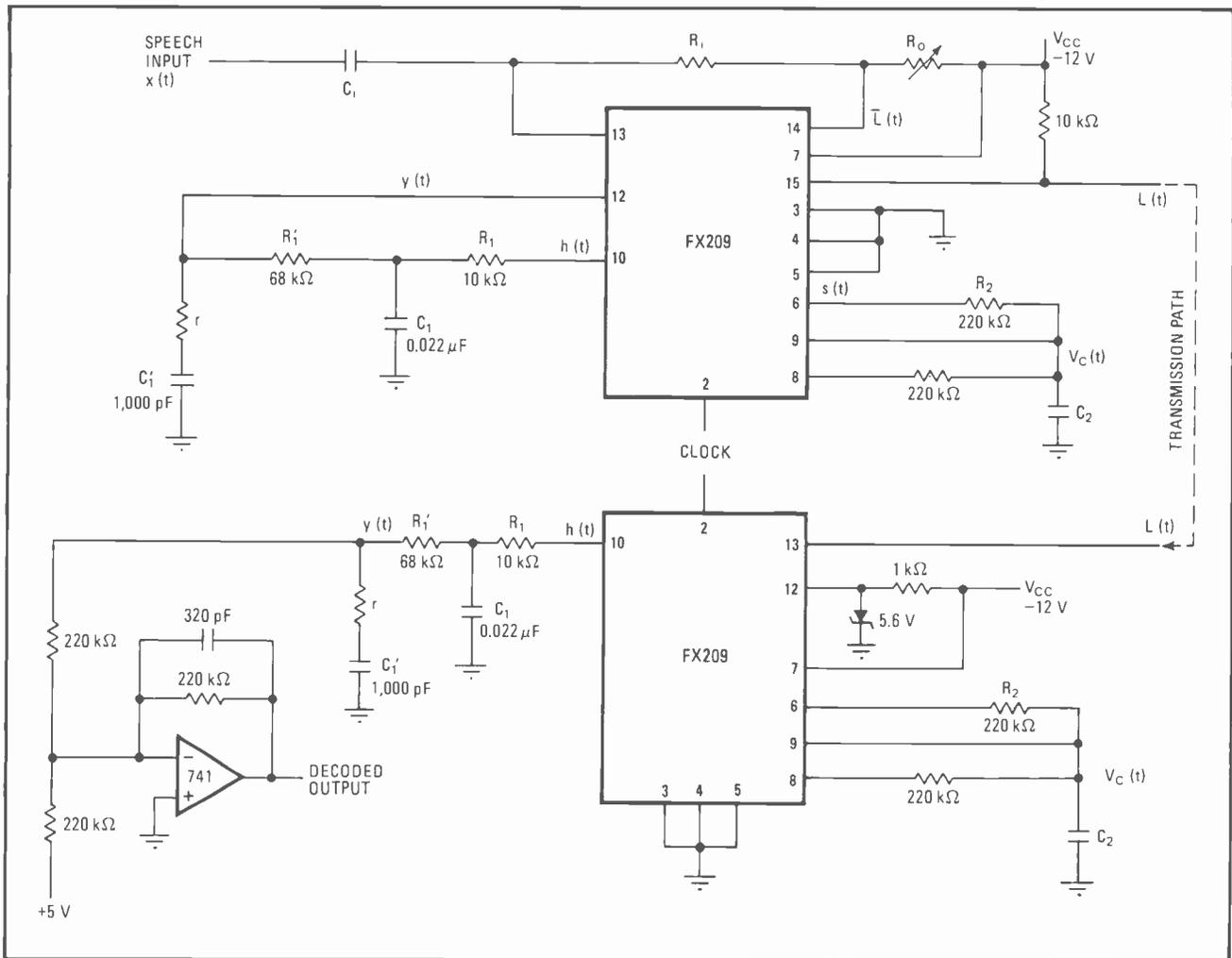
**8. Building block.** Putting together a CVSD encoder and decoder requires two integrated circuits, such as Consumer Microcircuits of America's FX209 delta modulator, along with several resistors and capacitors to provide the selected transmitted bit rate.
