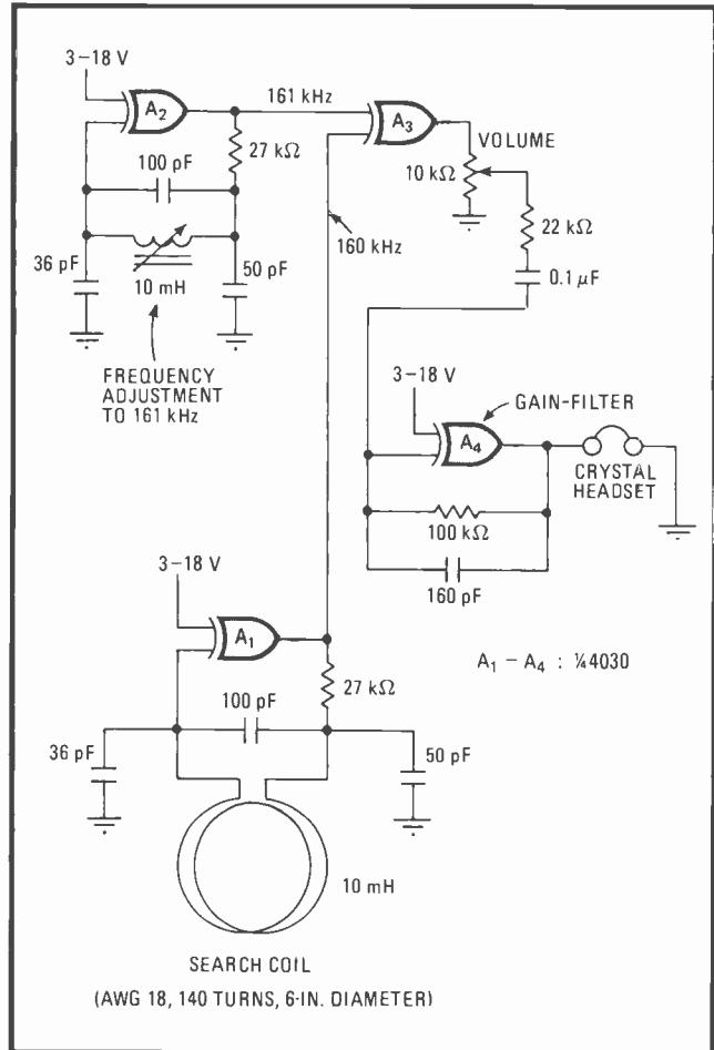
**Metal detector.** Two oscillators and a search coil form a simple metal detector. Objects near search coil change  $A_1$ 's frequency of oscillation and the 1-kHz output note produced by the mixing of oscillators  $A_1$  and  $A_2$ .  $A_4$  amplifies and filters audio signal.
