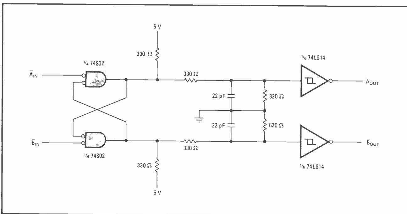
**First come, first served.** The input signal arriving first passes to an output, while simultaneously arriving signals produce an eventual output but no glitch. The resistor network raises the threshold of the Schmitt trigger, and the RC combination reduces glitch amplitude.
