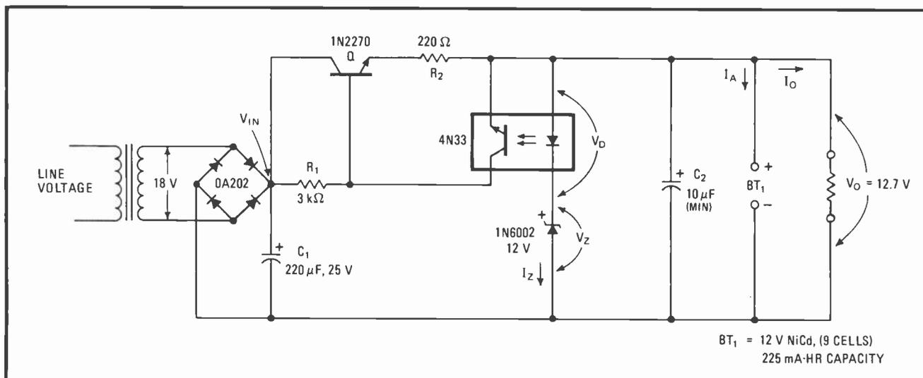
**Regulator or charger?** Circuit works as low-capacity battery charger or as voltage regulator when battery is removed. Use of optocoupler eliminates complex voltage-sensing networks. Output voltage and load current can be selected by suitable choice of  $R_1$ ,  $R_2$ , and zener diode.
