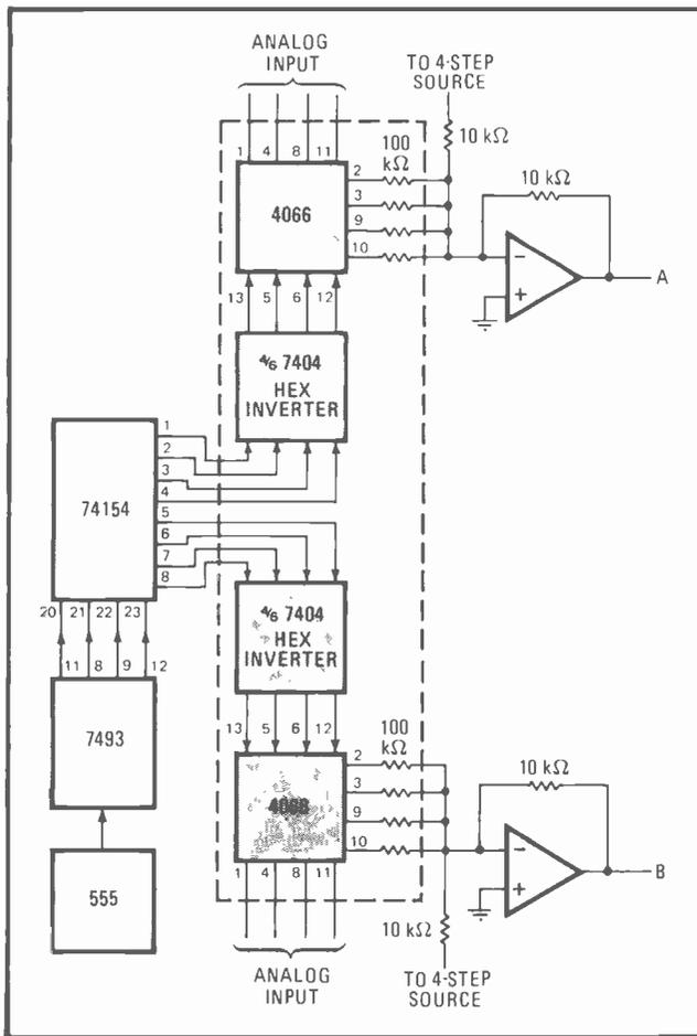
**3. Analog application.** Replacement of 74151 multiplexers by transmission gates permits observation of eight analog signals, as shown. Logic generator continues to function in same capacity, driving 4066 analog switches with digital gating signals.
