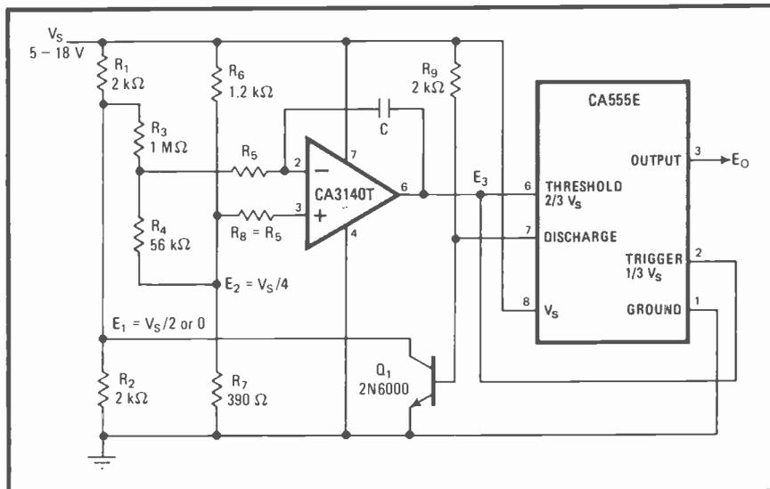
**Time-magnification.** Oscillation frequency of a 555 may be lowered 20 times or more if a low-input-current, integrating op amp is used to replace timing components. One oscillation every few days is possible if a high-value capacitor,  $C$ , is used in integrator.
