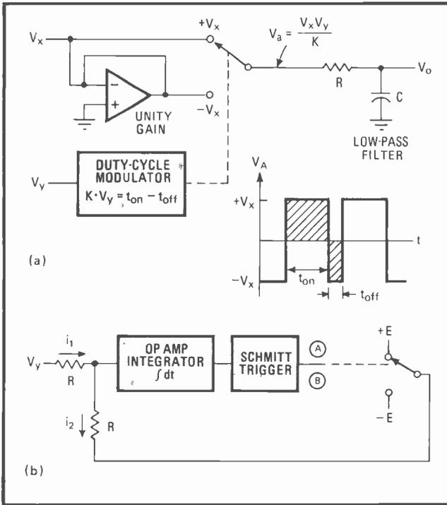
**1. Very linear.** Switching multiplier (a) is more accurate for finding product of two signals at low frequencies than IC transconductance multipliers. Duty-cycle modulator may be built with op-amp integrator and Schmitt trigger (b). Voltages  $\pm E$  and integrator together form oscillator of which the duty cycle is controlled by amplitude of  $V_y$ .
