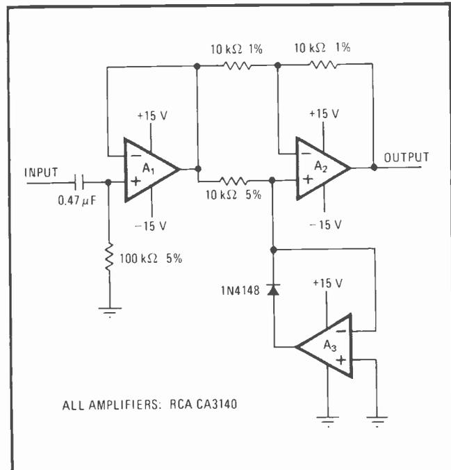
**Precision full-wave rectifier.** Op amp  $A_3$ , which ensures  $A_2$  follows positive voltages and inverts negative ones, has single-ended power supply to minimize slew time and maximize stability. Power-supply pins are decoupled with 0.47- $\mu$ F capacitors.
