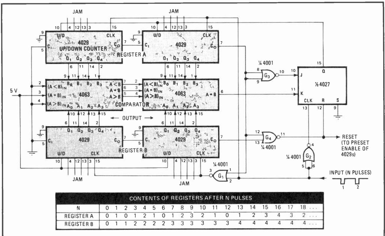
**N<sup>1/2</sup>.** Register B in the circuit yields the square root of N, rounded off to the nearest bit, where N is the number of input pulses received after the circuit has been reset to zero. Digital circuit eliminates shortcomings of detectors that measure analog voltages directly.
