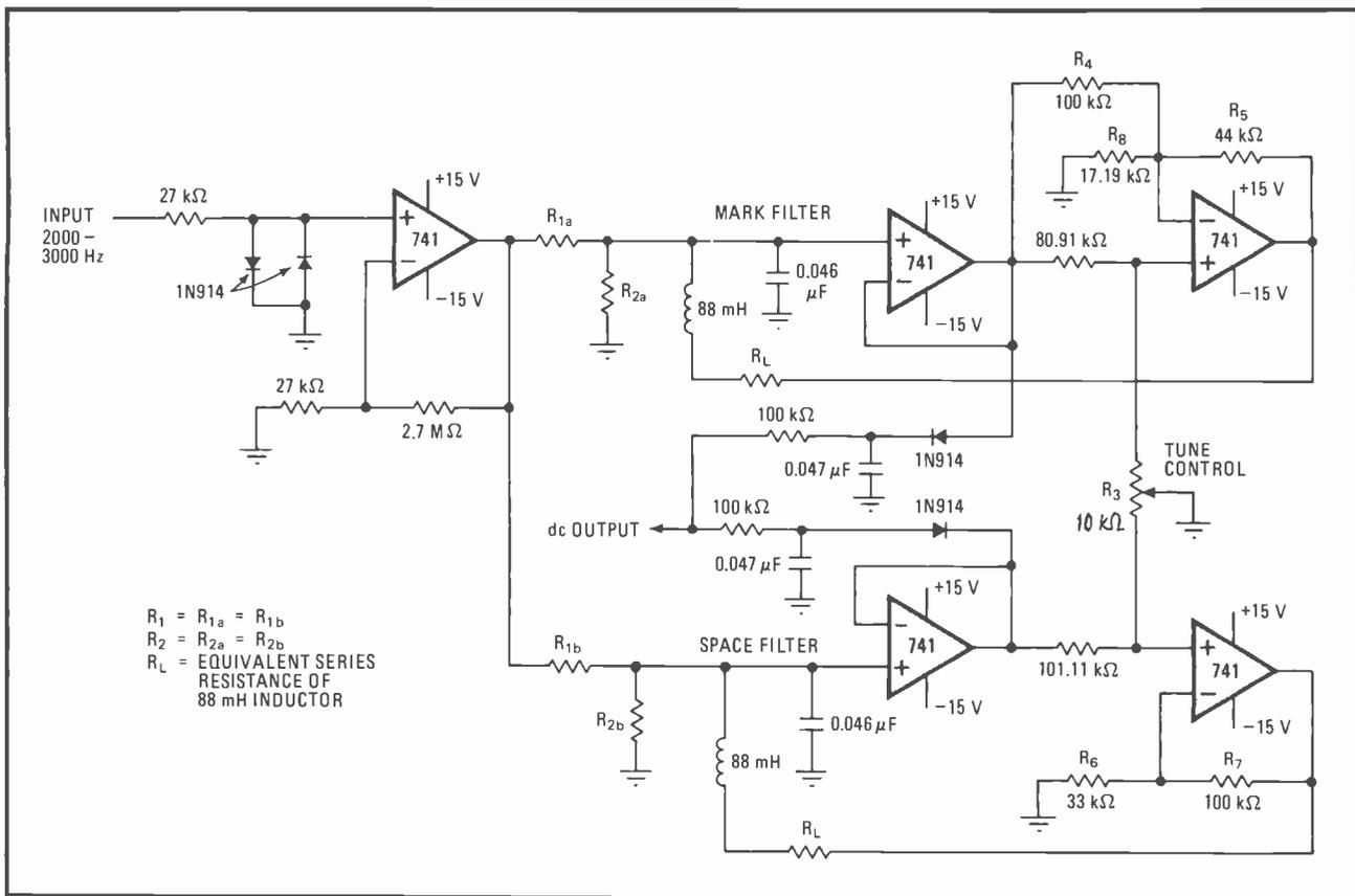
**2. A discriminating network.** Resistor-tuned filters provide one-control adjustment of mark-and-space frequencies. Shifts are continuously adjustable from zero to 1 kilohertz at a center frequency of 2,500 hertz and are linearly proportional to potentiometer setting.
