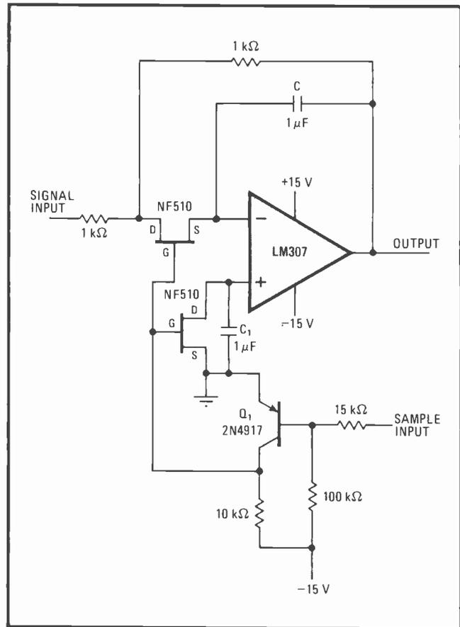
**Charge restorer.** Sample-and-hold response is improved if charge lost by hold capacitor  $C$  is replaced. Voltage change across capacitor due to op amp's inverting-port bias current is cancelled by compensating network. Droop rate, only 100 millivolts per 10-minute period, may be improved if capacitors  $C$  and  $C_1$  are matched.
