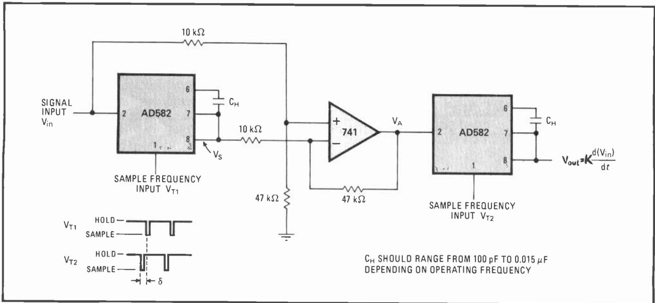
**2. Different differentiator.** Particularly useful at very-low-frequency signals, this differentiator uses a sample-and-hold and a difference amplifier to obtain the slope of the waveform. Second sample-and-hold recovers peaks of differentiated waveform. Negative pulse train (duty cycle approximately 1%) for sampling signals can be generated by a 555 timer circuit.
