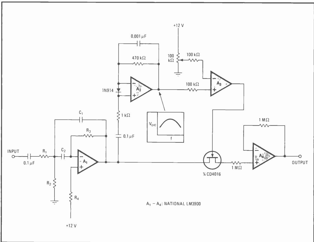
**Gated filter.** Circuit uses pass-band response of ordinary filter in generating voltage reference for gate switching. Transients caused by gate switching in the audio range are not detrimental to circuit performance but may cause concern at higher frequencies.
