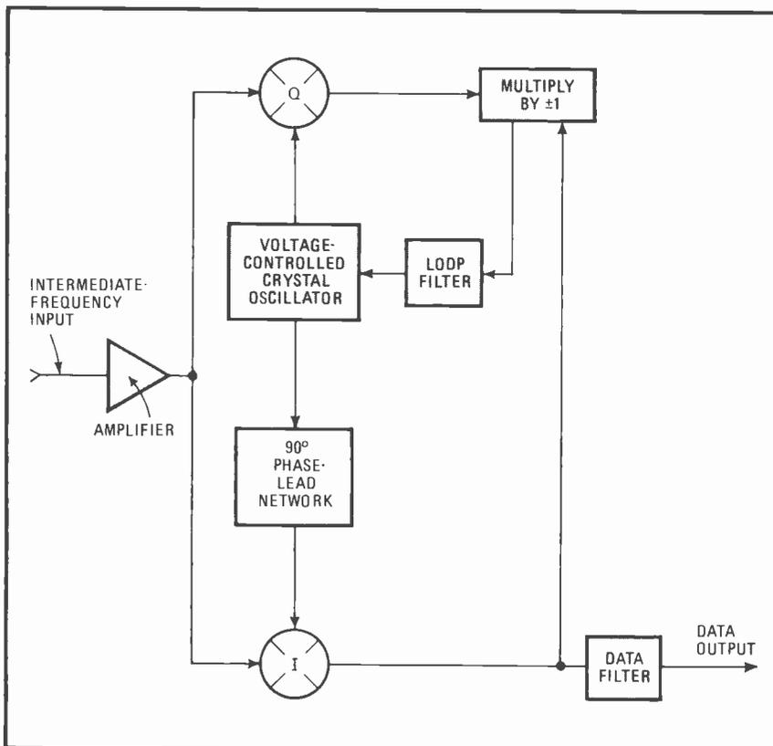
**The Costas loop.** An intermediate-frequency input signal is compared to the voltage-controlled crystal oscillator signal, and two quadrature signals are generated. The output from the Q (quadrature) channel is multiplied by  $\pm 1$  depending on phase detected by the I (in-phase) channel. The feedback loop facilitates tracking of the carrier frequency in high-noise environments and maintains locking despite phase reversals of the carrier caused by modulation.
