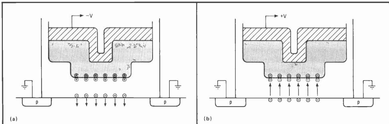
**2. Writing and erasing.** To write into an MNOS memory, a negative voltage is applied to the gate (a), repelling electrons from the nitride trap sites in the silicon-oxide-silicon-nitride interface and setting up a net positive charge. Conversely, erasure of data from the MNOS memory uses a positive voltage (b), which attracts electrons and results in a negative charge at the storage interface.
