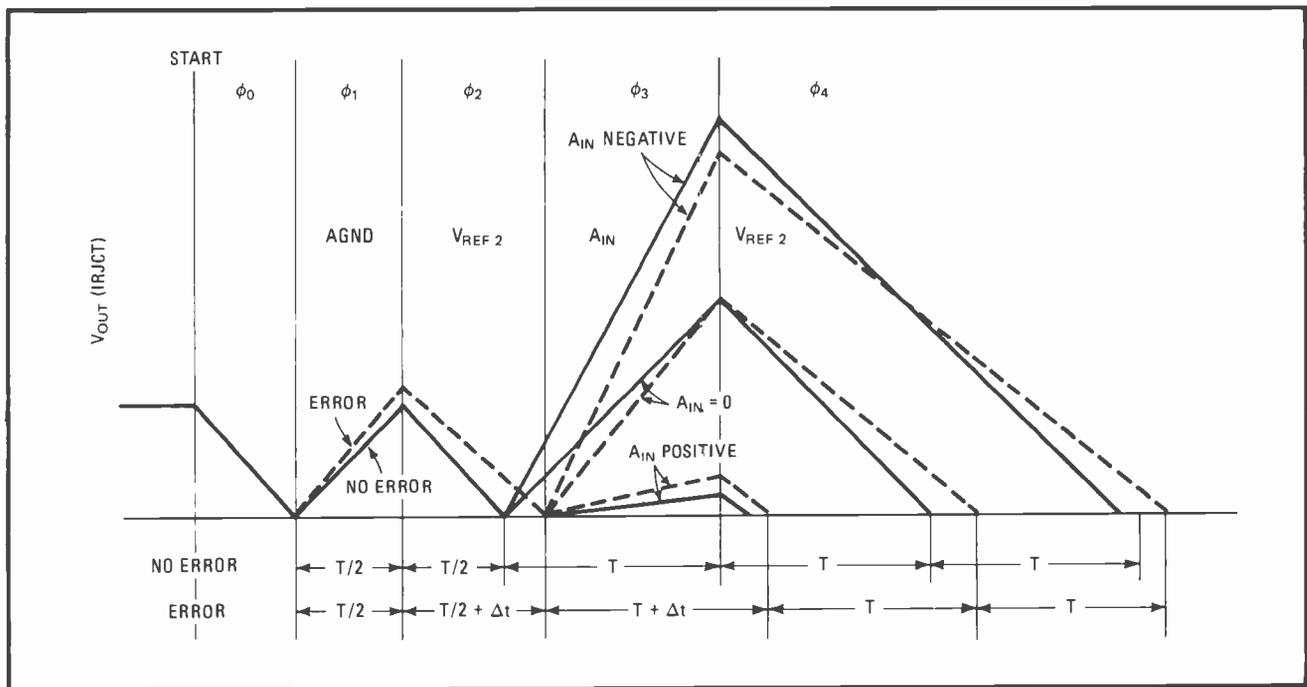
**2. Four-phase integration.** AD7550 uses quad-slope method to detect most errors, including op-amp offset voltage drifts. This method eliminates error by measuring comparator trip-time delay,  $\Delta t$ , converting  $\Delta t$  to a voltage and subtracting the voltage at end of cycle.
