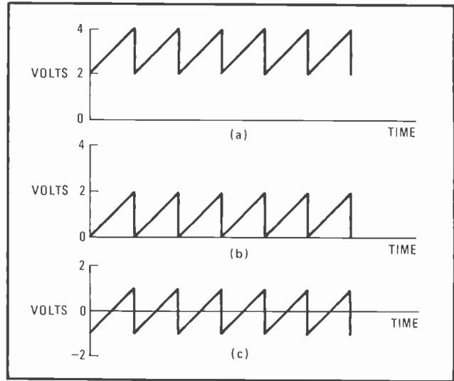
**1. Symmetry or clamping desired?** Input ramp at (a) is clamped to zero (b) or is symmetrical about zero (c). Circuit may be modified so that clamping to nearly any voltage level is possible.
