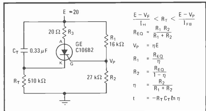
**Programmability.** An SCR oscillator retains the features of a unijunction-transistor circuit, including programmability of the firing point. Values shown yield an oscillation frequency of about 15 Hz. Gate-to-cathode voltage drop is neglected in the equations.
