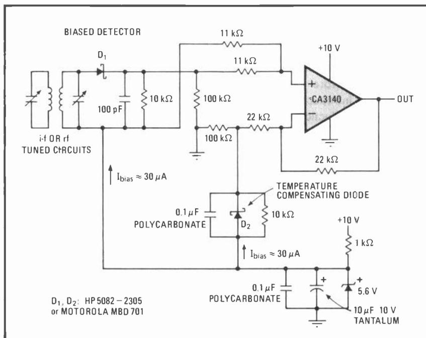
**Tweaked detector.** Even the old reliable a-m detector can be improved. Increased sensitivity, linearity, and dynamic range are obtained by dc biasing diode  $D_1$  into conduction, to eliminate voltage drop as seen by rf driver.  $D_2$  provides temperature compensation.
