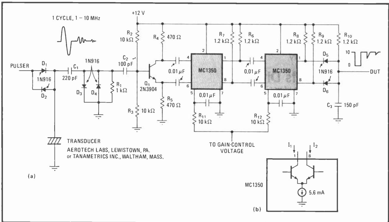
echo envelope is attained by recharging  $C_3$  through  $R_{10}$ . In some applications, it is desirable to provide a control to vary the fall time by adjusting  $C_3$  and to reject echoes of small amplitude by varying  $R_8$ ,  $R_9$ , and  $R_{10}$ .
