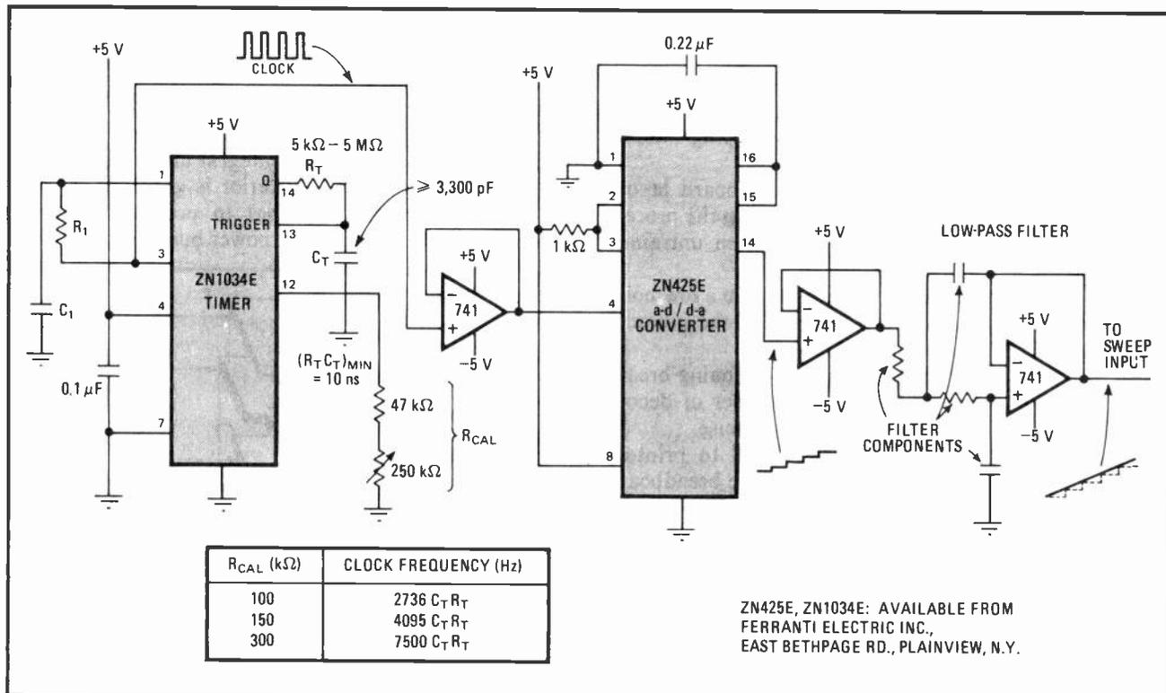
**Slow time base.** Low ramp frequency for X input of chart recorder, permitting long-period monitoring assignments of various systems, is generated by d-a converter and timer. Slope of ramp voltage with respect to time is determined by clock frequency.
