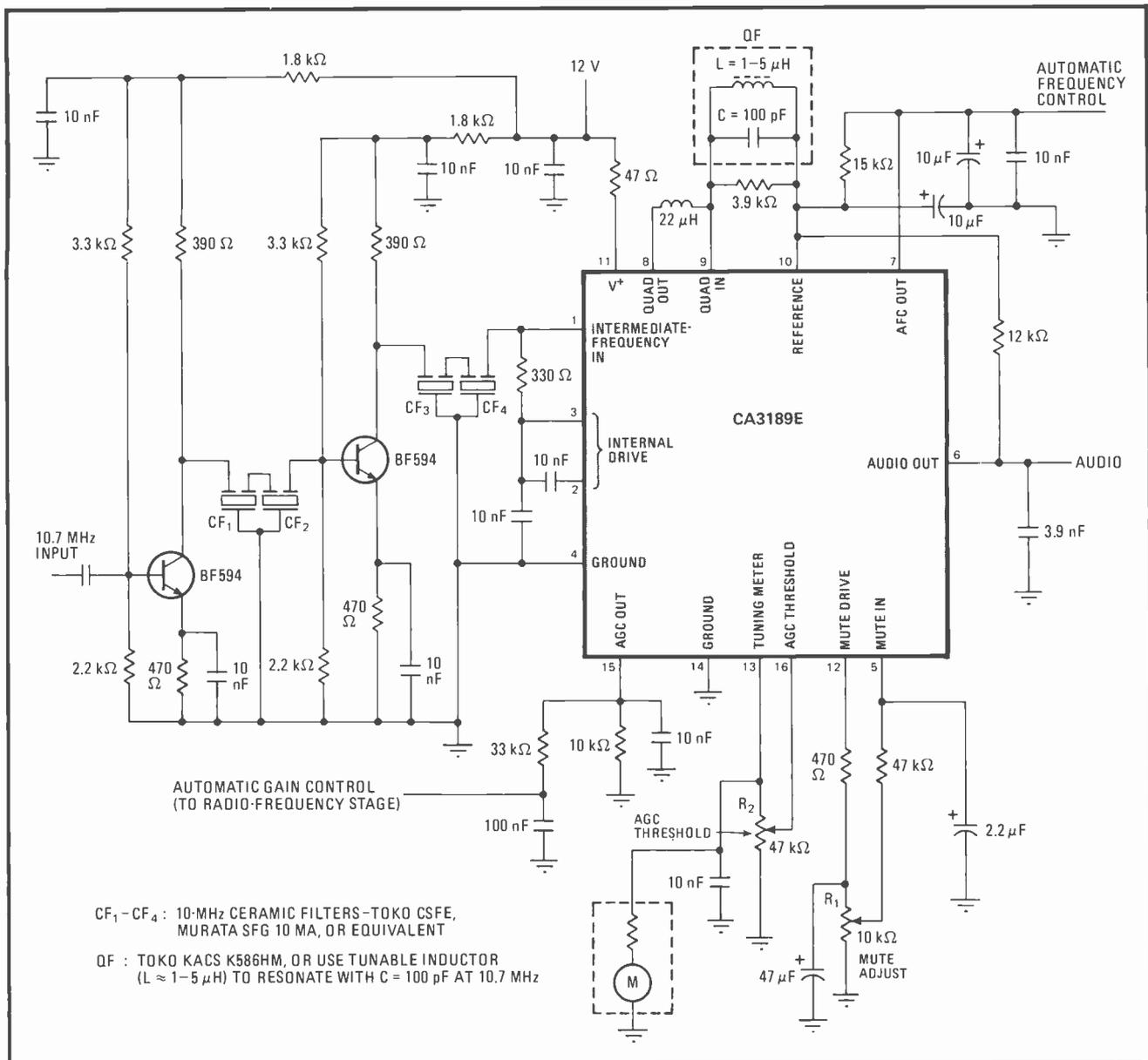
**1. Improved fm detector.** A good preamplifier and the CA3189 fm/i-f system provide optimum response. The circuit has greater noise immunity and better protection from a-m signal overload than detectors now used, and the agc threshold is selectable.
