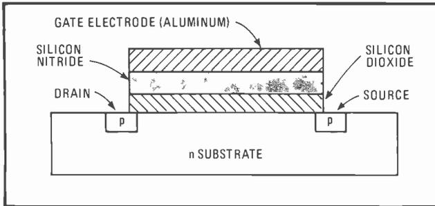
**1. The basic transistor.** To decrease their operating threshold, MOSFETs use a silicon-dioxide-silicon-nitride sandwich as their gate oxide. Without the dioxide, the nitride would store charge—a characteristic exploited in nonvolatile MOS memory design.
