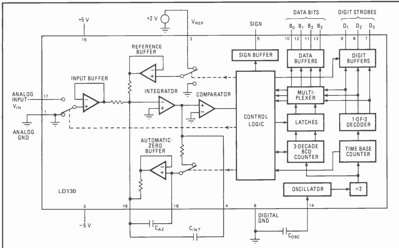
**2. Single chip.** Introduced last year, this complementary-MOS integrated circuit was the first single-chip quantized-feedback converter. Largely self-contained, the device requires only a voltage reference and three external capacitors, yet it delivers three digits of resolution.
