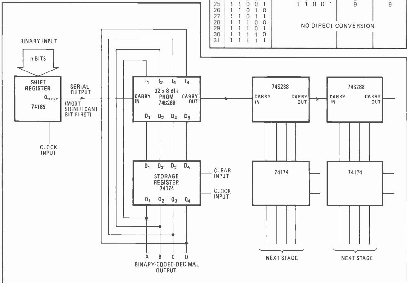
**BCD converter.** Storage register in feedback loop with programmable read-only memory allows continuous updating of the memory's contents. Multidigit conversion, if necessary, is relatively simple because cascade stages are connected by one lead only.
