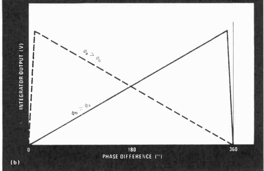
with respect to A. The output decreases when the phase angle of B decreases with respect to A. Thus the frequency relation of B to A may be determined from the slope of the integrator's output if the two signals are of similar but not identical frequency.
