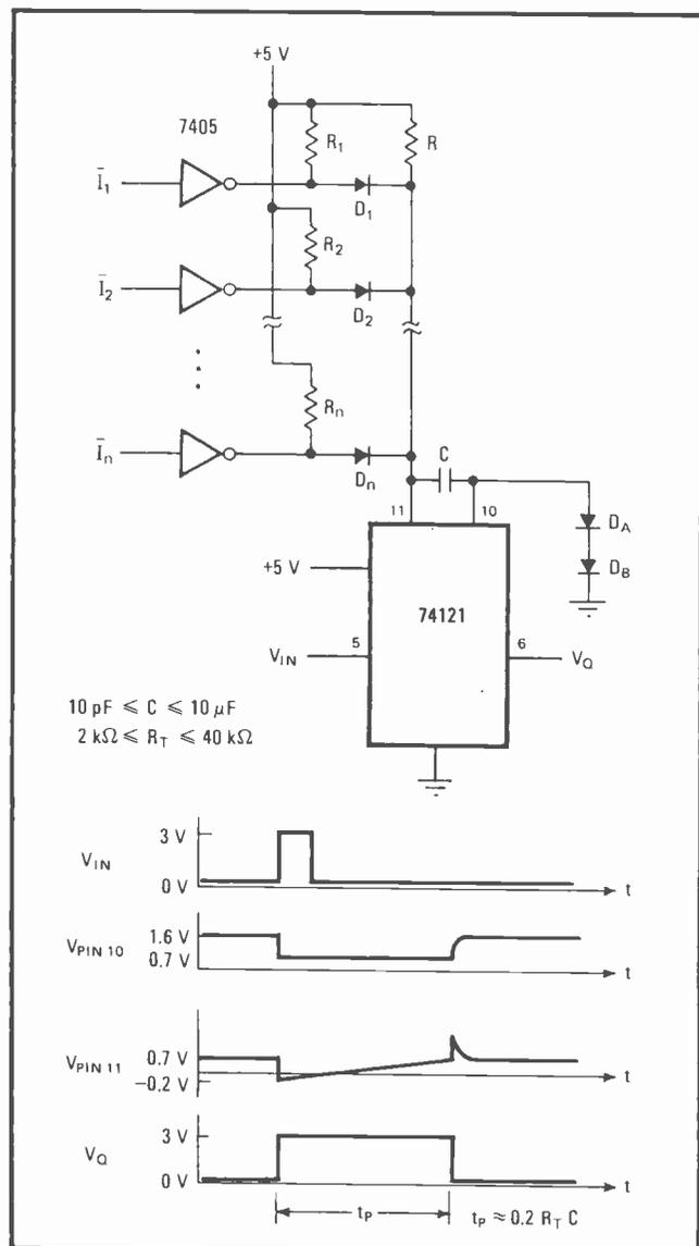
**2. Pulse width variation.** The use of diodes  $D_a$  and  $D_b$  clamps pin 10 of one-shot, permits TTL to drive and control the duty cycle. Actuating isolation diodes  $D_1$  to  $D_n$  alters the charging rate of C, providing a choice of duty-cycle times.
