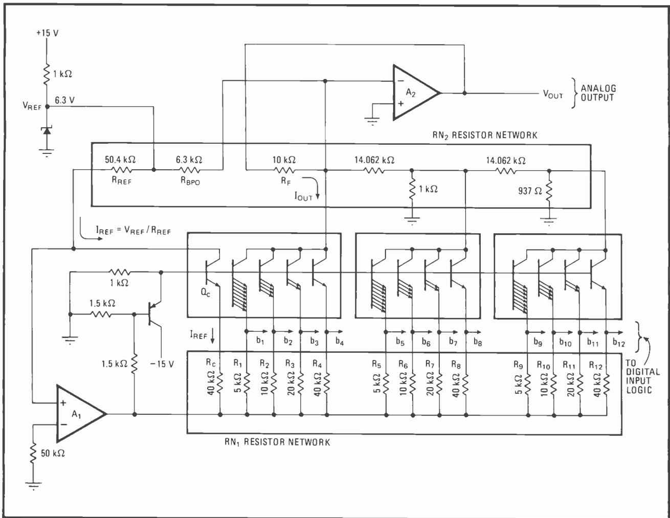
**2. Typical d-a circuit.** In general, the circuit design for a d-a converter largely compensates for tracking errors in the resistor networks and transistor current switches. By far the dominant error source is the drift of the zener diode that makes up the reference.
