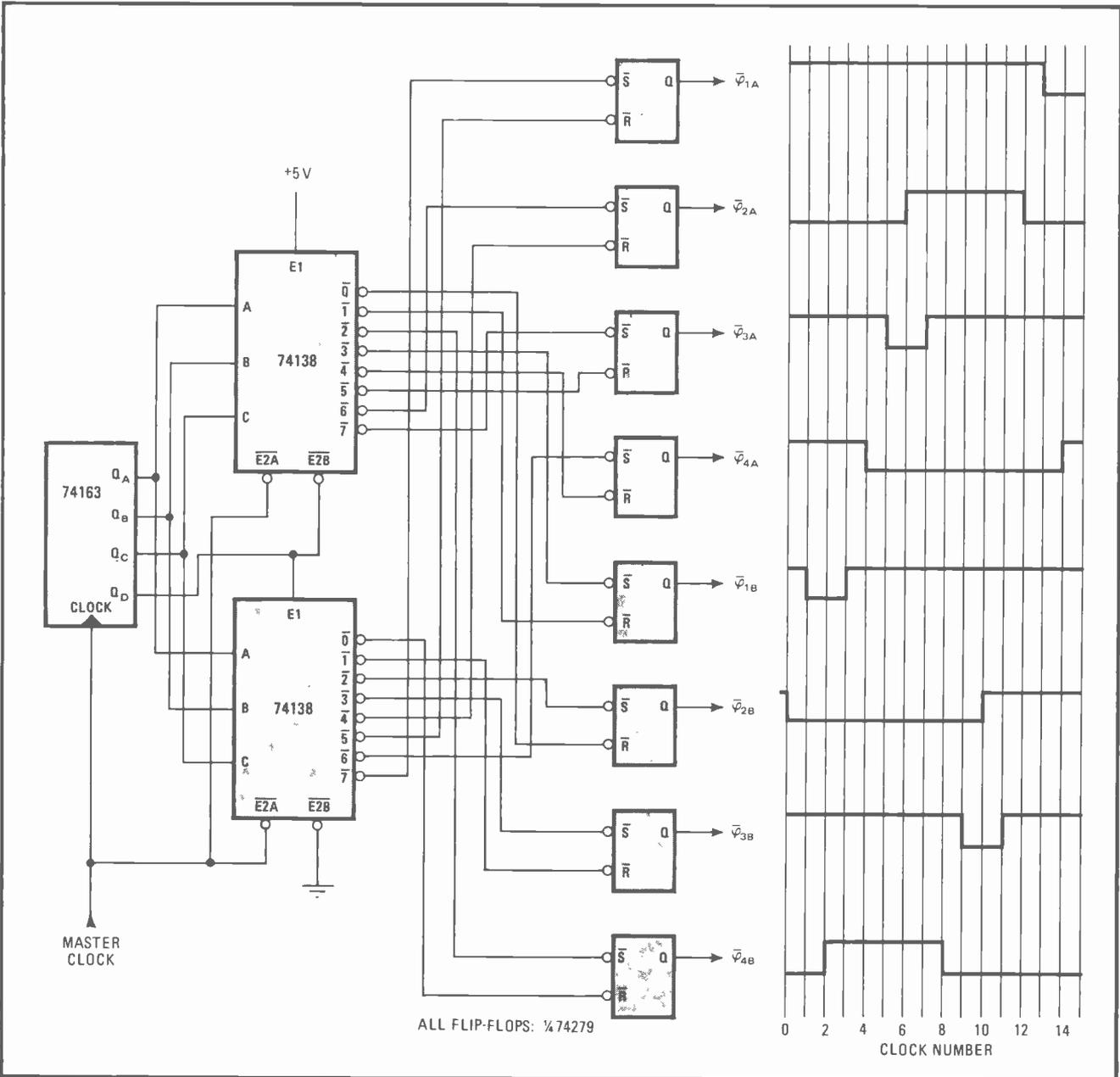
**Multiphase clock and waveforms.** Master clock can be stopped or started at any point in cycle without affecting the phase relationship at all. Skew in output waveforms can be limited to propagation delay of one gate, provided that edge-triggered flip-flops are used.
