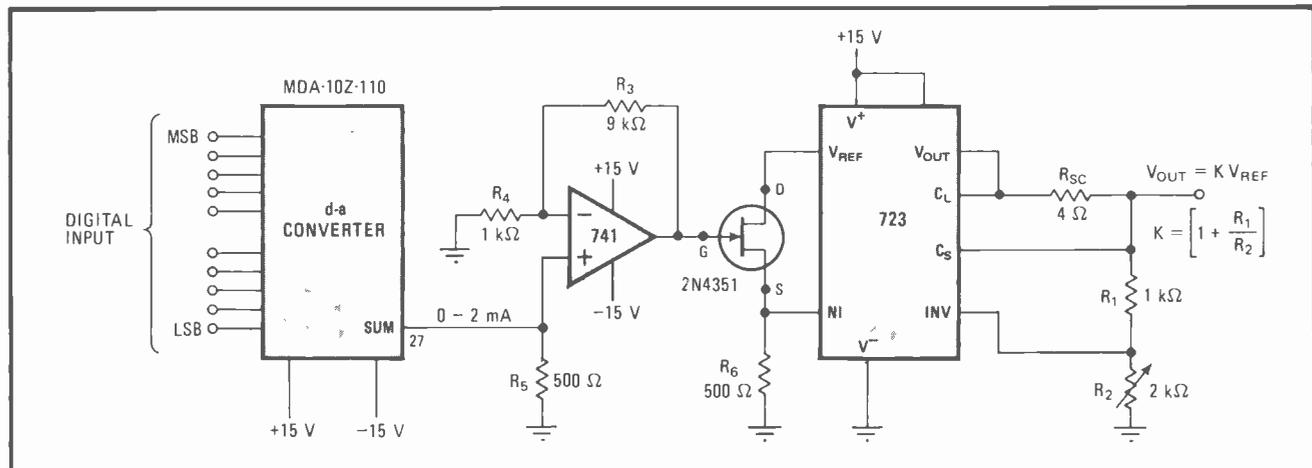
**1. Controlled voltage generator.** Digital-to-analog converter determines output voltage of regulator when FET is used as a voltage-variable resistor. If digital source is computer, specified voltages may be generated for automatic testing of components.
