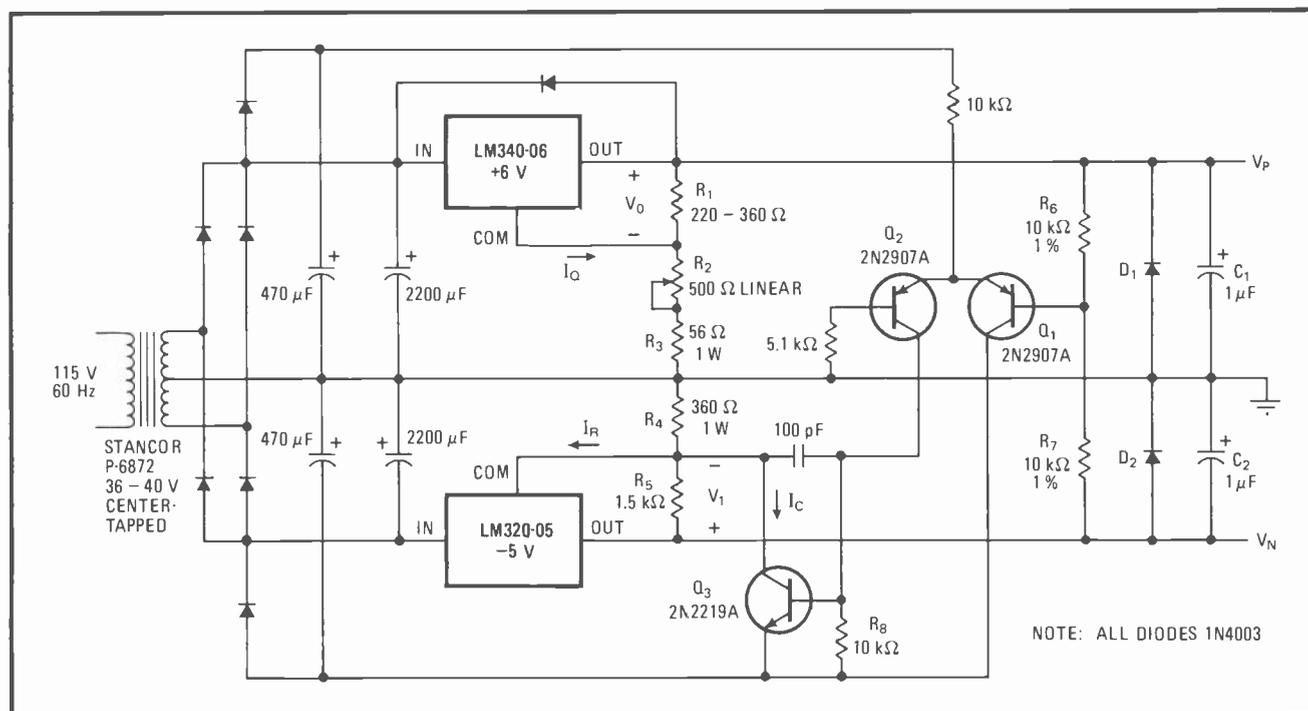
**Bipolar-tracking power supply.** Adjustable voltage output is obtained with fixed-voltage regulators if each regulator is connected back to back through current-varied networks. Circuit retains regulation properties, has high current capability, excellent trackability.
