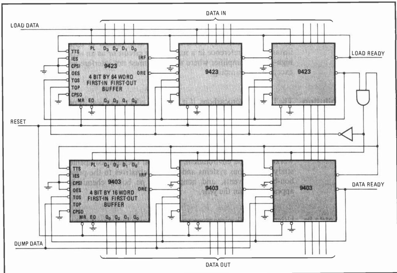
**No need for DMA controller.** Expandable FIFOs can store up to 80 12-bit words before interrupt request is serviced, eliminating need for direct-memory-access port. Several easily synthesized control signals generate interrupt and load signals, determine status of FIFOs.
