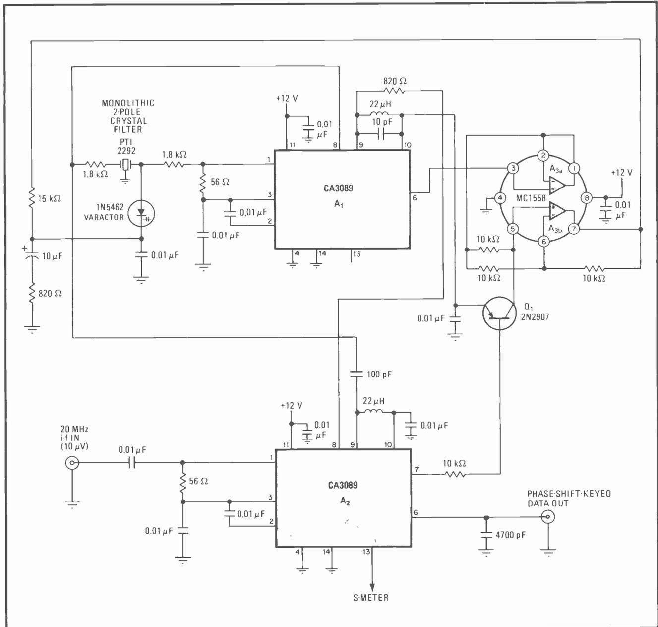
**2. Differential-PSK demodulator.** Two CA3089 phase-locked loops vastly reduce hardware needed for Costas loop demodulator. The circuit detects differential phase-shift-keyed signals with an i-f input of 20 megahertz. With proper attention to rf grounding and shielding, the detector can operate with signals as low as 10 microvolts. An S meter can be connected to pin 13 of  $A_2$  for indicating signal strength.
