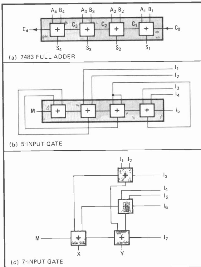
This is the basic design tool used in the design of any n-bit majority gate.
