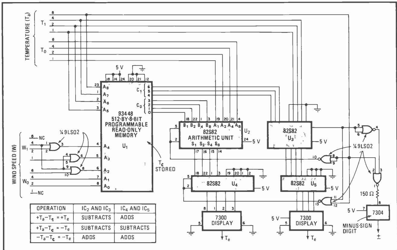
**Cold solution.** Circuit determines and displays wind-chill temperature ( $T_e$ ). Air temperature ( $T_a$ ) and wind-speed data (w) address PROM lines to access apparent temperature change ( $T_c$ ) brought about by given w at  $T_a$ . Arithmetic/logic units  $U_2$  and  $U_3$  add  $T_a$  and  $T_c$  to find  $T_e$ .  $U_4$  and  $U_5$  perform a 10's complement operation for the digital display units, for which they serve as an interface.
