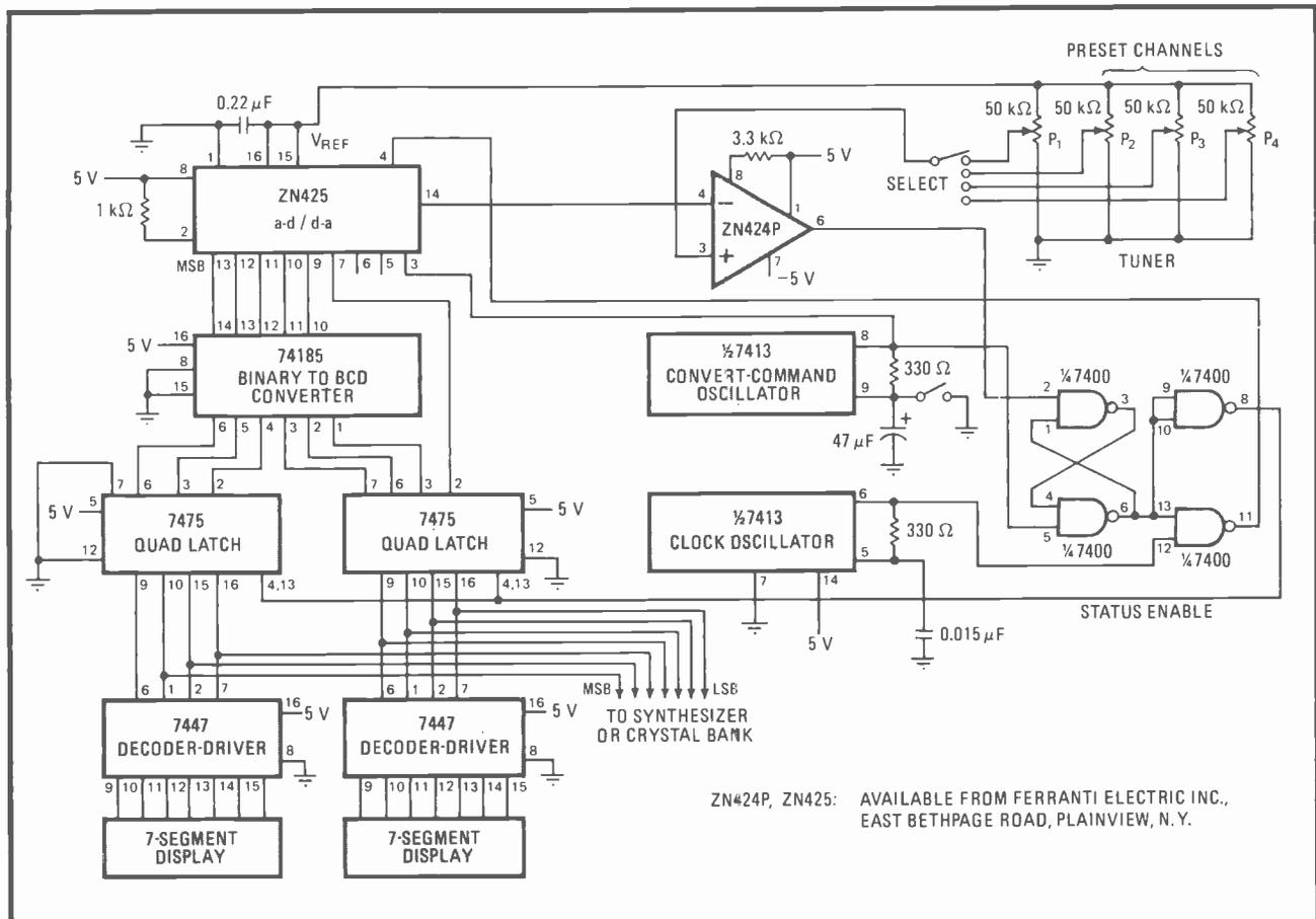
**Single-control synthesis.** Voltage derived from  $V_{REF}$  by 10-turn potentiometers is converted to BCD equivalent for driving synthesizer. Up to 64 channels are generated by 74185 and ZN425. Additional BCD converters, latches, and displays are needed for a 256-channel synthesizer.
