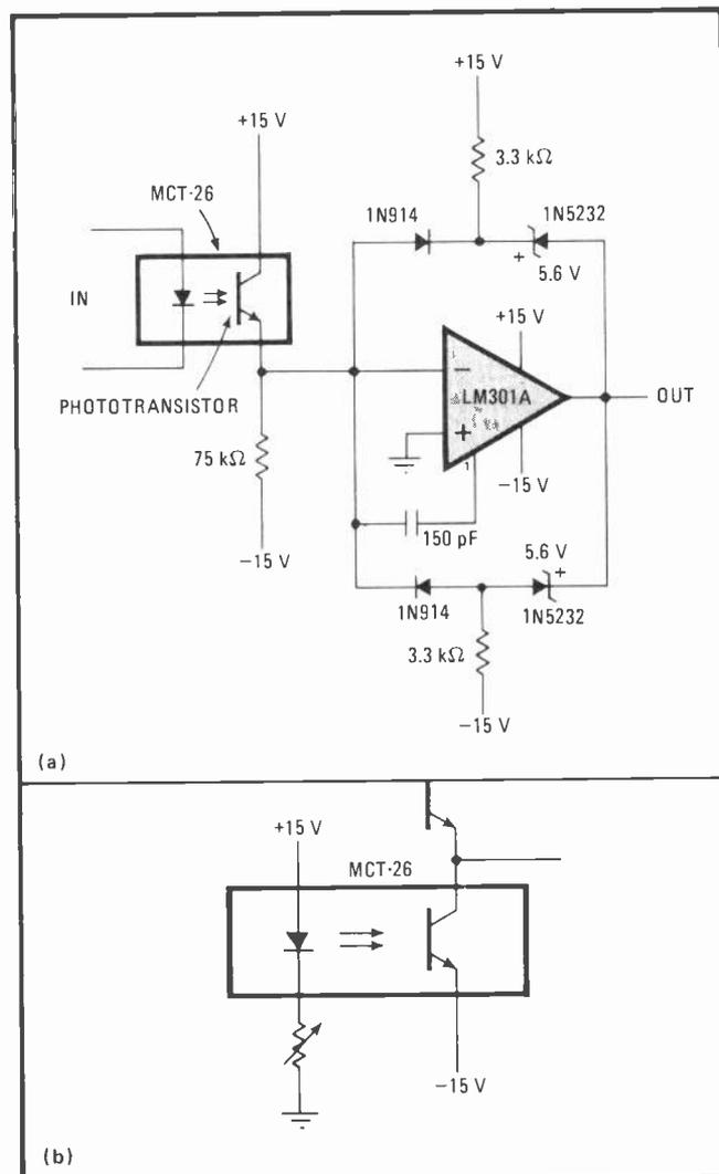
**Accurate transmission.** Phototransistor passes signals to output without pulse distortion. Two feedback loops with op amp work in zero-crossing detector (a) to reduce response time and prevent feedback currents that slow circuit speed, causing errors. Replacing a load resistor by second phototransistor (b) reduces temperature-generated errors by an order of magnitude.
