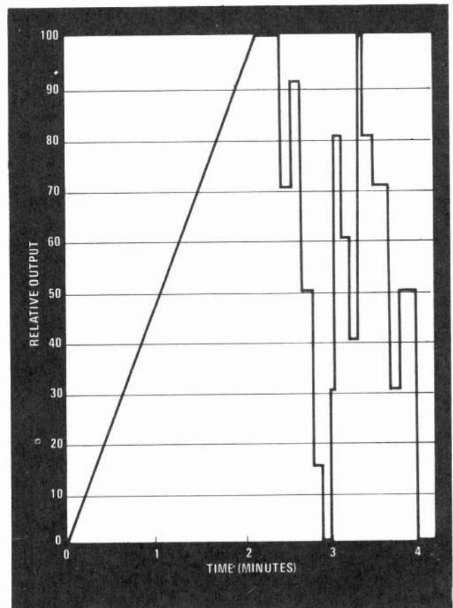
**System response.** Typical graph is accurately reproduced by Heath EU-205-11 strip-chart recorder. System linearity is confirmed with a ramp-test pattern, as shown on left. Right half shows a sample histogram. Total recording time is 4 minutes.
