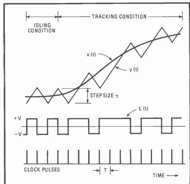
**3. Watching waveforms.** With no input, the tracking signal  $y(t)$  is a series of triangular waveforms corresponding to a binary signal  $L(t)$  of equal and opposite levels. In the tracking condition, the feedback signal attempts to track input signal  $x(t)$ .
