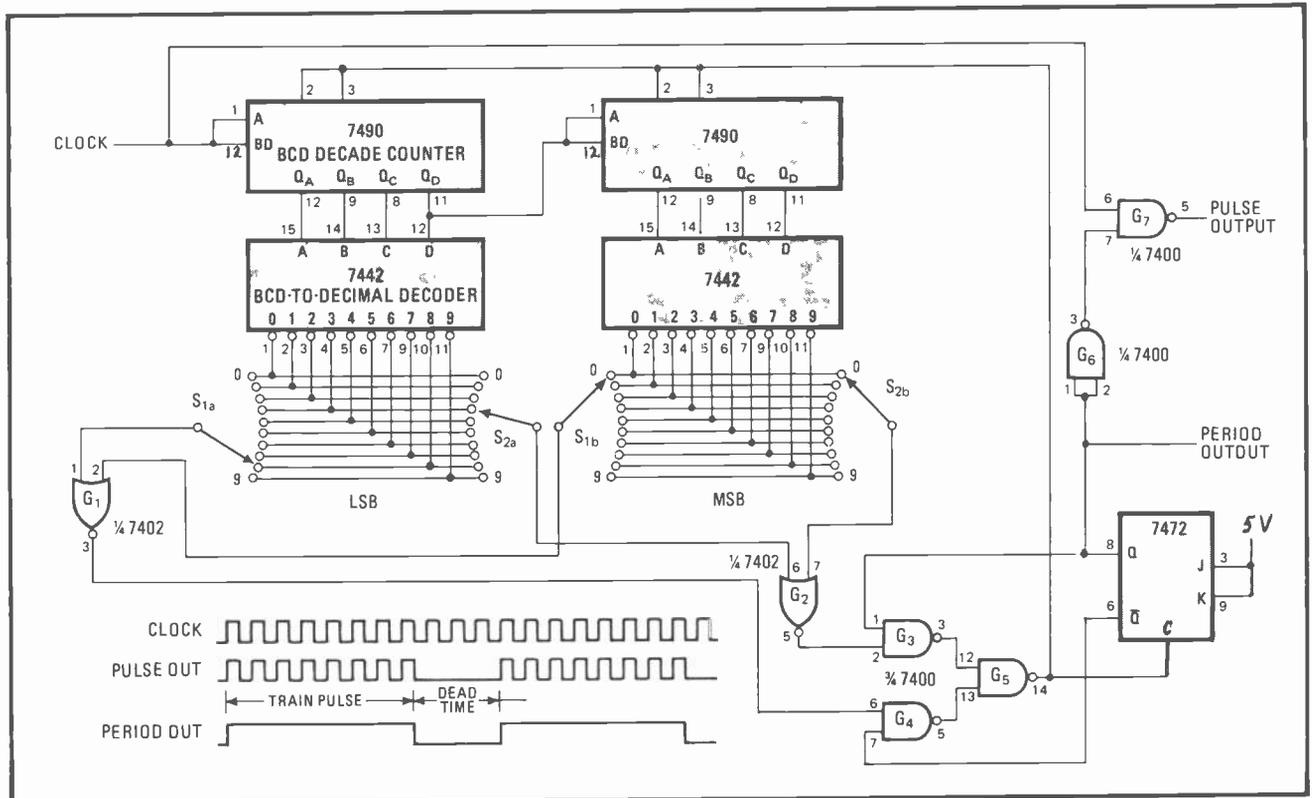
**Selectable.** Generator produces train of  $N$  pulse lengths followed by dead time of  $M$  clock pulses, set by 2-pole, 10-position switches  $S_{1a}$  through  $S_{2b}$ .  $N$  and  $M$  may assume any value of from 1 to 99. Switches are shown set for pulse train of 8, dead time of 3.
