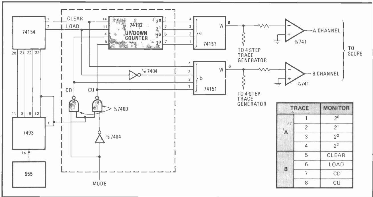
**2. Digital application.** Test of 74192 counter requires addition of inverters and NAND gates as shown, to derive logic signals for desired test sequence. Table specifies signal monitored by oscilloscope. Sync signal for scope is obtained from any point in trace generator chain.
