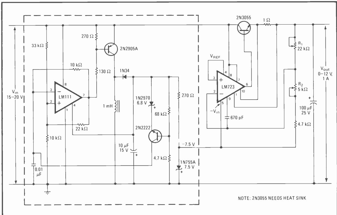
**Full-range regulation.** Dc-input supply is regulated all the way down to 0 V. LM111 and associated circuitry provide negative bias required for LM723 regulator. Regulator's internal-reference voltage,  $V_{REF}$ , is clamped to ground; output voltage is thus adjustable from 0 to 12 V.
