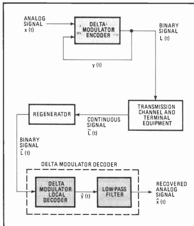
**1. Simple system.** A delta modulator produces a single binary signal  $L(t)$  from an analog input signal  $x(t)$ . The binary signal, degraded by transmission, is reshaped by the regenerator, decoded, and then filtered into a close replica of the original analog signal.
