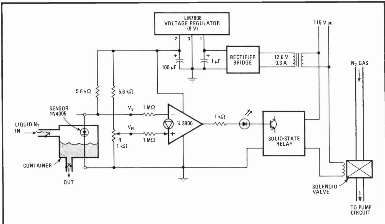
**Fixing the nitrogen level.** When liquid-nitrogen level in container is below the diode position, solenoid is turned on and pumps in more  $N_2$ . When level reaches that of diode, its junction voltage jumps from 0.7 to 1.05 V, turning off solenoid and stopping  $N_2$  inflow.
