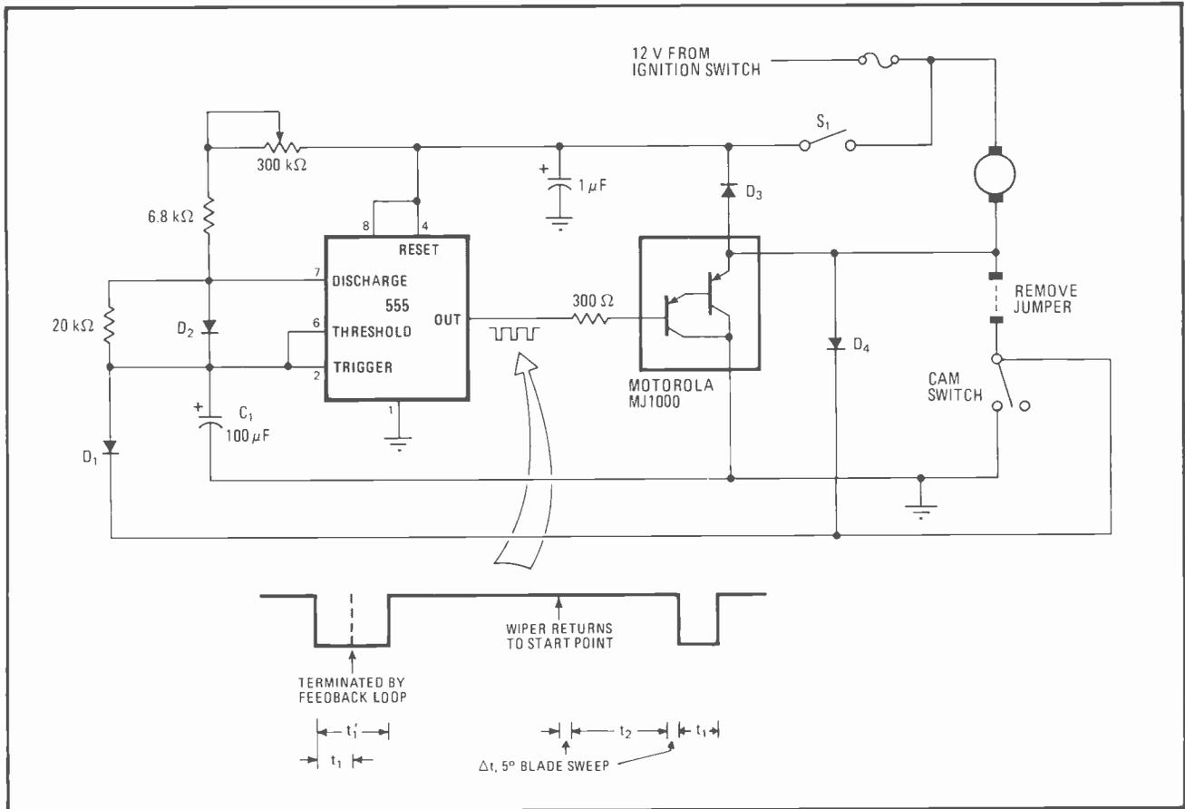
**2. Ground-contact system.** Suggested modification for many General Motors vehicles and other autos with positive-ground system uses same number of components as standard system. Wiper motor is energized by completing ground connection. Note that diodes  $D_1$ ,  $D_3$ , and  $D_4$  are reversed with respect to the polarities shown in Fig. 1 and that pulse-train polarity from 555 output is inverted.
