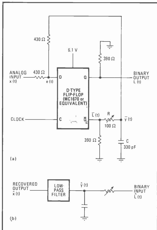
**6. High-speed linear system.** Just two components, a D-type flip-flop and an RC integrator, provide the encoding functions. Here the D-type flip-flop replaces the comparator and sample-and-hold circuit of Fig. 2; an RC integrator and low-pass filter do the decoding.
