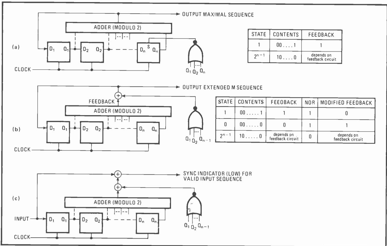
**Balanced states.** The usual  $n$ -stage, pseudo-random number generator cannot generate an equal number of 1s and 0s because it cannot cycle through the register's all-zero state (a). Modified circuit cycles through all  $2^n$  states (instead of the usual  $2^{n-1}$  states) and detects 0s (b). Circuit can be used in feed-forward mode to detect repeating sequences (c).
