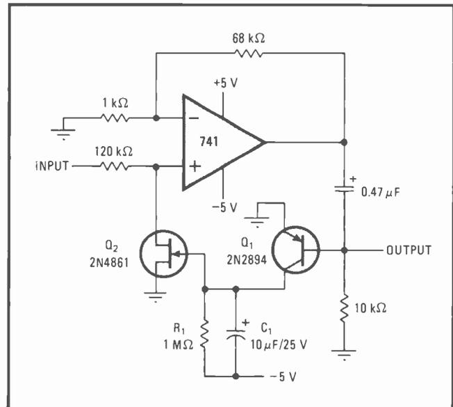
1. **Audio AGC.** Input voltage for distortionless output is from 20 millivolts to 20 volts in this quick-response AGC circuit. The input signal can have greater magnitude than the supply voltage because the maximum signal across the FET is 25 millivolts.
