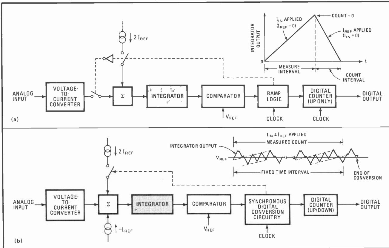
**1. Integrating.** The dual-slope analog-to-digital converter (a) has a two-phase operating cycle made up of measure and count intervals. However, the quantized-feedback a-d converter (b) performs the measure and count functions simultaneously in a fixed-time interval.
