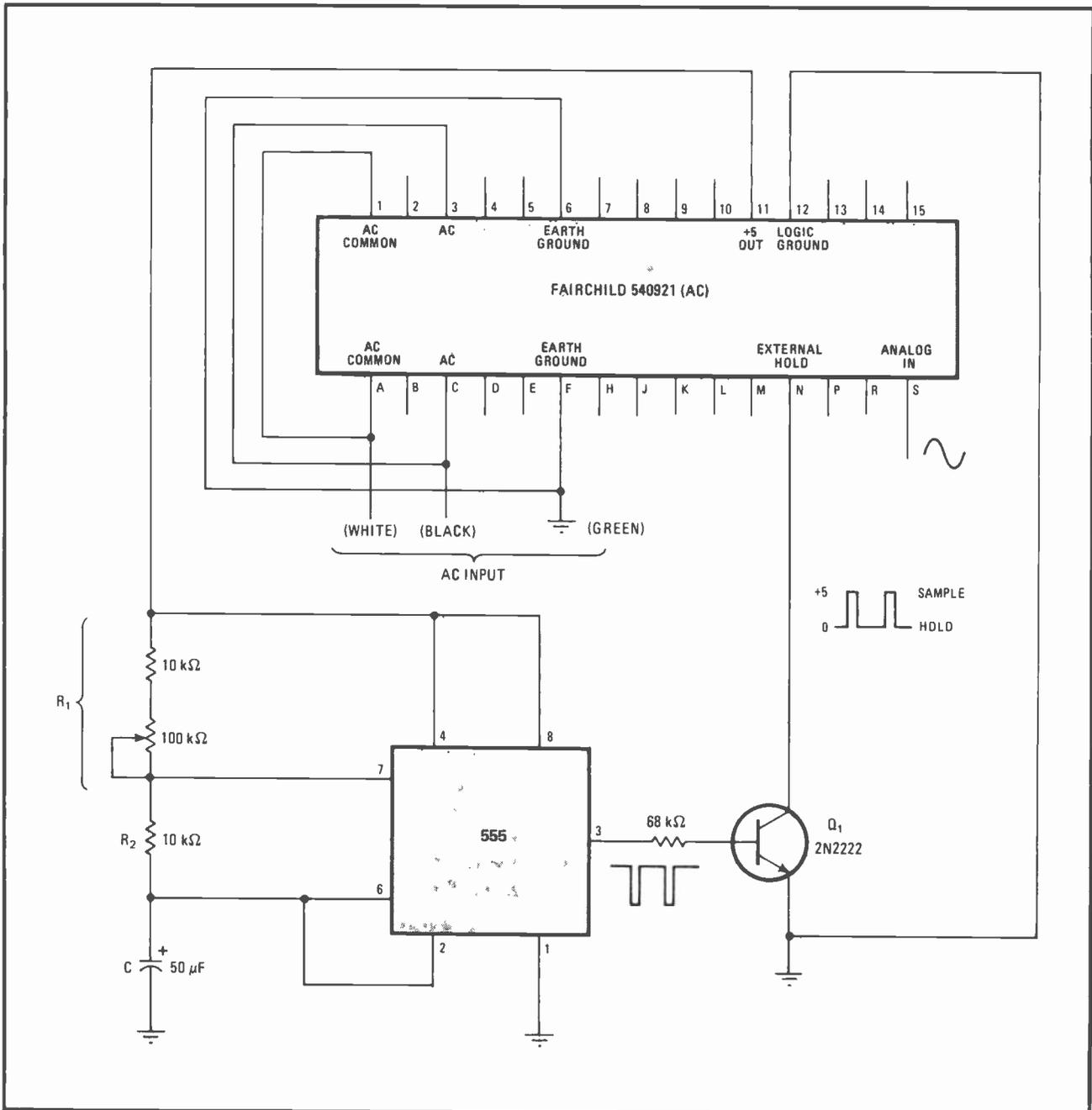
**Sample-and-hold timer.** A 555 extends the display period to relax hyperactive digital panel meters. The display can be frozen for 0.7 to 4.2 seconds, and updated every 1 to 4.5 seconds. Power for the circuit can be obtained from the DPM's 5-volt supply or a battery source.
