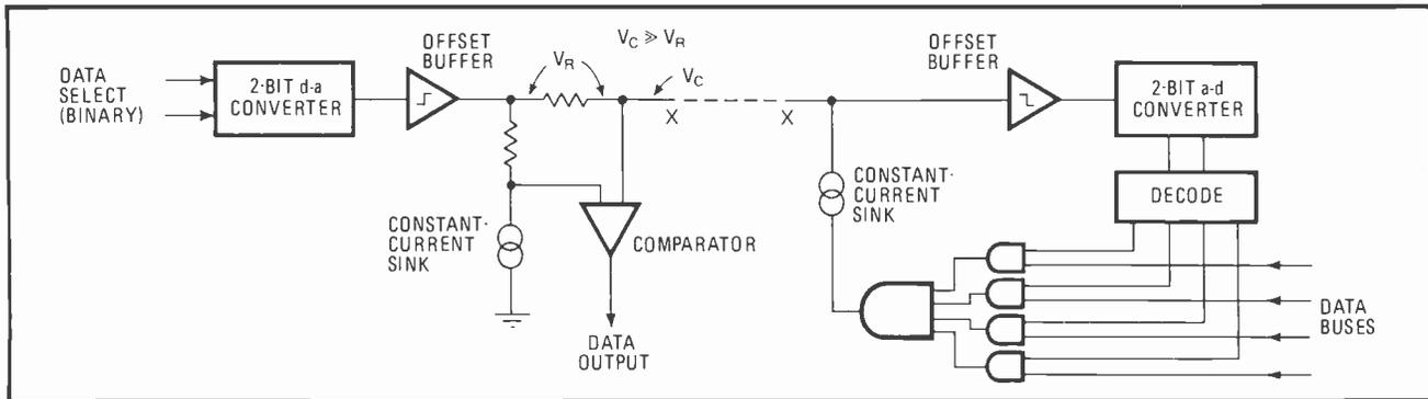
**2. Digital-data application.** Practical nonbinary system may be easily implemented. Two-bit d-a converter assumes duties of  $V_1$  in Fig. 1; a-d converter is  $V_2$ . Logic drives current sink  $I_2$ . Comparator is  $I_1$ . Offset buffers calibrate current sinks.
