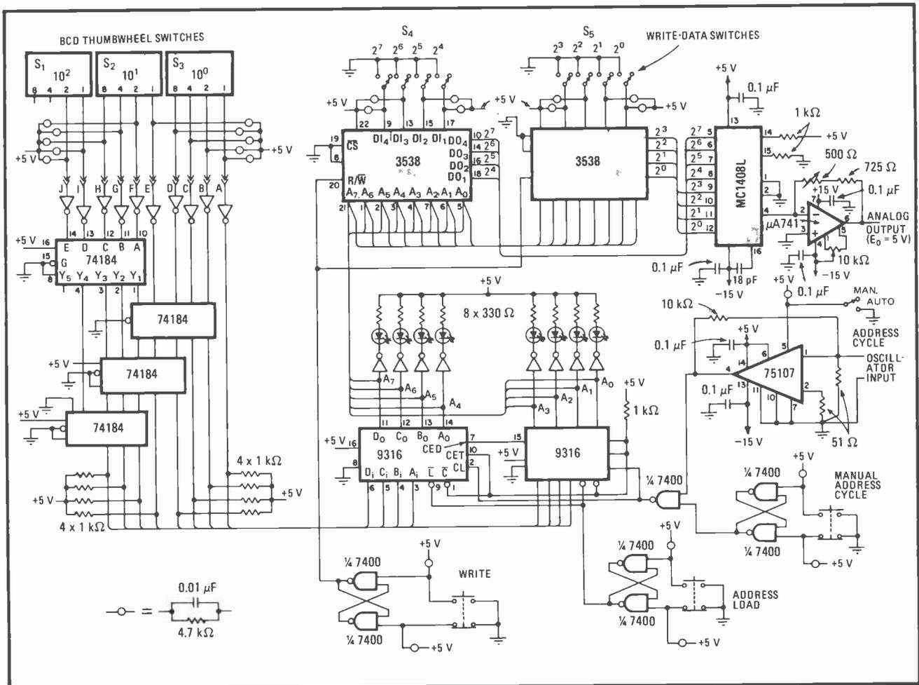
**Simple storage of complex waveshapes.** Programmable generator is capable of producing almost any complex low-frequency waveform. Once the digital equivalent numbers of the waveform are determined, they are stored in the 3538 random-access memories. The MC1408L digital-to-analog converter transforms the random-access memory's contents into the desired analog waveform.
