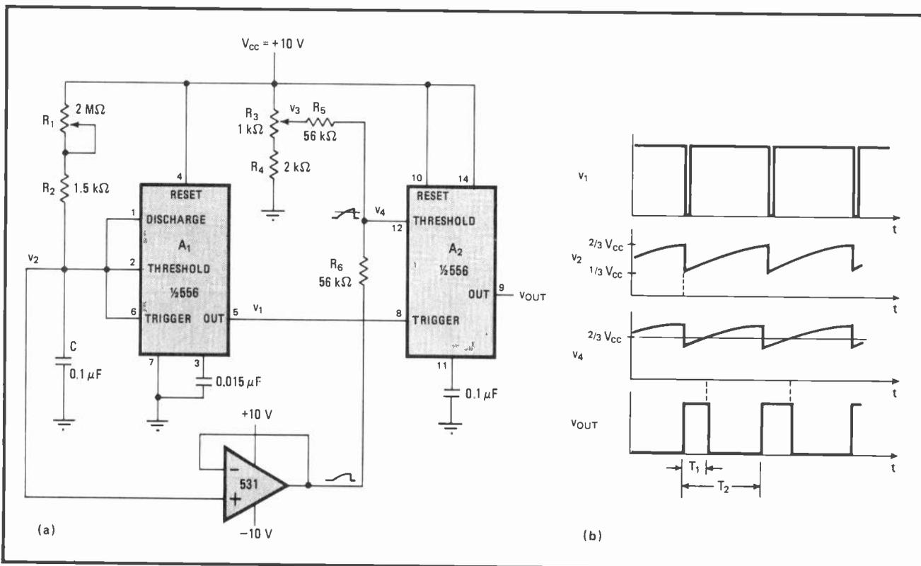
**No relation.**  $A_1$  runs at frequency set by  $R_1$ . But duty cycle is selected by  $R_3$ , which controls signal offset at threshold port of  $A_2$ . No feedback loops link  $A_1$  and  $A_2$ , thereby ensuring independent adjustment of rep rate and duty cycle. Timing diagram details operation.
