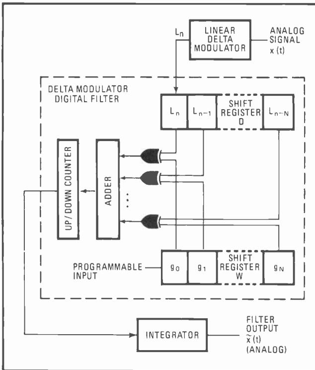
**9. Digital filter.** Digital encoding and filtering using delta modulation techniques requires several components. The filter accepts a binary input from the delta modulator, and the overall filter properties are changed simply by reprogramming the input to shift register W.
