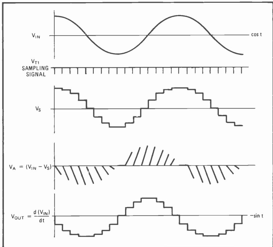
where  $E_f$  is the final output voltage at the time immediately before the next sample, and  $d(e)/dt$  is the change in input voltage between sampling intervals, or the derivative of the input signal with respect to time. The output waveforms in Fig. 1 indeed confirm this equation. How is the output generated?
