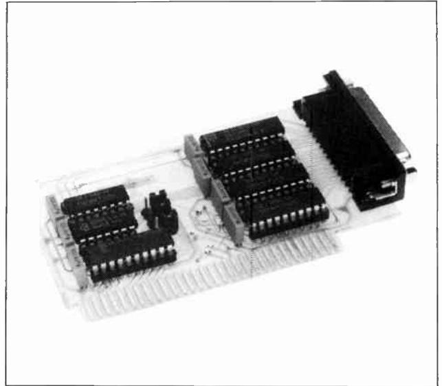
Fig. 28. Photograph of completed IBM interface board.
