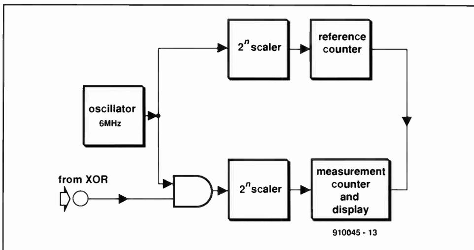
Fig. 3. Block diagram of the digital measuring section.
