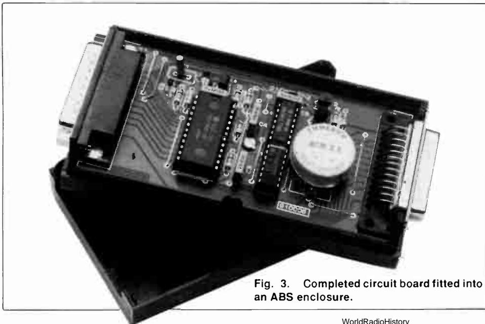
Fig. 3. Completed circuit board fitted into an ABS enclosure.
