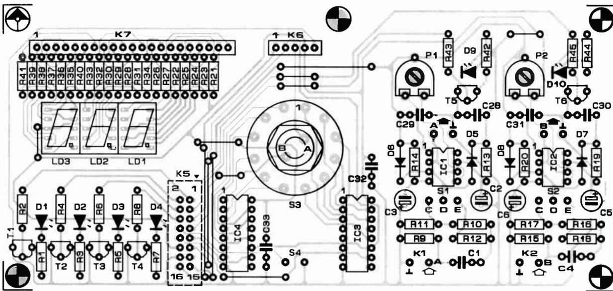
Fig. 8. Printed-circuit board for the displays, input stages, and selector switches.
