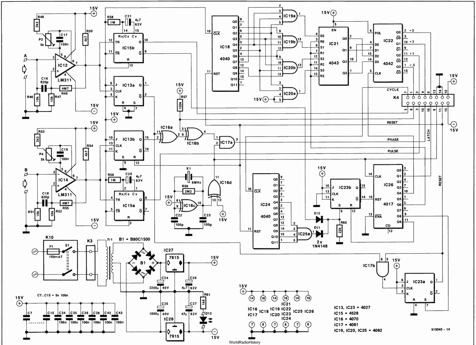
Fig. 4. Diagram of the circuit contained on the mother board.
