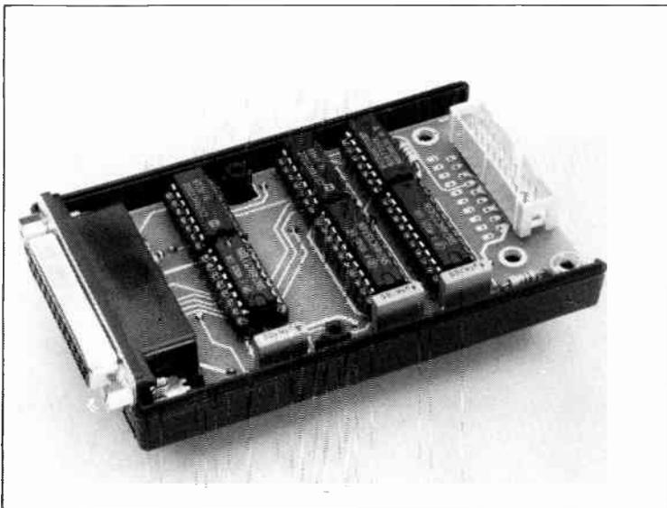
Fig. 27. Photograph of completed Atari interface board.
