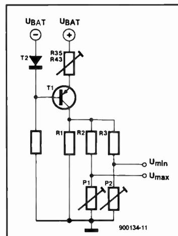
Fig. 7. Circuit for measuring the battery voltage with respect to earth.
