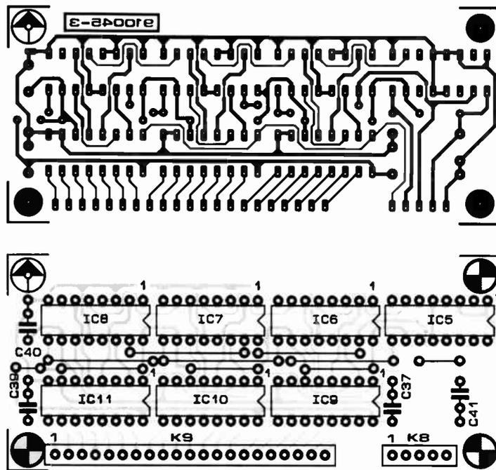
Fig. 10 Printed-circuit board for the logic circuits for the LED displays.
