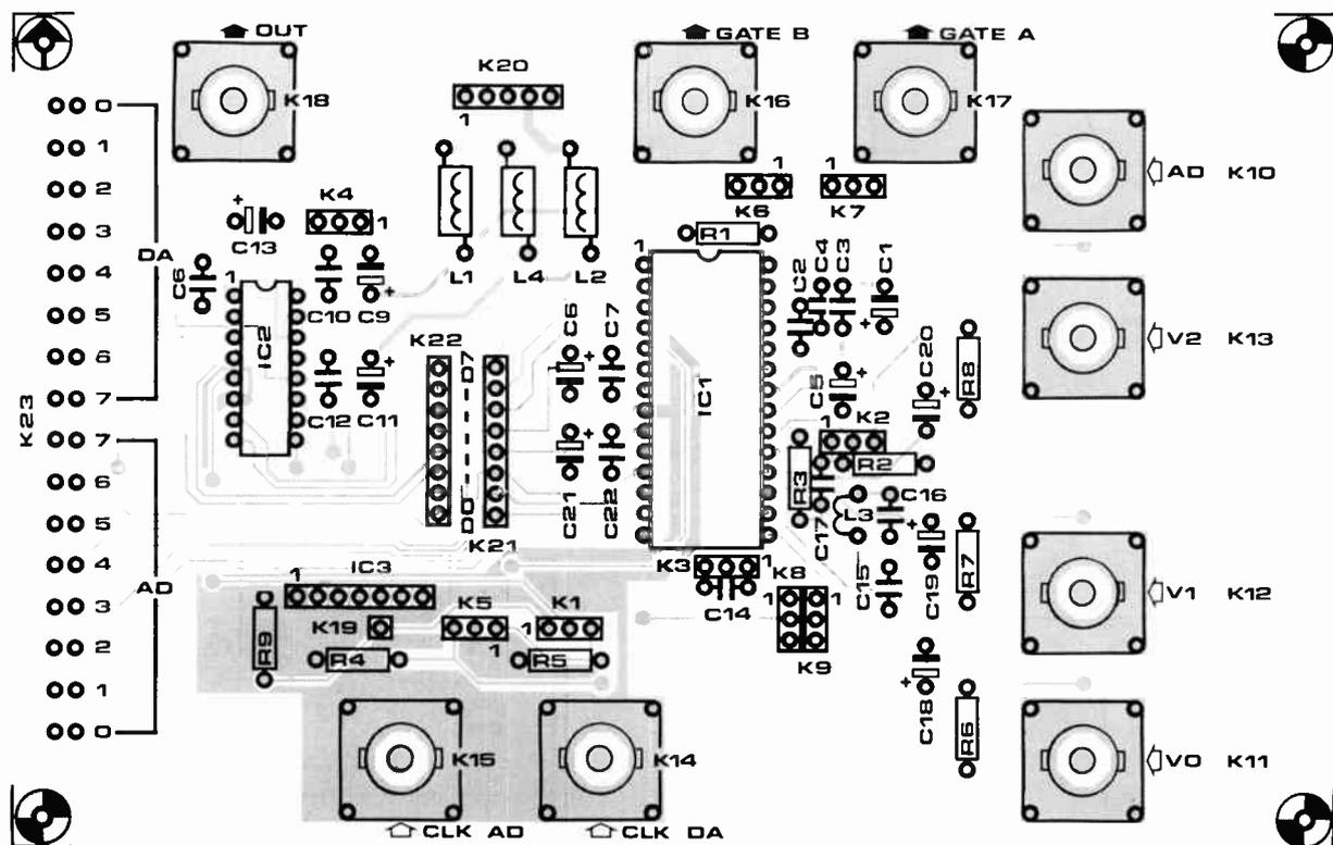
Fig. 11a. Component mounting plan of the double-sided printed circuit board. Note that the board is designed for PCB-mount BNC sockets.
