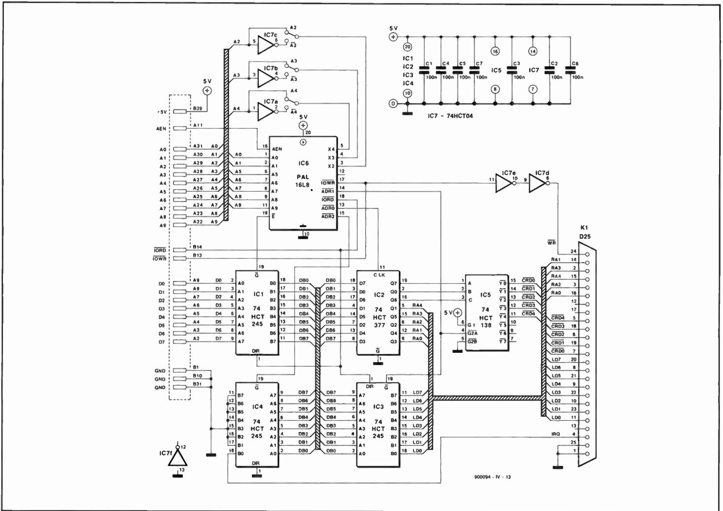
Fig. 21. Circuit diagram of the IBM interface.
