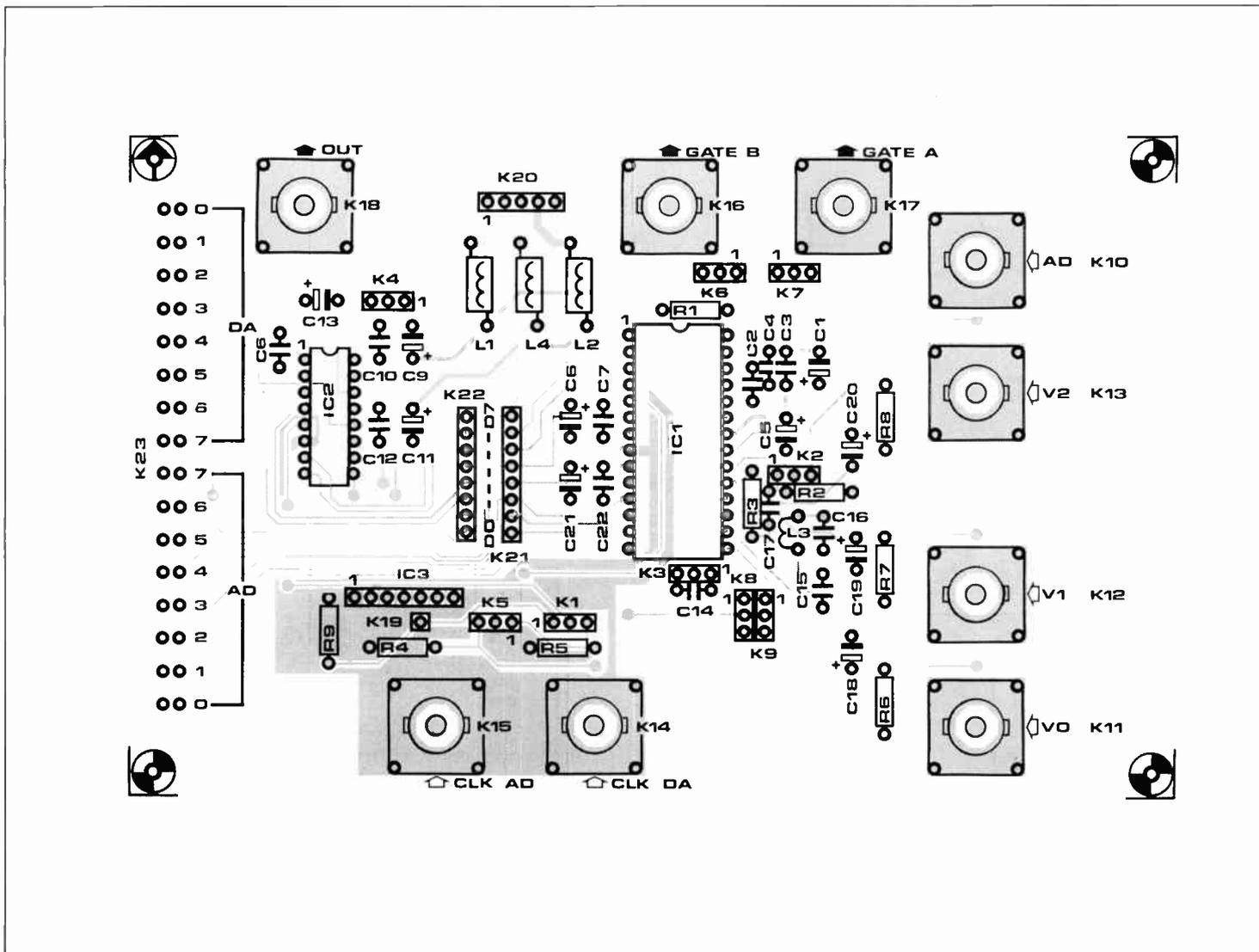
Fig. 11a. Component mounting plan of the double-sided printed circuit board. Note that the board is designed for PCB-mount BNC sockets.
