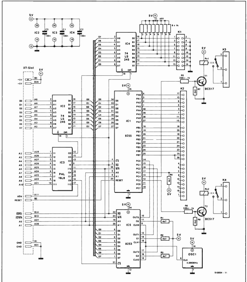
Fig. 1. Circuit diagram of the PC insertion card.
