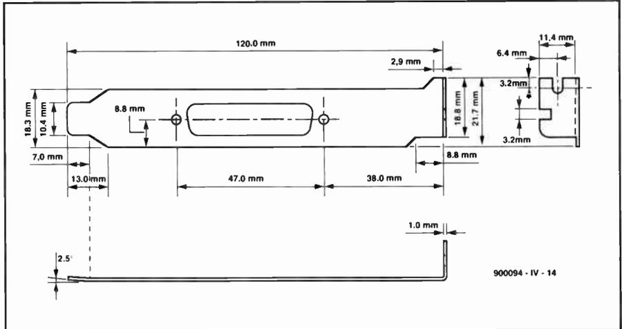
Fig. 24. The IBM interface print should be secured with a fixing plate as shown here.
