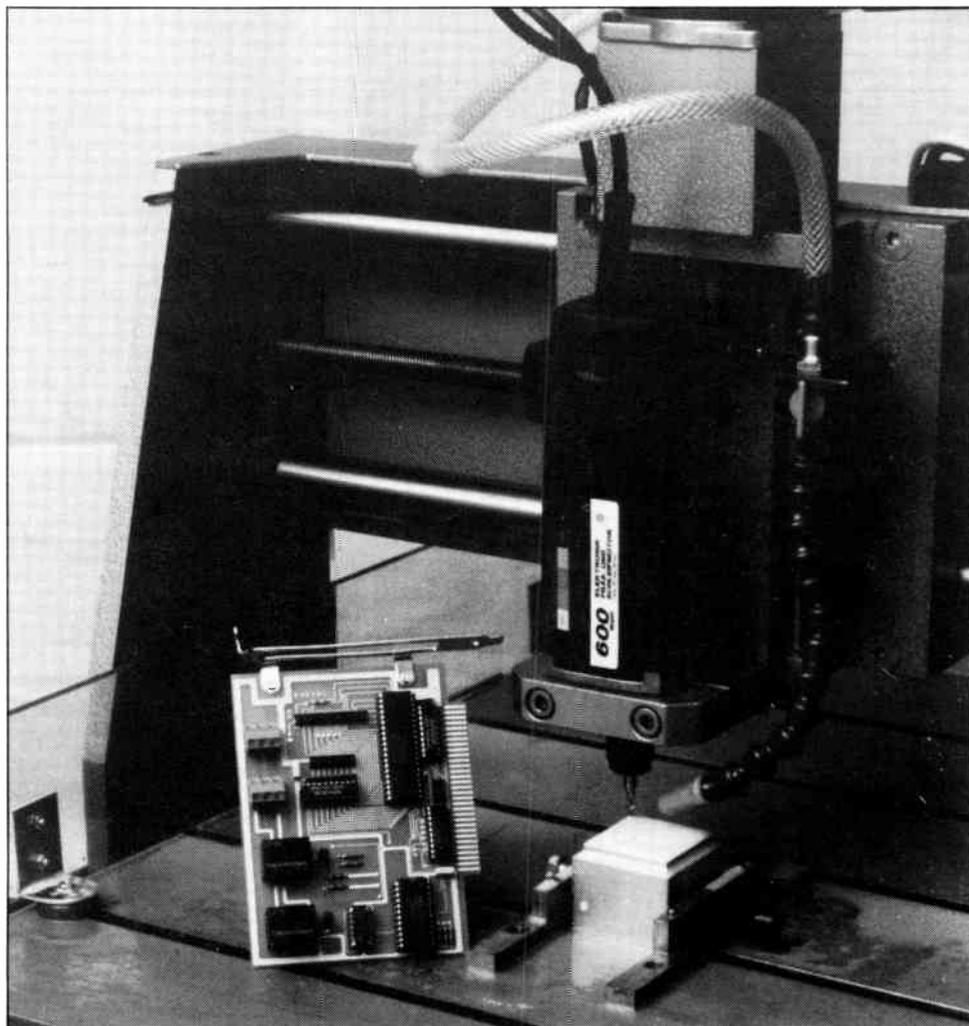
card offers 24 input/output lines, and has an additional timer/counter IC Type 8253, a quartz oscillator and two relays. The quartz oscillator makes the timing of the I/O card independent of the computer speed. The two relays have changeover contacts and are suitable for switching mains loads.
