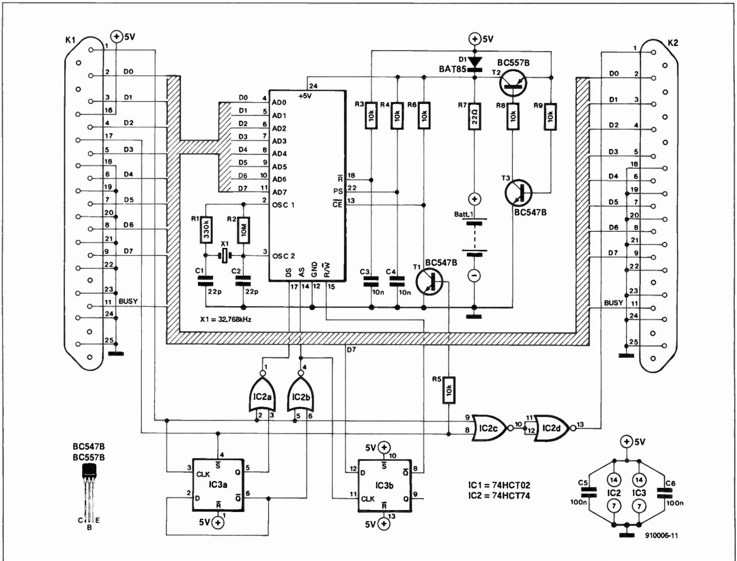
Fig. 1. Circuit diagram of the real-time clock.
