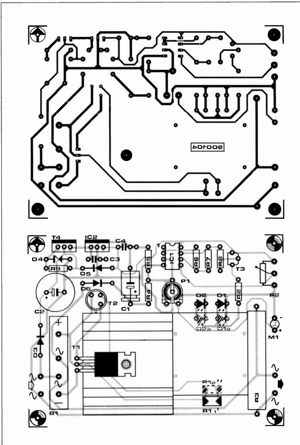
Fig. 4. Single-sided printed circuit board for the a.c. power supply.
