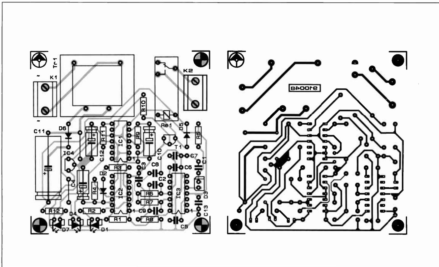
Fig. 5. Single-sided printed circuit board for the IR remote control receiver.
