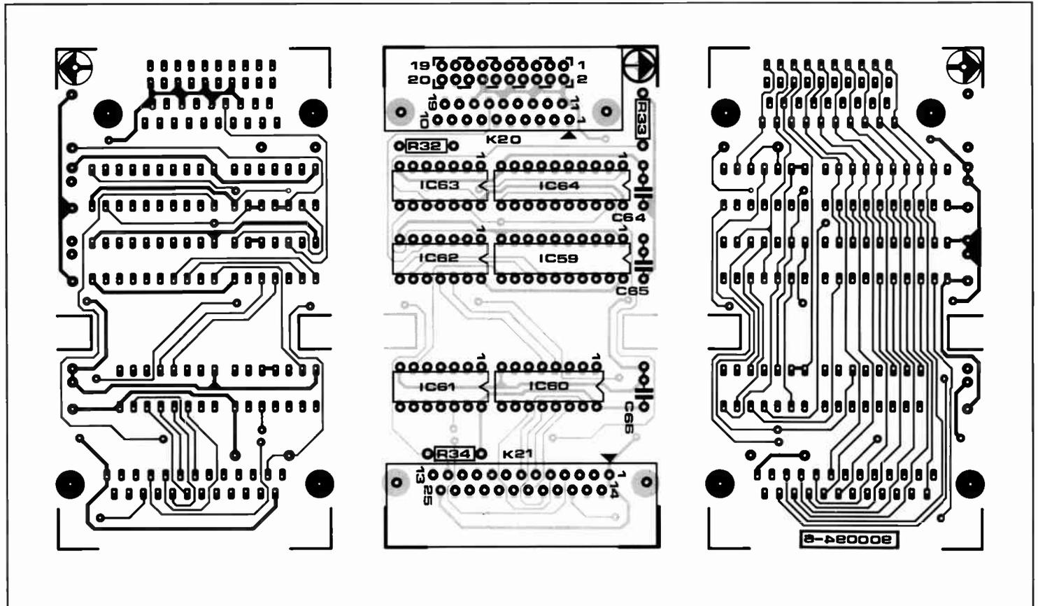
Fig. 20. The printed-circuit board for the Atari interface.
