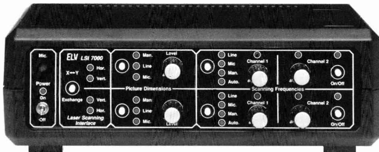
Following last month's description of the laser exciter and the mirror galvanometer assembly we now turn to a state-of-the art electronic control unit for the show laser.
