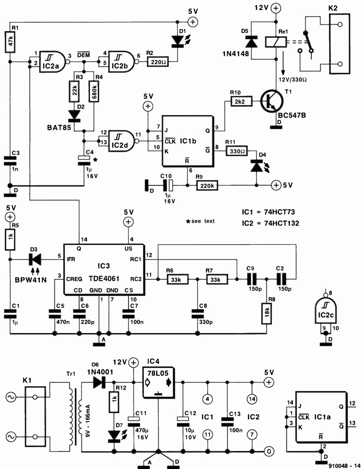
Fig. 4. Circuit diagram of the remote control receiver. The load to be switched is connected to the contact of relay Re1.
