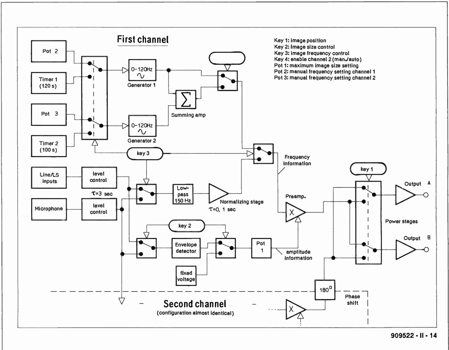
Fig. 8. Block diagram of the laser control unit.
