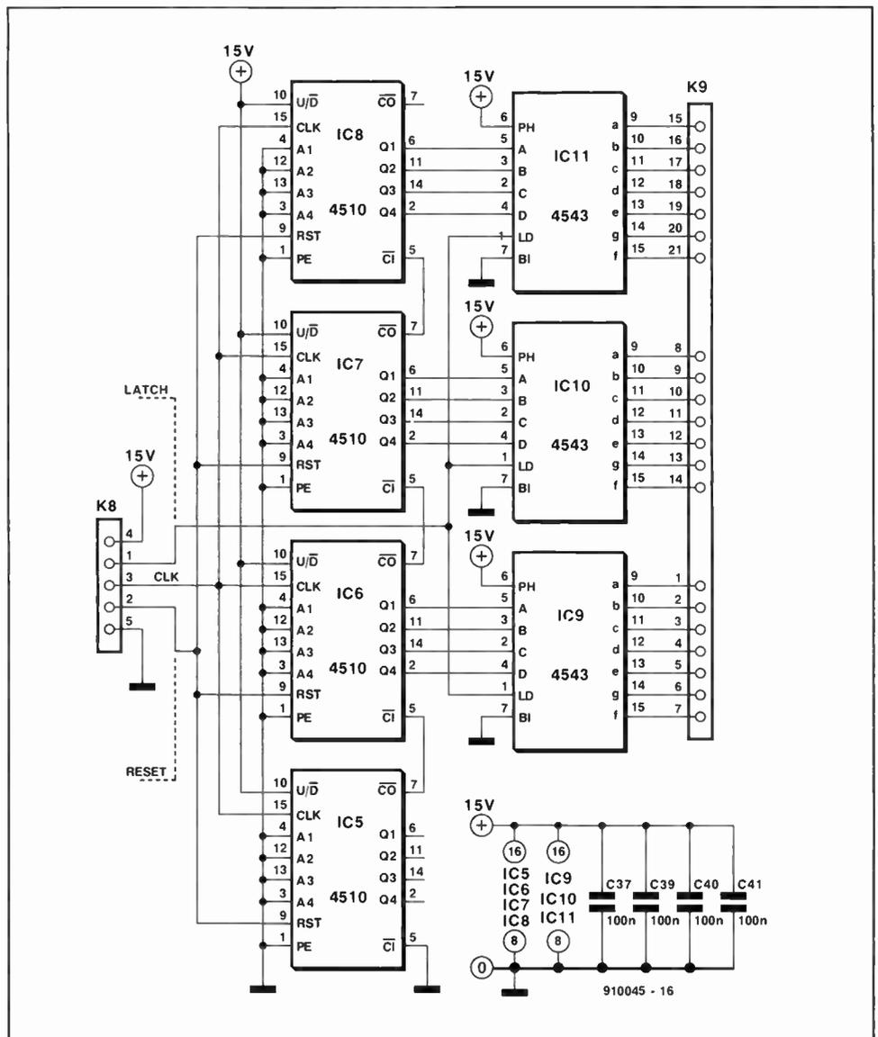
Fig. 6. Diagram of the logic circuits for the LED displays.
