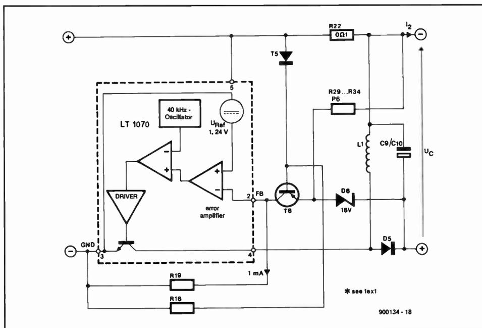
Fig. 5. The switch-mode power supply – see also Fig. 8.
