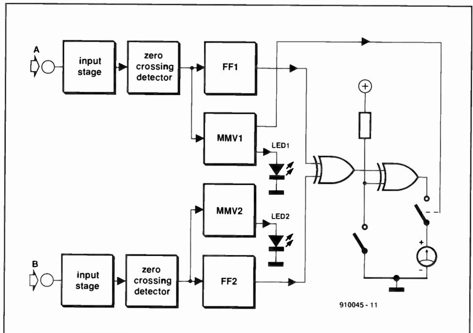
Fig. 1. Block diagram of the digital phase meter.
