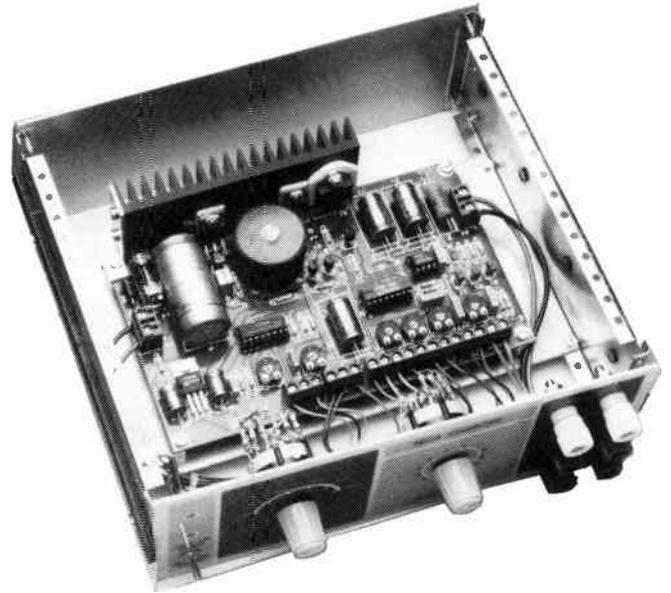
**T**HE charger is based on the Telefunken Type U2400B processor, which has been specially developed for this application. This device contains most of the logic circuits necessary for automatically controlling the charging of Ni-Cd batteries.
