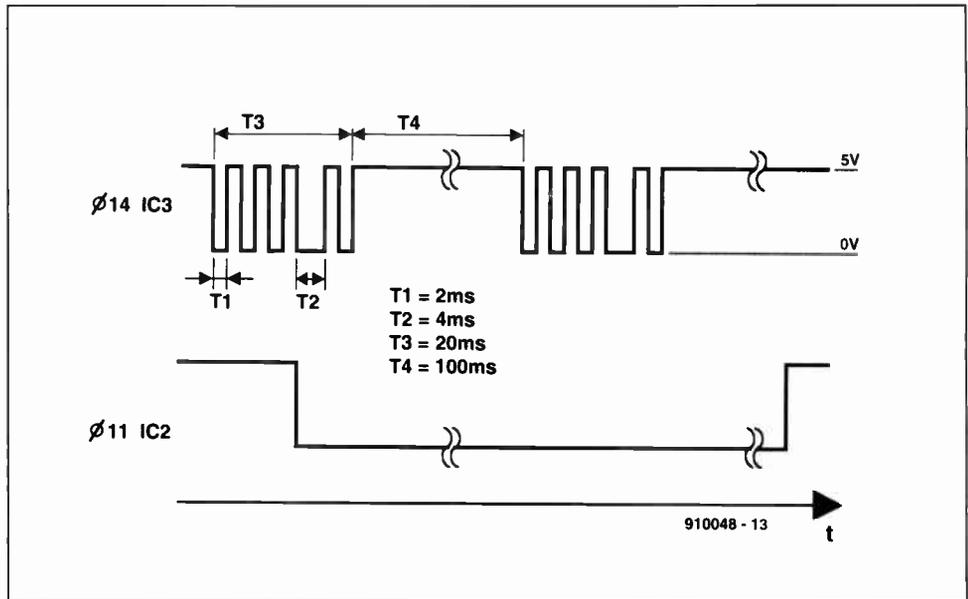
Fig. 2. Response of the the TDE4061 to a typical datastream produced by a TV remote control.
