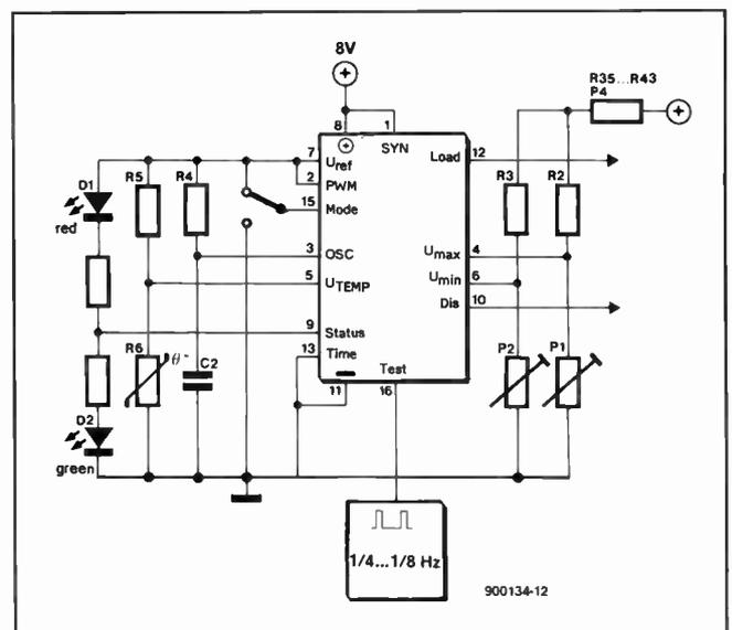
Fig. 1. Basic circuit for the U2400B processor.
