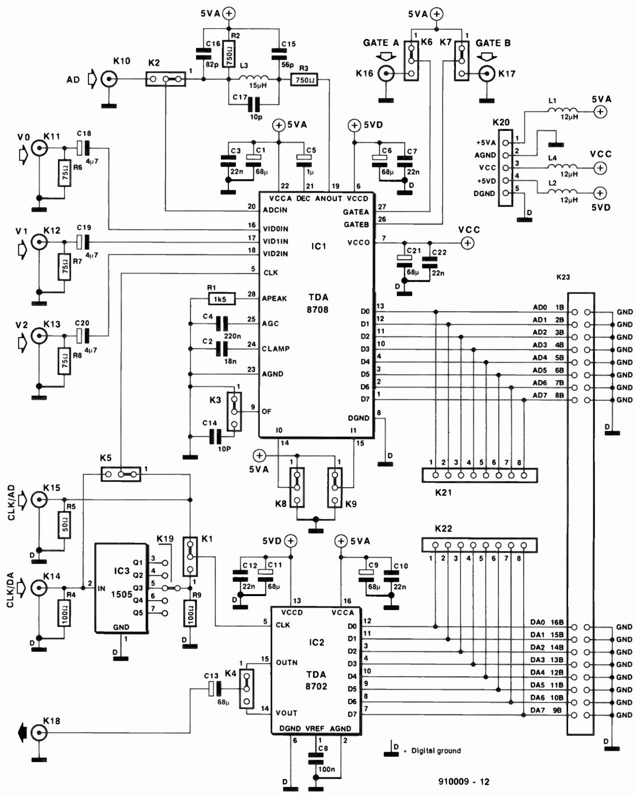
Fig. 10. Circuit diagram of the ADC/DAC converter card. You have the digitized video signal available at a resolution of 8 bits between connectors K21 and K22. A separate connector, K23, allows the card to be connected to a computer bus.
