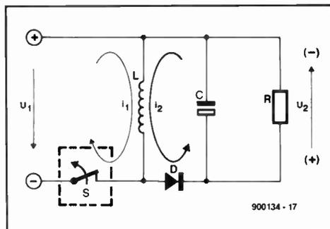
Fig. 4. Concept of a switch-mode power supply.
