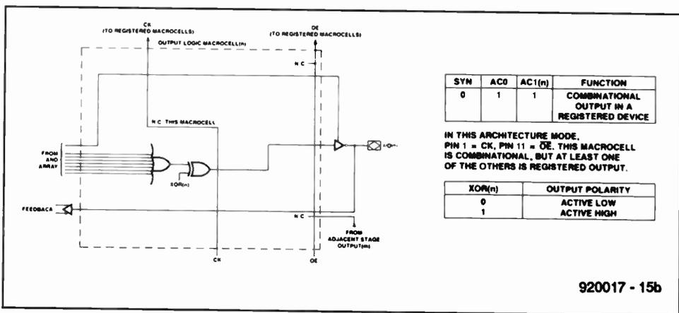
Fig. 6. Combinational output in a registered device.
