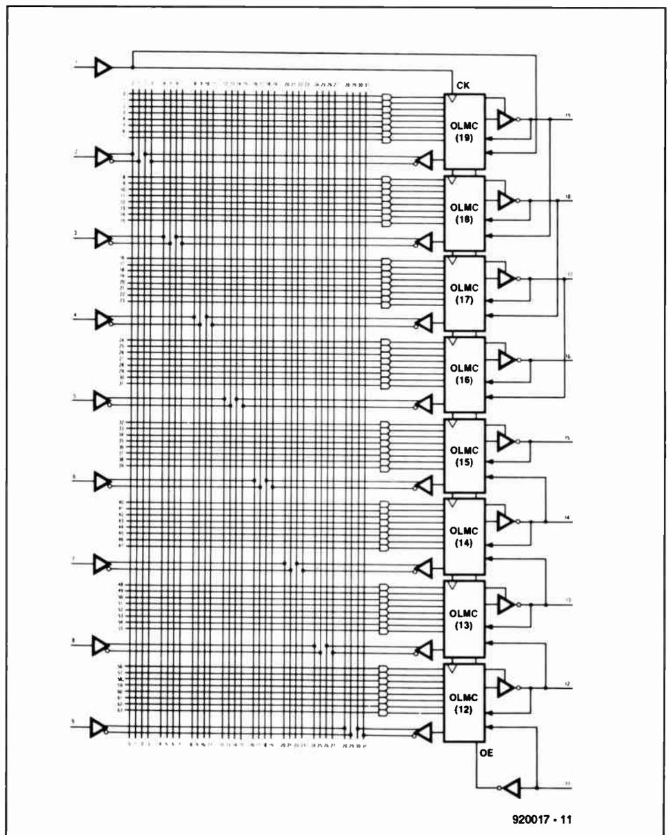
Fig. 1. Logic diagram of the 16V8 GAL IC.
