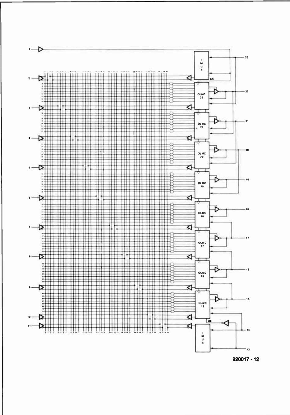
Fig. 2. Logic diagram of the 20V8 GAL IC.
