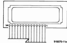
An LCD module has 14 connections, arranged in a single row of solder points, or in two rows of 7 at either side of the PCB. It is best to solder these points directly to a piece of 14-way flatcable. Pin 1 is marked by a '1' on the display board. Attention: when there are two connection rows, the solder points are numbered in pairs (see drawing above).
