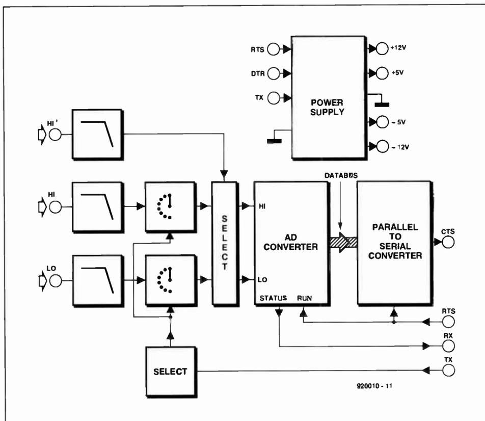
Fig. 1. Block diagram of the RS232-controlled A-D converter.
