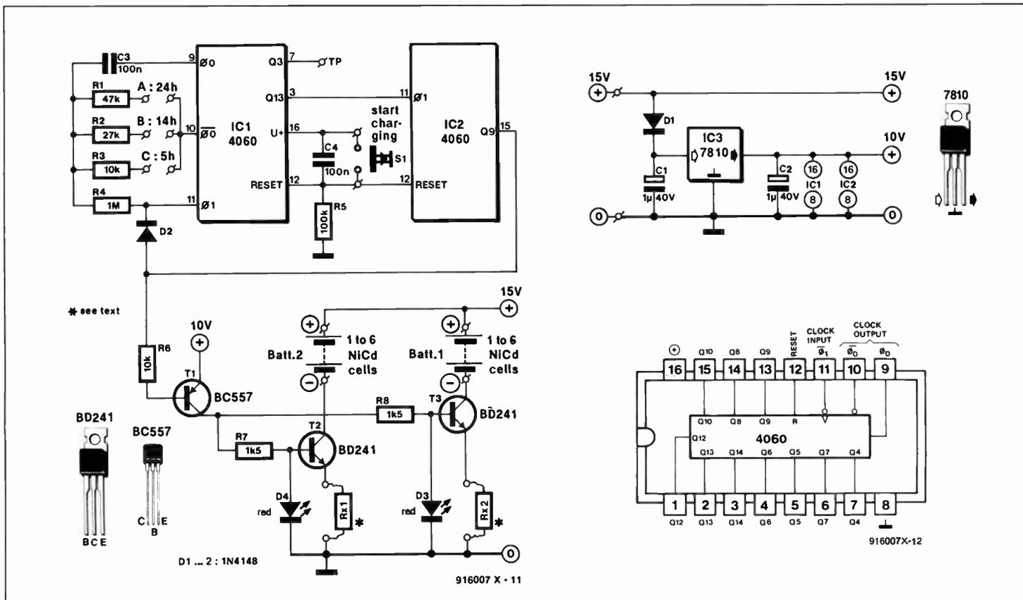
Fig. 1. Circuit diagram of the NiCd charger.
