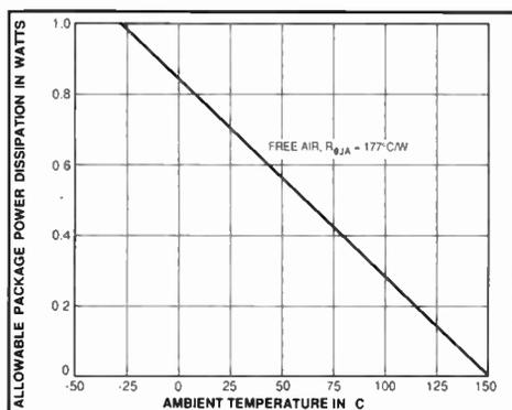
Fig. 2. Allowable power dissipation vs temperature characteristic.
