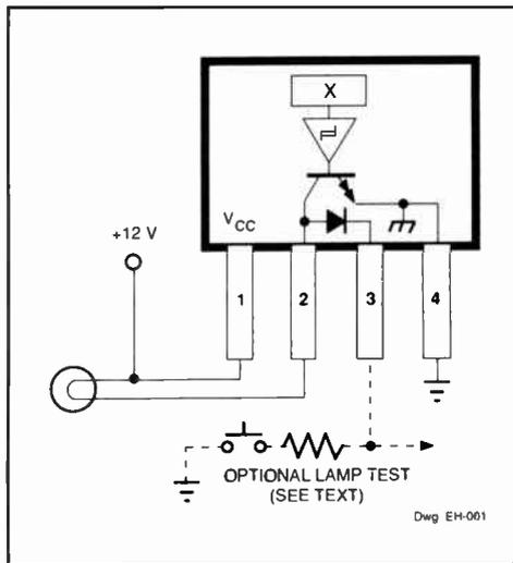
Fig. 6. Typical lamp driver application.
