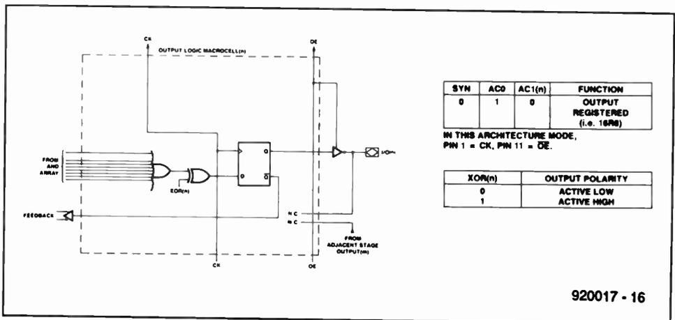
Fig. 7. Registered active high or low output.
