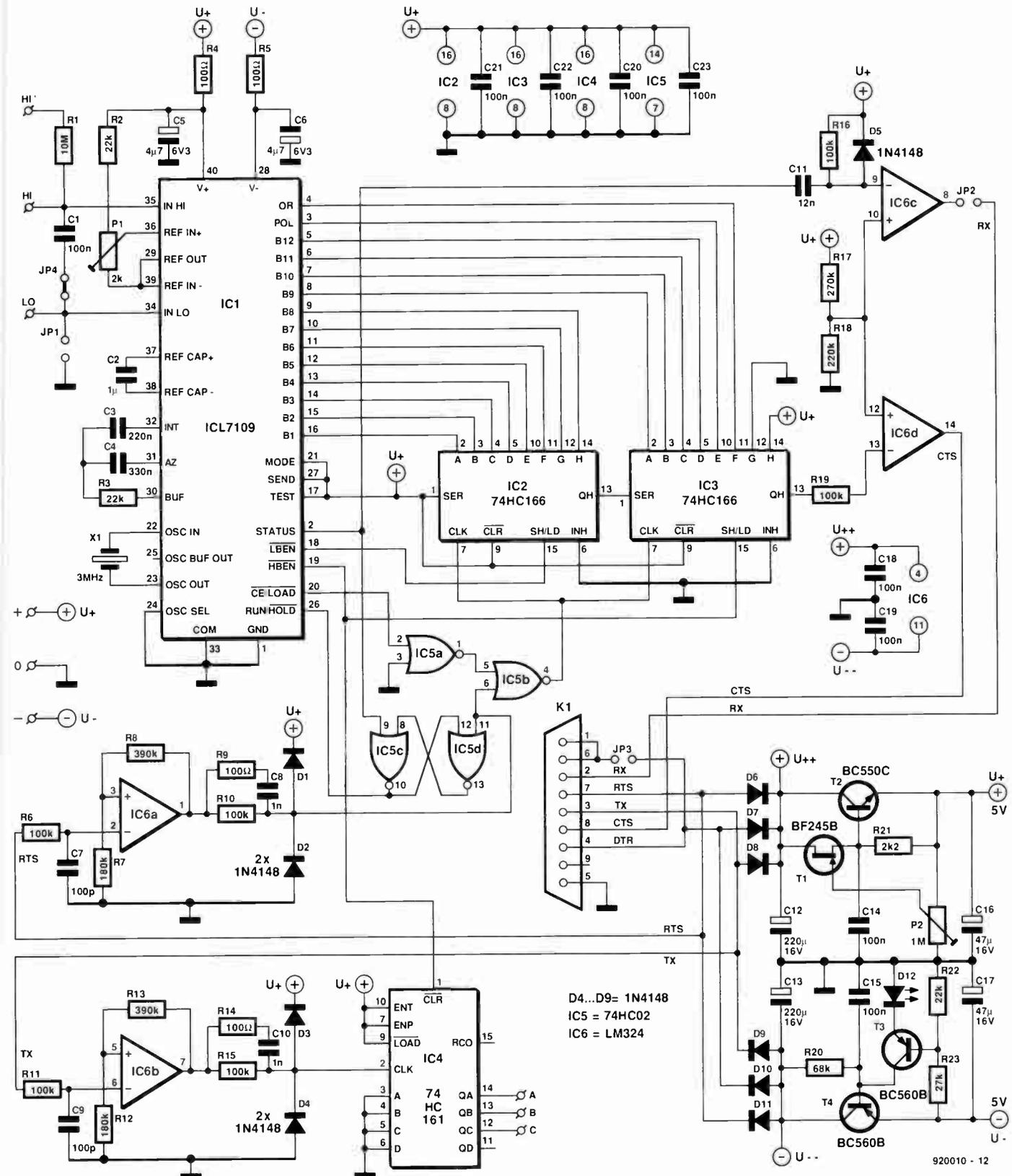
constructed on separate printed circuit boards. Note that the entire circuit is powered via the RS232 link to the PC.
