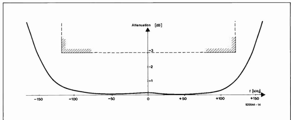
Fig. 9. TQF-2599 attenuation characteristic within pass-band. The ripple is quite small at less than 1 dB.
