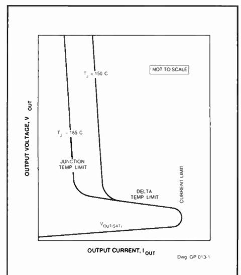
Fig. 5. Output voltage vs output current.
