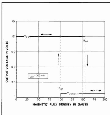
Fig. 3. Typical transfer characteristics at  $T_A = +25^{\circ}\text{C}$ .
