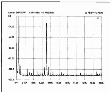
Fig. 4. Intermodulation distortion 500 Hz: 7 kHz; power ratio 4:1.
