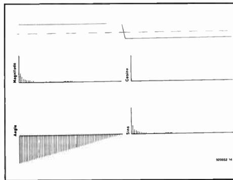
Fig. 9. Fourier plot of periodical DC wave.
