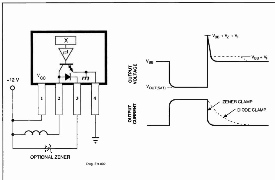
Fig. 9. Typical relay/solenoid driver application.
