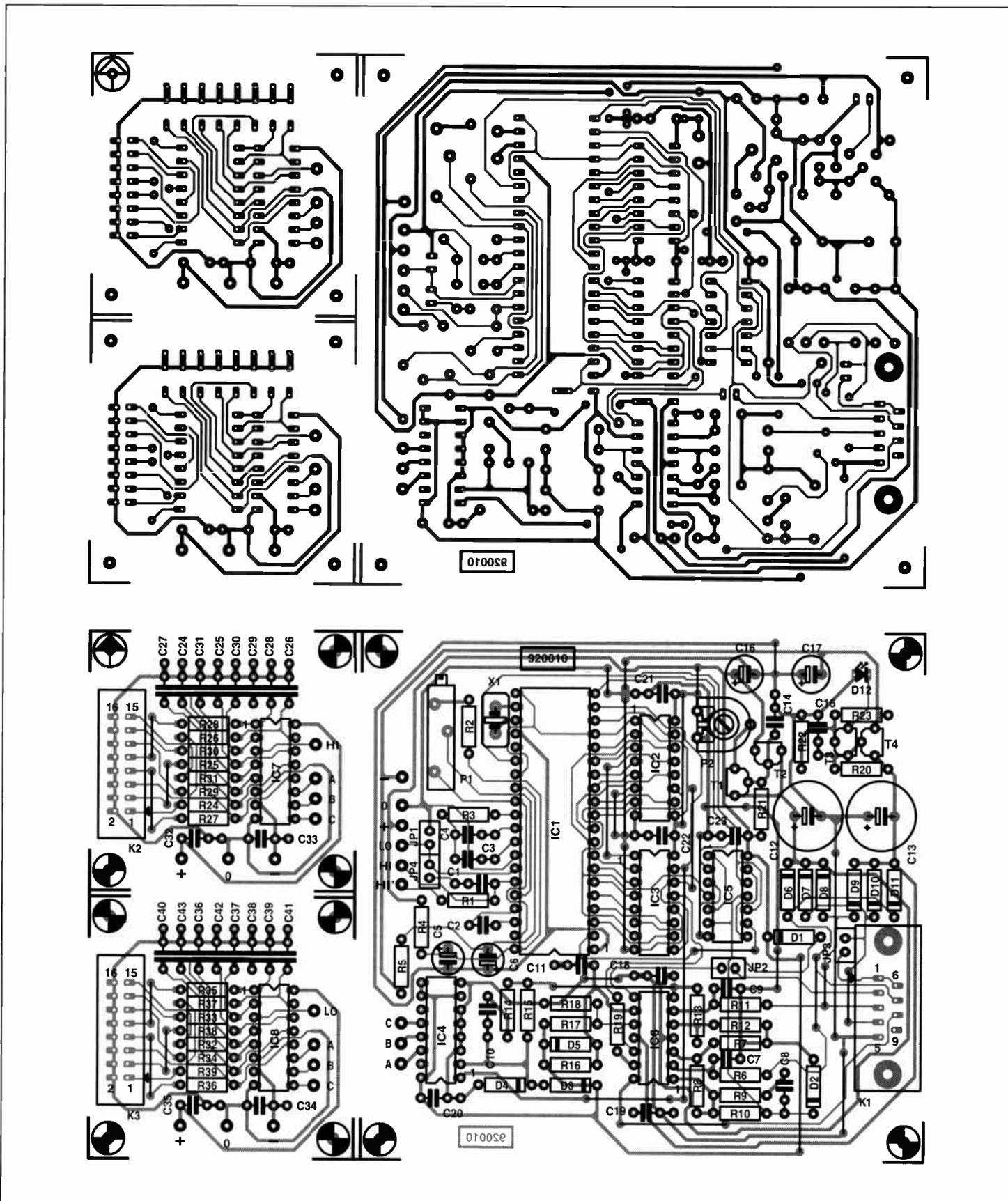
Fig. 6. Single-sided printed circuit board (track layout and component mounting plan) for the AD232.
