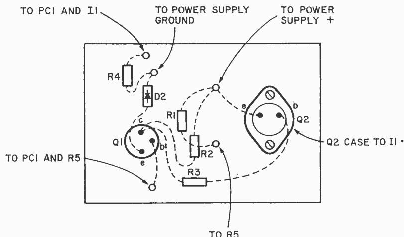
Suggested perf board layout, top view. See schematic for complete wiring.
