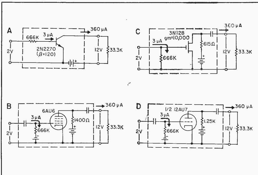
**Bet those techs flipped out when they saw how all four circuits could give the same results. Note identical input and output parameters for each circuit.**
