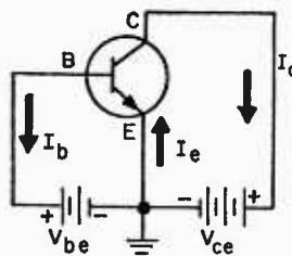
$$\text{CURRENT GAIN} = \frac{\Delta I_c}{\Delta I_b}$$
