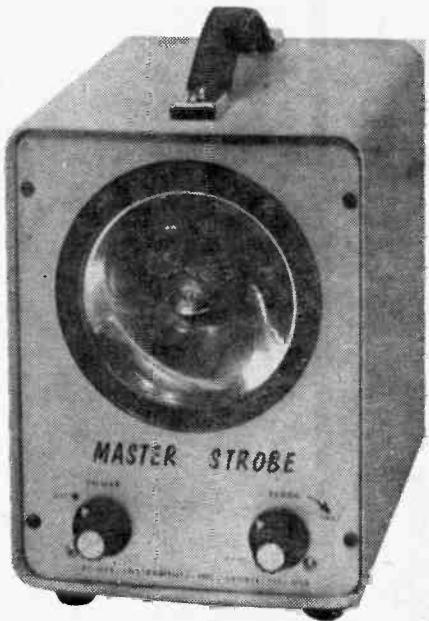
imbalance of wheels, and more. Master Strobe has a range from 400 to 6,000 flashes per minute. Rate of flashes can be controlled manually. A Sync position in the panel allows the unit to be synchronized externally by means of a contactor, voltage source, or Power Instruments photoelectric pickup. For more data, Circle No. 56 on Reader Service Coupon on page 17 or 103.
