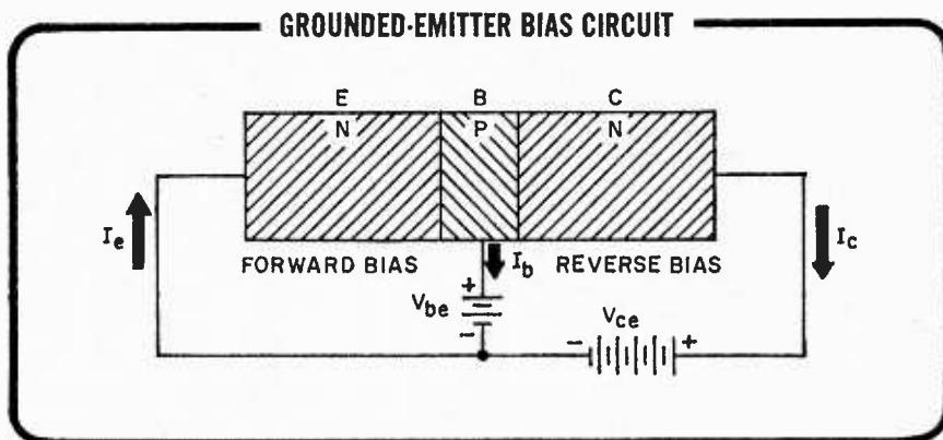
Consider another arrangement of the transistor. This arrangement is similar to the one showing a properly biased NPN transistor. The only difference is that the reverse bias between collector and base is provided by  $V_{ce}$  in series with but opposing  $V_{be}$  ( $V_{ce}$  is large compared to  $V_{be}$ ). This is called a **grounded-emitter** circuit.
