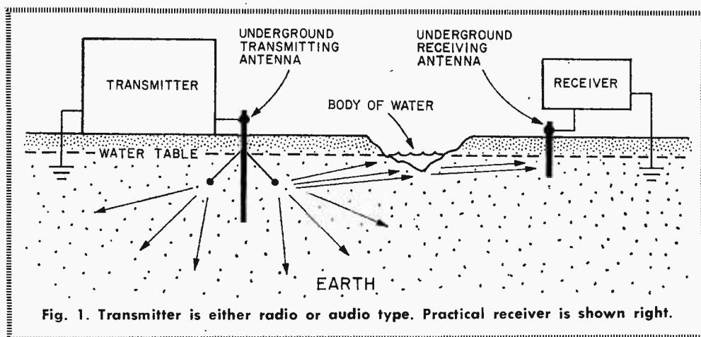
Fig. 1. Transmitter is either radio or audio type. Practical receiver is shown right.
