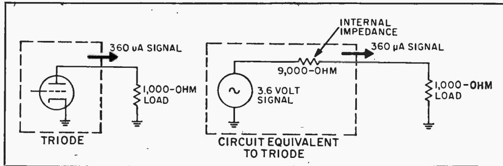
**Characteristic low internal impedance makes triode gain measurable in  $\mu$ u.**
