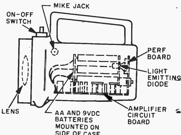
**Photo on page 94 shows inside view of receiver with quick disconnect plug for solar cell separation. X-ray views show suggested parts location in detail. AA batteries in transmitter power LED. 9-volt battery in each unit provides amplifier power.**
