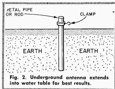
**Fig. 2. Underground antenna extends into water table for best results.**
