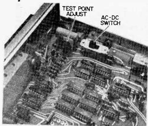
voltage and current is automatically indicated, and the decimal point is automatically located for each range. All ranges are overload protected by a fuse and/or a diode clamp. An overrange indicator shows if the applied voltage or current exceeds the range capability.
