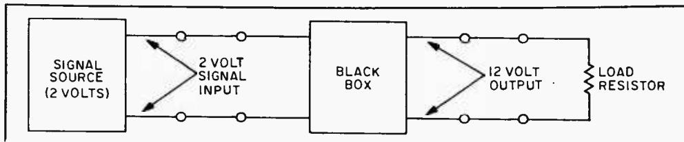
**Black box (slang for an unknown circuit) test set-up for input/output voltage measurements.**
