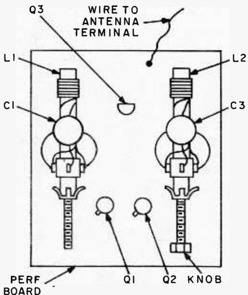
Basic parts layout involves angle brackets for mounting loopsticks. Suggested transistor orientation aids assembly; position Q1 and Q2 emitter leads toward front of board.
