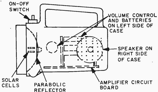
aperture of the lens when the lens is observed several feet distant. Adjust the receiver's solar cells so that the entire reflector takes on the dark color of the cells when observed straight-on. This means that all light striking the reflector will be reflected to the cells.
