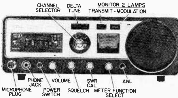
The front panel is packed with goodie features. Digital clock can turn rig on or function as an alarm clock. A single meter serves as an S-meter, relative power RF output meter and as an SWR meter for monitoring.
