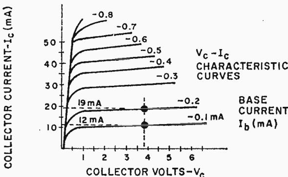
$$\beta = \frac{\Delta I_c}{\Delta I_b} = \frac{19 - 12 \text{ ma}}{0.2 - 0.1 \text{ ma}} = \frac{7 \text{ ma}}{0.1 \text{ ma}} = 70$$
