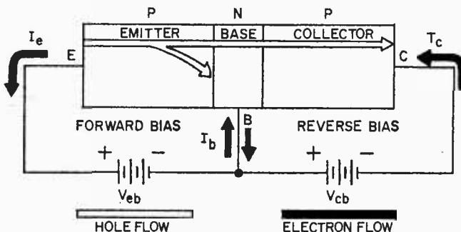
will forward-bias the emitter-base junction. In a similar fashion, a battery whose negative terminal is connected to the P-type collector will reverse-bias the collector-base junction.
