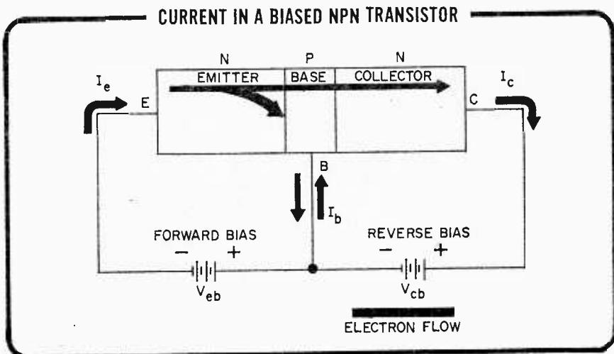
Since the base-collector junction is reverse-biased, very little current should flow through it. This current is produced by leakage due to  $V_{CB}$ .
