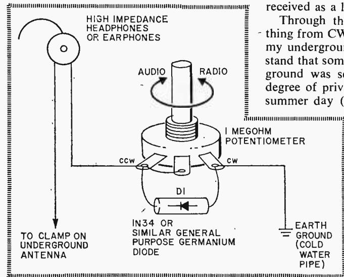
**Fig. 3. Circuit uses 3 parts.**
