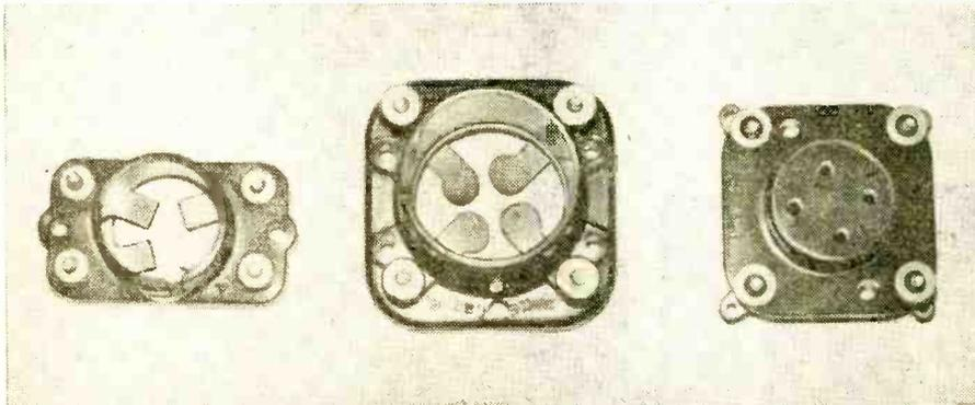
Four-pin tube sockets of very early radio—UV small, UV large, and UX.
