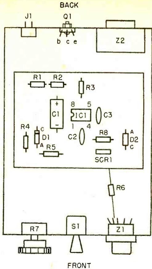
You can follow this layout exactly making point-to-point wiring connections underneath the perf board and to push-in clips. Take extra care to insure that correct polarity is applied.
