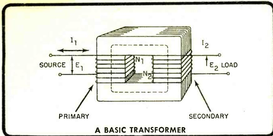
The basic transformer has two windings—primary and secondary—wound on a laminated-iron core. The two windings are insulated from each other and from the core.
