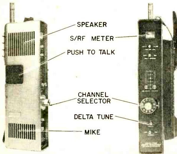
Double view of same T-1000. Use unit as a mobile without the battery pack shown. A 12-volt DC cord is available for mobile operators.
