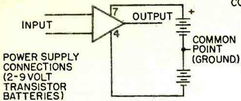
POWER SUPPLY CONNECTIONS (2-9 VOLT TRANSISTOR BATTERIES)
