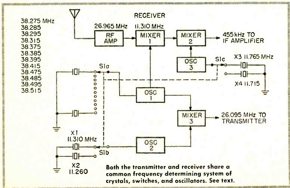
shrinking dollar, some manufacturers now replace the two crystals needed for the receiver (osc. 3) with a fixed-tuned circuit, reducing the total number of crystals to 14. Savings are reflected in a lower transceiver price.
