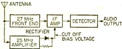
Perhaps the finest form of noise eliminator in CB is the RF-type employing a separate front end at 25 MHz that listens for "noise."
