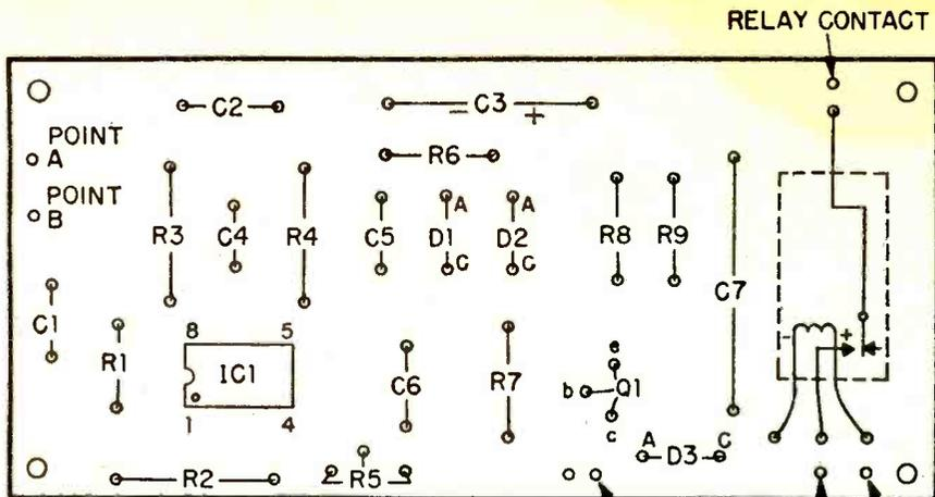
Bigger than life view (above) shows completed PC board with reed relay. Place C7 negative lead in hole nearest diode D3. Hole next to "-battery" is circuit common; connect to ground. See text. The minus side of battery (left) connects to Q1 (e).
