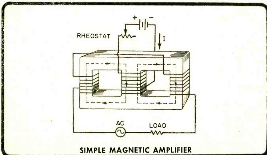
To make a magnetic amplifier, manufacturers wind two different coils on a core similar to the construction of a transformer. But instead of a primary and a secondary, this core has a *control* and a *load* winding.
