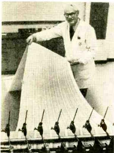
Ball point pen refills are kept drawing concentric circles for their entire writing lives in the pen testing machine. To meet standards, that writing life has got to be long enough for the refill to draw a continuous line of no less than 5,000 feet.
