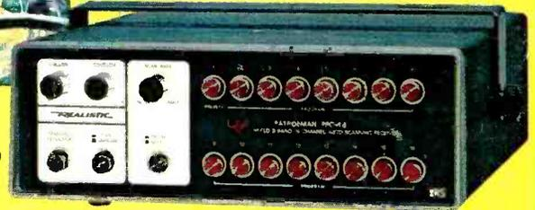
Scans up to 16 crystal-controlled channels, in any combination, on 30-50 and 148-174 MHz VHF and 450-470 MHz UHF. Like 16 radios in one! Lockout buttons and indicator lights for each channel, manual selector, squelch, variable scan rate, scan-delay in/out button, 12 VDC/120 VAC operation, mobile mounting bracket. Requires up to 16 crystals. U.L. listed. #20-165
