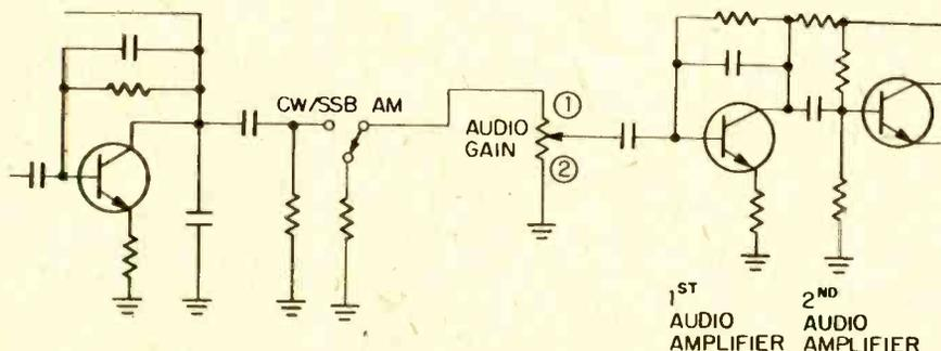
Nearly all of today's new receivers are transistorized. This typical schematic shows your audio take off points. Hook the inner conductor to 1, shield to 2.
