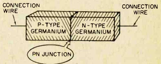
A solid-state diode consists of a section of P-type semiconductor material joined to an N-type section. The activity occurring at the junction of the materials is responsible for the unidirectional property of the diode. The contacting surface is called the **PN junction**.
