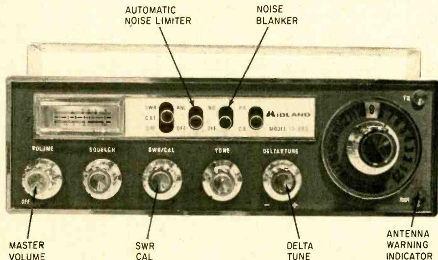
All functions are right up front on the panel, even the SWR calibrate control. The single meter does triple-duty for received signal strength, RF output, and SWR. The small lamp in the lower right hand corner labeled AWI goes on if the SWR rises well above a normal operating value.
