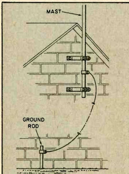
Though few CBERs bother to ground their antenna system, for your own safety the supporting mast should be connected through (at least) No. 8 copper wire to a copper rod driven into the ground. TV supply stores generally stock the ground rods. Grounding the antenna system should be standard practice even if it isn't the highest structure in your neighborhood.
