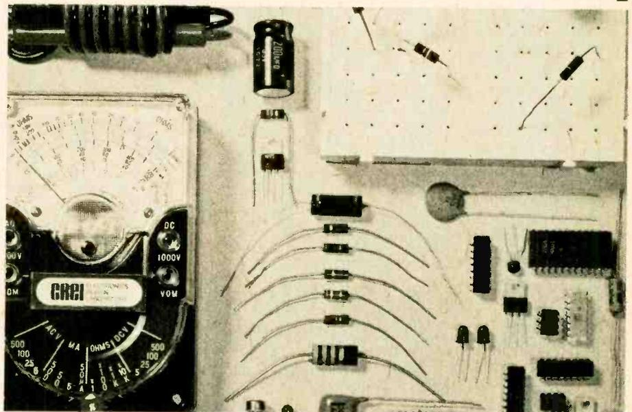
The 20,000-ohm/volt VOM, experimental breadboard, and some of the components supplied with the CREI course with Design Lab option.
