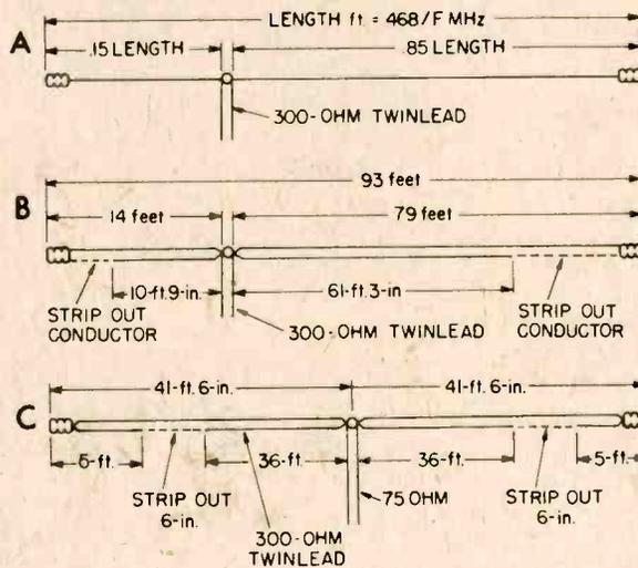
Three porcelain antenna insulators are used for antenna A. One separates each section of the antenna at the point of feedline connection. The other two insulate the antenna ends from the supporting structure. The antenna at B uses 300-ohm twinlead for the transmission line and the antenna elements. Only the ends at the feedline connections are wound together and soldered. Outside ends are separated, with one partially removed as shown. At C the use of 75-ohm line is called for.
