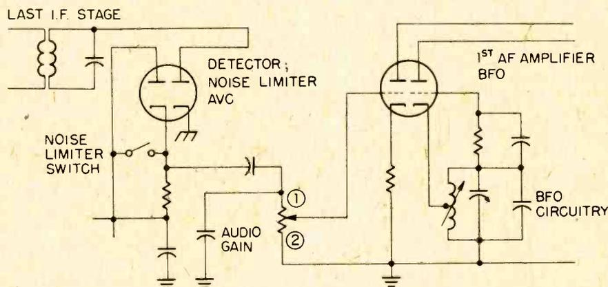
Many tube-type communications receivers are around and in first class shape. If you are still using one of the classics, connect to points 1 and 2 (ground).
