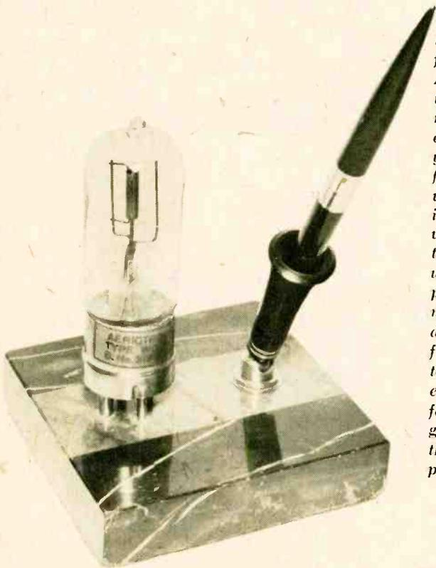
*Here we have the famous Westinghouse Aeriotron (WD-11) triode tube which made a big hit in the early 1920s because you could heat the filament (1.1 volts) with a 1½-volt drycell instead of using a 6-volt storage battery. In this case, the author used a desk pen set purchased at a rummage sale for 50¢, and drilled four small holes for the tube base pins to fit in, and then used epoxy glue to hold it fast. Green felt was glued to the bottom of the marble to protect polished desk surfaces.*
