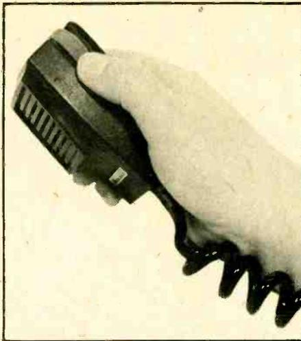
Highlight feature of the Midland 13-883 is the sub-master volume control built right into the microphone, allowing easy adjustment of the received signal's volume level.
