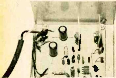
Power switching transistors Q2 and Q3 get slightly warm when operating at maximum supply voltage due, primarily, to the high 25-kHz switching frequency. Such transistors become less efficient as their maximum operating frequency is approached. A small heat sink made from a piece of aluminum which is fastened to the metal side of a transistor will serve adequately to cool the transistors.
