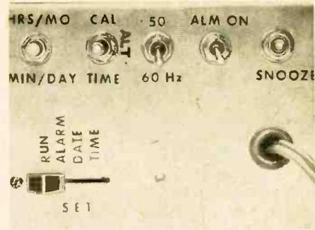
“Set” switch S1 (see the schematic) tells the clock which of its three functions you want to adjust with the left hand switch (S2). Just hold S2 in the up position to set hours or months; hold it down to adjust minutes or day of the month.
