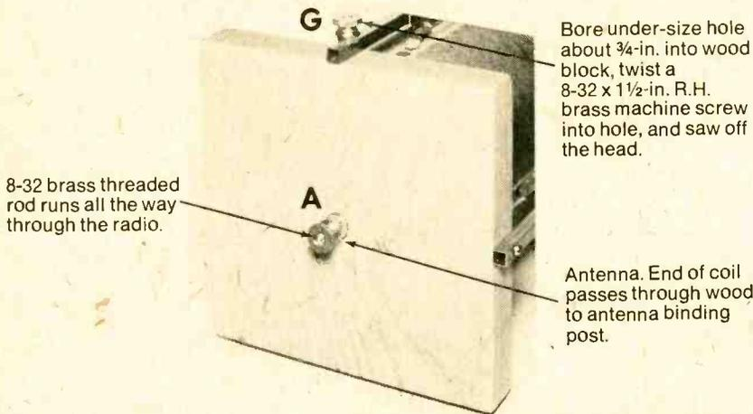
**A**SK JUST about any radio old-timer, including this writer, and he will probably tell you that his first radio was a home-brew slide tuning coil wound on an oatmeal box, a cat whisker and galena crystal detector, and a pair of earphones. This picture story shows how to make such a radio, and it looks much like the writer's first radio built not long after World War I.
