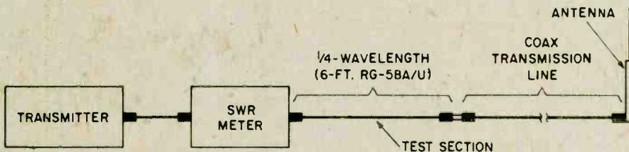
If there is substantial change in SWR readings when a 1/4-wavelength section of coaxial cable is installed between an SWR meter and the transmission line, the antenna is not 50 ohms. If the reading is the same, everything is well matched.
