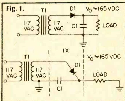
half-wave power supply. This simple circuit forms the basis for a complete family of voltage multiplying circuits, and is shown both in the standard schematic format and a simplified form that will facilitate the development of additional multiplier circuits.
