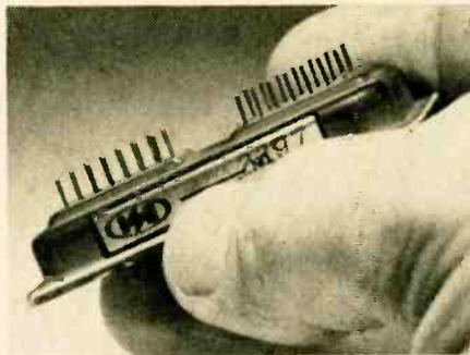
Just a pair of 14-pin dual-in-line IC sockets are needed to connect this compact display with the circuit board. Display is actually an 8-digit device originally for calculator use. Here we blank the third and fifth digits to separate hours, minutes, and seconds.
