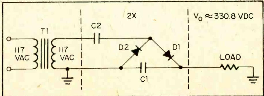
**Double Up.** By adding a second diode and capacitor combination to the basic half-wave circuit, as shown in Fig. 2, it becomes a voltage doubler circuit—effectively multiplying the peak value of the input voltage by two. Notice that the new diode, D2, and capacitor, C2, are connected in series (cascade) with the original diode, D1, and capacitor, C1, and are between them and the transformer, T1.
