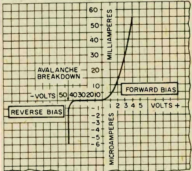
The reverse-bias region is to the left of the origin. Remember that the diode will not conduct in the reverse direction. This is true on the graph up to almost 40 volts of reverse bias. Above this value, small currents in the order of a few microamps start to flow. This current flow is due to the leakage. When the reverse bias reaches about 45 volts there is a sharp increase in reverse current. This is called **avalanche breakdown**.
