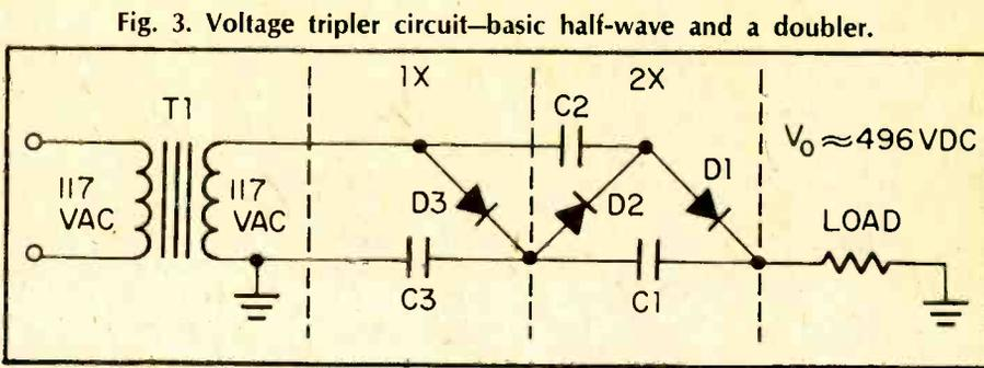
with a load is a function of the input voltage, the source impedance, the capacitor values, the forward voltage drop of the diodes, and the frequency of the input voltage. By assuming that the diodes are ideal (no voltage drop across them in the forward direction) and if the values of all capacitors are made equal (generally the best way to go) the approximate output voltage from a given circuit can be calculated using
