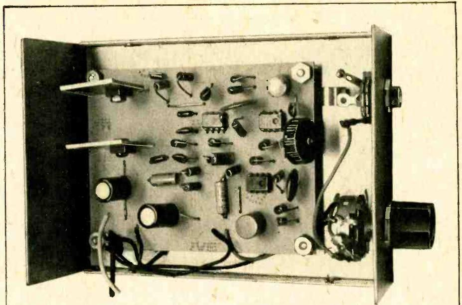
The minus power lead, speaker common lead, and PC board "common" all connect to a solder lug mounted to the case or PC board mounting assembly as shown here.
