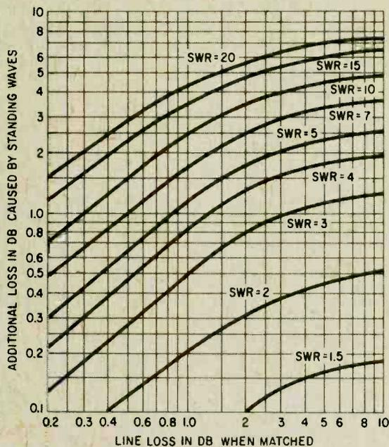
All transmission lines have an inherent minimum line loss when perfectly matched to the antenna. The greater the inherent "matched" line loss, the greater the additional loss caused by the SWR, and the greater the SWR, the greater the additional SWR loss. An SWR of 2:1 should be the maximum acceptable value for CB.
