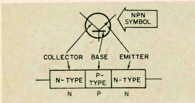
called a **junction transistor**. The symbol for this type of transistor showing the three elements (emitter, base, and collector) is shown. The three elements correspond to the cathode, grid, and plate, respectively, of a vacuum-tube triode.
