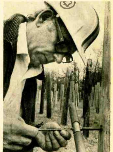
In this unusual setting, a timber product engineer tests his telephone pole forest for the longevity of the variously-treated poles. The test bore he is performing above will tell him how well the wood preservatives have been impregnated in the pole.
