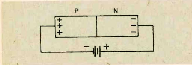
the positive battery voltage attracts free electrons in the N-type semiconductor away from the junction. The result is an absence of current flow because electrons and holes are not at the junction area and cannot, therefore, combine.
