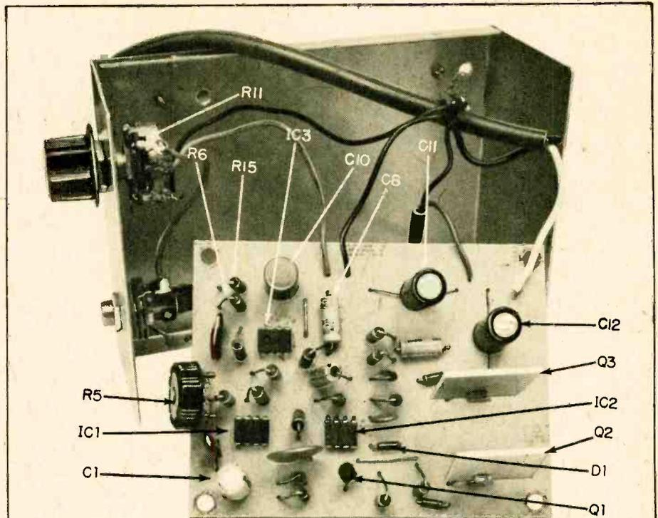
This X-ray view shows where to place parts on the circuit board. The view is of the top of the PC board where all parts but R11 fit.
