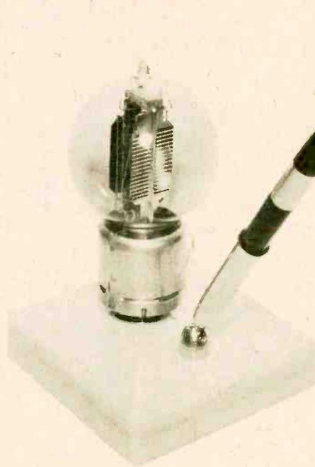
*Here is a Western Electric 216-A triode tube mounted on a block of onyx purchased at a sale for a few cents. The four pins on the bottom of the tube base were soldered to a small brass disc and then the brass disc was cemented to the onyx block with epoxy glue. The ball joint of the pen funnel was also glued to the onyx block.*
