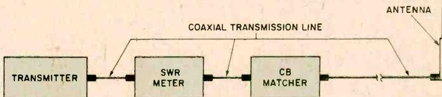
After the antenna system is tuned, this is the correct instrument arrangement for adjusting an antenna tuner (CB matcher). Adjust the matcher for minimum SWR between the transmitter and matcher, coincident with maximum forward power. Best results are attained if the transmission line is 12 feet or an exact multiple of twelve feet such as 24, 36, etc. And remember, a matcher cannot improve what is already an excellent antenna system. All coaxial transmission cable is 50 ohm.
