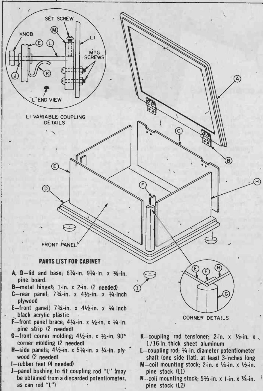
cardboard discs cemented onto the back of small plastic knobs. Fahnestock clips can be used in place of the terminals (J1, J2) on our model, and also in place of J3 for the headphone connections. Install the front panel on the cabinet and make sure that the spiderweb coils do not touch the top lid or bottom of the cabinet.
