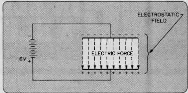
equals the battery voltage. The potential of the plate having an excess of electrons will be negative. The other plate, being deficient in electrons, will be positive.
