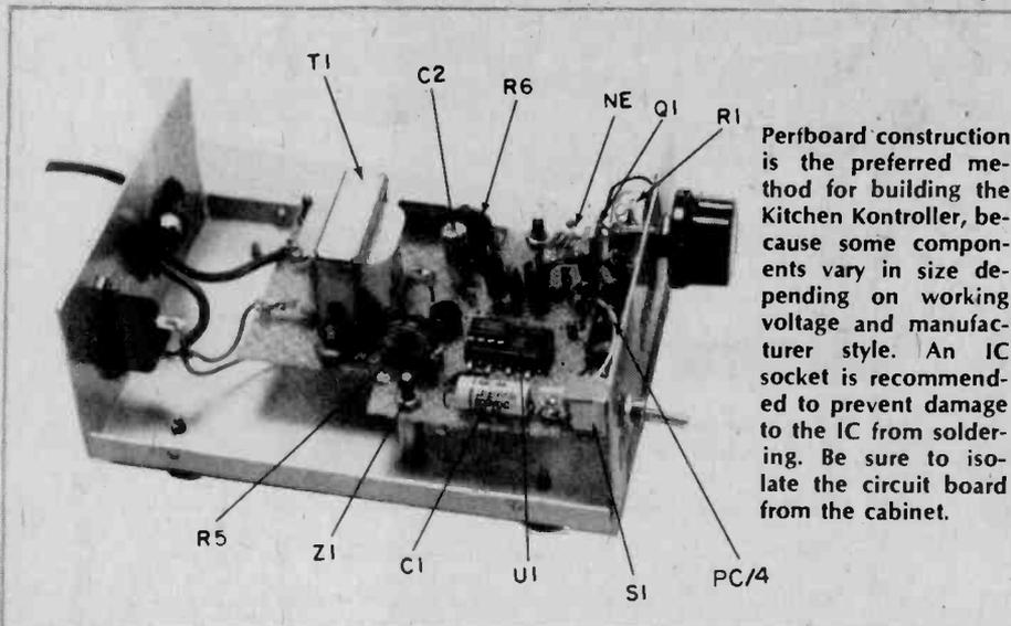
Perfboard construction is the preferred method for building the Kitchen Kontroller, because some components vary in size depending on working voltage and manufacturer style. An IC socket is recommended to prevent damage to the IC from soldering. Be sure to isolate the circuit board from the cabinet.
