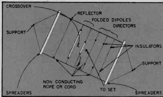
FIGURE 3. DIPOLE WIRES AND PLASTIC SUPPORT PIPE FOR ELEMENT 1.
