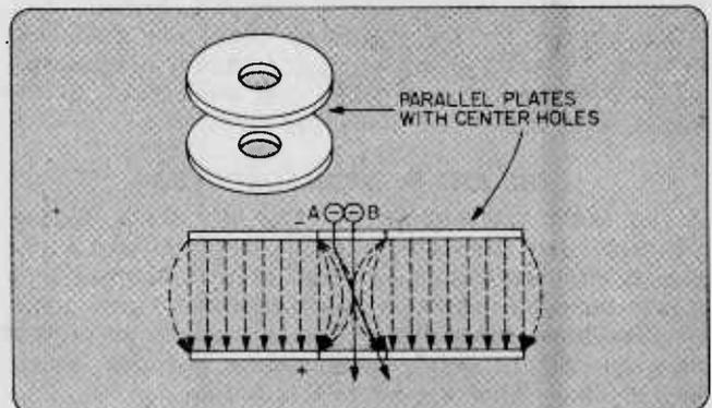
must pass through them. Also suppose the larger cylinder has a more positive charge. The distribution of the lines of force would look like the next illustration.
