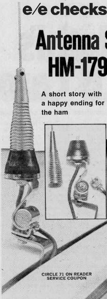
perform electronically in the same manner? With the SWR meter in line, it was an easy matter to check the broadbandness of the antenna by dialing up frequencies on the synthesizer at each extreme of the band. At 146 MHz, the frequency to which we had cut the whip, the SWR was not enough above 1:1 to budge the needle on the meter. In fact, at both 144.000 and again at 147.995, the SWR never exceeded 1.4:1. That, friends, is called "flat."
