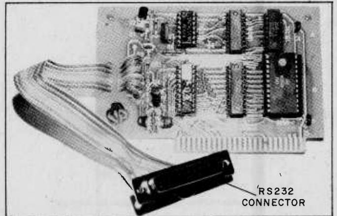
The Communications Card from Apple will, through use of a modem, allow an Apple computer to be utilized as an intelligent terminal. The "Com Card" gives the Apple an industry-standard RS232 output port. Circle 64 on reader coupon for information.
