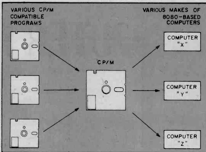
The CP/M operating system can be modified slightly to run on any 8080-based micro-computer. Applications programs can then be written to conform to CP/M's requirements rather than those of the computer. Thus, any computer running CP/M can use any of the thousands of independently produced programs written to run under that operating system.
