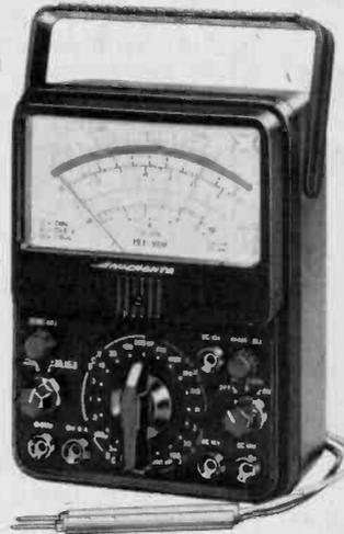
High-accuracy 25  $\mu$ A meter with single-knob range selector measures DC Volts: 0-3-1-3-10-30-100-300-1000 at 10 Megohms. AC Volts: 0-3-30-100-300-1000 at 10 k $\Omega$  per volt. DC Current: 0-100  $\mu$ A, 3-30-300 mA, 10A. Resistance: Rx1, Rx10, Rx1000, Rx10k, Rx1M (10 ohms center scale). d3: -20 to +62 in 5 ranges. Accuracy:  $\pm$ 3% DC,  $\pm$ 4% AC. 7x5 $\frac{1}{2}$ x3 $\frac{1}{8}$ " overall. With leads, test probes, batteries. 22-208 Sale 39.95
