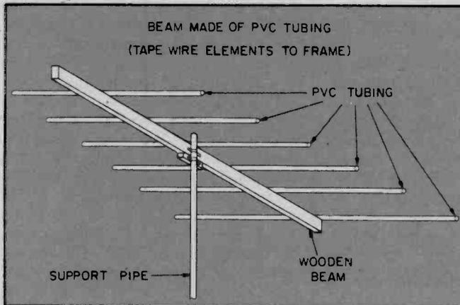
The frame for the wire beam is simple and cheap to build. The shaft can be sturdy wood or metal. Use U-bolts to secure a two-by-four to the mast and clamp the PVC, antenna element supports to the two-by-four. If the support pipe is too high above its base then you should add guy lines to keep the antenna vertical and rigid.
