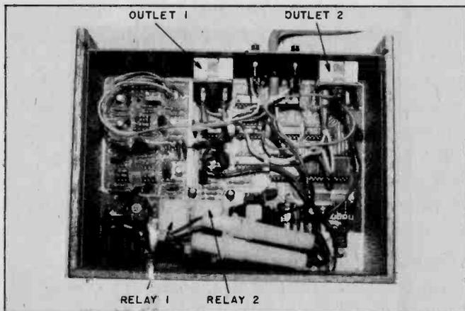
Mountain Hardware's Remote unit is another, easy to assemble project, owing to the scrupulously detailed instructions. Each remote will control one or two appliances of up to 500-watts each through two relay-switched AC outlets located on the back side.
