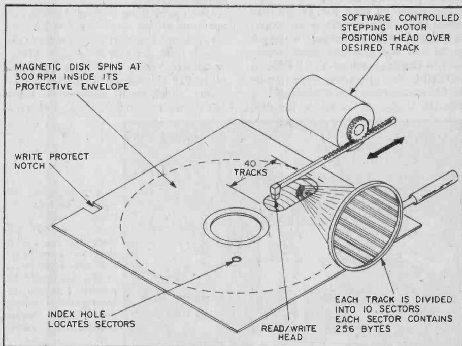
There are many different sizes and types of floppy disks but they all look much like the one in this diagram. The disk tracks are not visible lines but rather sectors of a single magnetic coating. The read/write head is positioned by a stepping motor. Some systems have read/write heads for both sides of the disk. Index hole marks the first sector.
