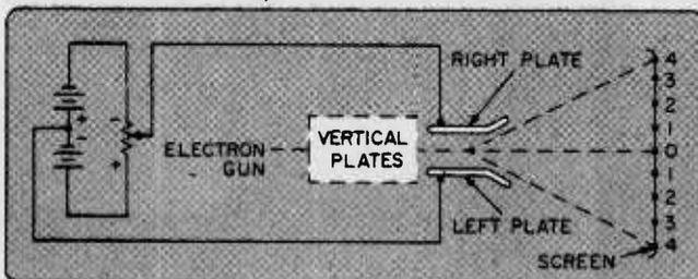
The beam returns to the zero position when the potential difference between the plates again becomes zero. Moving the arm toward the other end of the resistance will cause the left plate to become more positive than the right. The direction of the electric force reverses, and the beam moves from 0 through 4'. If the movement of the potentiometer arm is at a linear (uniform) rate, the beam will move at a steady rate.
