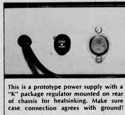
meter should indicate the desired output voltage. After a few minutes, carefully feel the regulator IC's flange. It should be no hotter than hot tap water. If touching the regulator case is painful, use a larger heat-sink to cool it down.
