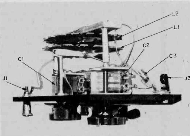
Follow the exploded parts diagram on the next page for assembly of the mounts for L1 and L2. The picture at left gives a top view of the assembly, while the drawing gives a side view. If your variable capacitor doesn't have a tapped hole for the spacer screw, drill an 1/8-inch hole in its side, and use self-tapping screw.
