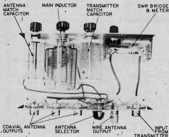
The tight spacing of the interior components is the reason for the low power rating. When more than 250-watts output is used, some arcing may occur. This is characteristic of all miniaturized antenna tuners. 4-antenna capacity of the SST allows you to put up plenty of experimental antennas for comparison tests. Circle number 75 on reader service coupon.
