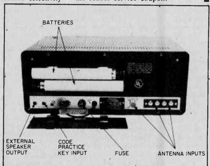
The rear apron has appropriate antenna connectors for just about any type of antenna you might possibly wish to utilize. If you are contemplating portable operation, just slip a few batteries into the convenient holder, roll up your antenna, and hit the road!
