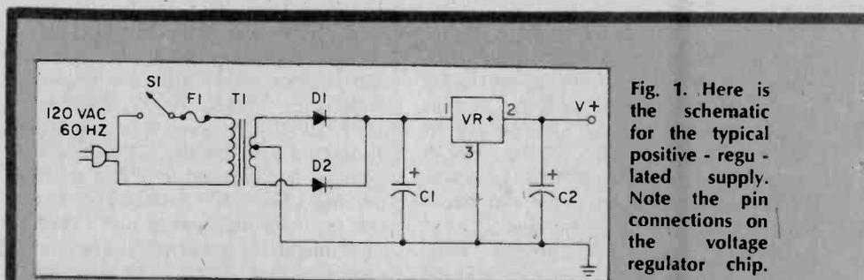
Fig. 1. Here is the schematic for the typical positive-regulated supply. Note the pin connections on the voltage regulator chip.
