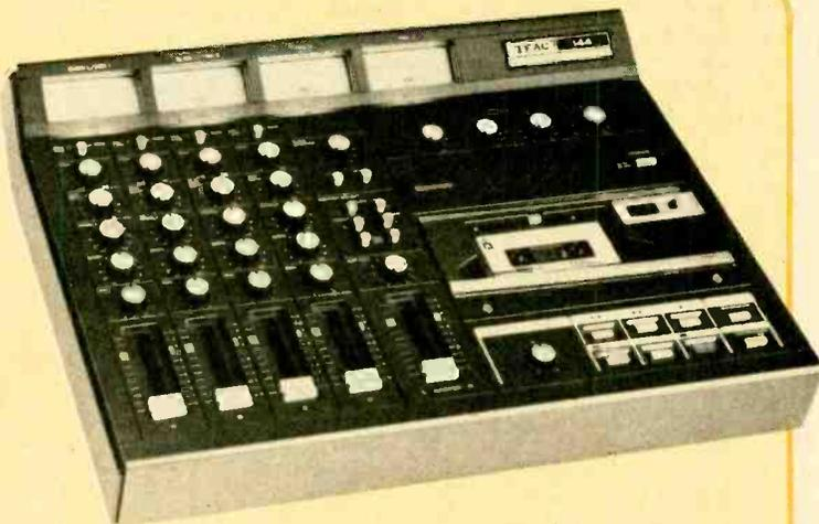
A compact, ready-to-play speaker system, Altec-Lansing's model 9842 (left) features a 12-inch woofer and complimentary 2-way compression driver/horn. Available with or without grille in two cabinet styles, each model has electronic overload protection. Circle number 76. TEAC's model 144 mixer/recorder (above) handles 4, frequency-equalized channels, and its built-in 4-track cassette recorder allows mix down right in the same unit, simplifying dubbing chores. Circle 74 on service coupon.
