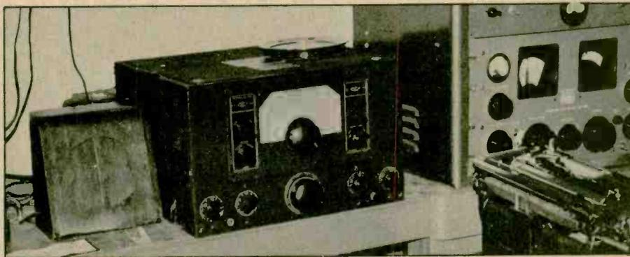
This National Radio Corporation long wave receiver dates from the 1930s. Sets like this one were used aboard ships and at coast stations to monitor distress calls and ship-to-ship traffic on the low-frequency bands below 500 Kilohertz reserved for these purposes.
