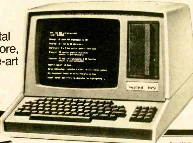
EXCLUSIVE! TRAIN WITH THE NEW H89 NTS/HEATH ALL-IN-ONE MICROCOMPUTER! NTS's Master Course in Microcomputers now includes this remarkable new desk-top computer. Features floppy disk storage, "smart" video terminal (terminal has its own microprocessor, doesn't share one with computer as do most desk models), two Z80 microprocessors, 16K RAM expandable to 48K, professional keyboard.
