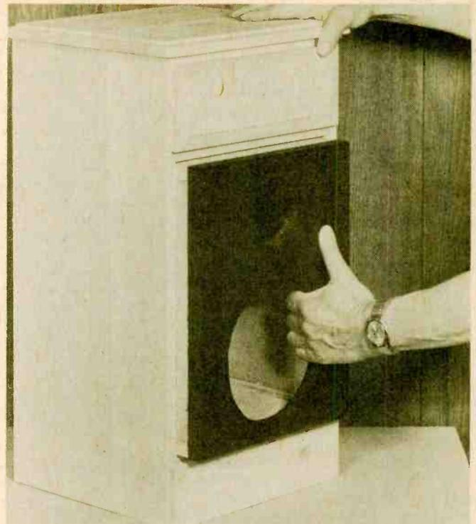
Properly assembled, the speaker box should fit inside the opening in the night table with no space at sides.
