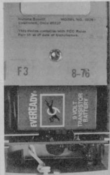
The main body of each transmitter is easily removed from the wall. A 9-volt battery can be quickly and easily replaced.
