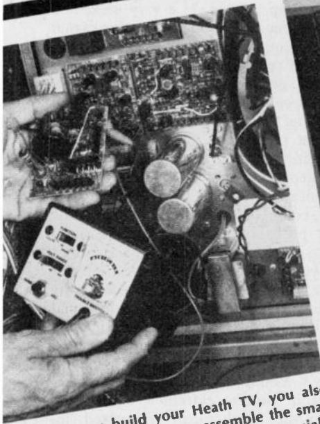
The four boards for the optional programmer attach to the inside of a door on the pull-out section of the chassis. Pre-wired harnesses plug into the individual PC boards. The top bank of pushbuttons (left) are for programming the system.
