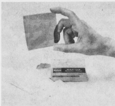
Kodak color printing filters. Typical filter designation CP20Y means color filter with a .20 density; the color is yellow.
