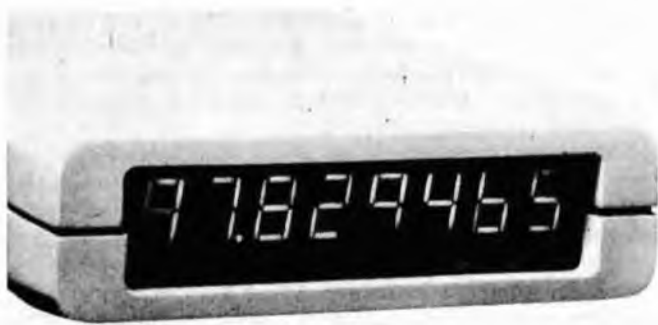
The MAX 100 from Global Specialties Corp. is a portable eight digit counter for field or lab use. Range is 20 Hz to 100 MHz. Suggested retail is $149. Circle 64 on Readers Service Card.
