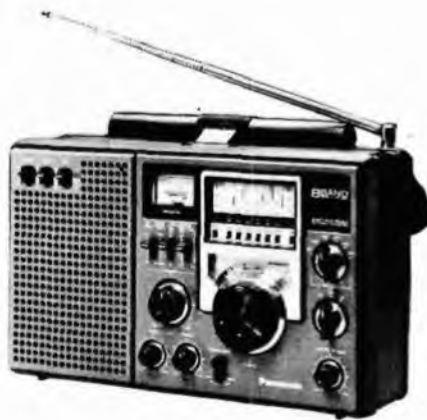
CIRCLE 78 ON READER SERVICE COUPON Panasonic's RF-2200 is an excellent example of a portable, general coverage SW receiver. The front end is a dual conversion type.
