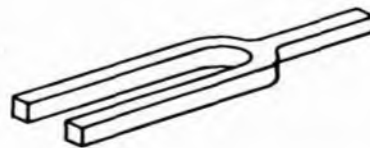
Fig. 3. The geometry of the tuning fork produces a continuous pure tone for a long time when struck gently. It is favored by piano tuners as a convenient way to carry a source of accurately-known tone or pitch.
