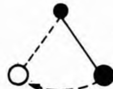
Fig. 1. A long pendulum swings at a rate determined by its length and weight at the end of the arm. To experiment at home, the arm should be made of light thread (no weight) and a small heavy mass (all the weight concentrated at one point).
