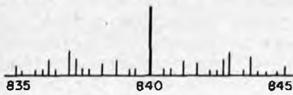
Fig. 6—Complex audio modulating signals generate complex sideband frequencies.
