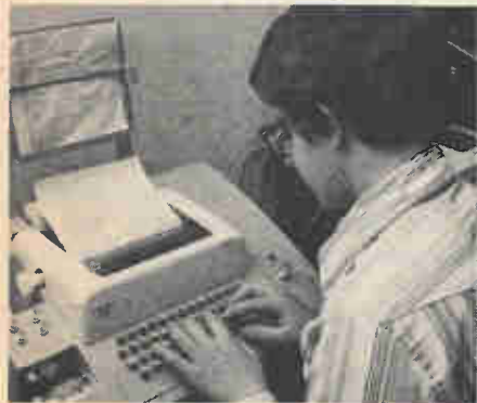
Here it is—the standard of reference for many time-share and personal computer installations. This model 33 teletype is used whenever hard copy, a written record, is required. The model pictured is an ASR—Automatic Send and Receive. Visible to the left is the paper tape punch and reader.
