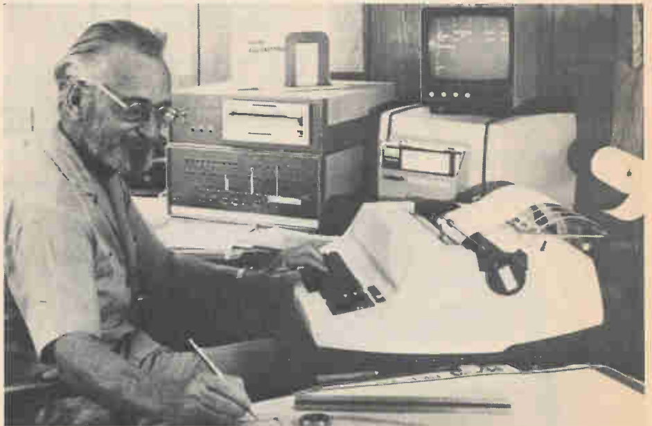
This computer hobbyist, Jay Moss of California, started off with a basic Altair microcomputer. He demonstrates how one can expand a system well beyond its original intentions. With a modified-Selectric printer, floppy discs and more he soon discovered the computer's capitalistic tendencies after using it in his plumbing contracting business.
