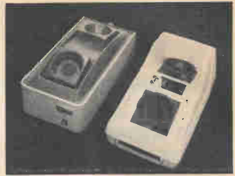
Here, shown in size relationship to each other, are two forms used for data storage; a mini-floppy disc, and a data cassette.
