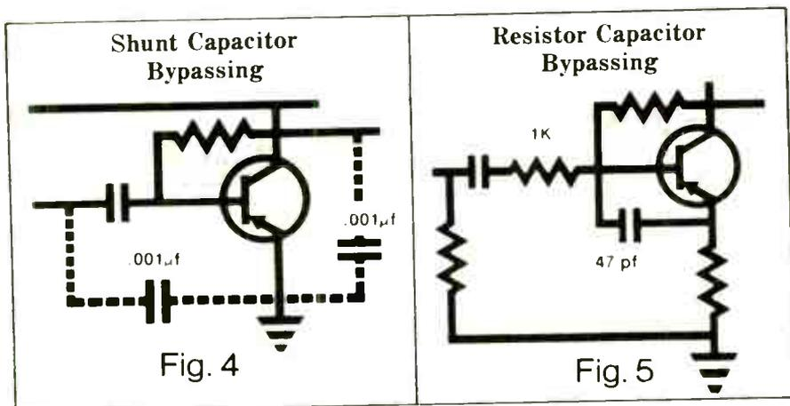
Leads should be kept as short as possible especially with bypass capacitors. The lead length determines the resonant frequency, and therefore, the effectiveness of bypassing. Bypassing directly to the emitter is often more effective.
