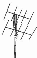
several different directions are received, and it can be obtained as a kit which clamps to an existing TV mast. To complete the installation, a length of 300-ohm flat lead-in is used to connect the antenna to the FM receiver.
