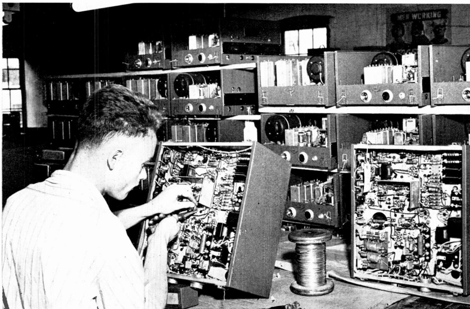
FIG. 5, THE 9TH STAGE BRINGS THE SETS ALMOST TO COMPLETION. DESPITE COMPLICATED CIRCUITS, WIRING ERRORS ARE VERY RARE
