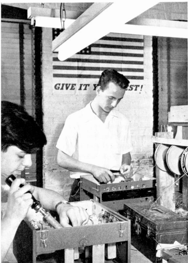
FIG. 3, LEFT, 3RD AND 4TH STAGES. FIG. 4, RIGHT, PRE-FORMED WIRING HARNESS SIMPLIFIES WIRING AT THE 5TH ASSEMBLY STAGE
