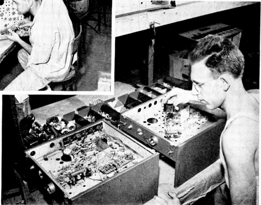
FIG. 1, ABOVE, THE FIRST ASSEMBLY STAGE. AT THE LEFT IS THE MODEL SET WITH ALL PARTS MOUNTED THAT ARE PUT ON BY THE OPERATOR AT THIS POSITION. MODEL SETS AT EACH STAGE SERVE TO MAINTAIN STANDARDS OF WORKMANSHIP
