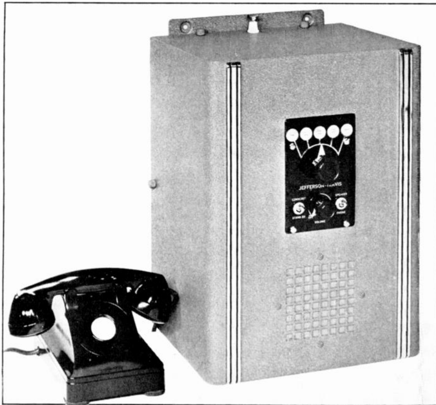
FIG. 1. THIS 18-WATT UNIT OPERATES ON FIVE CRYSTAL-CONTROLLED FREQUENCIES
