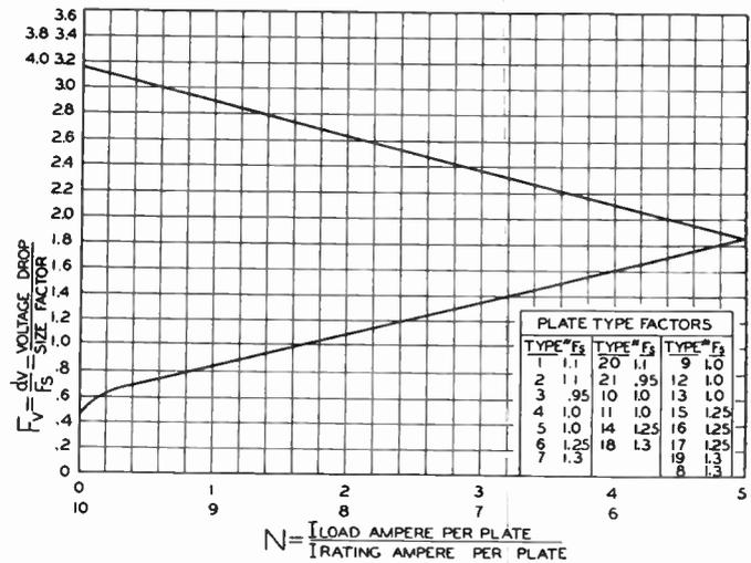
FIG. 9. CHARACTERISTIC ILLUSTRATING RELATION OF  $F_v$  AND  $N$  FOR DIRECT CURRENT AND BLOCKING CIRCUIT APPLICATIONS
