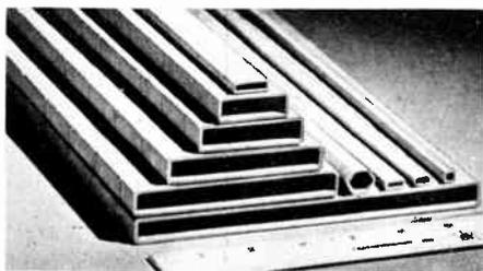
**Paper Tubes:** Of Kraft paper, fish paper, red rope, acetate, or combination materials, with tolerances to .002 in., are being produced by Paramount Paper Tube Co., Glasgow Avenue, Chicago. Sizes range from 3/16 to 4 ins. square, or in rectangular cross section.
