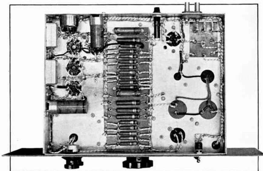
FIG. 2. UNDER SIDE OF OSCILLATOR CHASSIS SHOWS WIRING CENTERED AROUND THE RESISTOR MOUNTING BOARD
