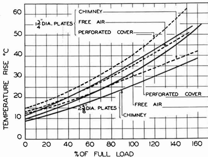
FIG. 2. CHARACTERISTICS OF TWO SELENIUM RECTIFIERS UNDER THREE DIFFERENT COOLING CONDITIONS OF OPERATION
