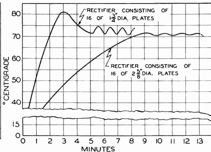
FIG. 4. TIME-TEMPERATURE CHARACTERISTICS, ILLUSTRATING THE PERFORMANCE OF RECTIFIERS WITH BI-METAL STRIPS
