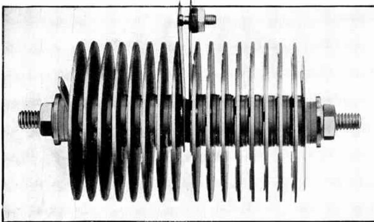
FIG. 3. TWO HALF-WAVE RECTIFIERS FOR OPERATING MAGNETS IN ACCOUNTING MACHINE
