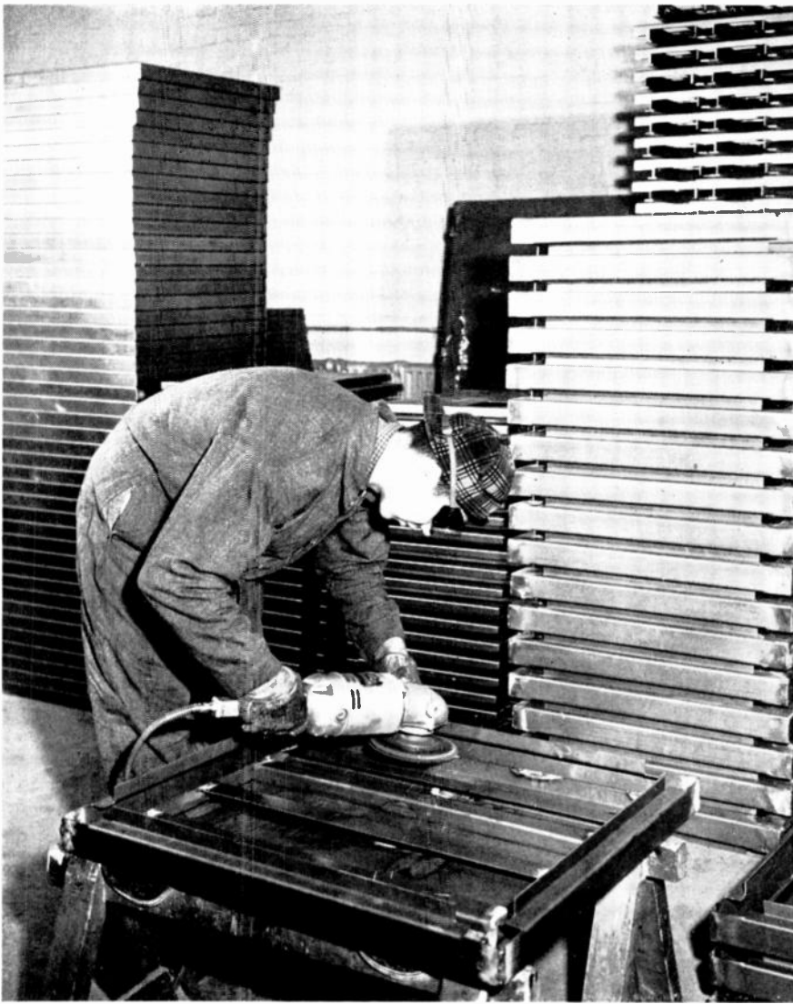
FIG. 5, BELOW: ARC WELDING IS USED TO JOIN THE FRAME MEMBERS. FIG. 6, ABOVE: WELDED JOINTS ARE SMOOTHED BY A SANDER
