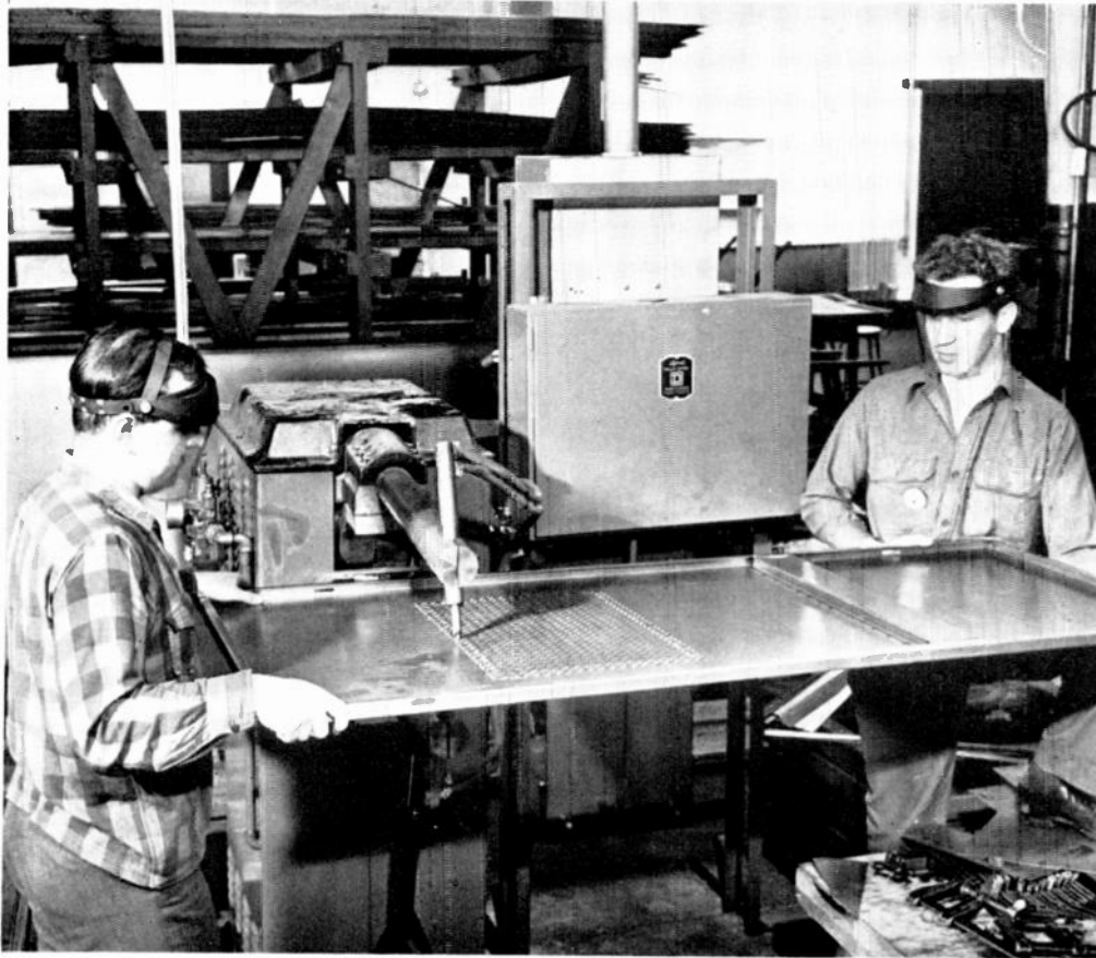
FIG. 8. SPOT WELDING THE VENTILATING SCREEN ON A TRANSMITTER DOOR
