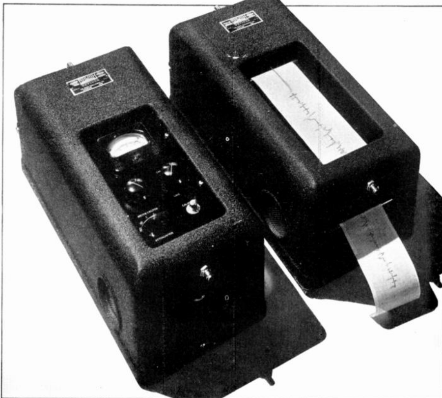
FIG. 3. SINGLE-PEN OSCILLOGRAPH WITH THE ASSOCIATED VACUUM TUBE AMPLIFIER
