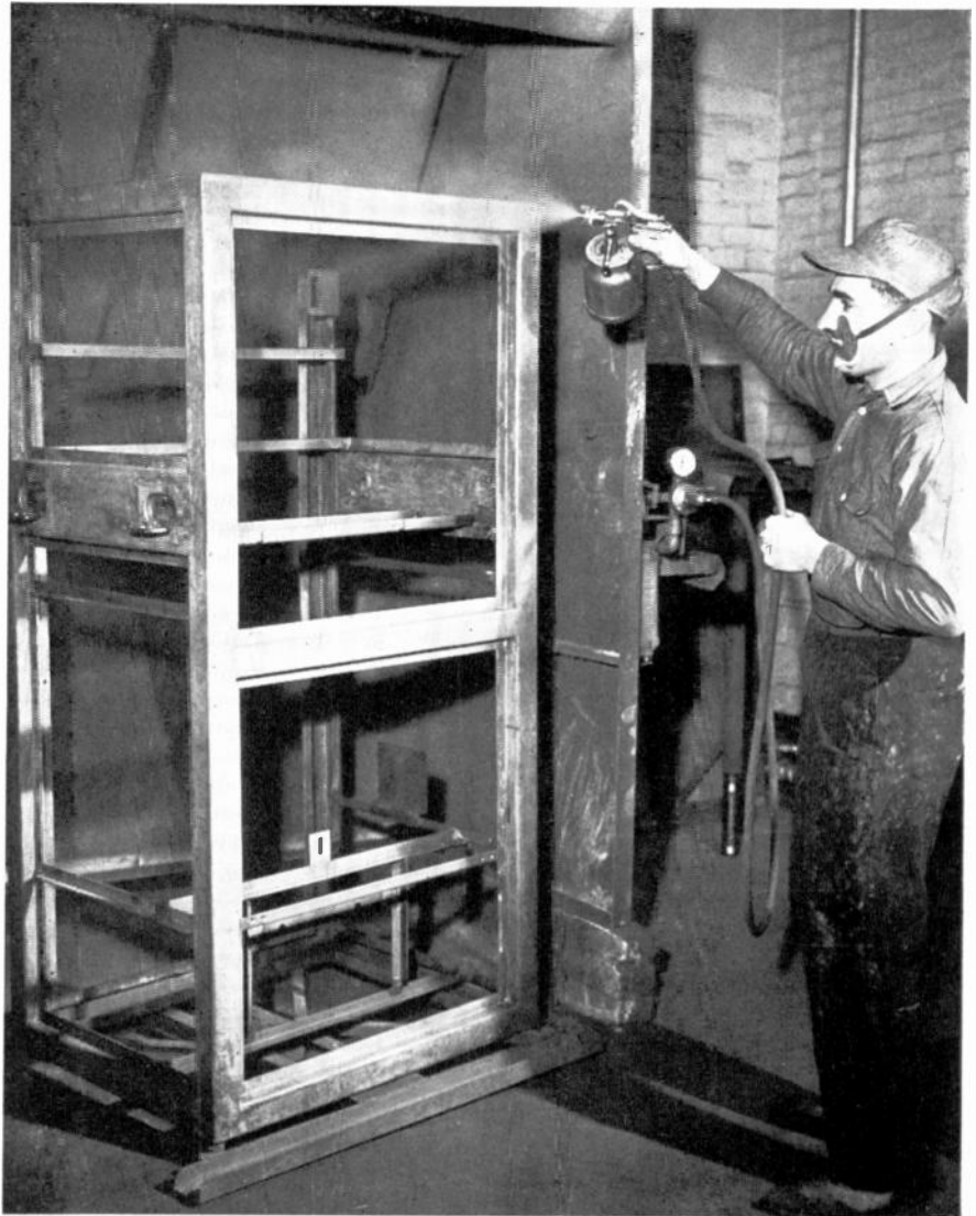
FIG. 4, BELOW: PUNCHING HOLES IN A STEEL PANEL. FIG. 7, ABOVE: SPRAYING ZINC CHROMATE ON A COMPLETED TRANSMITTER FRAME
