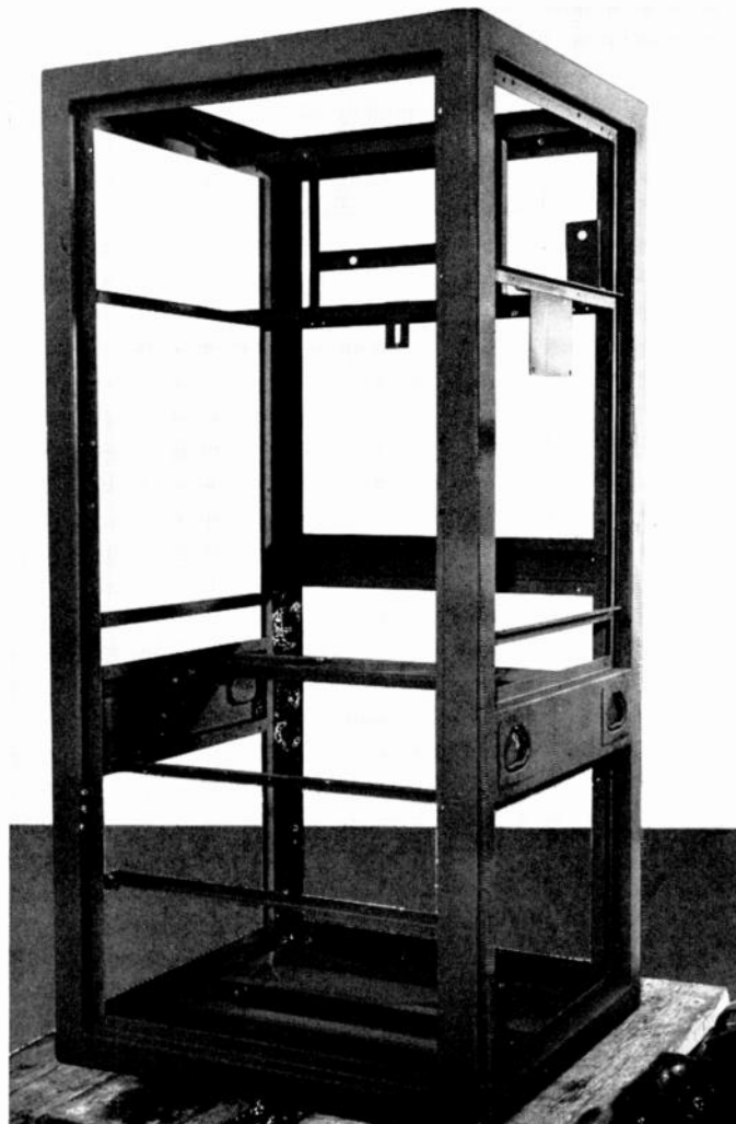
FIG. 1. WELDED STEEL TRANSMITTER FRAME COMBINES MINIMUM WEIGHT WITH GREAT RIGIDITY REQUIRED FOR MODERN EQUIPMENT
