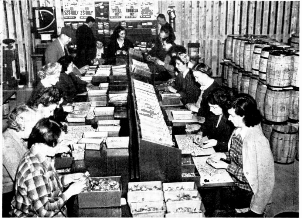
FIG. 2: WOMEN SORTERS RECOVER MANY SMALL PARTS WHICH ARE GATHERED UP BY SWEEPERS, ALONG WITH TONS AND TONS OF NUTS, SCREWS, WASHERS, AND RIVETS. IN MANY RADIO PLANTS, THE METHODS USED BY REPUBLIC CAN BE ADOPTED
