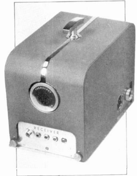
FIG. 1. 6-VOLT MOBILE RECEIVER. A SIMILAR SET, OPERATING ON AC, IS USED FOR MAIN STATIONS
