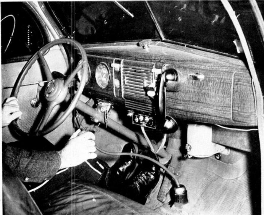
FIG. 4. DASHBOARD CONTROLS OF THE FM LINK 3-WAY CAR INSTALLATION. THE EXTENSIBLE HANDSET CORD IS KEPT AWAY FROM THE DRIVER'S FEET BY THE USE OF ELASTIC CONSTRUCTION
