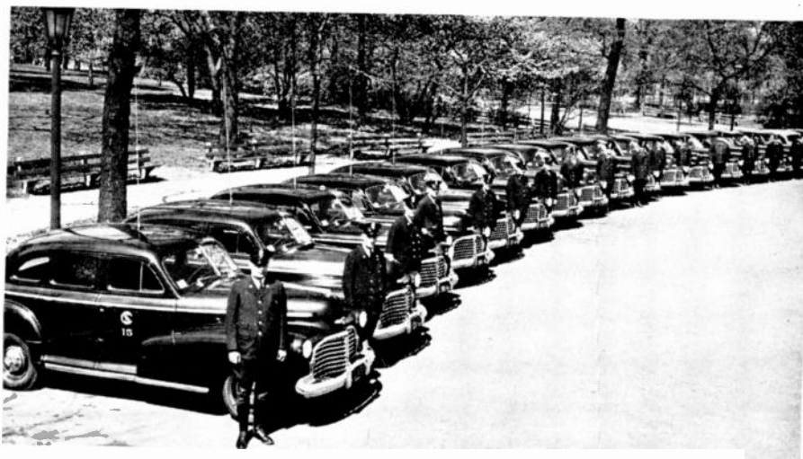
FM-EQUIPPED SERVICE CARS OF THE CHICAGO SURFACE LINES ARE ROUTED FROM HEADQUARTERS BY TWO-WAY COMMUNICATIONS TO SPEED HANDLING OF EMERGENCIES. MAIN STATION AND CARS USE MOTOROLA EQUIPMENT
