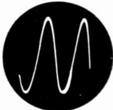
Sine waves of a tuning fork, A-440 cycles per second. Note the pure wave form absolutely devoid of harmonics. If secondary waves are superimposed on the fundamental wave, we have the harmonics or overtones which distinguish voices or instruments.
