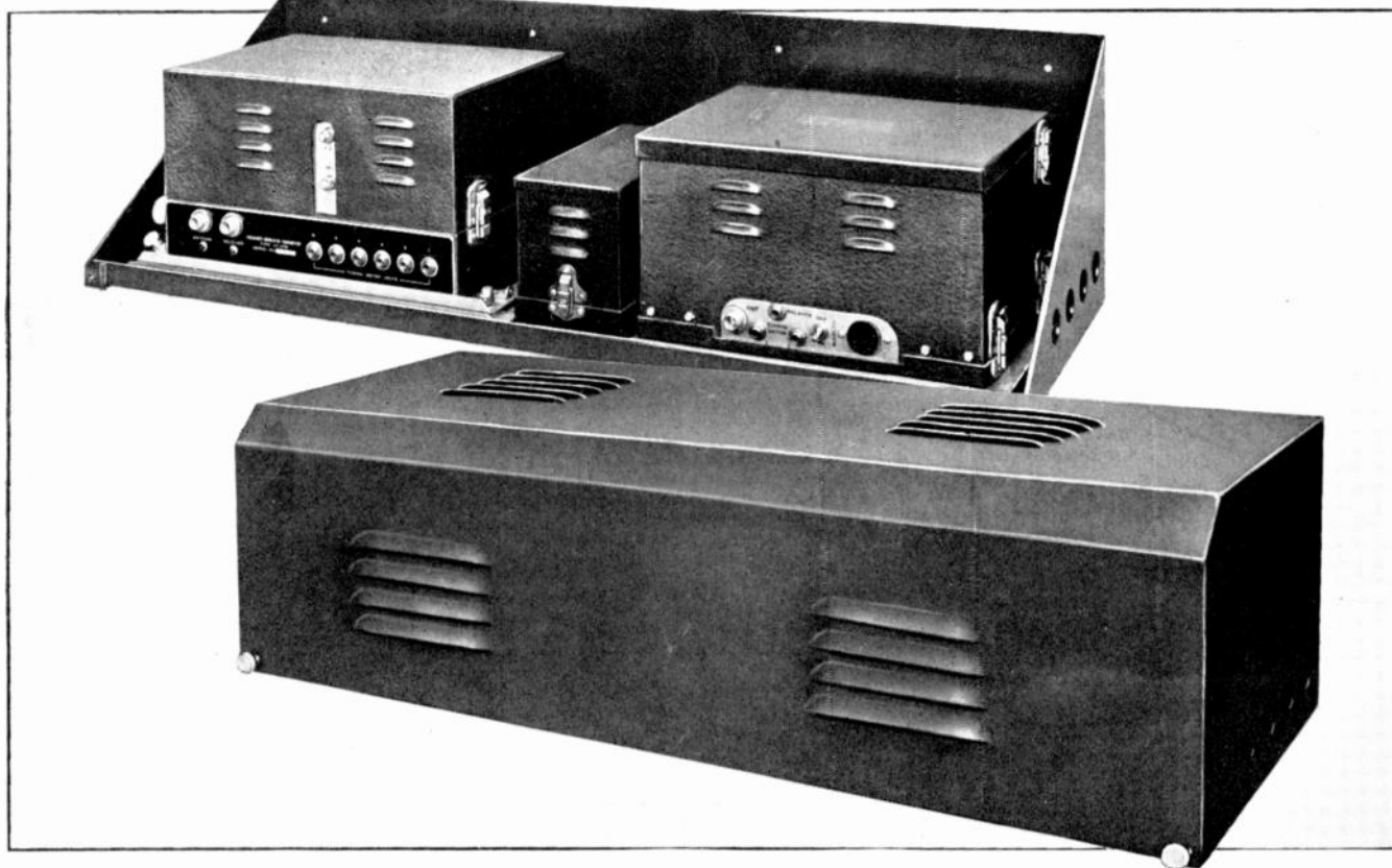
FIG. 6. MOBILE FM EQUIPMENT IS MOUNTED IN A STEEL CABINET. LEFT TO RIGHT ARE THE TRANSMITTER, POWER SUPPLY, AND RECEIVER. CURRENT IS FURNISHED BY STORAGE BATTERY ON STEAM OR DIESEL-ELECTRIC LOCOMOTIVE
