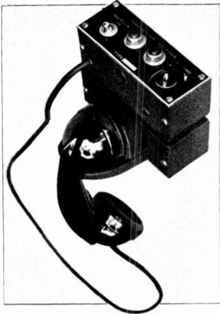
FIG. 7. HAND SET AND CONTROL UNIT FOR FM RADIO LOCOMOTIVE INSTALLATION
