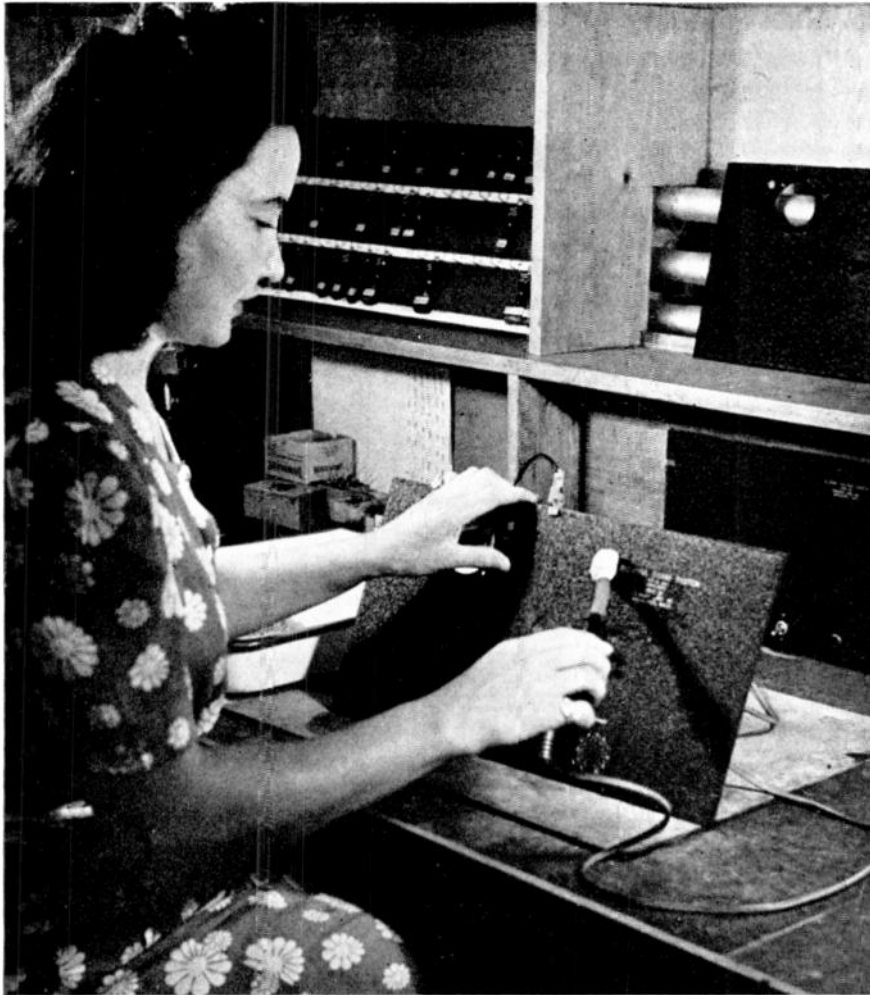
CADMIUM PLATING PROTECTS LETTERS ENGRAVED THROUGH WRINKLE FINISH
