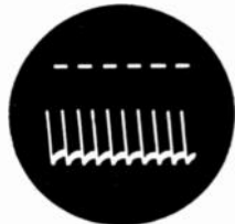
Oscillogram showing the precise wave form of the DuMont Variable-Frequency Stimulator for brain surgery and research. The remarkable uniformity of wave form and amplitude of the stimuli, is clearly disclosed here. Time interval: 1 millisecond.
