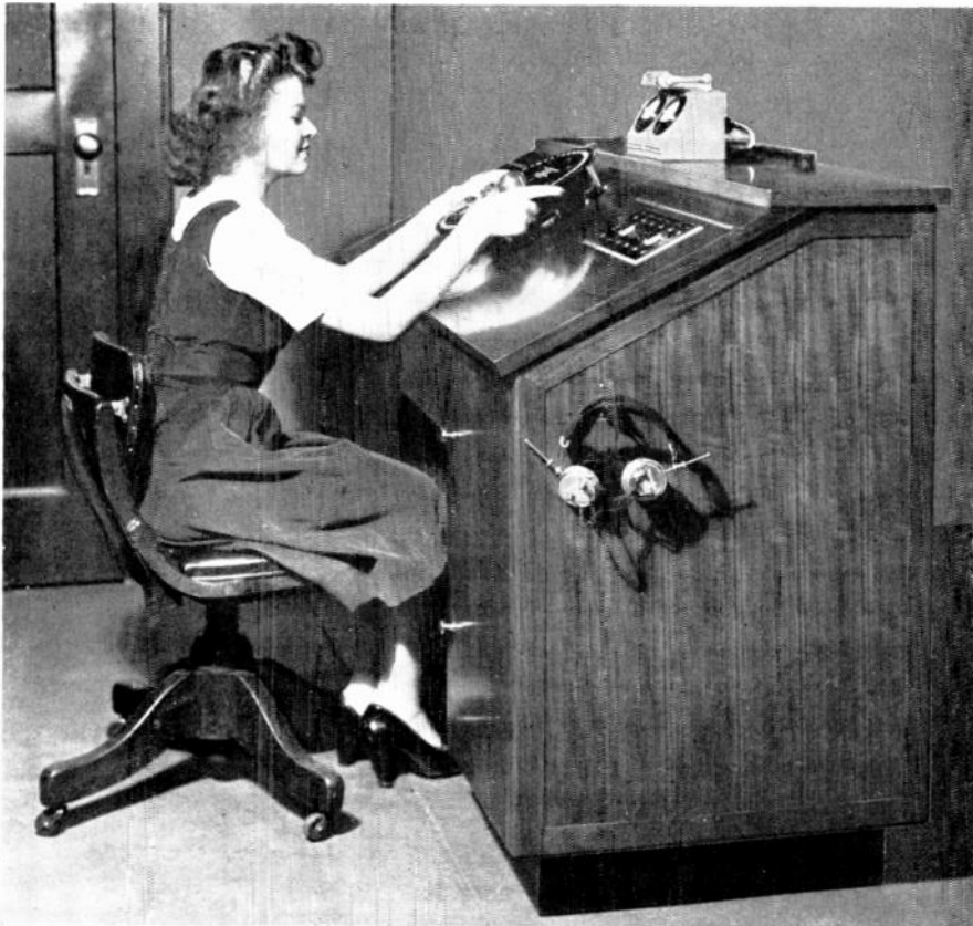
FIG. 2. OPERATOR CALLS OUT READINGS TO RECORDER, AND WATCHES THERMOMETER
