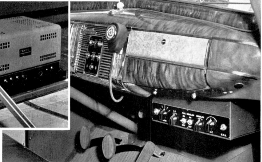
FIG. 3. ABOVE, TRANSMITTER AND ANTENNA INSTALLED IN A STATION WAGON. FIG. 4, RIGHT, CONTROL PANEL, MICROPHONE AND RECEIVER MOUNTED ON THE DASH BOARD
