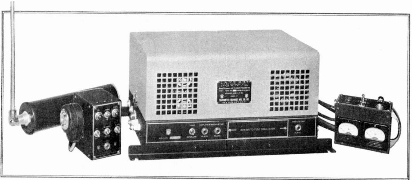
FIG. 5. THE ANTENNA AND LOADING COIL, CONTROL BOX AND MICROPHONE, 2-FREQUENCY TRANSMITTER, AND TEST SET
