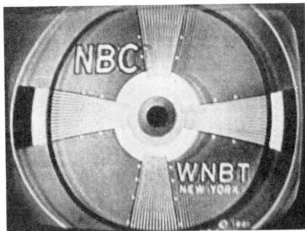
FIG. 12. GHOST DUE TO MULTIPATH DISTORTION FROM A REFLECTING OBJECT ONE-EIGHTH MILE FROM THE RECEIVER
