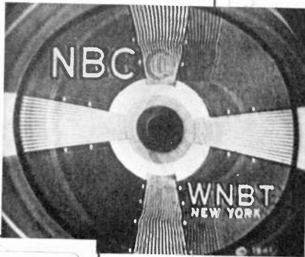
FIG. 10, BELOW. IN THIS CASE THE REFLECTION IS FROM AN OBJECT NEAR THE TRANSMITTER. THIS ALSO CAUSES A FIXED GHOST AT THE RECEIVER. FIG. 12A, RIGHT. ACTUAL PHOTO OF A FIXED GHOST, DISPLACED TO RIGHT OF MAIN PATTERN
