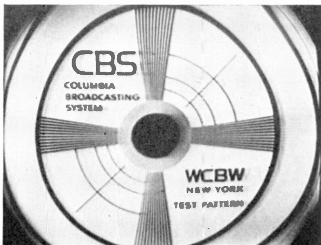
FIG. 30. CHANNEL NO. 2 TEST PATTERN AS RECEIVED ON PREWAR TELEVISION RECEIVER OPERATED AT AVERAGE LOCATION
