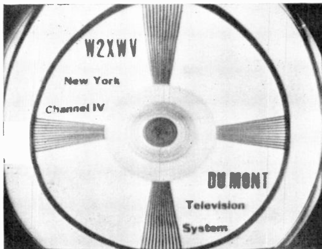
FIG. 31. CHANNEL NO. 4 TEST PATTERN AS RECEIVED ON PREWAR TELEVISION RECEIVER OPERATED AT AVERAGE LOCATION
