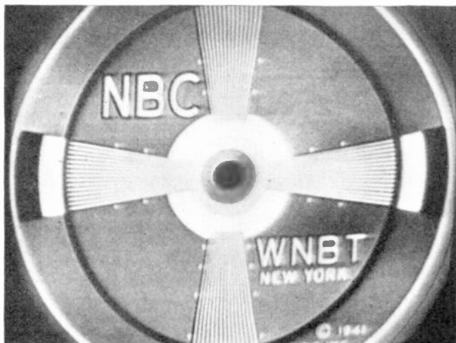
FIG. 29. CHANNEL NO. 1 TEST PATTERN AS RECEIVED ON PREWAR TELEVISION SET OPERATED AT AVERAGE LOCATION
