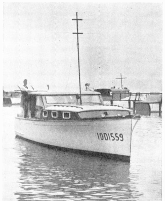
FIG. 5. THE HURRICANE II WITH THE DOUBLE DIPOLE EMPLOYED BY AUTHORS TO OBTAIN RECEPTION DATA PRESENTED HERE
