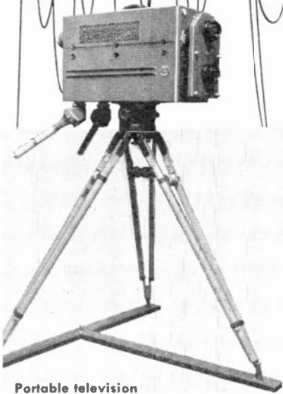
Portable television camera developed by RCA engineers. An improved version of earlier models, this camera uses an orthicon-type pickup tube; has a built-in view finder and focusing device.
