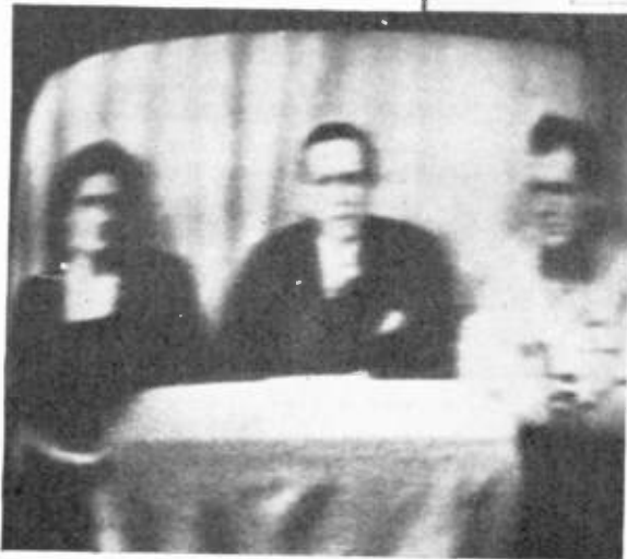
Type C — Racing Ghost ★ The appearance on the screen for the racing ghost is a main image of good intensity with ghost patterns of relatively weak intensity which appear to travel rapidly across the main image when the receiver is in motion.
